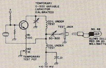
Fig. 24. Oscillator test setup.
