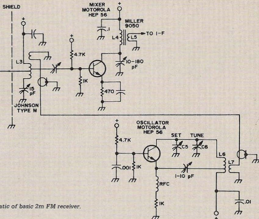
Fig. 6. Schematic of basic 2m FM receiver.
