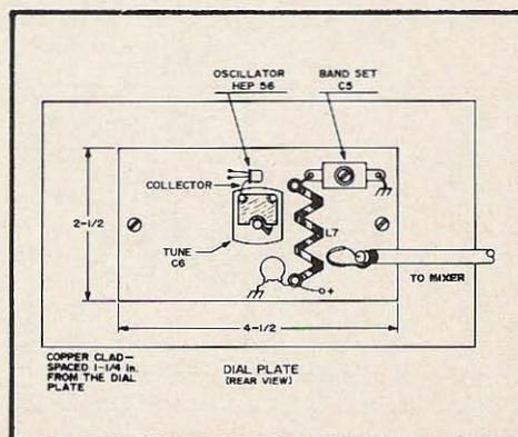
Fig. 7. Dial-mounted local oscillator
