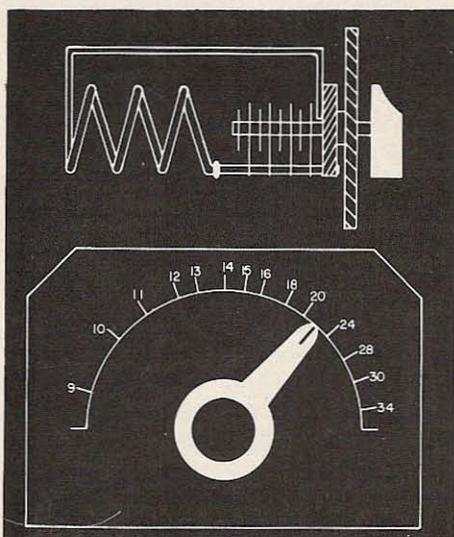
Fig. 1. Typical absorption wavemeter.
