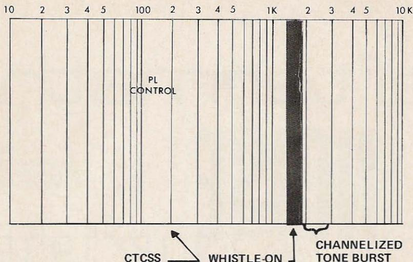
Fig. 1. Audio spectrum showing tone allocations.
