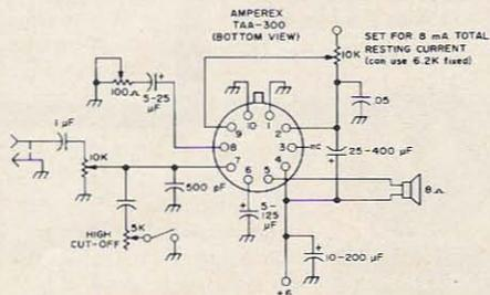
Fig. 13. Audio amplifier IC.
