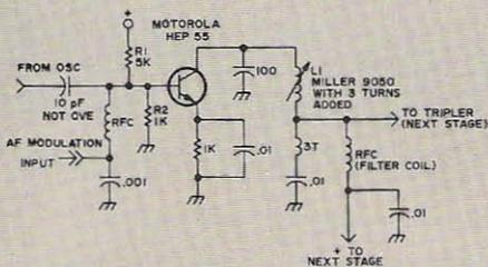
Fig. 25. Schematic of phase modulator/amplifier.
