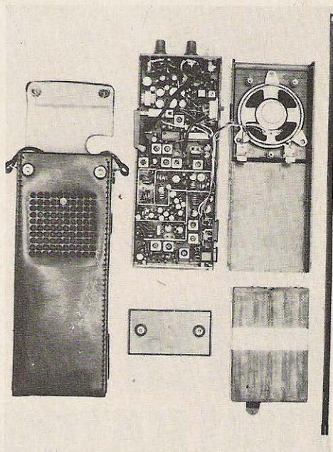
The stages of the HT-2 are isolated from one another by thin shielded partitions. The "guts" can be removed easily from the transceiver housing for service in the unlikely event that such action might be necessary.
