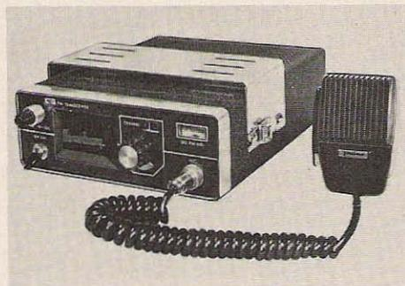
*Drake's Marker Luxury is designed as a mobile/base station. An integral supply allows connection to 115V primary power; the supply is bypassed when the unit is connected to a car battery. The Drake unit has a back-lighted channel indicator and an illuminated meter. Crystal positions are provided for 12 each, transmit and receive. Each crystal has an adjacent micro trimmer. Though rated at 15W output, typical Marker Luxury units approach the 20W mark.*
