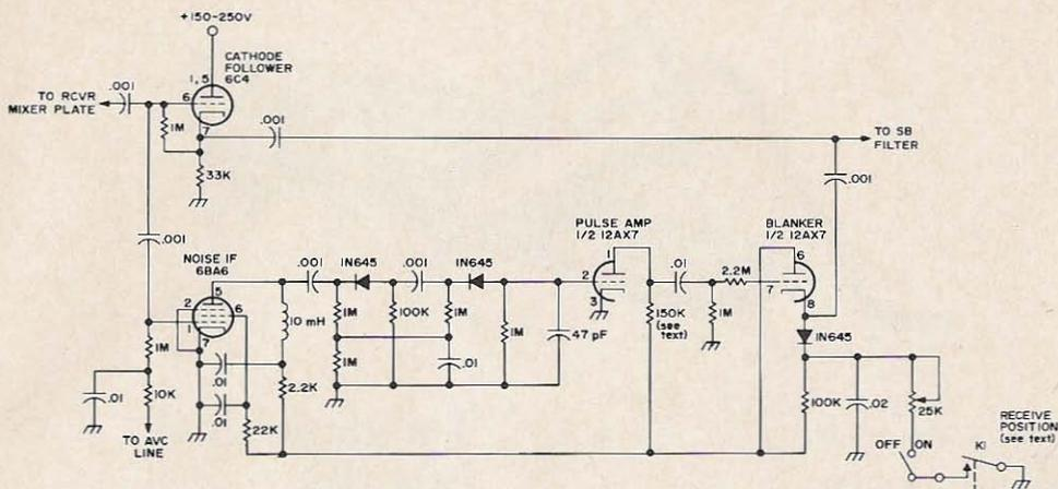
Fig. 1. Revised schematic of the noise blanker that really works!
