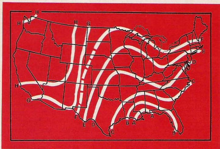
Fig. 3. The contours of this map are for fixed transmission outage time and can generally be used in conjunction with the curves of Fig. 4 to predict the effect of rainfall on path reliability.
