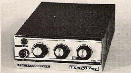
The Tempo FM-V import offers an unusual buy in terms of performance-per-dollar-of-investment. At \$225, the unit will produce up to 15W of rf, and offers sensitivity, selectivity, and noise immunity comparable to the highest priced transceivers. Though the FM-V has no panel meter, it does contain an internal meter socket that allows monitoring of all stages, including discriminator.
