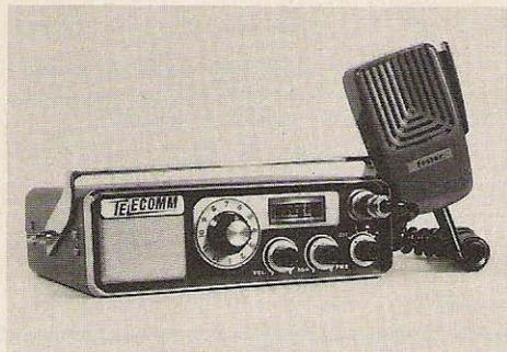
Telecomm, a California company, imports the 10W unit pictured here, but stocks the integral modules as well. The module boards include the receiver, transmitter, and rf power amplifier. The Telecomm has 12 transmit and receive crystal positions, a front-mounted speaker, and three switch-controlled power output levels.
