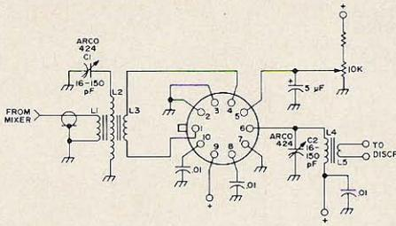
Fig. 8. 10.7 MHz i-f, bottom view of IC.
