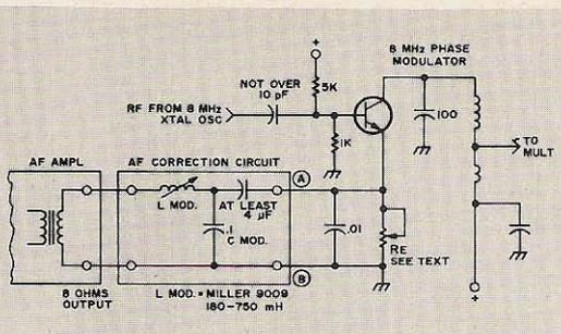
Fig. 19. Phase modulator interconnect circuitry.
