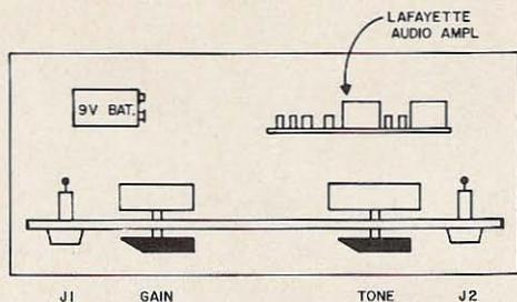
Fig. 3. Handy af assembly, top view
