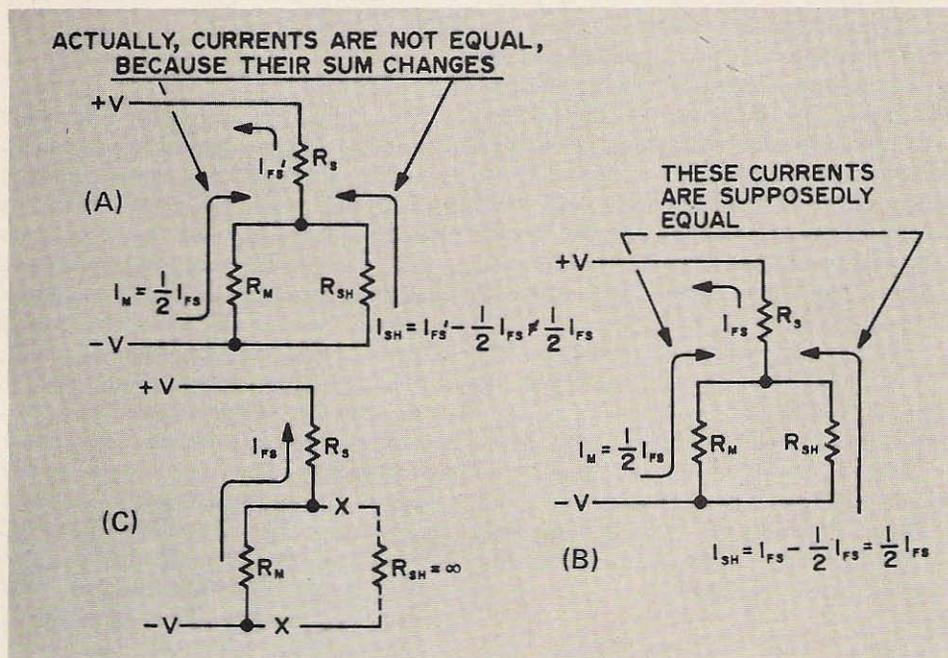
Fig. 2. The two-resistor technique. (A)  $R_{SH}$  disconnected and  $R_S$  adjusted for full-scale deflection. (B) What supposedly happens when  $R_{SH}$  is reconnected. (C) What actually happens! Note that  $I_M$  and  $I_{SH}$  are not equal if  $I_{FS}$  changes.
