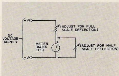
Fig. 1. Standard circuit for measuring meter resistance.
