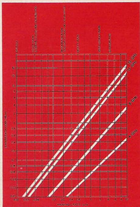
Fig. 2. Theoretical curves show how attenuation increases with rainfall rate (based on calculations by Ryde and Ryde).
