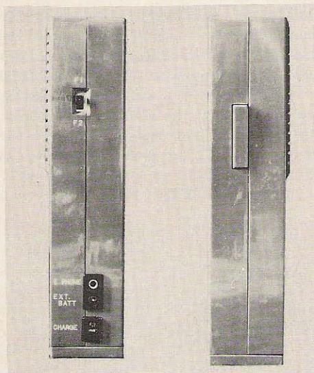
Varitronics' HT-2 is a 2-channel, 2W hand-held transceiver that comes with nicad batteries, carrying case, battery charger, and crystals for .34/.94 and .94 direct. Sensitivity of the receiver section is 0.4  $\mu$ V for 20 dB of quieting.
