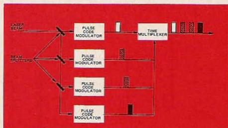
The theoretical capacity of such a system staggers the imagination. The suggested bit rate would be about  $2 \times 10^{14}$  bits per second—the equivalent of 1,920,000 video signals.
