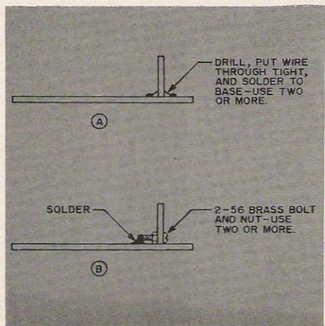
Fig. 16. Methods for fastening insulated strips to baseboard.
