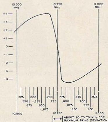
Fig. 12. Discriminator dc output curve.
