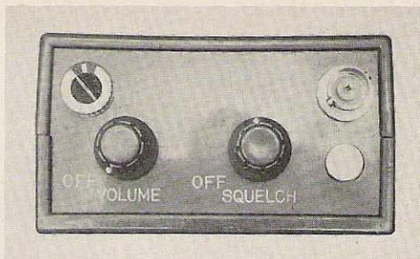
The top of the HT-2 contains on-off and volume control, squelch control, a BNC antenna connector (which also mates to the antenna supplied with the transceiver), and a battery-level indicator.
