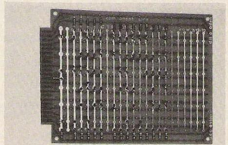
This photo of the call letter matrix board shows the layout of the diodes for W6FNO. The same board is used for other calls, though the diode placement will vary.
