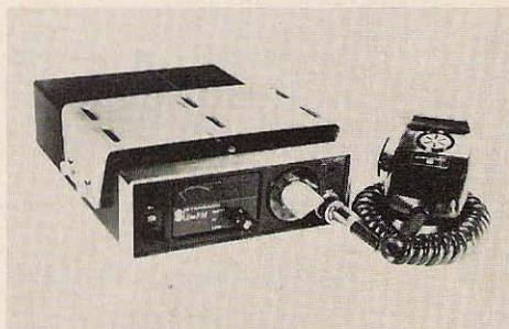
*Standard's new SR-C826M uses a beefed-up receiver borrowed from the company's type-accepted line of marine units. Among other improvements over the early Standards: more rf amplification stages and increased selectivity.*
