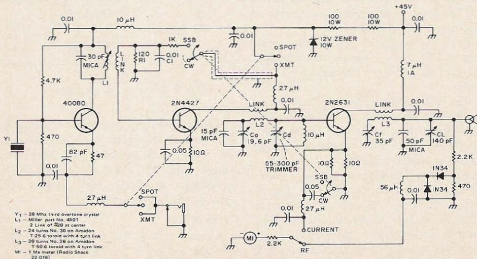
Fig. 1. Transmitter schematic.
