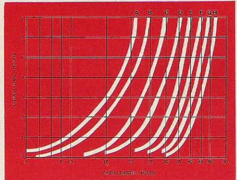
These curves, for use with the contour map of Fig. 3, are based on 11 GHz paths with 40 dB fade margins.
