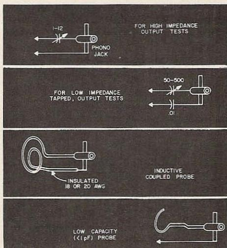
Fig. 4. Coupling methods.
