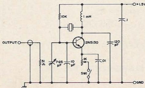
Fig. 1. Schematic diagram of the "Point Eight" Signal Source, the "poor man's Model 80."
