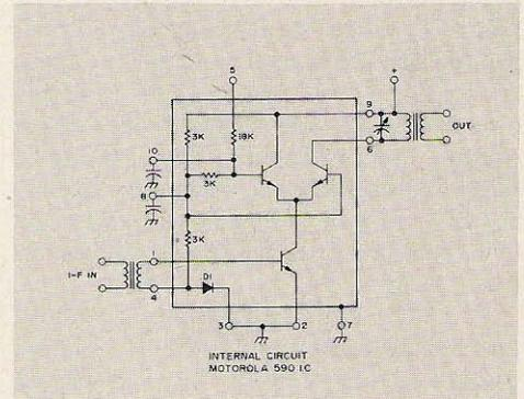
Fig. 10. Internal circuit of Motorola's HEP 590 IC.
