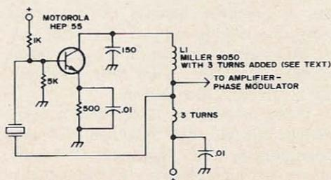
Fig. 21. 8 MHz oscillator schematic.
