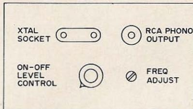
Fig. 2. Minibox layout of the signal source panel.
