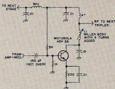
Fig. 26. 8 MHz tripler schematic.
