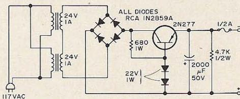
Fig. 2. Power supply schematic.
