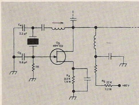
Fig. 2. FET replaces vacuum tube in the H23 oscillator to complete the transistorization operation. Components not labeled in the sketch are those components that are already part of the existing oscillator circuit.
