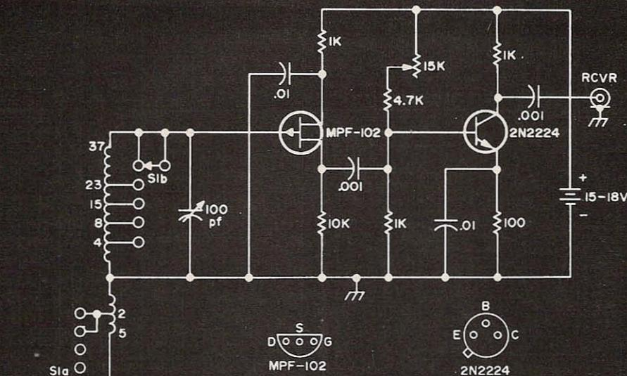
Fig. 1. Schematic of the preselector. All resistors can be quarter-watt types; capacitors should be ceramic.
