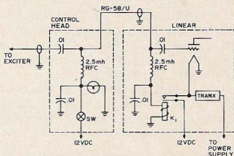
Fig. 1. Remote switching of linear amplifier.
