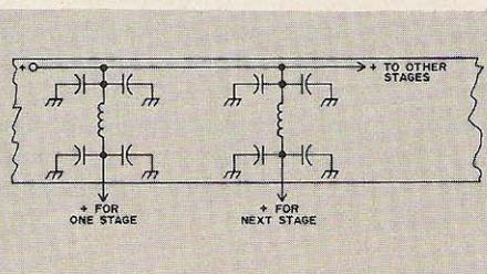
Fig. 18. UHF filters for interstage coupling.
