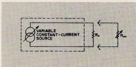
Fig. 3. A constant-current source is used to measure meter resistance.
