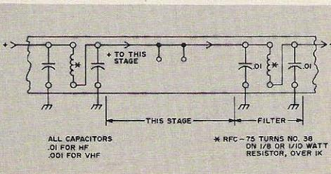
Fig. 17. Miniature filters, interstage.
