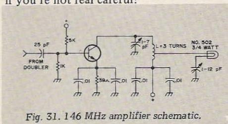
Fig. 31. 146 MHz amplifier schematic.
