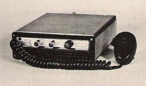
*The Simpson Model A transceiver is one of the few that have received FCC type-acceptance for operation on the adjacent marine band. This durable FM unit has removable top and bottom cover plates that give easy access to internal circuitry. Sufficient volume exists inside the housing to mount tone units or other add-on circuits.*
