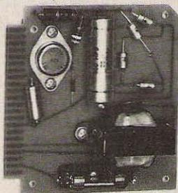
Regulated power supply module provides +3.6V to digital, identifies logic and matrix boards.
