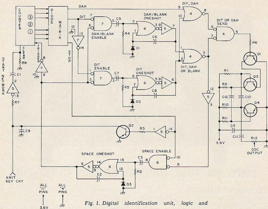
Fig. 1. Digital identification unit, logic and schematic diagram.
