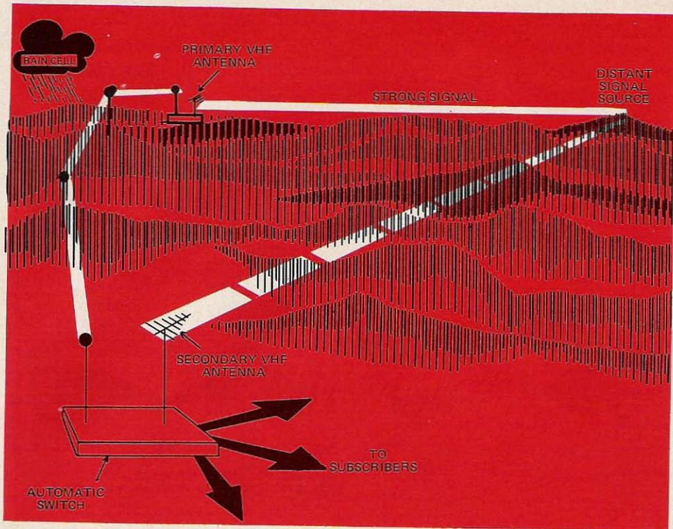
Fig. 5. Many CATV systems can use a secondary off-the-air antenna as a back-up for a microwave link.
