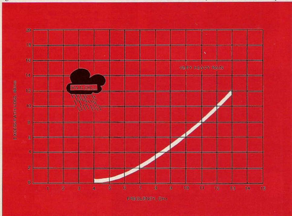
Fig. 1. Excess path loss caused by heavy rain increases rapidly with increasing frequency.
