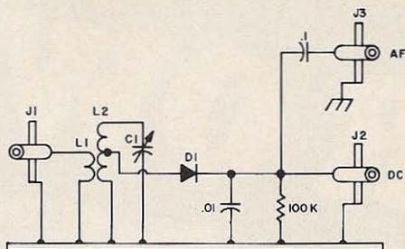
Fig. 2. Tuned diode detector.
