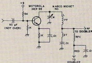
Fig. 28. 24 MHz tripler schematic.
