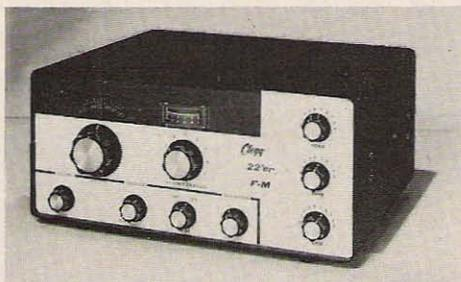
The Clegg 22'er uses vacuum tubes in the final to produce more power output than any of the available transistor rigs. The tunable receiver is calibrated to mark existing FM channels. The transmitter section is crystal-controlled, and runs approximately 35W out. The receiver section is highly selective and as sensitive as they come. Unit operates from 115V ac or 12V dc.
