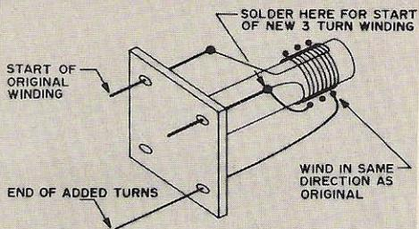
Fig. 22. Miller 9050 coil with added turns.
