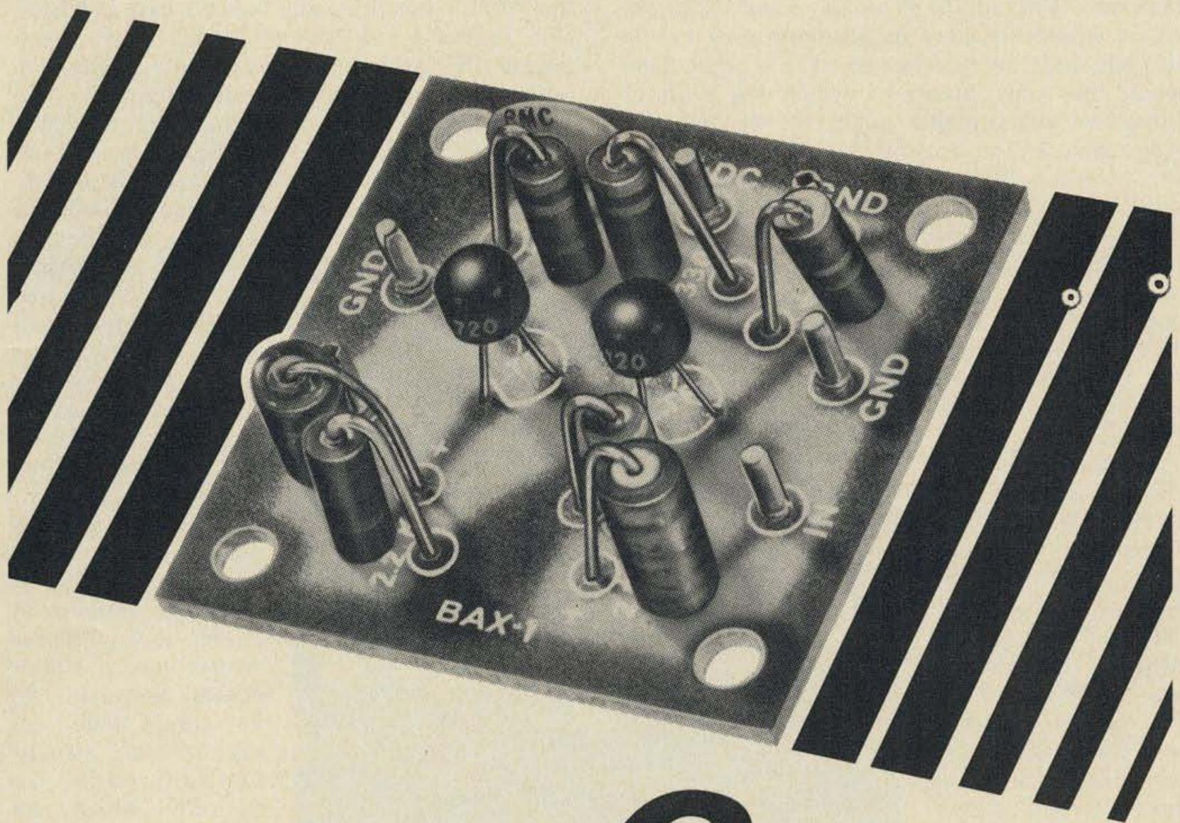
International BAX-1 Broadband Amplifier is a general purpose unit which may be used as a tuned or untuned amplifier in RF and audio application. For example: when used as untuned RF pre-amplifier connect between antenna and receiver antenna posts. Ideal for SWL, Experimenter or Amateur applications. Easy to build. Complete Kit.....\$3.75
