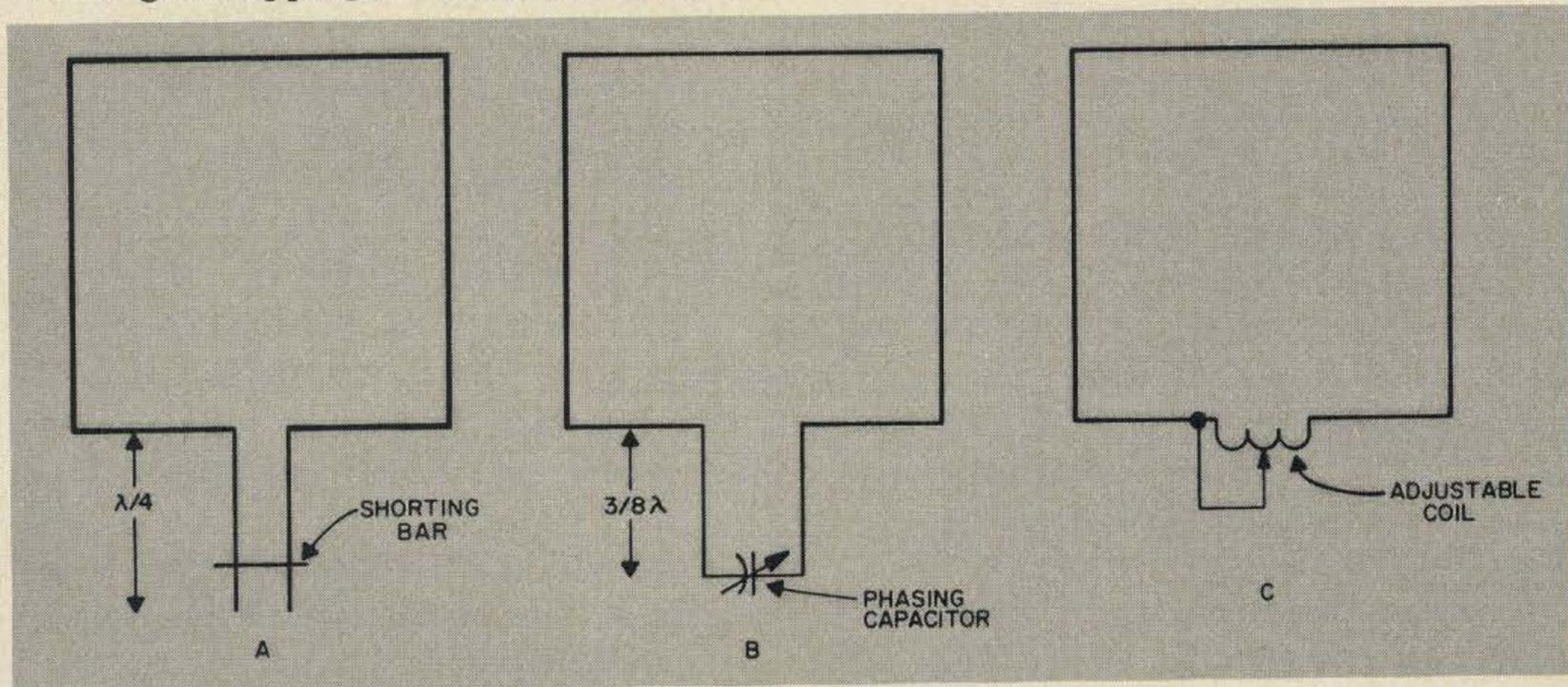
Fig. 1. Basic methods of tuning quad reflectors.
