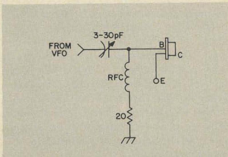
Fig. 2. Simplified input circuit, 2 watt, 6 meters. (Temporary)
