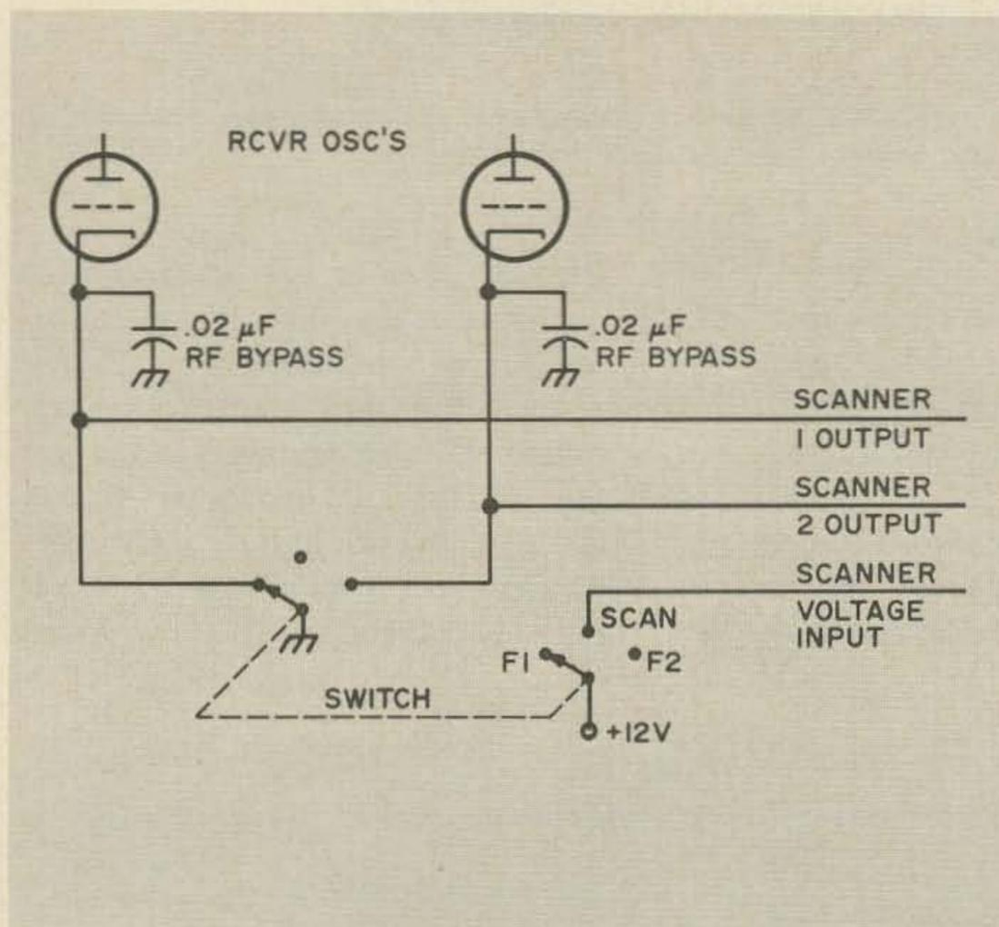
Fig. 4. This wiring diagram shows how the frequency selection is controlled. In the F1 and F2 positions, the appropriate cathode is
