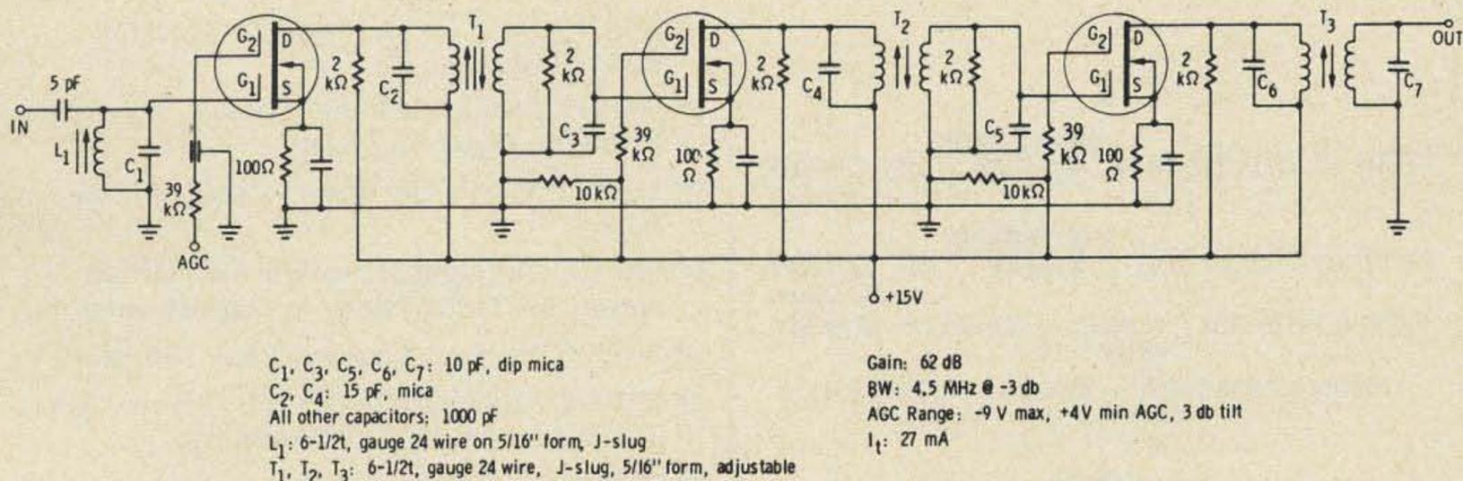
Fig. 6. 45 MHz i-f strip using the FT0601.
