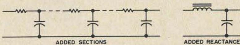
Fig. 7. When performance of simple filter of Fig. 6 is not adequate, either or both of two routes may be taken to improve it. Sections may be added (left) or additional reactances may be included (right). Usual filters encountered in practice do both; design technique is rather complicated but results justify it.
