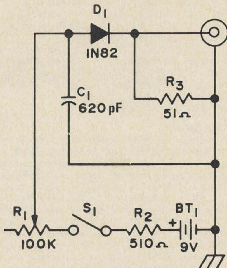
The 51Ω resistor is approximately equal to the receiver input impedance. It will take about 10 minutes to wire this up. Have fun with the noise!
