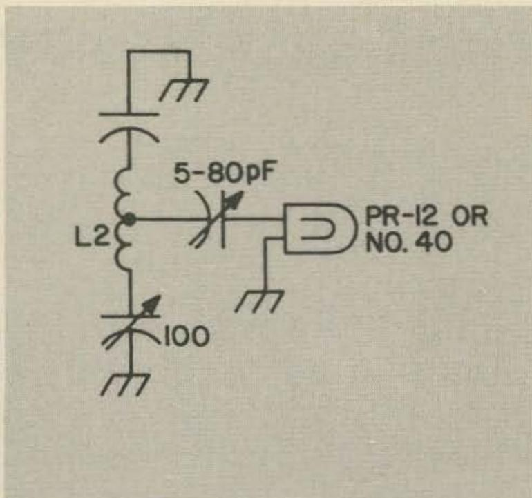
Fig. 3. Output test circuit.
