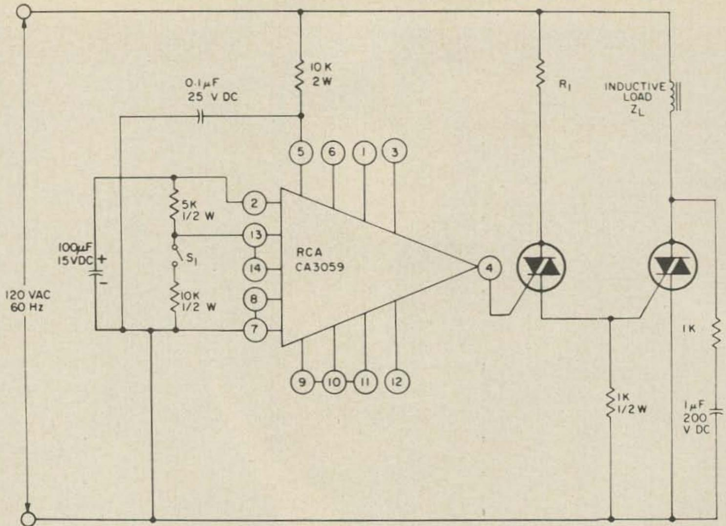
Fig. 5. Practical power switch. Heavy inductive loads can be handled by adding the 0.1  $\mu\text{F}$  capacitor and by cascading the two triacs (RCA 40526 and 2N5444). With the latter heavy-duty triac,  $R_1$  should be the highest suitable value less than 10  $k\Omega$ .
