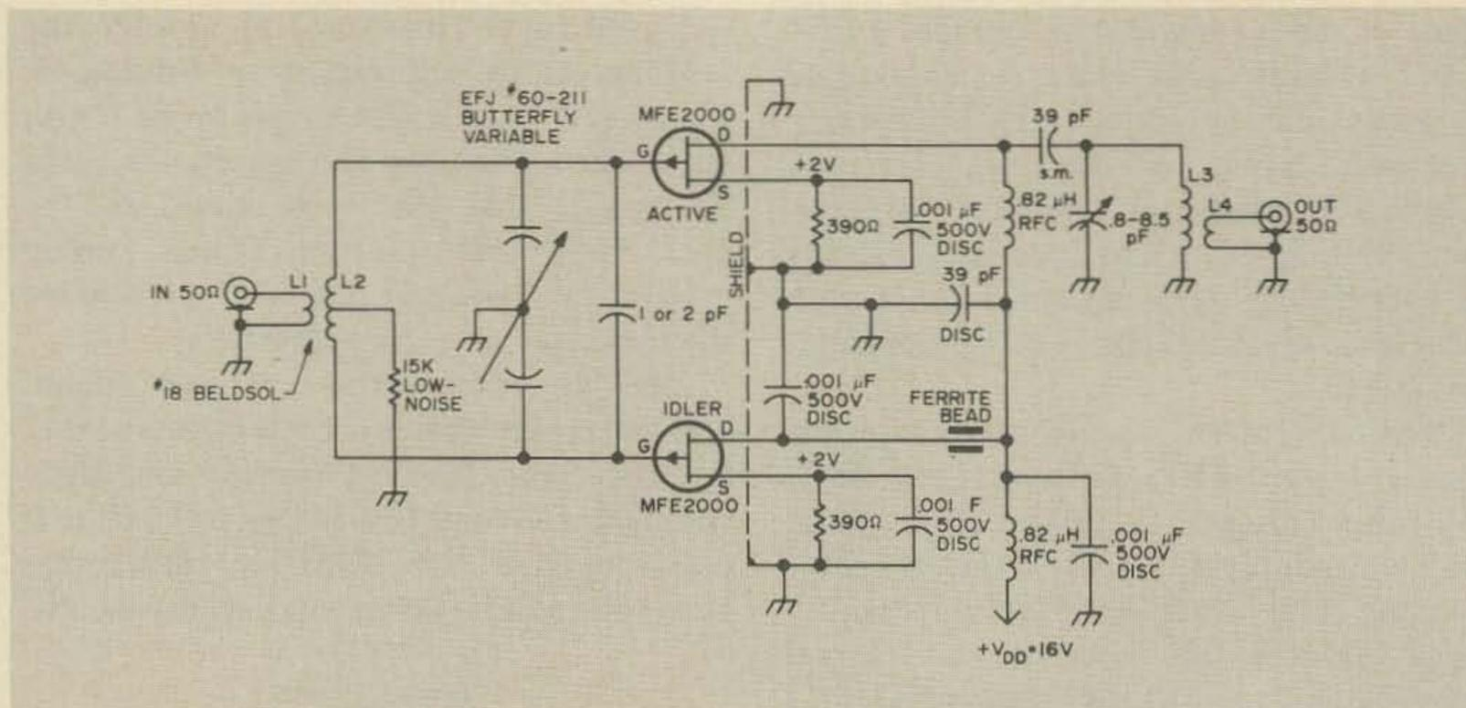
Fig. 2. Low noise J-Fet preamplifier for 2 meters.
