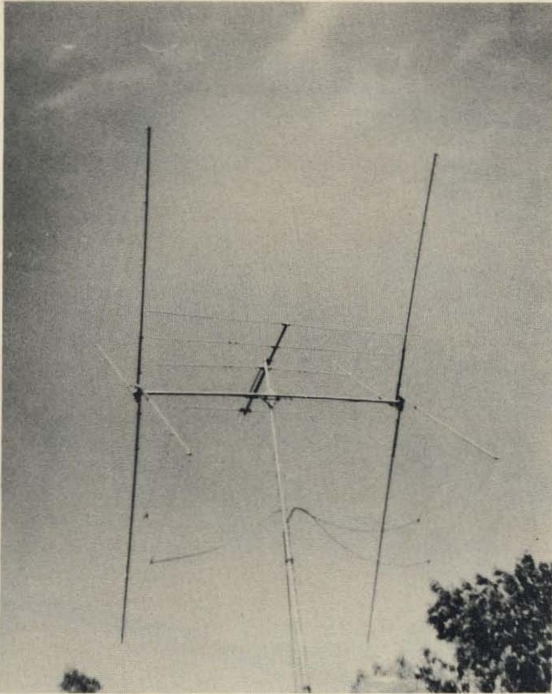
*10 and 15 meter quad with remote tuning stubs.*
