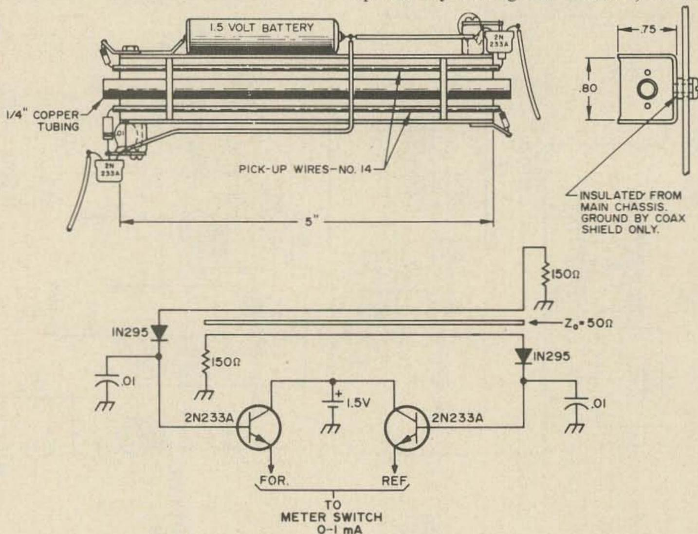
Fig. 2. Swr bridge assembly and placement data.
