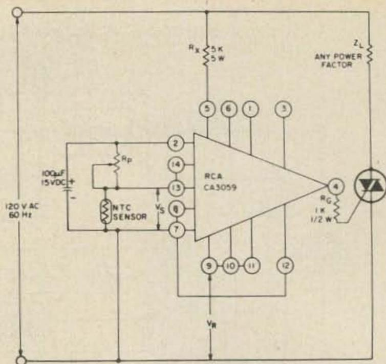
Fig. 4. Differential comparator circuit. The load is switched on when the voltage difference between  $V_S$  and  $V_R$  becomes less than 50  $\mu$ V. Note the jumper between terminals 7 and 12, which deactivates the anti-RFI feature.
