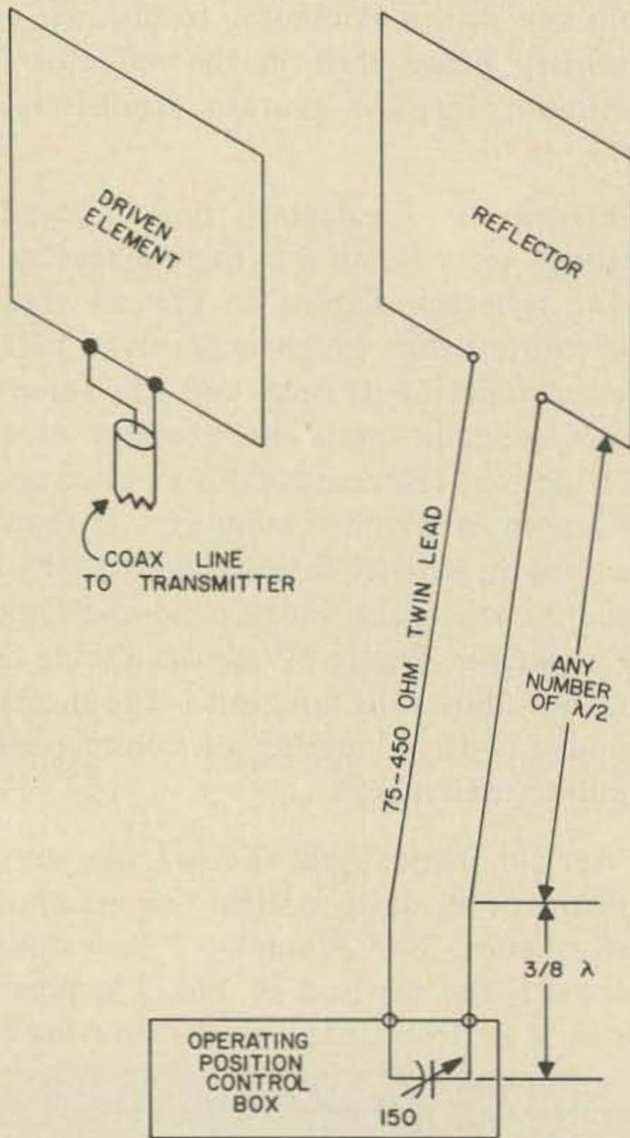
Fig. 2. Arrangement for remote tuned stub.
