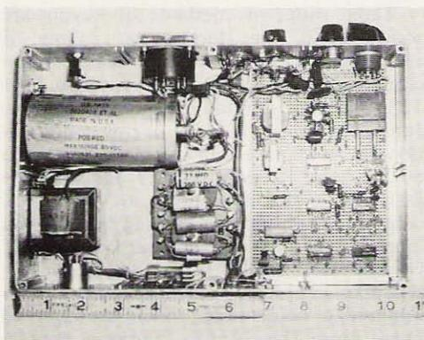
Interior bottom view. The dipplugboard was wired by a dextrous midjet. The bridge rectifier was mounted directly on the filter capacitor to avoid ground loop problems. Note heat sink on IC1.
