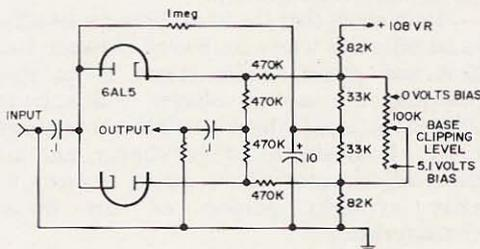
Fig. 5. Earle threshold modified for base clipping.
