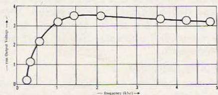
Fig. 5. Measured output voltage from buffer.
