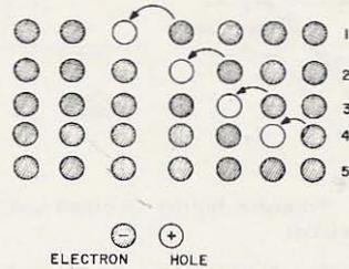
Fig. 3. Charge carrier flow.
