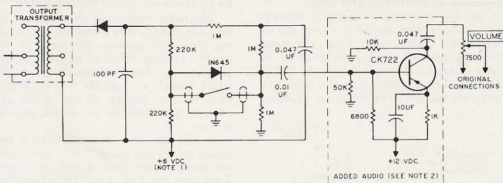
Fig. 2. Modified 2nd detector, clipper and audio. If the added audio is not required the .01 may be connected directly to the volume control.
