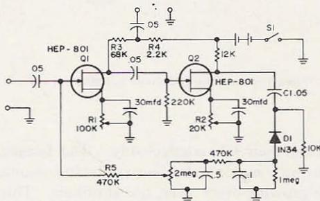
Fig. 1. Audio Compressor using two HEP-801 FETs. All resistors  $\frac{1}{2}$  watt, all capacitors are in  $\mu$ f.
