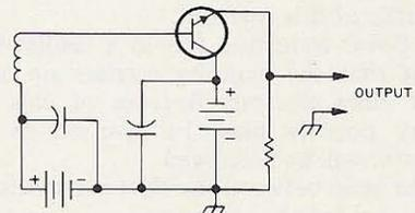
If the output of the amplifier is recoupled to the input, it is called an oscillator. This oscillator has a specific frequency which is
