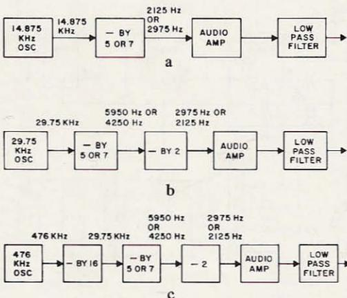
Fig. 1. Three stage evolution block diagrams.
