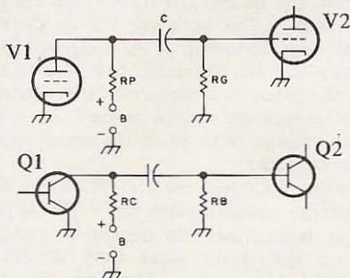
Fig. 1. Resistance Coupled amplifiers;
