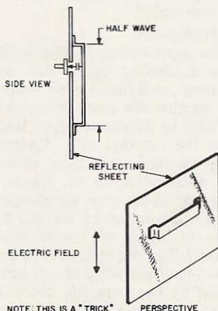
Fig. 6. Horizontal dipole which is vertically polarized.
