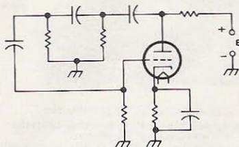
Fig. 2. Phase-shift oscillator.
