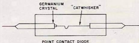
One side of the germanium is placed against one of the conductors, while the other side is attached by a fine phosphor-bronze or beryllium-copper wire nicknamed "cat whisker."
