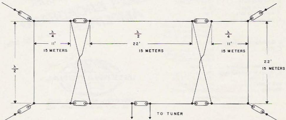
Fig. 1. Basic single section Sterba Curtain.
