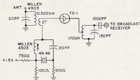
Fig. 10. 50 mhz converter for auto radio.
