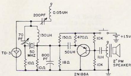
Fig. 9. 50 mhz phone transmitter.
