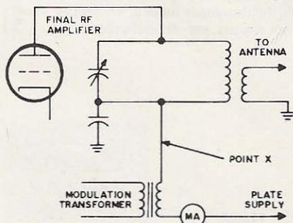
Fig. 1. At point "X" the voltage is dc plate voltage with ac modulation voltage superimposed on it.
