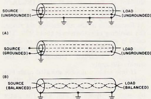
Fig. 4. Triaxial and Twinax cable shield connections.
