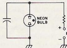
Fig. 7. Neon bulb relaxation oscillator.
