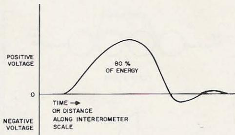
Fig. 5. Waveshape of radiation from a conducting sphere.
