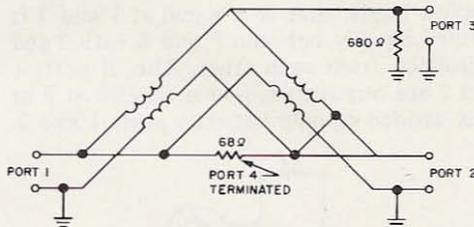
Fig. 6. Low-cost power summer/divider. Coils can be wound on 1 meg ¼ watt resistors. One device built for a special application had four turns of No. 26 wire twisted together on each form. This device had excellent characteristics over a frequency range that covered 350 to 550 mhz. To lower the frequency, simply add a few more turns. Also, better results (lower losses) can be had by using two toroid forms such as the T50-10.
