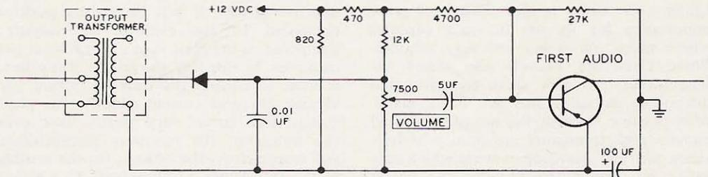
Fig. 1. Original 2nd detector and 1st audio.
