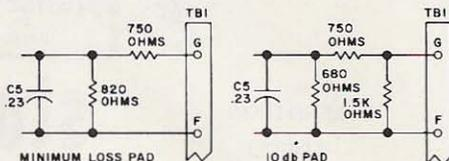
Fig. 8. Alternate output pad diagrams.
