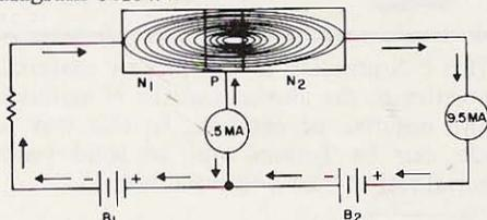
In the case of B<sub>1</sub>, the current flows from the negative pole of the battery through the current limiting resistor (if it were left out almost infinite current would flow burning out the transistor) from the end part to the P- material and through the meter which shows a small flow of current. This type biasing is called forward bias. As shown in the case of B<sub>2</sub>, a great amount of current flows as in the meter reading; this section is reversed bias.
