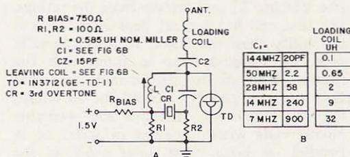
Fig. 7. Basic crystal controlled oscillator.
