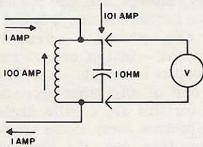
Fig. 2. Voltage drop across any single impedance in a resonant circuit is affected by  $Q$  as shown here. This circuit has  $Q$  of 100 since 1 amp of current overcomes losses to maintain 100 amps of circulating energy. If impedance of capacitor is 1 ohm, voltmeter will measure 101 volts across the capacitor, although only 1 amp is flowing in external portions of circuit. Meter impedance must, of course, be taken into account since it will load circuit and effectively reduce  $Q$ .
