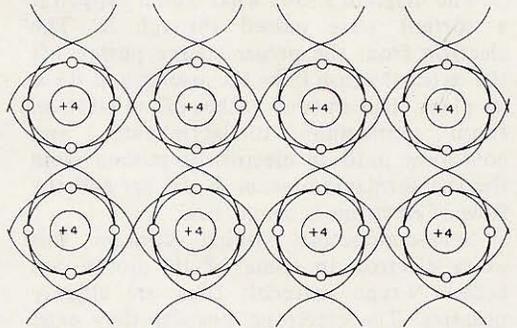
In the diagram all of the electrons go into the orbits of the other atom; however, there are never more than four electrons around an atom at one time.
