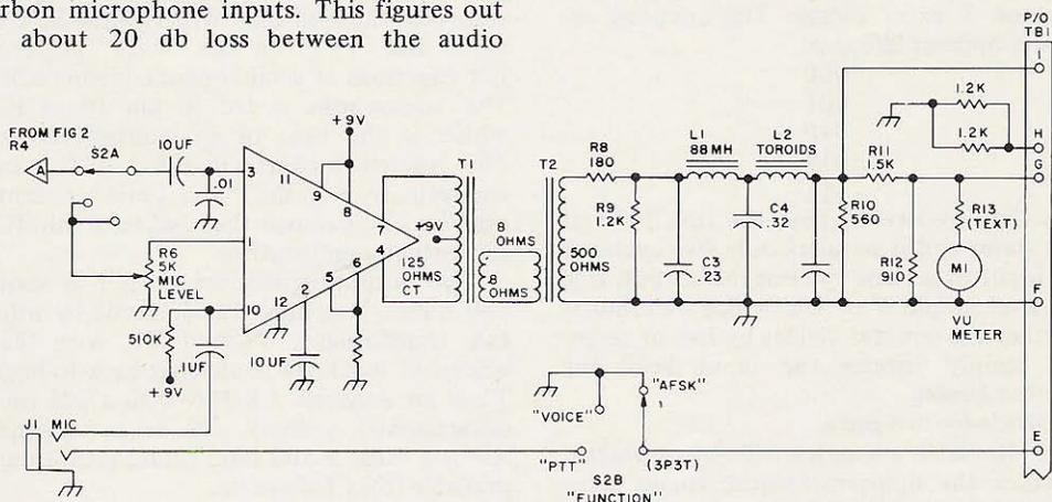
Fig. 4. Audio amplifier and output network schematic.
