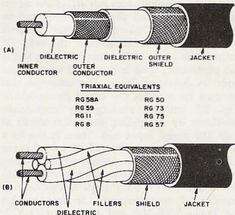
Fig. 3. Triaxial and Twinax cable construction.
