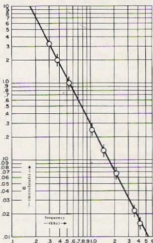
Fig. 6. Capacitance vs oscillator frequency.
