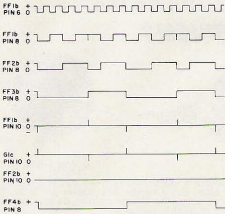
Fig. 3a. Mark condition waveforms.
