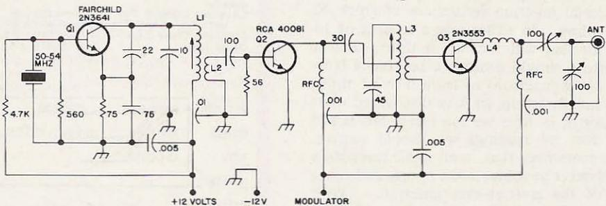
Fig. 1. Schematic of 2 1/2 watt transmitter. L1 and L2 = 6 turns # 20 On iron core 3/8" ceramic form. Links are 2 turns # 20 insulated at bottom of L1 and L2. L3 is center tapped. These coils are 'war surplus' used 'as is'. Both windings are 1/2" long. L4 = 6 turns Airdux 516 or BW 3007. Q1 = Fairchild 2N3641; Q2 = RCA 40081; Q3 = Bendix B3466 or RCA 2N3553 or 40341 (all heat-sunked).
