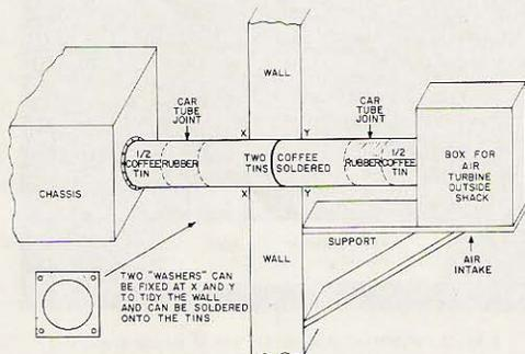
You have guessed it - it's a 3-1000Z Eimac tube which is loaned by a friend, and I dare not risk overheating it. It's a tube worth taking trouble over and a good supply of air is the least you can do for it. The air blower was mounted on brackets on the wall outside and coupled up with more inner tubing and a weather-proof roof tied on.
