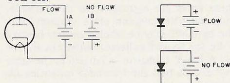
This same theory applies to the semiconductor diode. When the batteries' - pole is connected to the N part of the diode and the + pole to the P side, current flows. When the battery is reversed, no current flows because of the lack of electrons carriers in the P region. When the battery is connected forward again, both holes and electrons cross the junction, join with each other and cancel charges. This allows the electrons to enter the N side and leave the P side.
