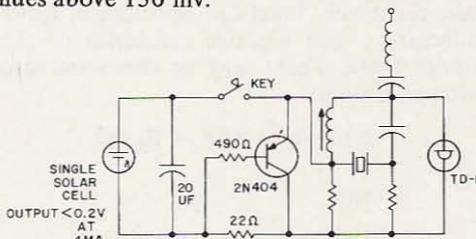
Fig. 8. Solar powered CW transmitter.
