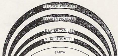
Fig. 1. Illustration of the ionospheric layers as they would appear during daylight hours.
