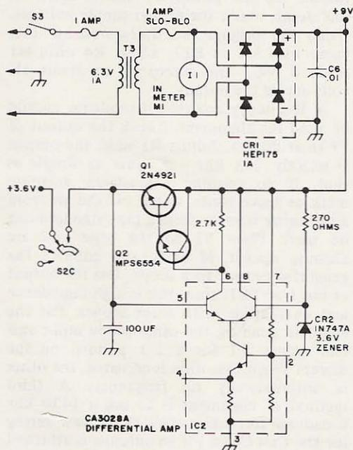
Fig. 5. Power supply schematic.
