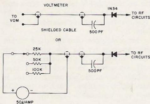
Fig. 2. Meter for finding ground loops.
