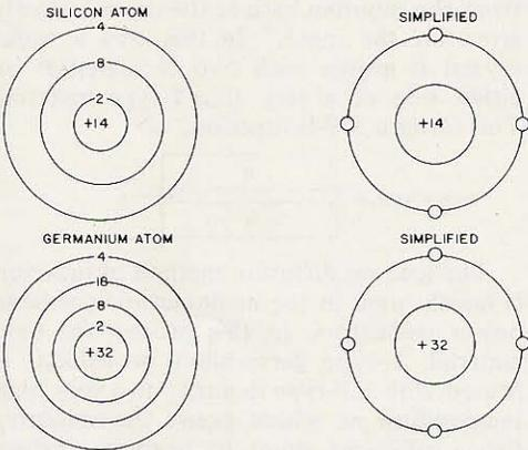
As shown in the diagram, both silicon and germanium have similar outermost shells, therefore they have almost identical properties. Silicon and germanium are in a crystal lattice which accounts for most of their conducting properties.
