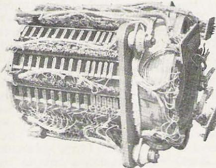
Military surplus made by HUGHES for the AF. Condition appears excellent due to being enclosed in air tight case with terminations on plug connections. 134 read/write heads, 12 heads phase adjustable timing. Integral drive motor 115 volts 400 cycle.
