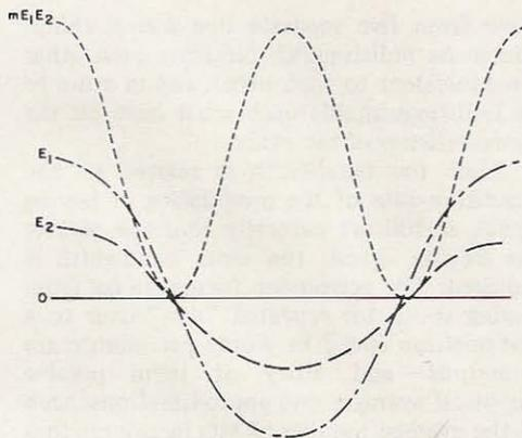
Fig. 9. Mixer action is shown here. Dotted waveform is the output signal of sample circuit, produced by multiplying two input signals E1 and E2. This plot, traced from one produced by a digital computer, extends over only one cycle and so does not show envelope variations described in text. It does, however, show how multiplication of two sine-wave signals produces a third signal which is the sum of the two original signals.
