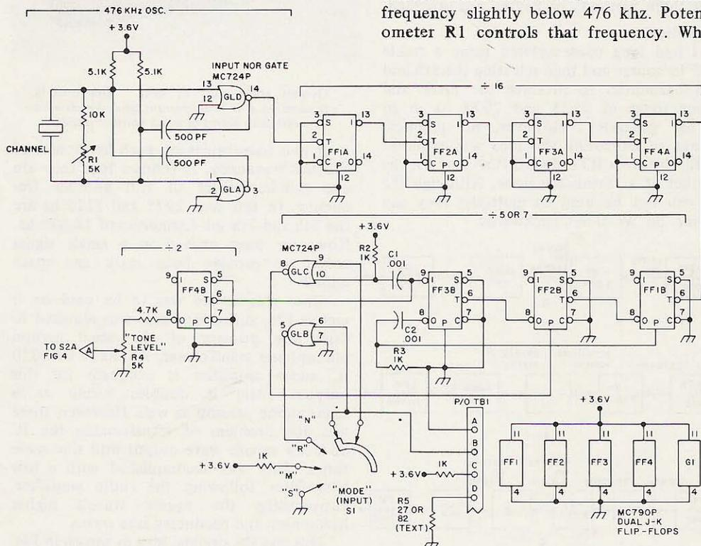
Fig. 2. Digital mark space tone generator schematic.
