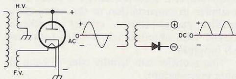
In the first circuit, a vacuum tube is used. Because of this, a filament voltage supply is needed which uses a great amount of current and also generates a great amount of heat. In the semiconductor circuit, no filament power is needed, thus no large power supply and no heat is generated. Also, semiconductor diodes are about 99% efficient. In a single
