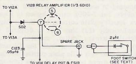
Fig. 1. Foot switch control for VOX delay.
