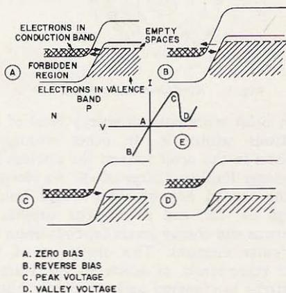
Fig. 5. Energy band diagram of tunnel diode junction.
