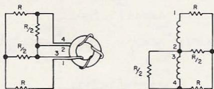
Fig. 1E. Basic hybrid or toroid Magic T. This transformer is similar to the 4:1 impedance transformer, but note that the leads are connected differently. Also, there is only 2:1 impedance ratio between 1 and 3 and 4 and 3. This is the basic device from which the power summer/divider is derived.
