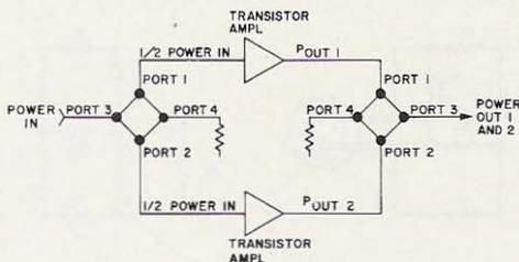
Fig. 7. Block diagram illustrating how the Magic T at the input isolates transistor amplifiers 1 and 2 from each other and from the driver. This permits them to operate independently. Their outputs are added in another Magic T at the output.
