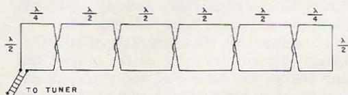
Fig. 2. Multi-section Sterba Curtain.
