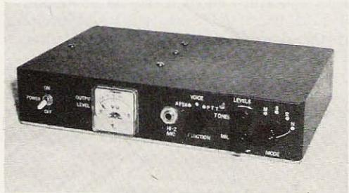
Overall angle shot of unit. The unit is housed in a cast-aluminum box which was covered with wood-grained contact paper.
