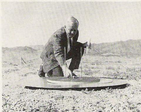
New antenna designs are tested out on 1/40th of the wavelength before the final installations are made. Here is a model of the 10 khz antenna to be built for WWVH. The model is on 400 mhz.
