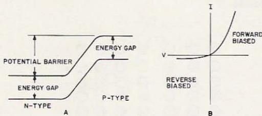
Fig. 4. Potential barrier of diode and I-V characteristics.
