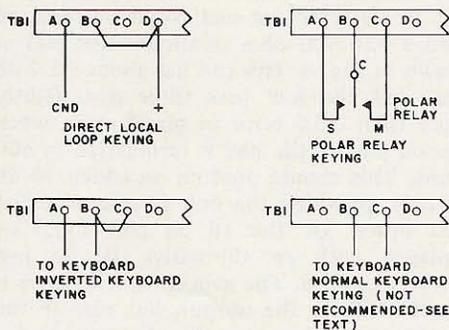
Fig. 7. Keying connection diagrams.
