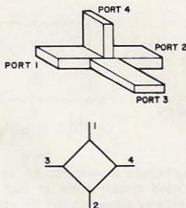
Fig. 2. Waveguide Magic T with a diagram representation.
