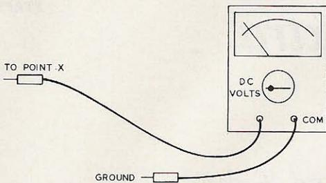
Fig. 2. Meter at dc volts.
