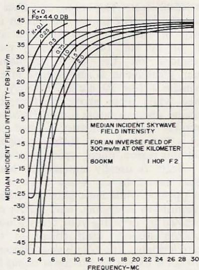
Fig. 3. A typical field-intensity graph for incident skywaves. The appropriate absorption-factor K is used to predict the received field strength in  $\mu\text{v}/\text{meter}$  (microvolts excited per meter of antenna length). The curves show the variations in received field strength for a kilowatt of rf power radiated from a dipole antenna. Corrections are required for different power outputs and antenna gains.
