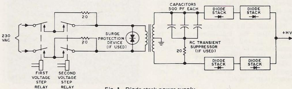
Fig. 1. Diode stack power supply.
