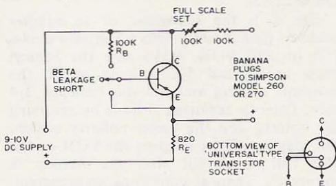
Fig. 2. This circuit will provide direct reading of transistor beta right on your VOM ohm scale. Polarities are shown for PNP type.
