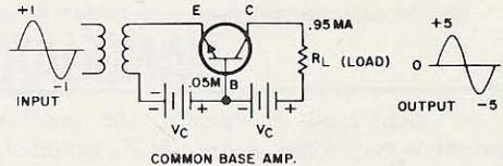
Since much more voltage may be placed on the collector of the transistor than on the emitter, more voltage and thus more amplitude is added to the input signal.
