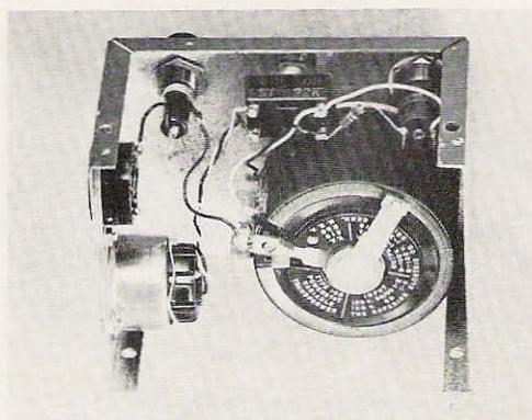
Parts layout inside the Variac box. Use plastic insulated solid wire.
