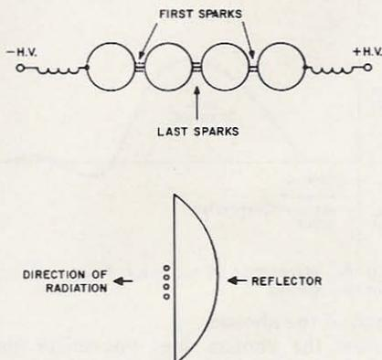
Fig. 4. One of Marconi's first radio transmitters.
