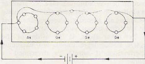
The diagram shows what would happen if a current were passed through it. The electron from the power source pushes off the extra electron from the arsenic and takes its place. This in turn pushes off an electron from germanium to germanium, and continues until an electron is pushed from the last germanium atom in the bar and the flow of electrons is completed.
