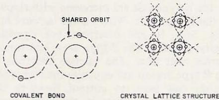
Fig. 2. Lattice structure.
