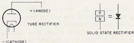
If a battery is connected across a diode, the current (which flows from - to +) will only flow in one direction. In Fig. 1A the negative of the battery is connected to the cathode and the positive to the anode or plate (see appendix). Electrons are given off from the filament and collected by the plate. However, when the battery is reversed, (Fig. 1B), the + to the cathode and the - to the anode, no current flows for the cathode does not have a surplus of electrons which it can "boil off."
