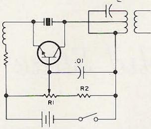
This circuit will oscillate at higher frequencies, depending upon the transistor that is used. The crystal (a quartz crystal in a case) which is connected across the collector and the emitter, keeps the oscillator resonating at a specific frequency. The crystal acts like a high Q (quality factor) series as a resonant circuit. The coil is a tuned tank circuit which also determines the resonant frequency; however, not as exactly as does the crystal.
