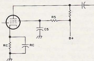
Fig. 5. Tetrode amplifier showing bypass capacitors.
