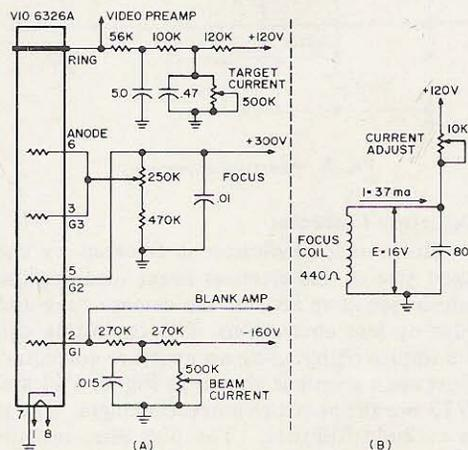
Fig. 5. Vidicon and focus coil.
