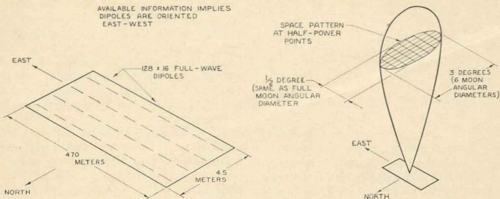
Fig. 1. The antenna system at Cambridge, just completed, which located the only four known pulsars. Electrical switching can sweep the beam lobe N-S and E-W across the sky.
