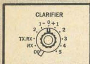
**CLARIFIER CONTROL** — Does the work of an external VFO — allows operator to vary receive frequency 10KHZ from transmit frequency, or may be used as an extra VFO combining transmit and receive functions.
