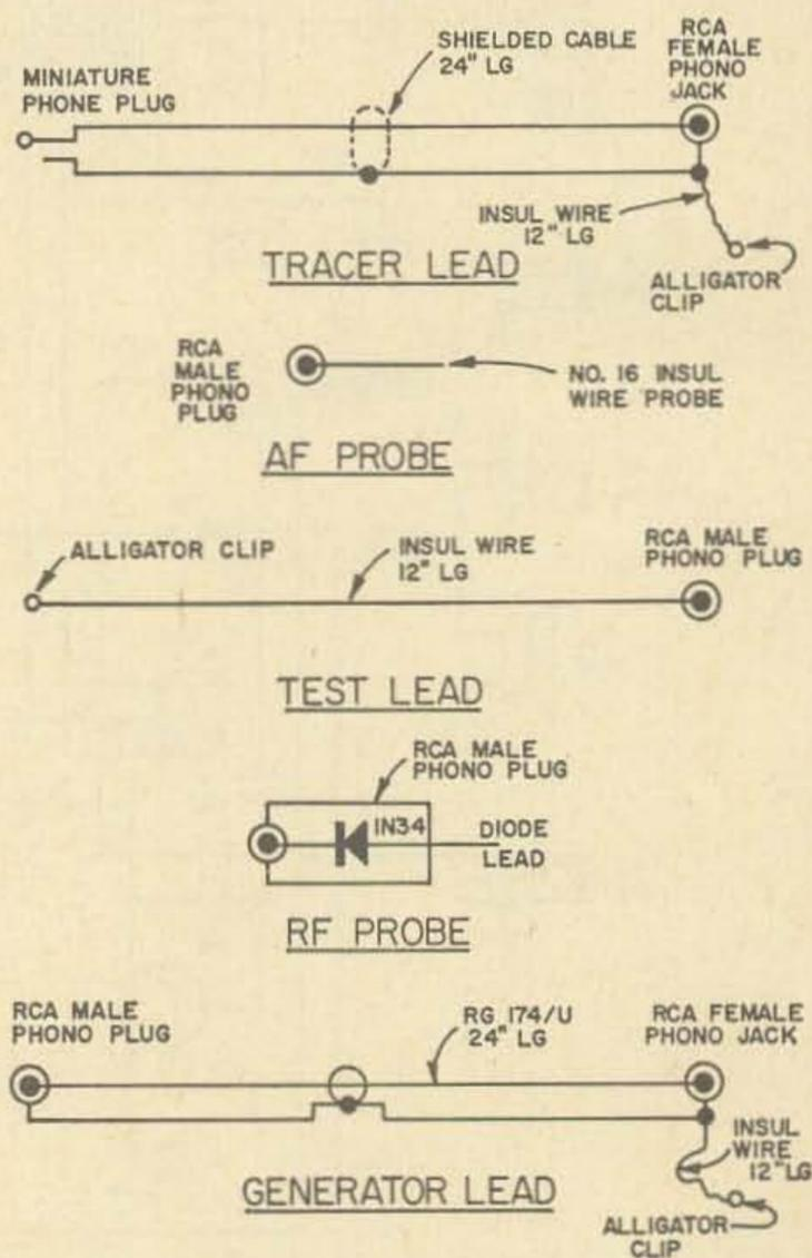
Fig. 3. Test leads and *rf* test probe construction.
