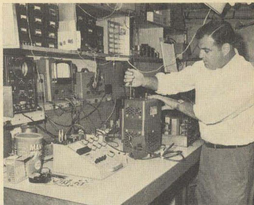
*Here Bill is removing Sola CV transformer to facilitate connection of adapter (seen with cabling attached in front of CV) for use with standard ac line plugs. Use of adapter precludes necessity for permanent installation, cable hookups, etc.*
