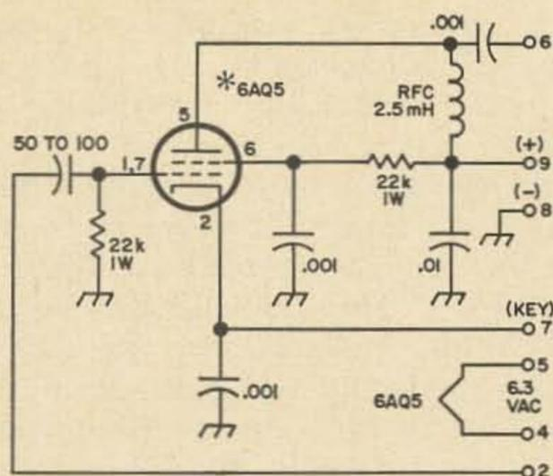
\* MOUNTED IN RIGHT ANGLE PRINTED CIRCUIT TYPE TUBE SOCKET (ELCO NO. 05-4006, 05-4007)
