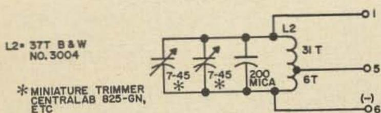
Fig. 3. The tank circuit card diagram.
