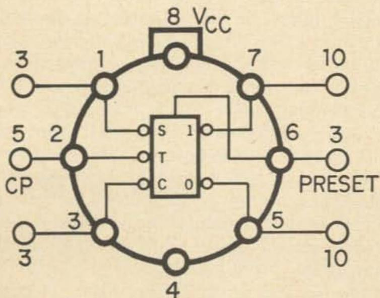
Fig. 3. The logic symbol of the uL 923.
