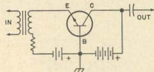
Fig. 7. Common base circuit was earliest. It has voltage gain, but no current gain. Input impedance is low and output impedance is high. Transformer input shown here can be replaced with coupling capacitor as in subsequent figures. Similarly, output load resistor can be replaced by transformer primary.
