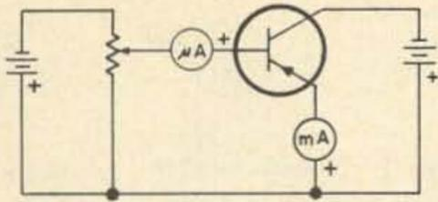
Fig. 3. Alpha factor of a transistor can be measured directly in this test set-up. Text explains technique.
