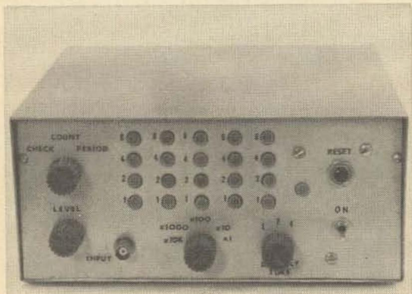
A simplified frequency counter that can be used in checking the drift of a variable frequency oscillator can be easily built at a minimum of cost thanks to the large availability of low-cost integrated circuits.
