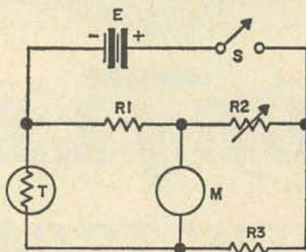
Fig. 4. Bridge type temperature measuring device.
