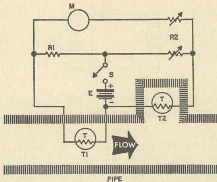
Fig. 5. Typical circuit of a flow meter to measure either liquid or gas flow.
