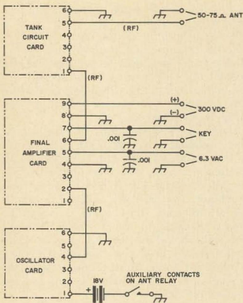
Fig. 4. Card socket wiring diagram.
