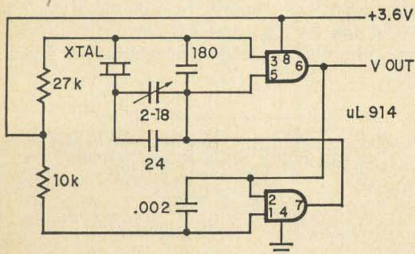
Fig. 8. The 100 kHz crystal oscillator.
