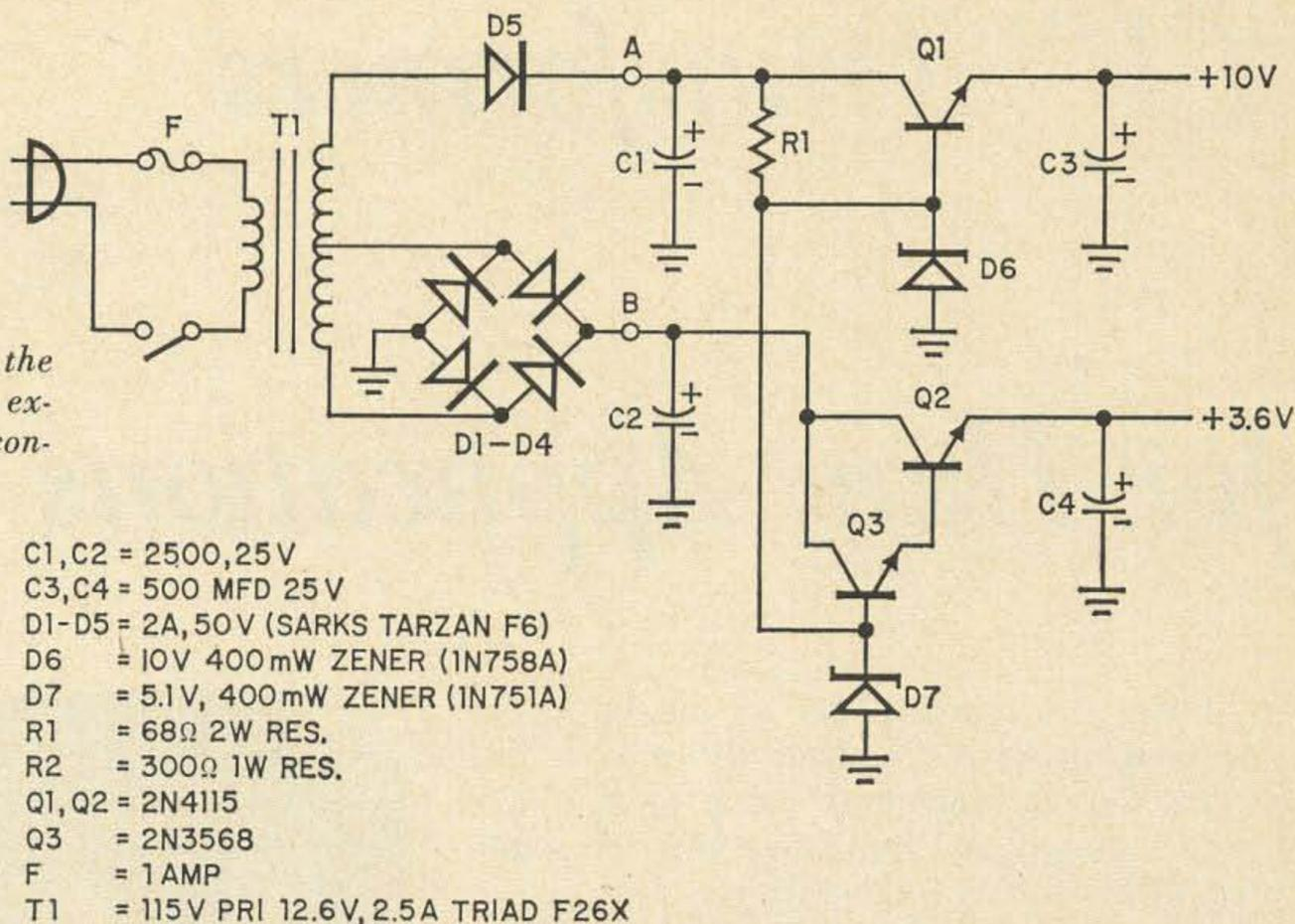
power supply is broken at points A and B and the auto battery adapter is connected to these points.
