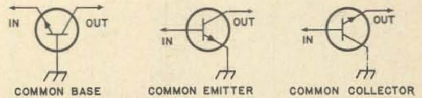
Fig. 6. The three basic transistor circuits are shown here. While all are related, characteristics of each differ from the others.
