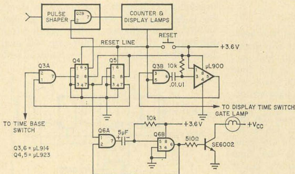
Fig. 11. Diagram of the program generator.
