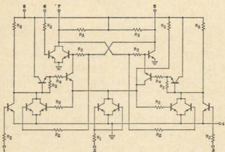
Fig. 2. The schematic of a uL 932 JK Flip-Flop.
