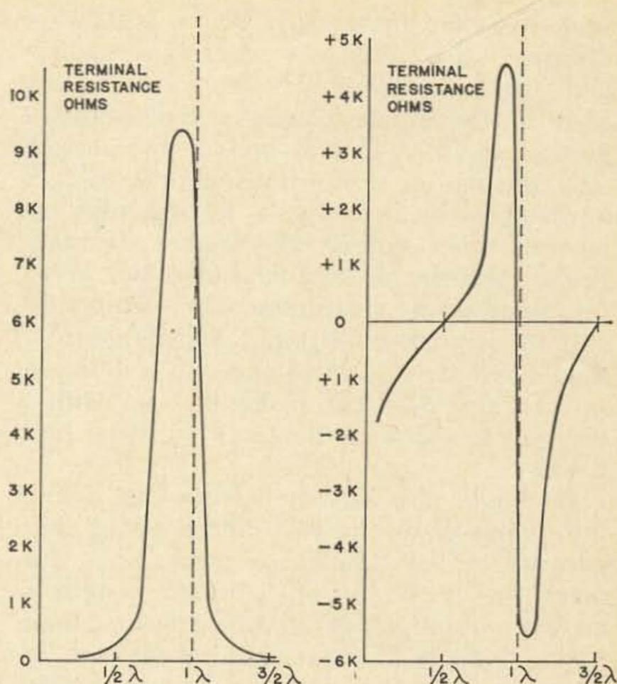
Fig. 2. Free-space resistance and reactance values for a dipole having a wire diameter of  $\lambda/100,000$  (approximately AWG #26 wire used on 40 meters). Of interest is the fact that when the dipole is an even multiple of a wavelength long (physically), resonance as defined by zero reactance actually occurs at a slightly shorter length. The curves basically repeat for longer length antennas except that the peak amplitudes slowly decrease.
