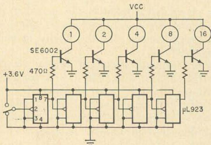
Fig. 6. Five counter modules connected together can count, hold and display a total count of 31.
