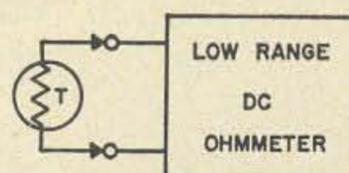
Fig. 3. The thermistor as a low current ohmmeter.
