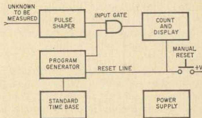
Fig. 1. Block diagram of typical frequency counter.
