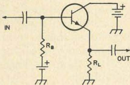
Fig. 8. This is common collector circuit. Both input and output current flows through load resistor  $R_L$  and the result is high input impedance, low output impedance. Voltage gain is less than 1, but current gain can be high.
