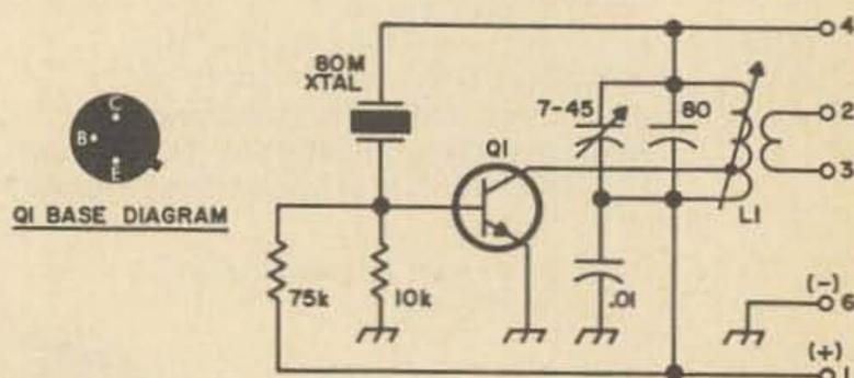
Q1 = 2W NPN 100 MHz SILICON TRANSISTOR RADIO SHACK
