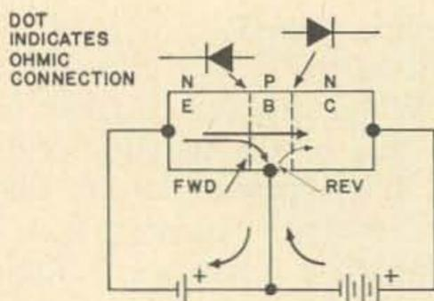
Fig. 2. Forward-biased emitter-base junction permits electron flow. Most electrons from emitter, however, pass right through the base region into the collector material, and this reduces the amount of reverse bias on the collector-base junction. The result is a variation of resistance in the collector circuit, which amounts to amplification.
