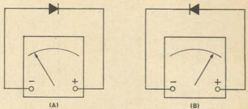
Fig. 3. Checking semiconductor diodes.
