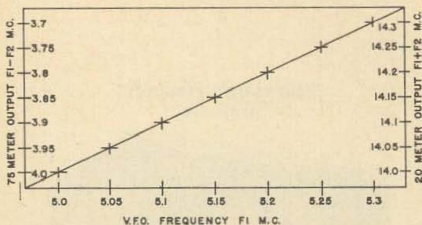
Fig. 3. Twenty and 75 meter frequency translation relationships to 5 MHz vfo.
