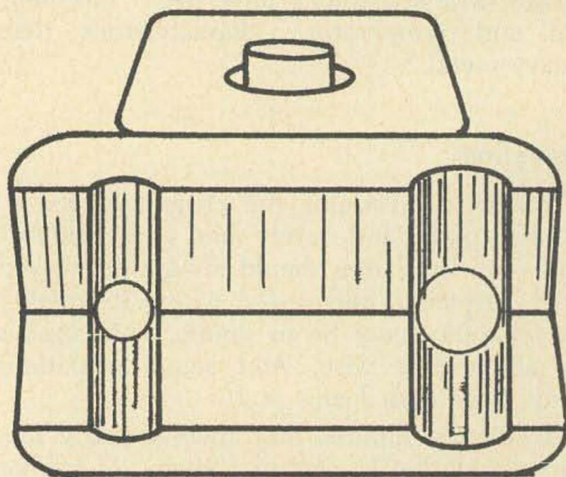
*Fig. 10. How to notch a pair of fingernail clippers to make a handy wire stripper. A post through the center of the clippers will block a notch placed there, unless very short sections of insulation are to be removed.*
