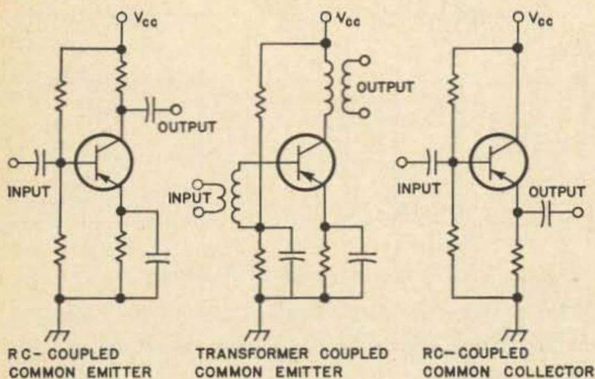
Fig. 2. Three common types of transistor amplifier circuits.
