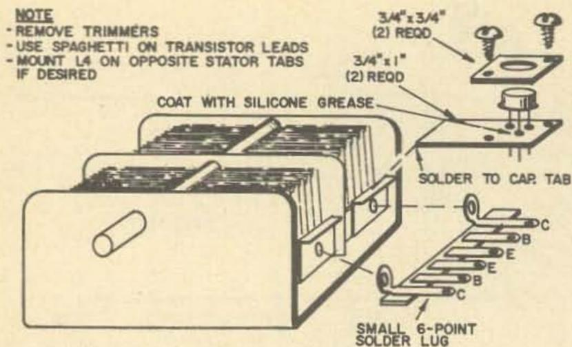
Fig. 2. Details of the heat sink.
