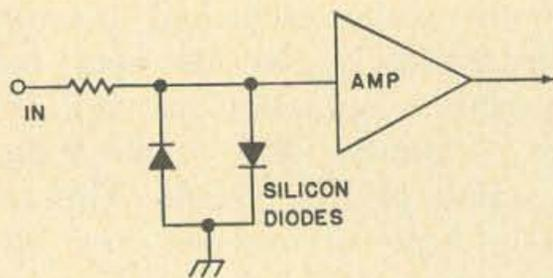
Fig. 10. Amplifier can be protected against excessive input signal voltage as shown here. Diodes are essentially open circuits at voltages less than threshold (about  $\frac{1}{2}$  volt) and have no effect on small signals. Above the threshold, diode becomes short-circuited and cuts off overvoltage signal.
