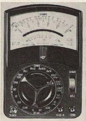
DC mA: .05, 50, 500. Decibels -20 to +62 db. Few small VOM's read up to 5000 volts, yet this is just what you need for testing your rig. 3" meter with mirror for high accuracy of readings. This meter has both the low scales and sensitivity for checking transistor circuits as well as the high ranges for transmitters. Buy one for the shack and one for the car. Light and rugged for traveling.
