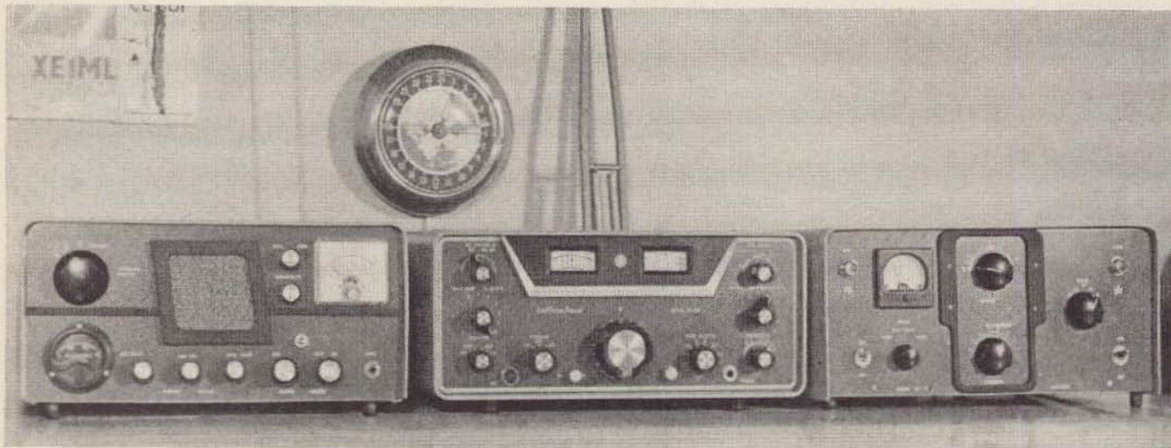
Author's setup has station accessory control unit on the left which matches SR-150 and homebrew copy of 30L-1 linear. Antenna switch is at top left and SWR meter is at top right. SR-150 plate meter is at lower left and lower knobs are for phone patch and audio compressor controls.
