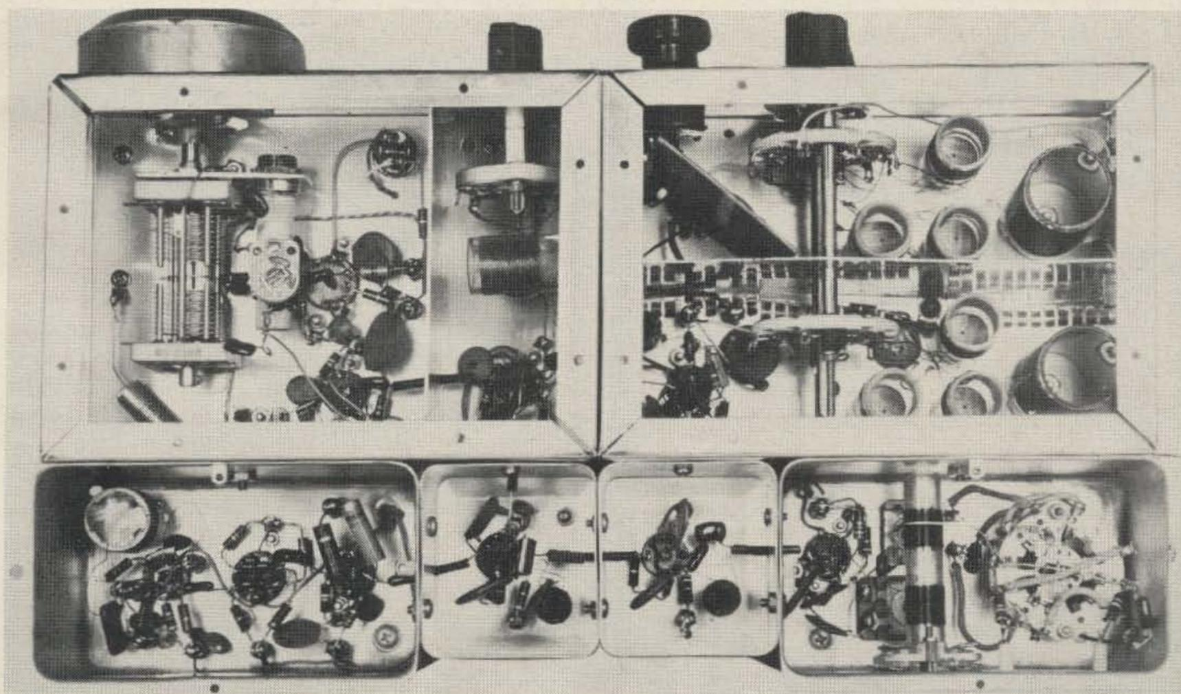
Wiring of the converter. The chassis in the upper right contains the rf amplifier circuitry. The upper left-hand chassis contains the vfo and 3.5-4.0 MHz output stage. The four small chassis on the bottom are, from the left, 1 MHz crystal-controlled reference and harmonic generator, two amplifier stages and the 1.75 MHz frequency discriminator.
