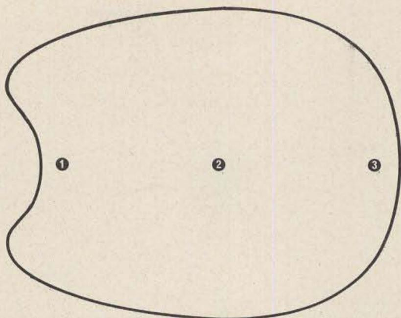
Fig. 3. Pattern of the array with 25% of the power at element 1 (0°); 50% of the power at element 2 at -90°; and 25% of the power at element 3 at -180°.
