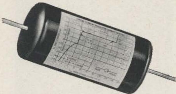
A new series of current regulating diodes covering the current range from 0.22 to 4.7 mA with 32 devices is now available from Motorola Semiconductor Products, Inc.
