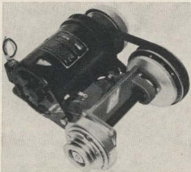
A portable alternator capable of delivering a constant power output of 2500 watts @ 115 volts, with a frequency variation of only  $\pm 2.5$  Hz has been announced by Prosser Industries, Inc. The model 2511A features an automatic transmission which compensates for input speed changes through 1800-3600 rpm to maintain a constant output of
