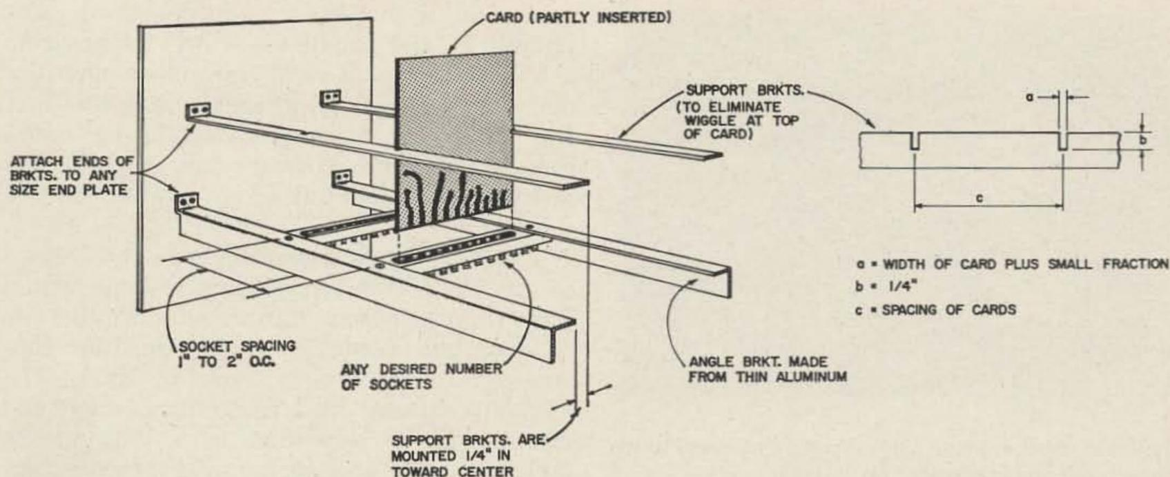
Fig. 1. Construction of a card frame to hold surplus computer cards and connectors. Although provision for only two cards is shown in this drawing, almost any practical number of cards may be held in one frame.
