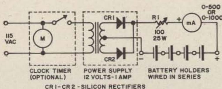
Fig. 1. Typical dry cell charging circuit. See text for discussion of circuit values.
