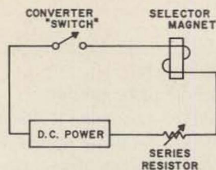
Fig. 4. Installation of the RTTY converter in the local loop to energize the printer from received RTTY signals.
