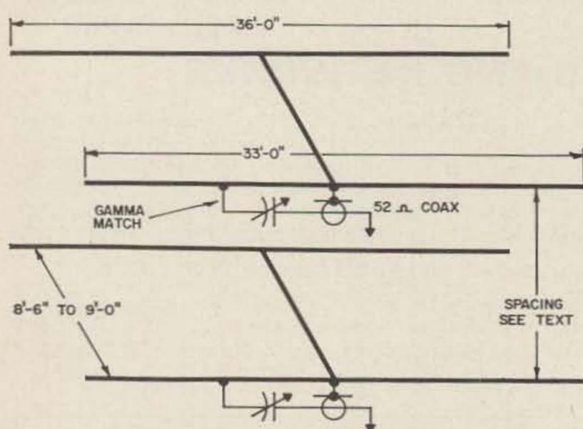
(B) BASIC DESIGN OF TWO-ELEMENT BEAMS USED IN TESTS
