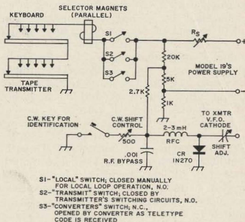
Fig. 5. The "Mainliner" frequency-shift keying circuit described by K8DKC in the May 1965 issue of QST. The resistor  $R_s$  is adjusted for 60 mA through the selector magnets.
