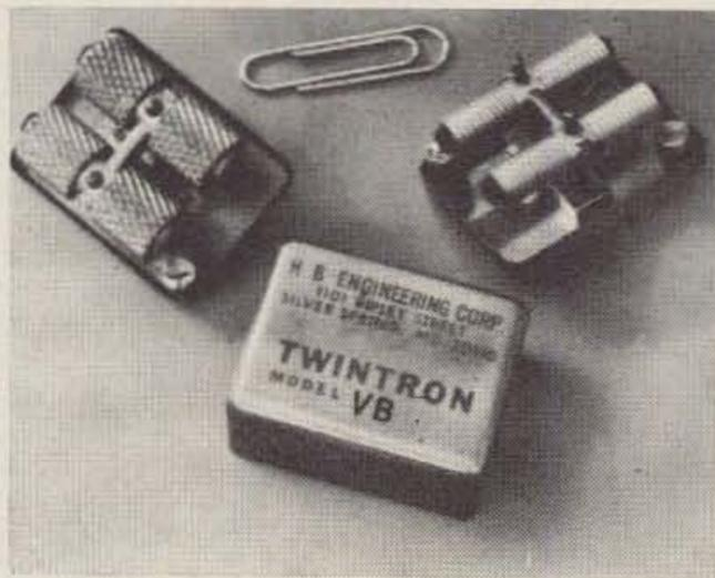
Here's a new device for electronics experimenters and builders of radio controls for model aircrafts and boats. It is a tunable, low-cost, electromechanical resonator, called the Twintron. The Twintron can be used in audio oscillator circuits, as a narrow band reject or pass filter and as a tone echo reflector.
