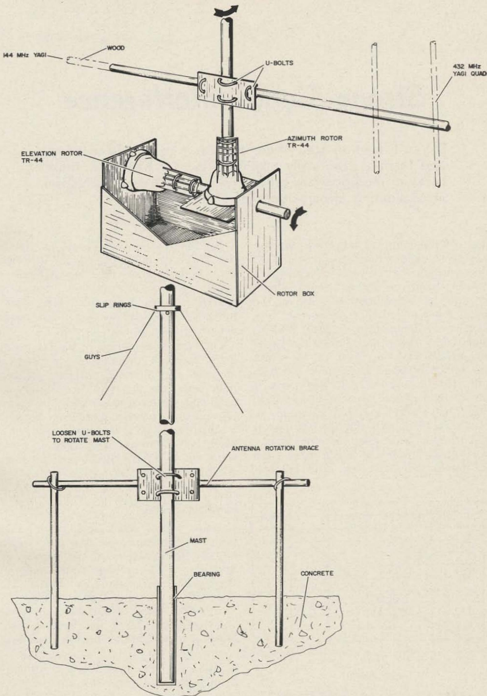
Fig. 1. Construction of the simple antenna mount used by W4HJZ for moonbounce and satellite tracking.
