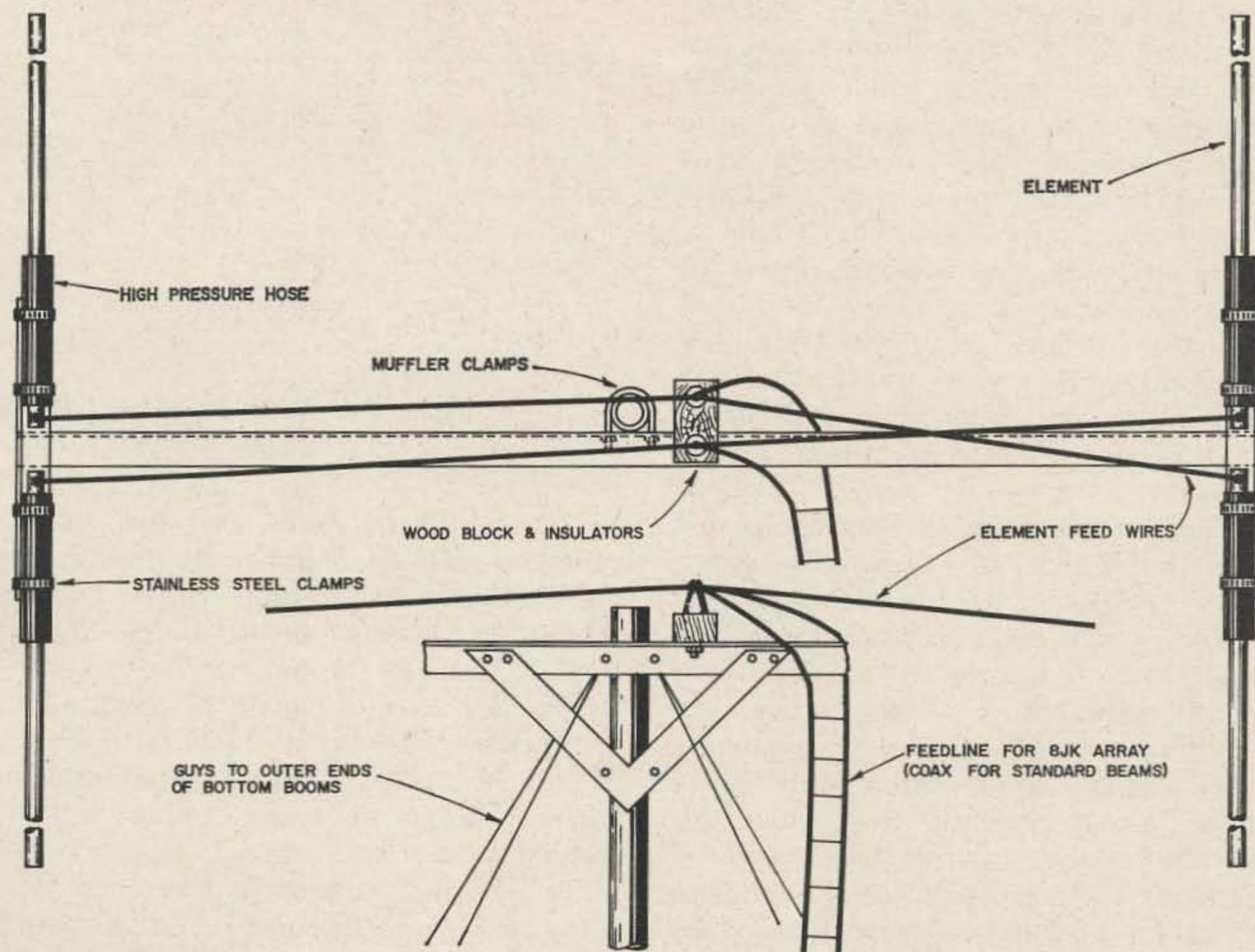
Fig. 2. Boom and element construction of the 8JK beam antennas used in the stacked-antenna experiments.
