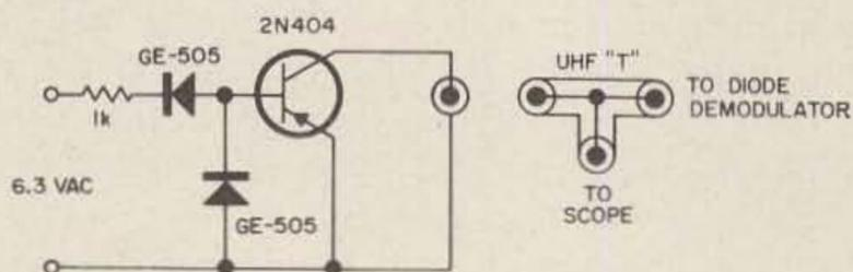
Fig. 1. Schematic of the solid-state chopper.
