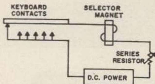
Fig. 1. With the local loop shown here, the teletype operator can type on the keyboard and activate the printer for printing.
