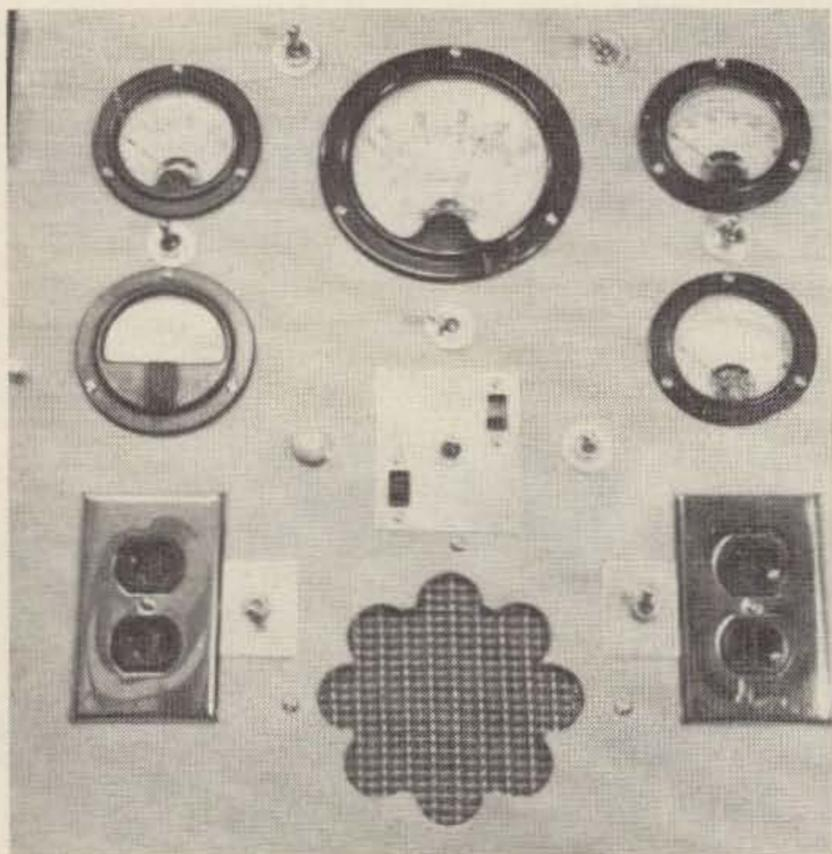
Note that the individual input receptacle to each of the four ammeters is not shown on the photograph. The reason for this is that I did not recognize the desirability of this feature until after the photograph was taken. All 'on'—'off' switches are turned 'on' by pushing the switches 'up'. All meter selector switches position by actuating toward the desired meter.
