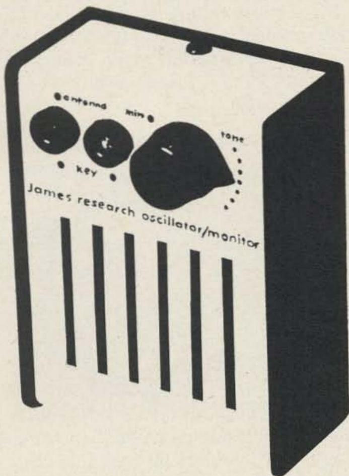
This unit can be used for many purposes. It is a broadband detector, coupled to a dc amplifier which triggers an audible tone oscillator and speaker for use as a DC oscillator/monitor. It will detect any rf power source of as little as 10 milliwatts without direct connection to the unit. The input detector will respond to any frequency between 100 kHz and 1000 MHz and a stiff wire pickup antenna of 8 inches in length is all that is required for most rf detection uses.
