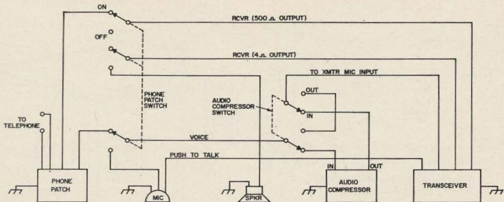
Fig. 1. Basic wiring diagram of the station control unit at K6ZHO.
