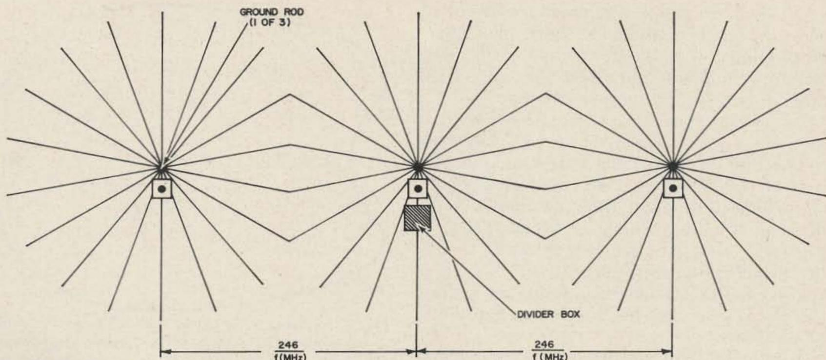
Fig. 2. Physical layout of the three-element vertical 40-meter array.
