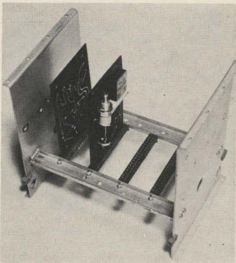
The computer card frame used by K1EIJ. If trouble is experienced with loose and wiggling cards, use the support brackets shown in Fig. 1.
