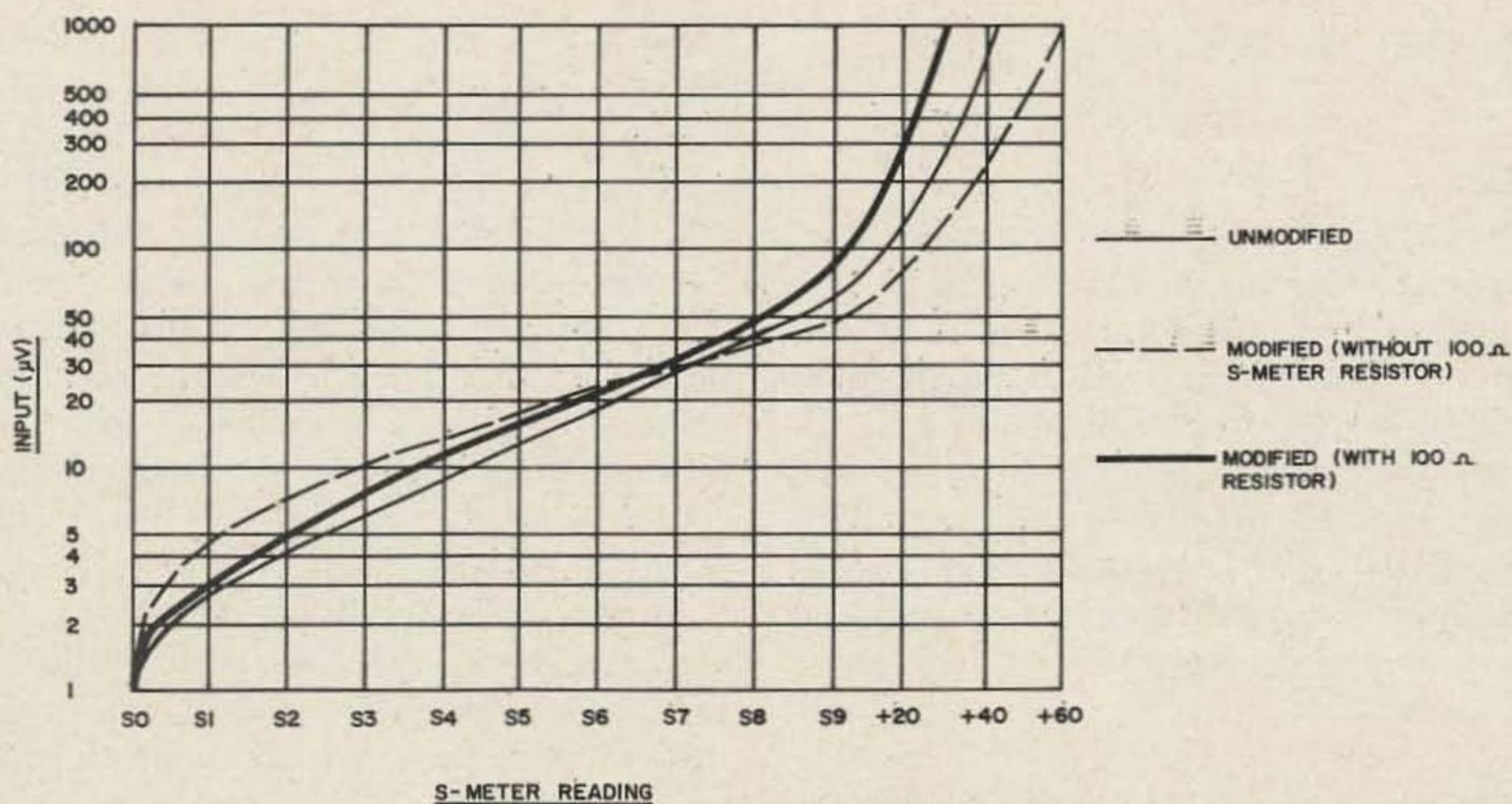
Fig 2. S-meter calibration for modified Collins 75S-3A, with the 100-ohm resistor in parallel with the meter. The slight bend in the curve at S-8 appears to be typical. Each 20 dB segment of the meter actually requires from 13 to 15 dB increase in receiver input, thus making antennas and linear amplifiers look somewhat better than they are.
