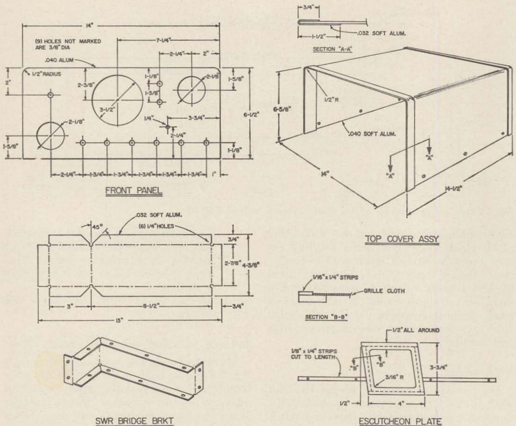
Fig. 2. Construction details of the station control unit. With this construction, the unit matches the author's other equipment as shown in the photograph.
