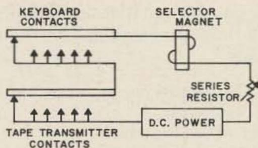
Fig. 2. With this local loop arrangement, the printer will print from either the keyboard or the tape reader.
