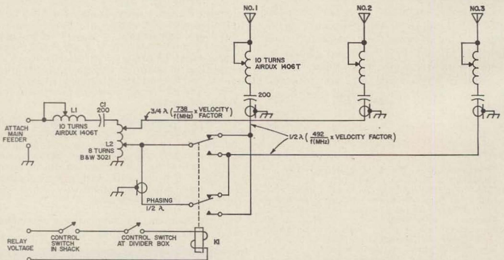
Fig. 1. Diagram of the 40-meter vertical array. The spacing between elements is 34 feet, 3 inches. The  $\frac{1}{2}$ -wave phasing line using RG-8/U coax is 45 feet long (54 feet, 7 inches for foam coax). The  $\frac{3}{4}$  wave phasing line is 67 feet, 6 inches long (81 feet, 9 inches for foam).
