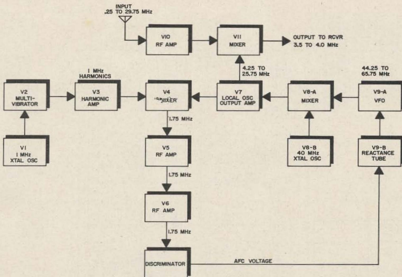
Fig. 1. Block diagram of the wideband converter which covers from 500 kHz to 29.5 MHz. A complete description of its operation is given in the text.
