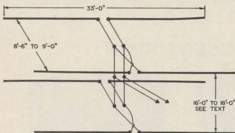
(A) BASIC DESIGN OF 8JK BEAMS USED IN TESTS
