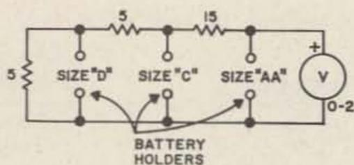
Fig. 2. Tester for dry cells. This tester puts a load on a standard carbon-zinc cell approximately equal to its 10-hour intermittent discharge rated load. A 40-ohm load should be used when testing AAA or N size cells. A 9-volt transistor battery should be tested with a 250-ohm load and will give six times the voltage listed in Table 1.
