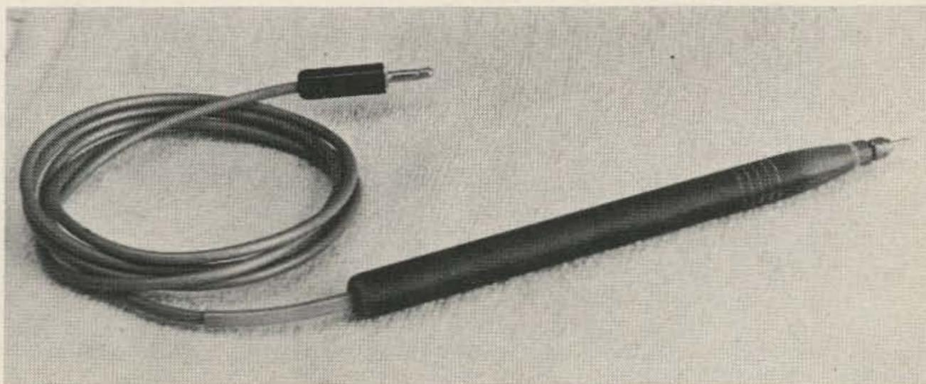
to pin 8 of the 12AU7A cathode follower. This gives upscale deflection for positive voltages. The wire lead is the meter's positive terminal.
