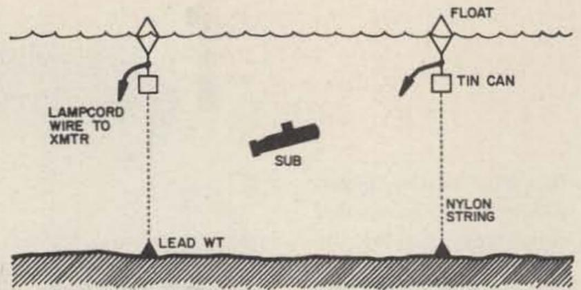
Fig. 3. Horizontal antenna used in further underwater radio control tests. The propagation from this antenna is shown in Fig. 4.
