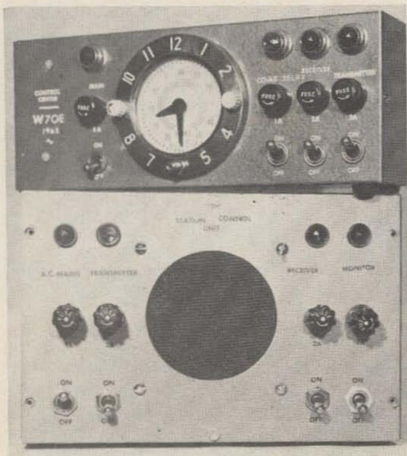
Simple control centers for the novice station: the upper unit includes the station clock; a loud speaker may be substituted as shown in the lower unit.
