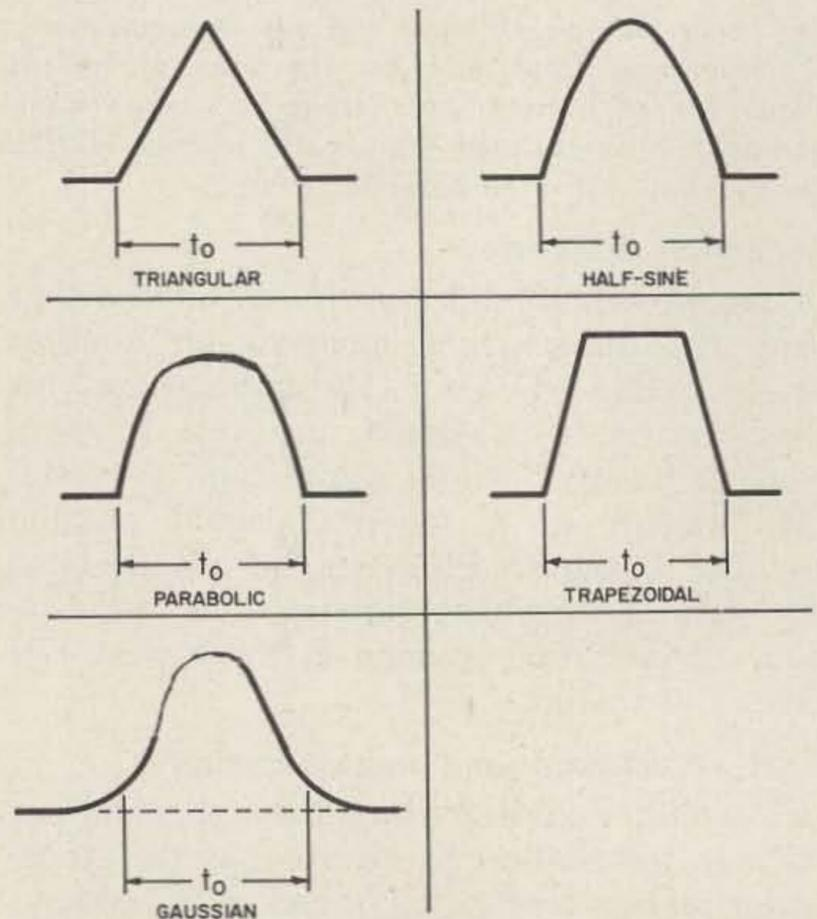
Fig. 2. Other pulse shapes which may be encountered—triangular, half-sine, parabolic, trapezoidal and gaussian.
