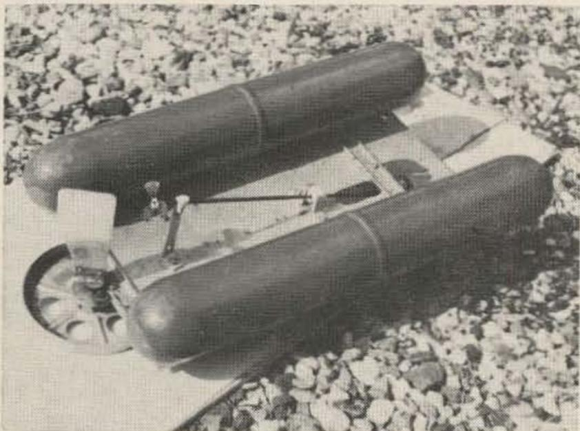
Bottom view of the beached radio-controlled catamaran showing the drive propeller and motorized rudder control. This "cat" could be completely controlled by a radio transmitter and antenna mounted beneath the surface of the water.
