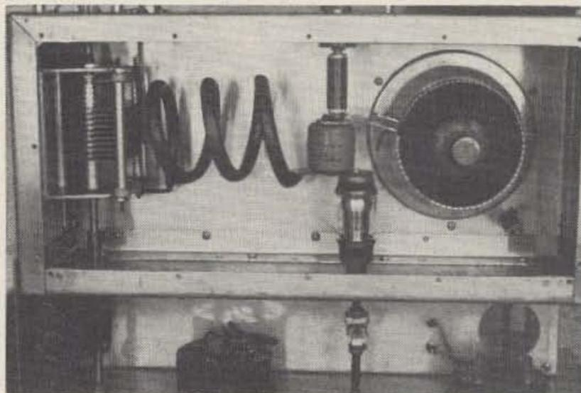
Top view showing the inside of the final plate compartment. The high-Q tank circuit provides good stability. The strap in the lower right corner is used for neutralization. A homemade rf choke is supported by the door knob capacitor on the rear wall.
