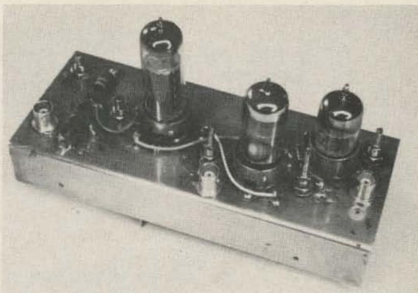
Transmitting converter. Top view showing the solder-in feedthru capacitors and general dc wiring.
