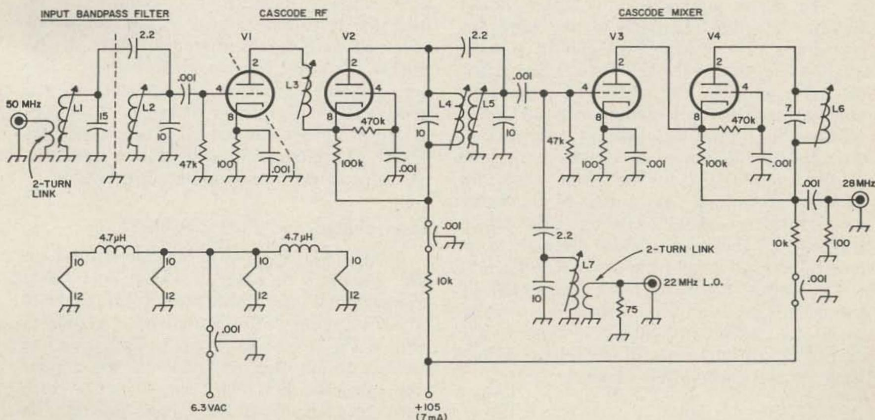
Fig. 3. The six-meter converter section of the 2 kW PEP transmitter. The cascode rf amplifier uses two 6CW4's for maximum performance. The 22-MHz local oscillator input is picked up from the transmitting convert. Coil values are given in Table 2. All tubes are 6CW4/6DS4.
