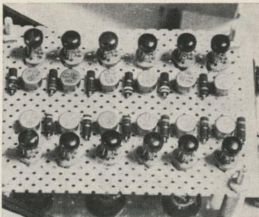
Inside view of the count indicator, showing how the 12 stages of IC's and associated transistors are mounted on punched board which measures 3 x 4 1/4 inches.
