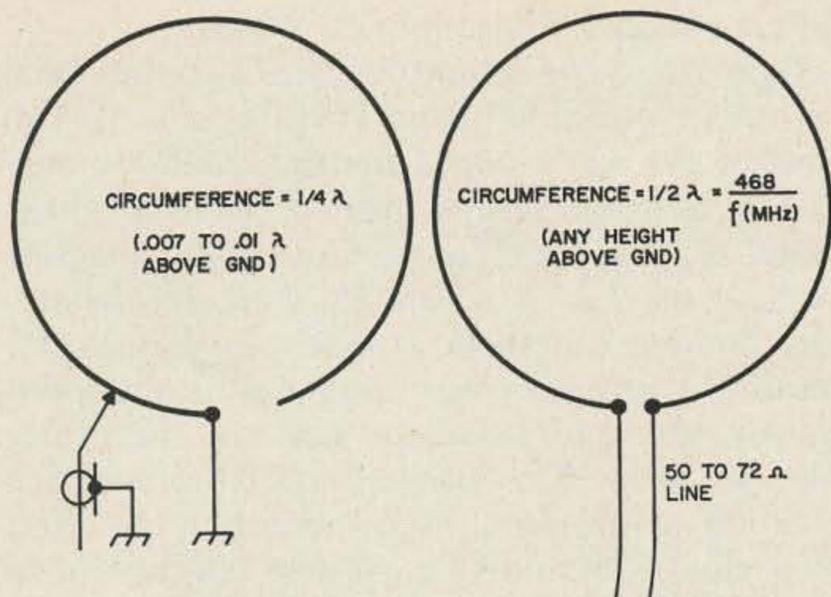
Fig. 1. Basic dimensions of the one-quarter wave and one-half wave ring radiators used for fixed/portable operation by WIDCG.
