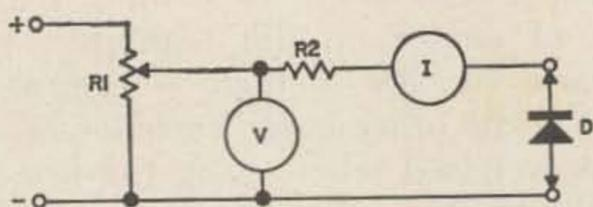
Fig. 3. A simple diode tester used by VK7RG for checking PIV.
