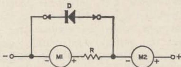
Fig. 4. Protecting a sensitive meter movement with a silicon diode.  $M_1$  is the meter being protected,  $M_2$  is for temporary measurements. The value of  $R$  is increased until meter  $M_1$  reads about one-percent low as indicated by  $M_2$ .
