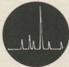
**Scanning Function** — approximately 250 kHz sweep width — indicates two signals above and three below the received signal, the strongest signal about 30 kHz down the band, down frequency being to the right.
