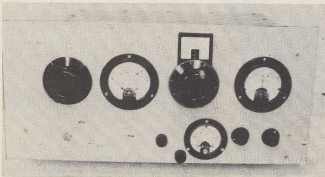
Front view of 2 kW transverter, left to right: output loading, plate current, plate tuning, screen current; bottom: driver tuning, driver coupling, final-grid current, final-coupling, and grid tuning.
