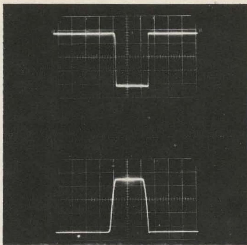
Fig. 6 Output waveform of the circuit in Fig. 5 for minimum pulse width. The sweep speed of the oscilloscope is 1  $\mu\text{second}$  per division.
