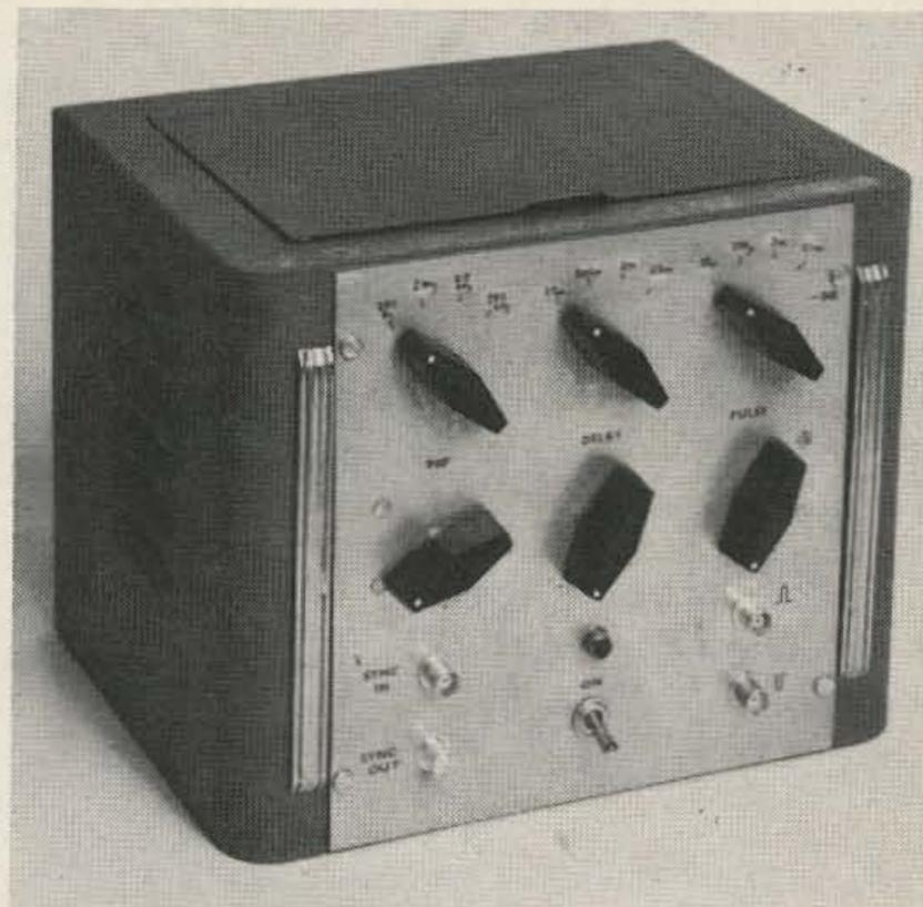
Fig. 7 The pulse generator. This unit uses integrated circuits and transistors to provide pulse repetition rates from 20 Hz to 200 kHz, pulse delays from 20 microseconds to 20 milliseconds and pulse widths from 20 microseconds to 20 milliseconds. A square wave output is also available.
