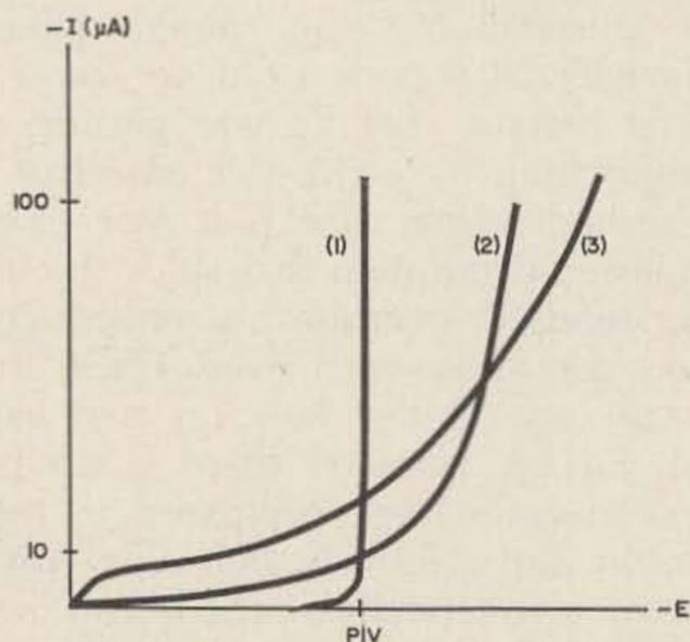
Fig. 2. The reversed-biased characteristics of zener diodes (1), silicon diodes (2) and germanium diodes (3). Note that this drawing is shown upside down from the usual presentation.
