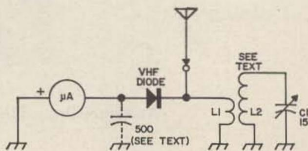
Fig. 1. Schematic diagram of the 220 MHz wavemeter. The coils are described in the text.
