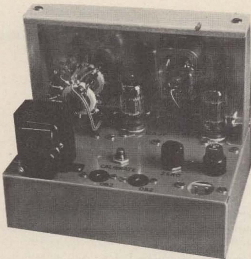
Fig. 2. Back view of dc VTVM. In this shot the OB2's were pulled out for a better view. The lip at top of the panel makes a convenient handle.
