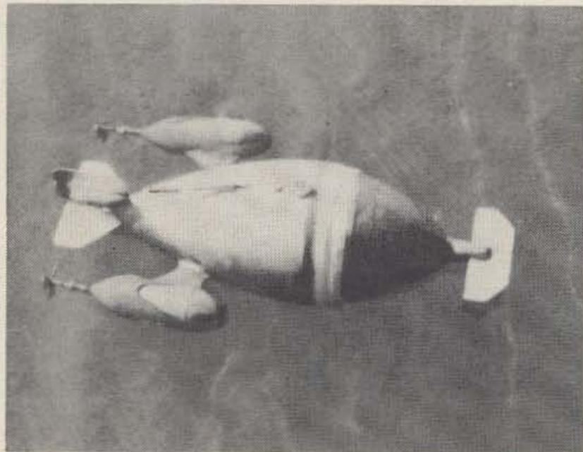
Radio-controlled submarine used by K6BIJ in his underwater radio propagation tests.
