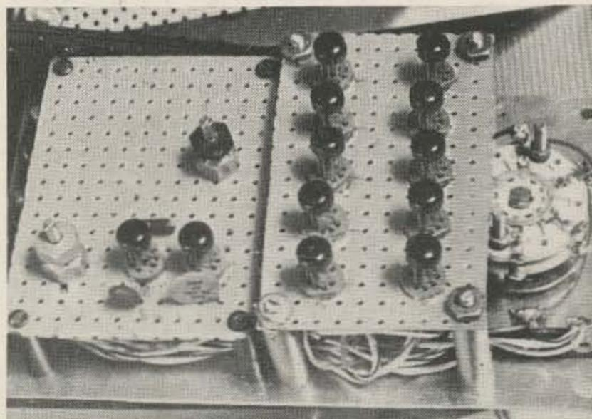
Inside of the count controller. At the right is the switch which selects the various ranges and functions. In the middle is the frequency divider section and interval switcher with gate. This punched board measures  $3\frac{1}{4} \times 2$  inches.
