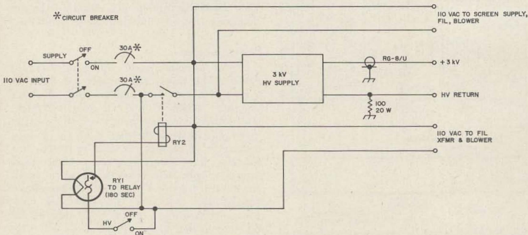
Fig. 7. High-voltage power supply controls which are used in the 4CX1000A transverter. The 3000-volt high-voltage supply is not shown since most builders will use what they have available in the junk box.
