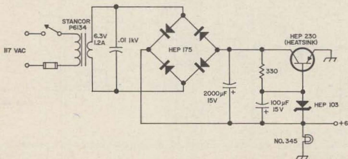
A regulated power supply for the pulse generator shown in Fig. 5.
