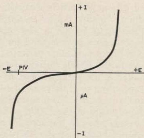
Fig. 1. Typical diode characteristics. Note that the current scales above and below the voltage axis are in different units.
