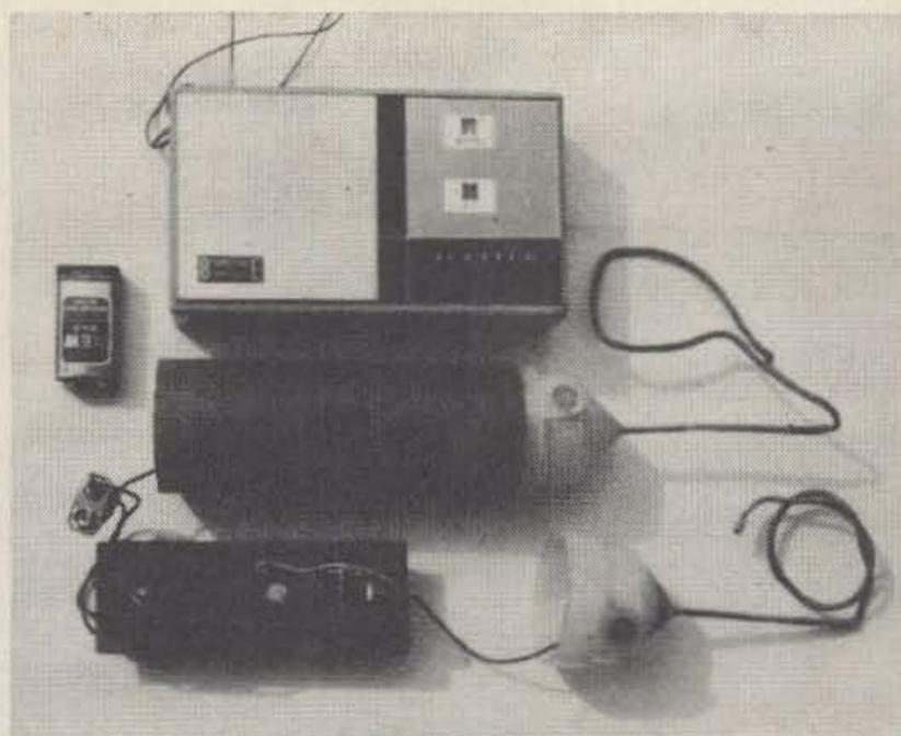
The 1-milliwatt, 4 MHz transmitter used by K6BIJ in his underwater propagation tests. The receiver is a Japanese transistor model that covers the marine band up through 4 MHz.
