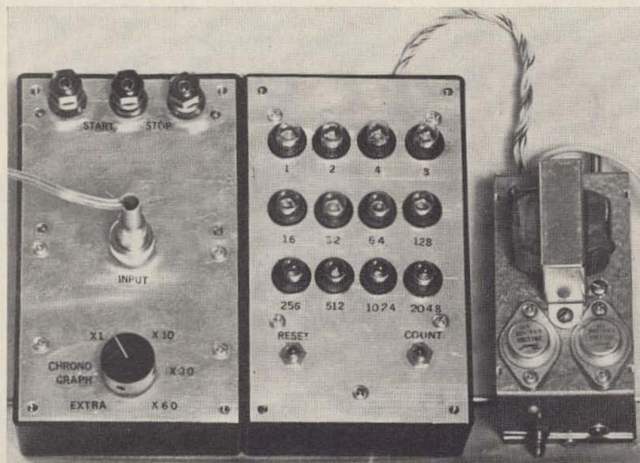
Top view of the count indicator (middle), the count controller (left) and the power supply (right). The three terminals on the top of the count controller are used when the unit is used as a chronograph for measuring bullet speeds.
