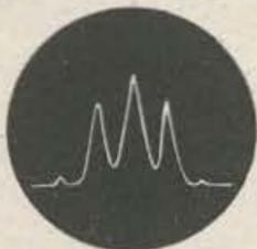
**Analyzing Function** — 10 kHz preset sweep width — indicate carrier 100% modulated by 2 kHz tone-log scale.
