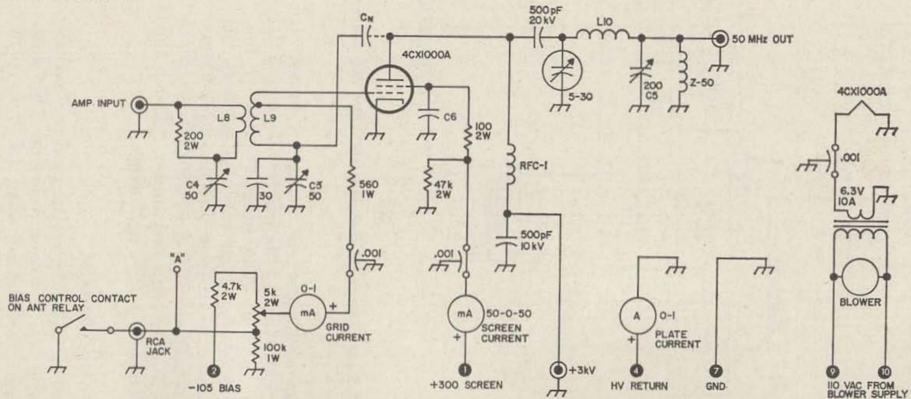
Fig. 2. Schematic diagram of the transmitting 6-meter converter and 4CX1000A amplifier. Coil values for this unit are given in Table 1. All feedthrus are .001 ceramic.
