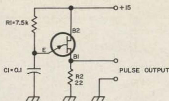
Fig. 3. A simple unijunction transistor relaxation oscillator which will generate the pulse chain. The pulse repetition rate is determined by  $R_1$  and  $C_1$ ; the on time is controlled by  $R_2$  and  $C_1$ .
