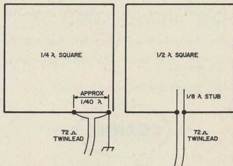
Fig. 2. Forming the rings into squares distorts the horizontal radiation pattern somewhat, but the antenna is still essentially omnidirectional.
