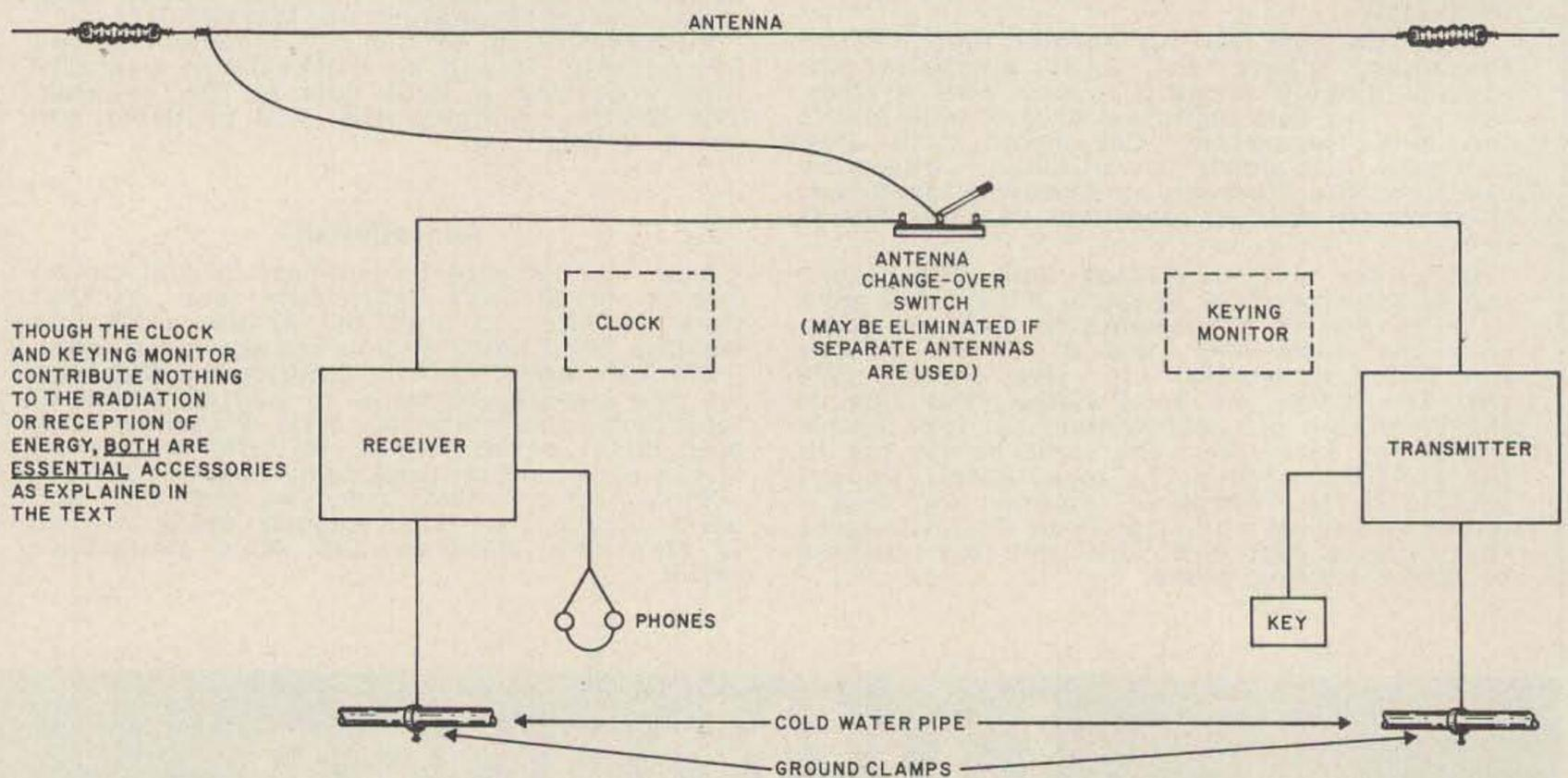
Basic equipment for the novice station. While the clock and keying monitor contribute nothing to the radiation or reception of energy, both are essential accessories as explained in the text.
