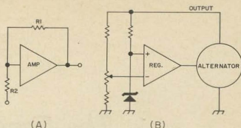
Fig. 2. Block diagram of the solid-state alternator. The system used closely resembles the simple dc feedback amplifier in A. In this type of amplifier, the gain closely approaches  $R_1/R_2$ . If the gain is very high, the regulator in B will not allow the preset voltage to change until the alternator is no longer capable of delivering the required current.
