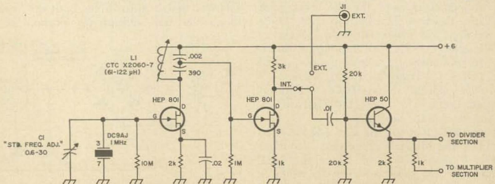
Fig. 9. One MHz oscillator-buffer section.
