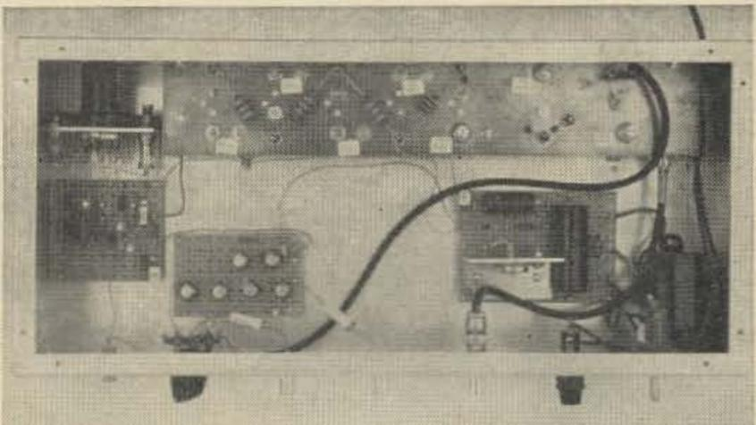
Fig. 12. VHF calibrator built with HEP 558 J-K flip-flops in the divider section. This photograph shows the unit in early stages of construction, with only one decade of dividers in use. Later four more HEP 558's were added to provide a second decade.
