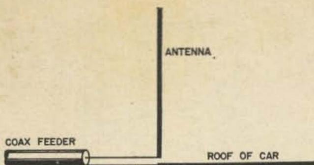
Fig. 2. Apparent effective antenna on 10 meters with the arrangement in Fig. 1.
