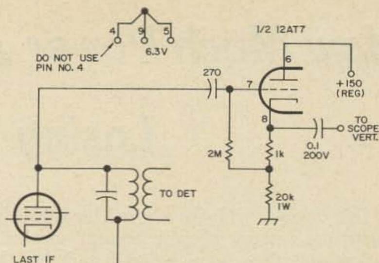
Fig. 14. Cathode follower circuit which is used to isolate the last *if* stage from the oscilloscope.
