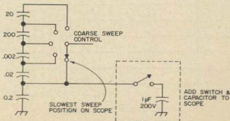
Fig. 15. Adding a capacitor to the scope's sweep circuitry to slow down the trace for CW monitoring.
