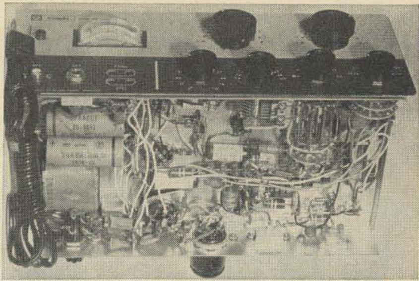
Joe's little T-60 rig in the final wiring stages. Later FN showed him how to lace and cable the loose wiring into a neat harness.
