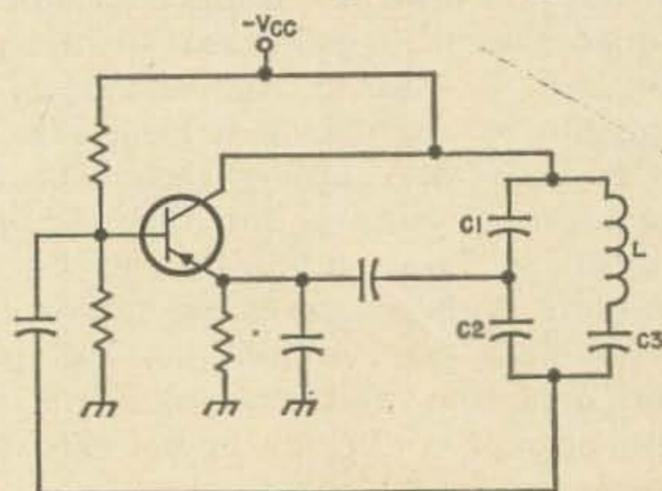
Fig. 19. The transistor Clapp oscillator. Excellent frequency stability can be obtained with this circuit because the capacitors  $C_1$  and  $C_2$  may be made large enough to swamp out any capacitive effects of the transistor.
