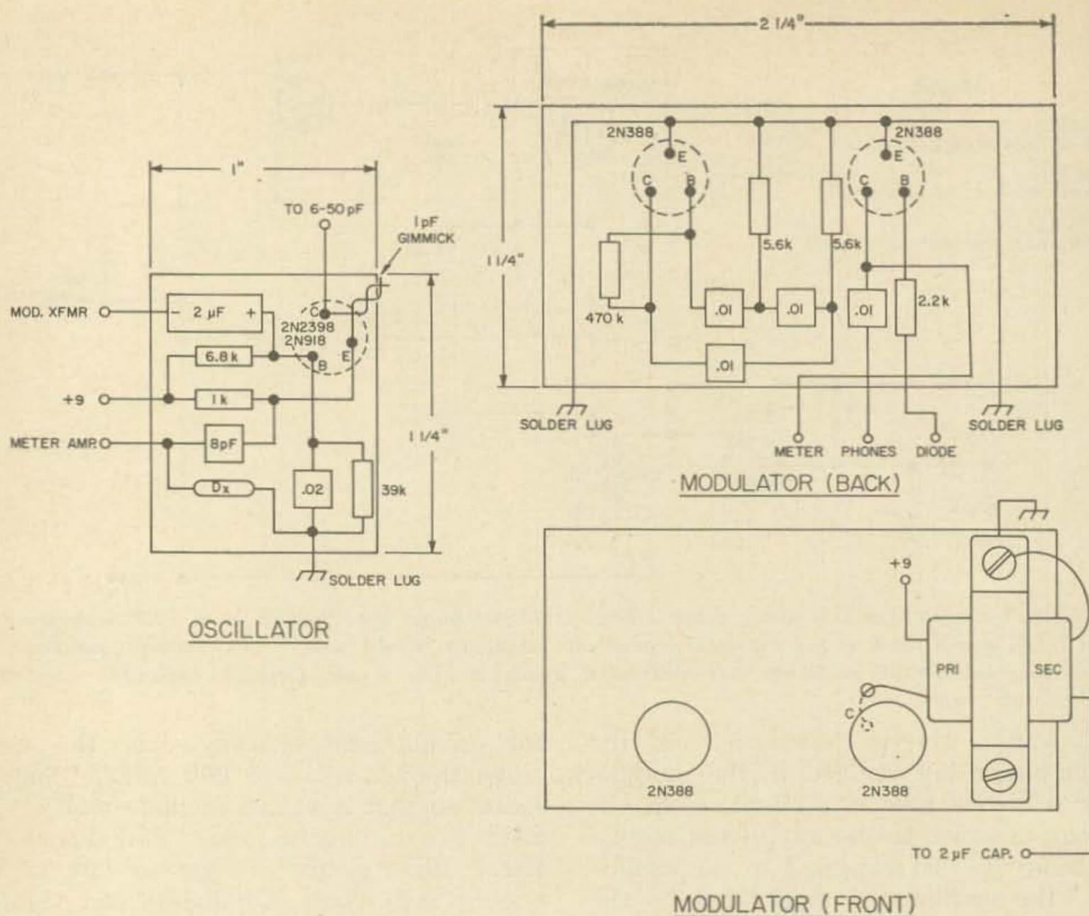
Fig. 2. Layout of the two circuit boards used in the case, the circuit could be easily adapted to one board, and even to printed circuitry.
