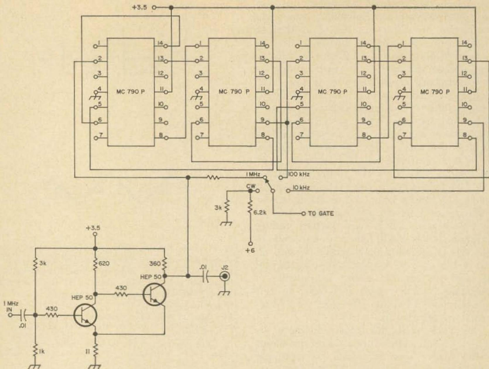
Fig. 4. Divider section uses integrated circuits to generate 10 kHz and 100 kHz marker signals from a 1 MHz crystal. The unmarked resistor in the 1 MHz should not be there—short it out. This two-meter calibrator offers a choice of calibration modes: 144 MHz alone, 144 MHz  $\pm$  1 MHz, 144 MHz  $\pm$  100 kHz, or 144 MHz  $\pm$  10 kHz. The mode-switching allows one to go from a rough 1 MHz interval frequency check to a 100 kHz interval check, and finally, to a 10 kHz interval check.
