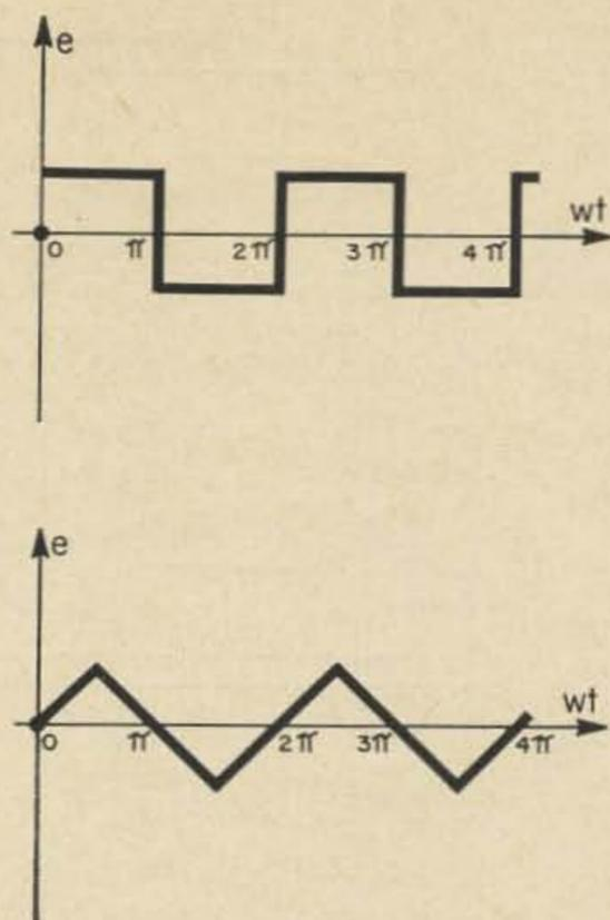
Fig. 2. Two nonsinusoidal waveforms which may be used for harmonic generation. The Fourier series of the square wave indicates that harmonics fall off at the rate of  $1/n$ , where  $n$  is the harmonic number. The harmonics of the triangular wave fall off at the rate of  $1/n^2$ .\*
