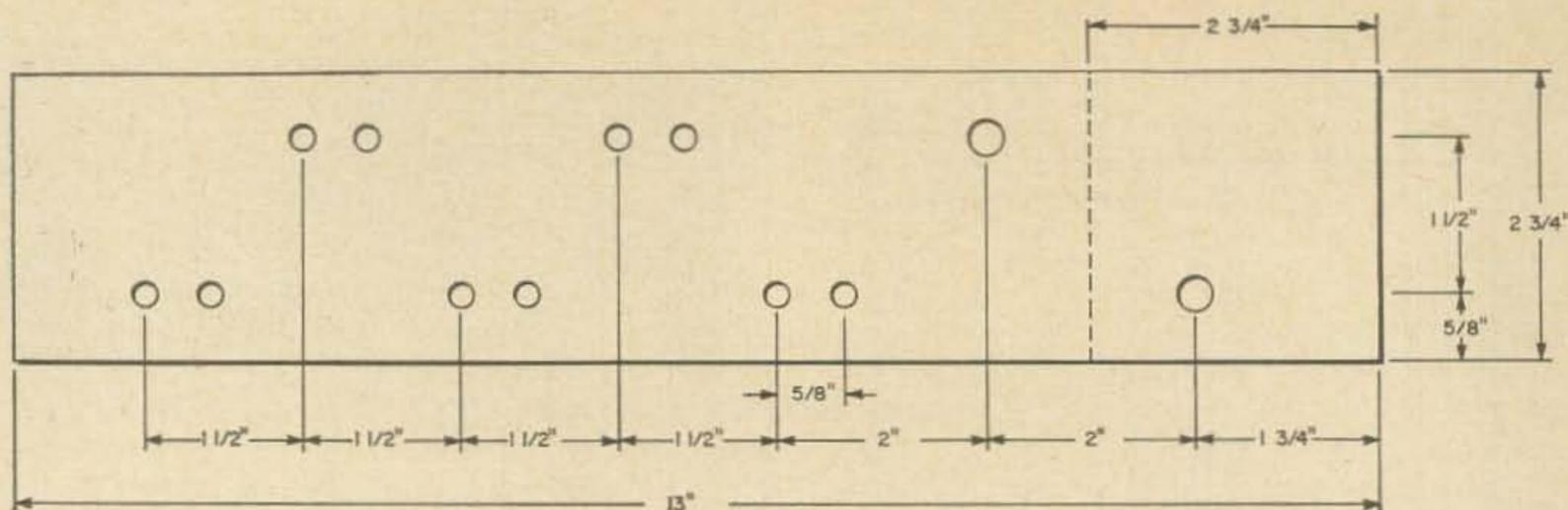
Fig. 14. Template for the top plate of the multiplier assembly.
