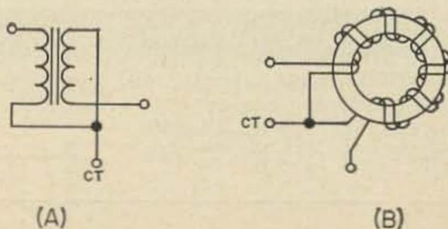
Fig. 3. A balanced, center-tapped inductor wound on a toroid core.
