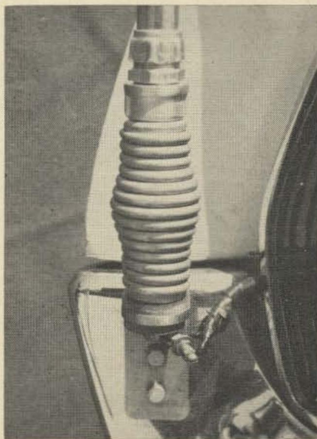
Construction of the base section of the W6IEL mobile antenna.
