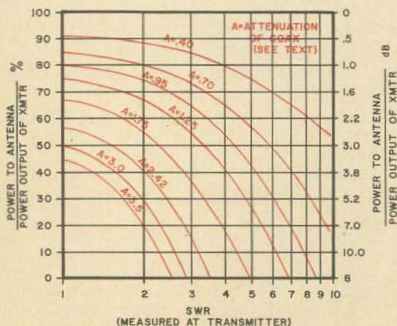
Fig. 1. Ratio of power at antenna to power at transmitter versus SWR.
