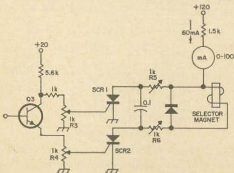
Fig. 3. The complete SCR printer-magnet driver circuit with the trigger, Q<sub>3</sub>.
