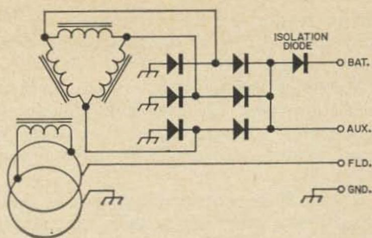
Fig. 5. Schematic of a Motorola alternator showing the delta-connected stator used in the 55-ampere model. Also shown is the isolation diode and auxiliary terminal connection.
