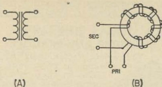
Fig. 2. Winding a high-frequency transformer on a toroid core.
