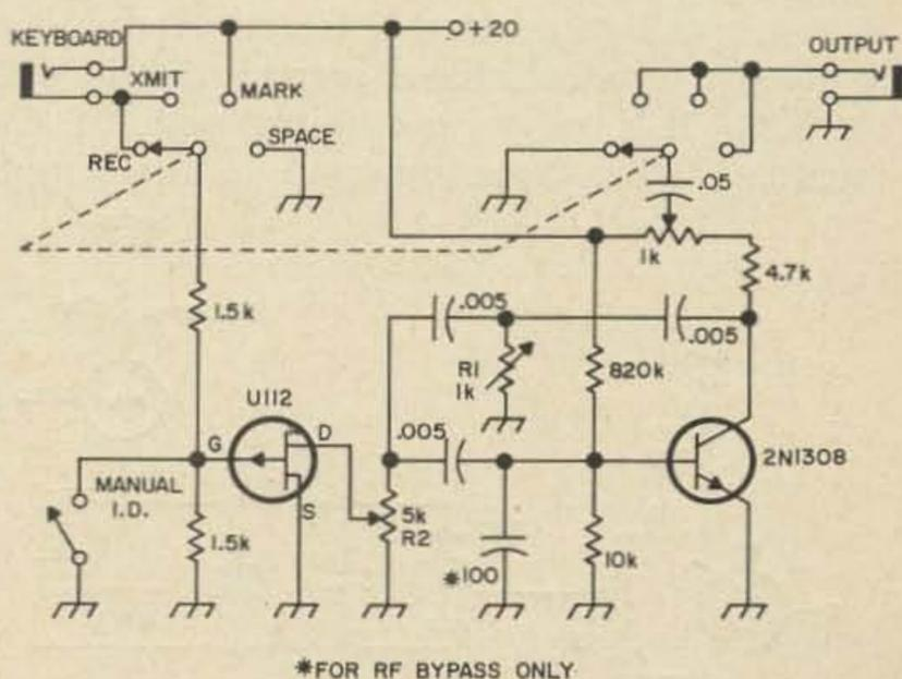
Fig. 1. The AFSK phase-shift oscillator used in the Semi-RTTY system. This circuit features equal mark and space output levels, no switching transients, isolation from the keyboard and a simple shift system—an FET used as a resistor.
