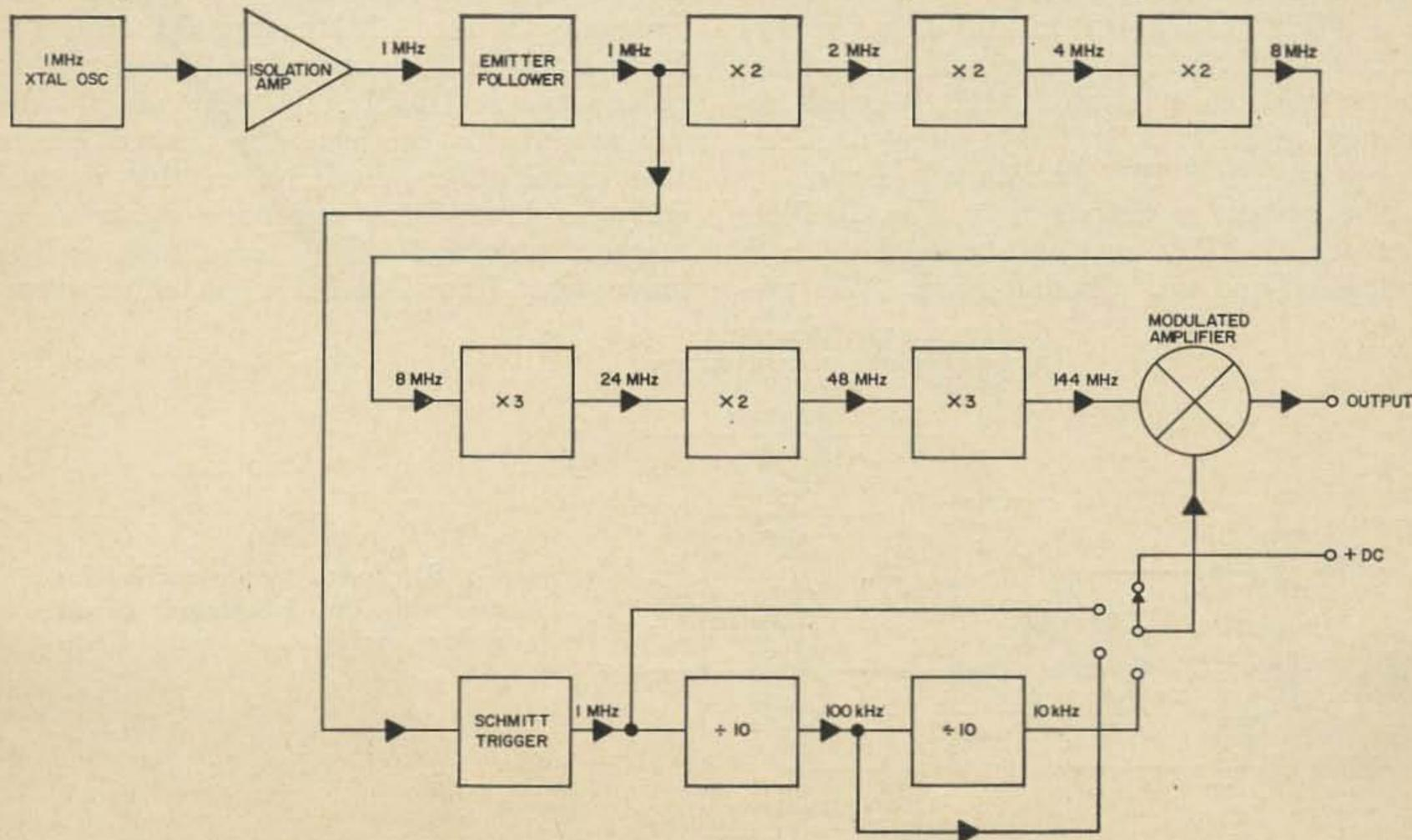
Fig. 3. Block diagram of the VHF man's calibrator.
