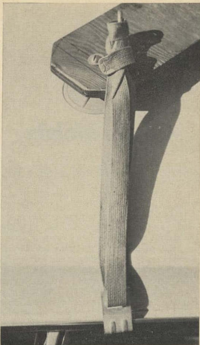
The X-mount is secured to the car with suction cups, gutter clips and straps as shown here.
