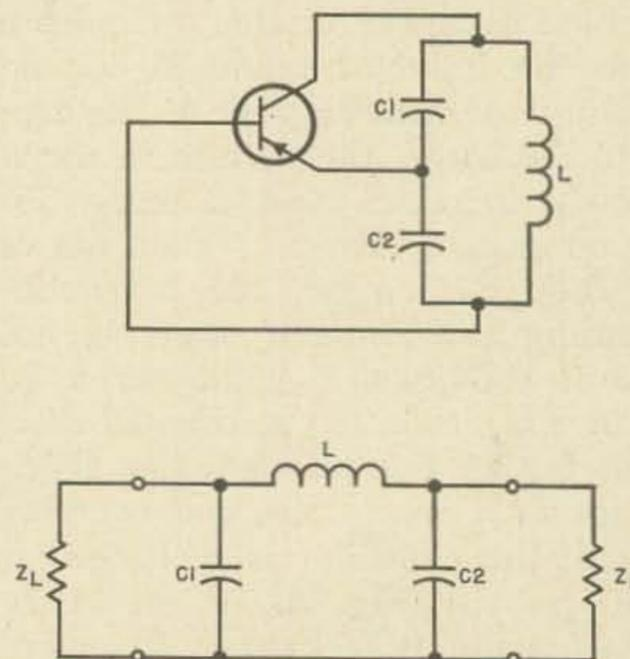
Fig. 4. The basic Colpitts oscillator. Bias resistors and power supplies have been left out for clarity. Since the input and output impedances of the transistor ( $Z_L$  and  $Z_I$  respectively) load the tuned circuit, the circuit may be further simplified by replacing the transistor with two resistors representing the loading.
