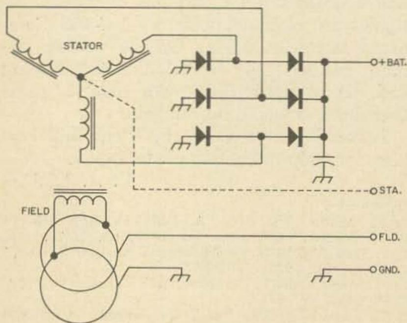
Fig. 1. Typical alternator schematic showing wye-connected stator windings: the stator midpoint is brought out to a terminal only on Ford (Autolite) units.
