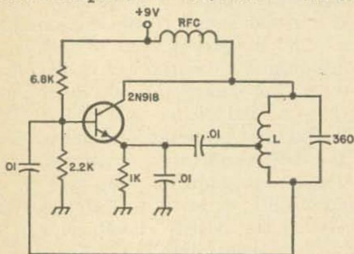
$L = 10\text{-}1/2$  TURNS NO. 26 ON J.W. MILLER 4500 SLUG-TUNED FORM. TAP 2-3/4 TURNS FROM BOTTOM.
