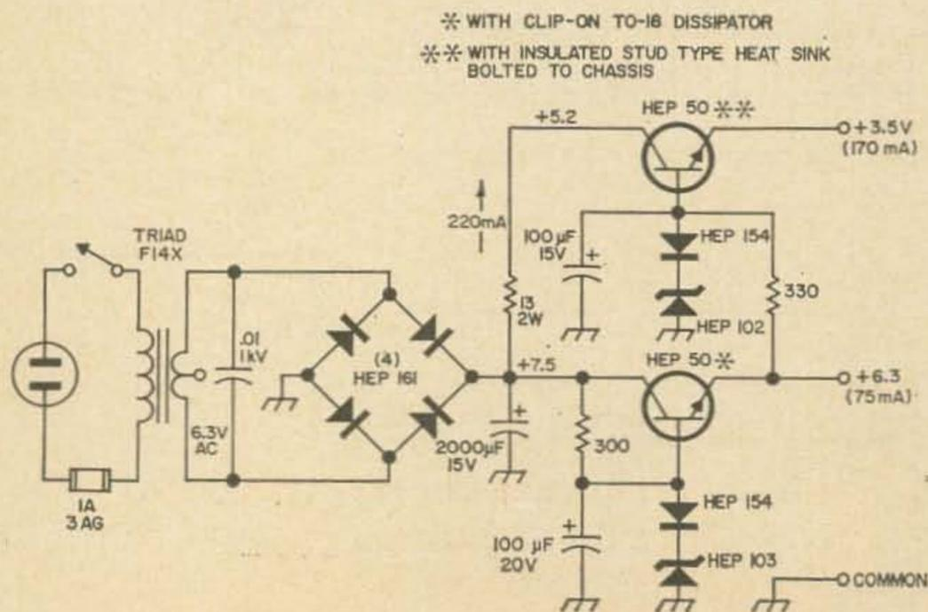
Fig. 5. Power supply section for use with the integrated circuit divider of Fig. 4.
