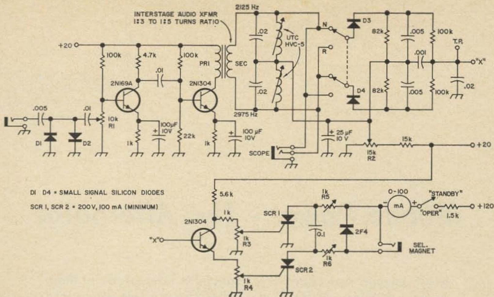
Fig. 4. Circuit of the complete semi-RTTY tuning unit.
