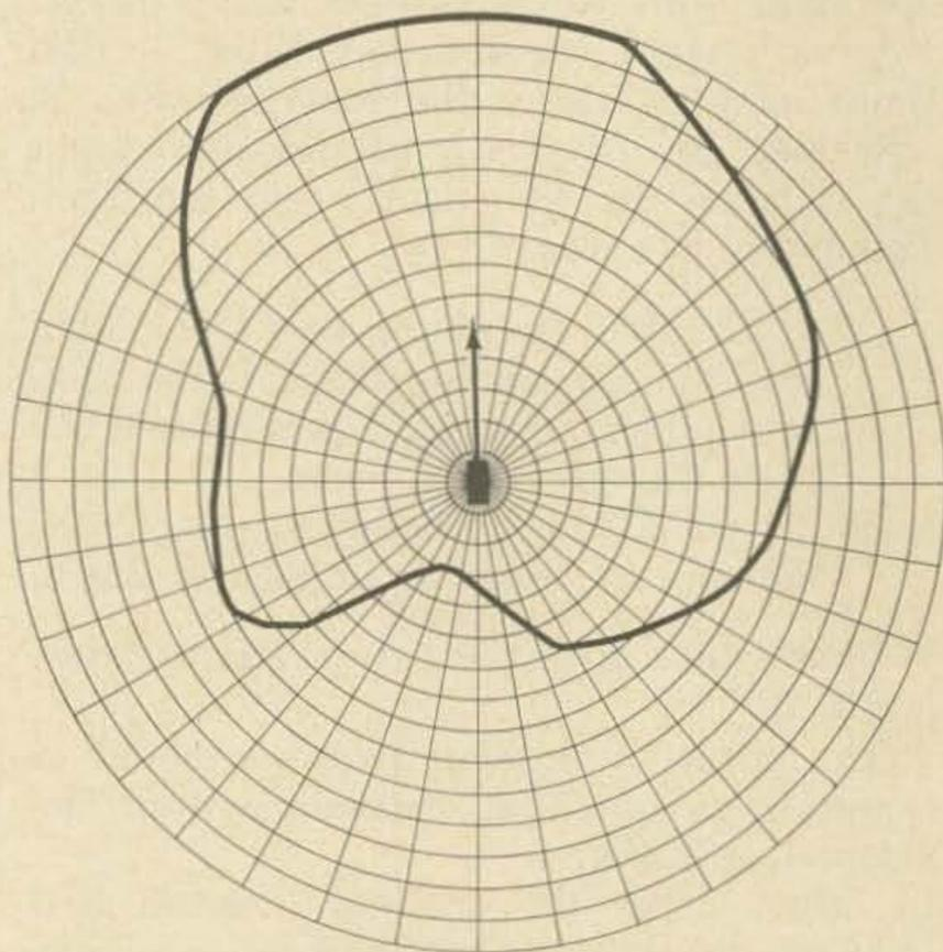
Fig. 6. Directional pattern of the antenna as mounted in Fig. 5.
