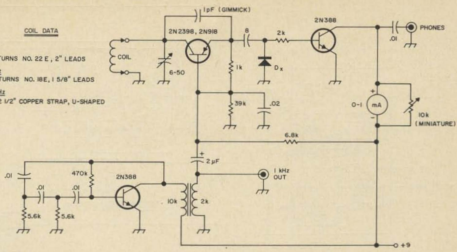
Fig. 1. Circuit diagram of the great dipper. Note that although the 2N2398 is a PNP transistor, the 2N918 is NPN, and if used as the oscillator transistor, problems would arise with voltage polarity. The diode  $D_x$  may be almost anything that you have available. The 1 pF gimmick capacitor consists of 1 1/2" of twisted wire.
