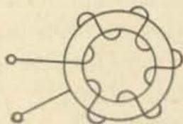
Fig. 1. A toroidal-core of six turns. When using toroids, there is no such thing as half a turn—if the wire goes through the center of the core, the turn counts as one full turn.
