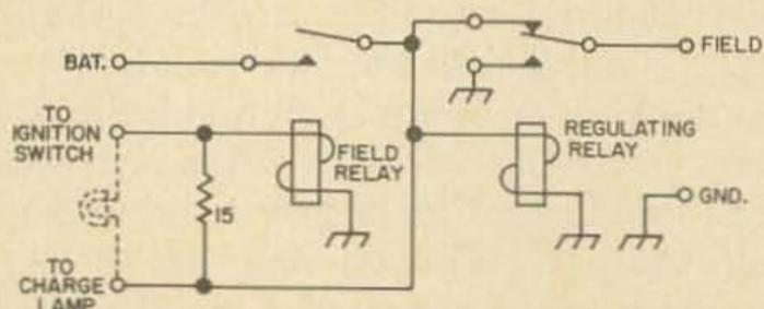
Fig. 3. Schematic of the two-relay regulator with a terminal for operating a charge-indicator lamp.
