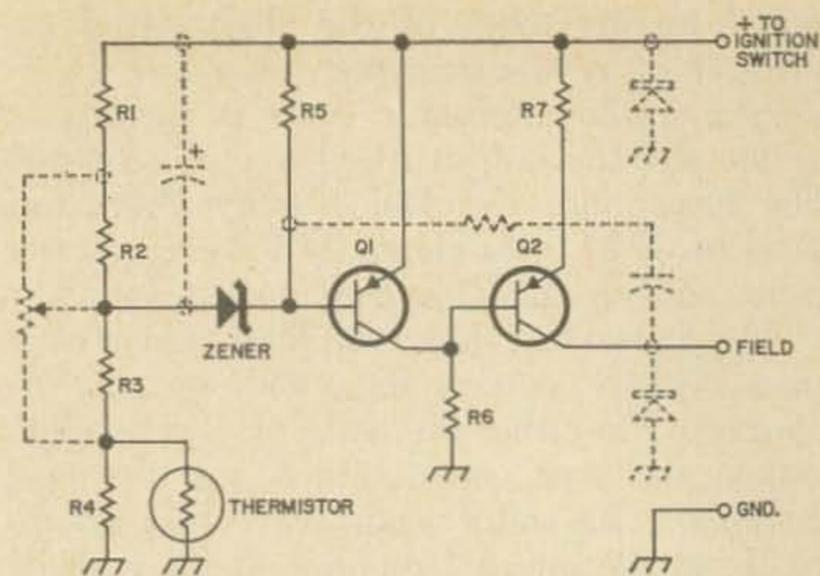
Fig. 4. Schematic of a typical solid-state regulator. Components shown connected by dashed lines are used by some manufacturers, but not all of them.
