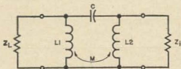
Fig. 11. The basic Hartley oscillator without bias resistors and power supplies. The circuit may be further simplified as shown by substituting resistors  $Z_L$  and  $Z_i$  for circuit loading by the transistor.
