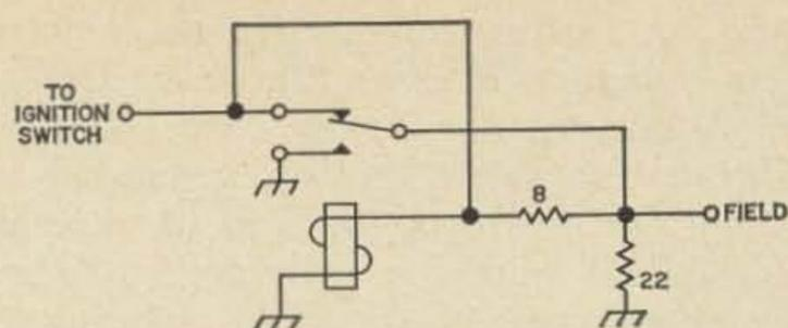
Fig. 2. Schematic of a single-relay regulator.
