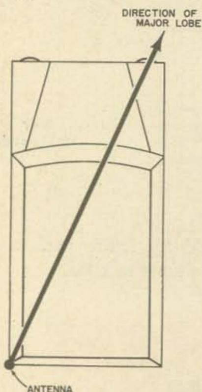
Fig. 1. Directional pattern of a vertical mounted in the rear left corner of a station wagon.
