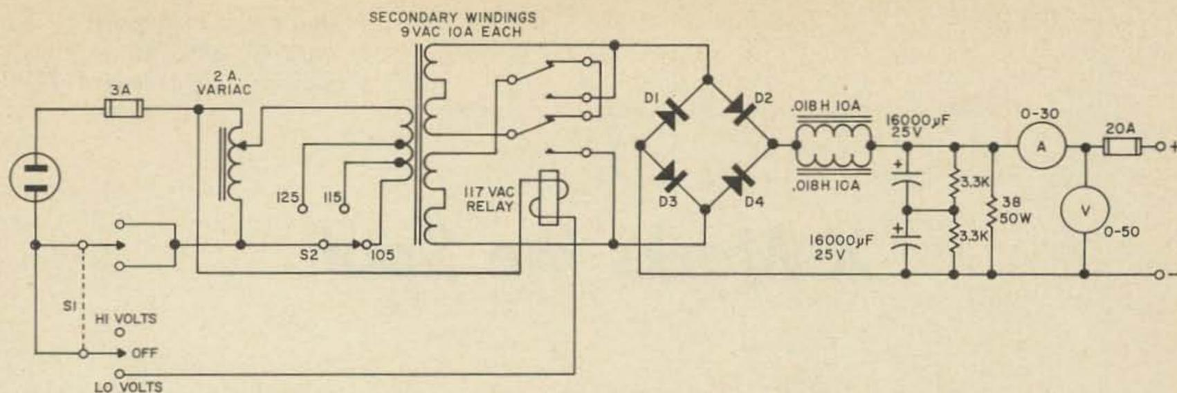
Fig. 1. Schematic of the 20-amp power supply. The 1600  $\mu$ F filter capacitors consist of sixteen 1000  $\mu$ F units wired in parallel. A minimum of 8000  $\mu$ F should be used. The diodes are 100 PIV, 20-amp units available from Meshna.
