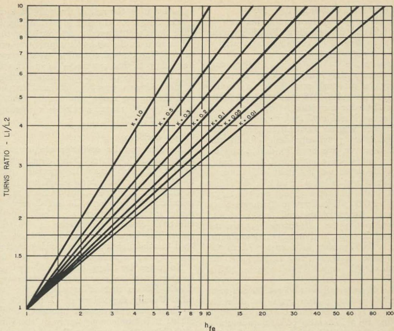
Fig. 17. Graph for determining the tap point on the tuned-circuit inductor in a transistor Hartley oscillator when the forward current gain ( $h_{fe}$ ) and coupling coefficient ( $k$ ) of the coil are known.
