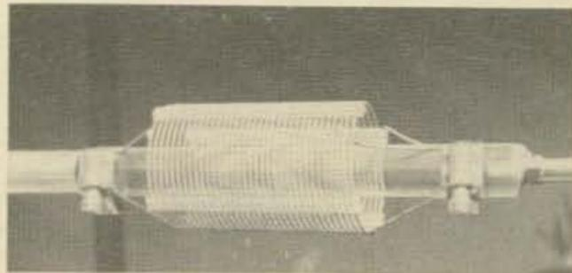
The loading coil. Note the support wires, which are connected from the first and last turns of the air-wound coil.
