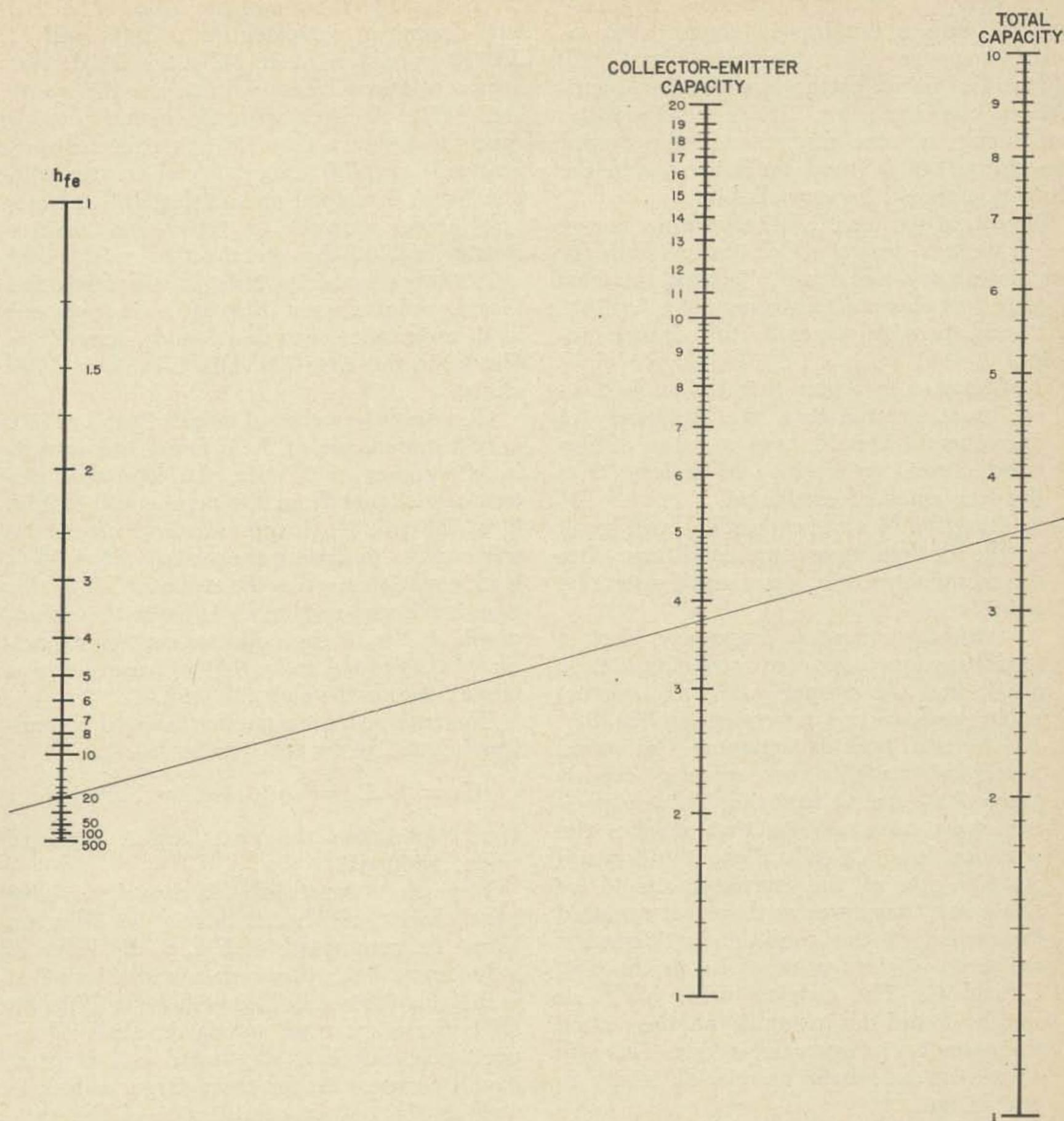
Fig. 9. Nomograph to find the required collector-emitter capacitor in a transistor Colpitts oscillator when the forward current gain ( $h_{fe}$ ) and total tuned-circuit capacitance ( $C_T$ ) is known. In this case, forward current gain of 20 and total tuned-circuit capacitance of 355 pF requires a collector-emitter capacitor of 375 pF.
