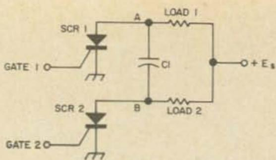
Fig. 2. Basic SCR circuit which is used to drive the printer magnet.
