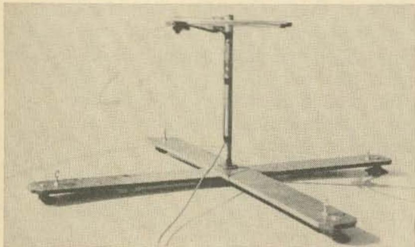
The X-mount is slid around on the roof of the car until it is centered, then the straps are put in place. In this picture the mount is being used to support a commercial two-meter halo antenna.
