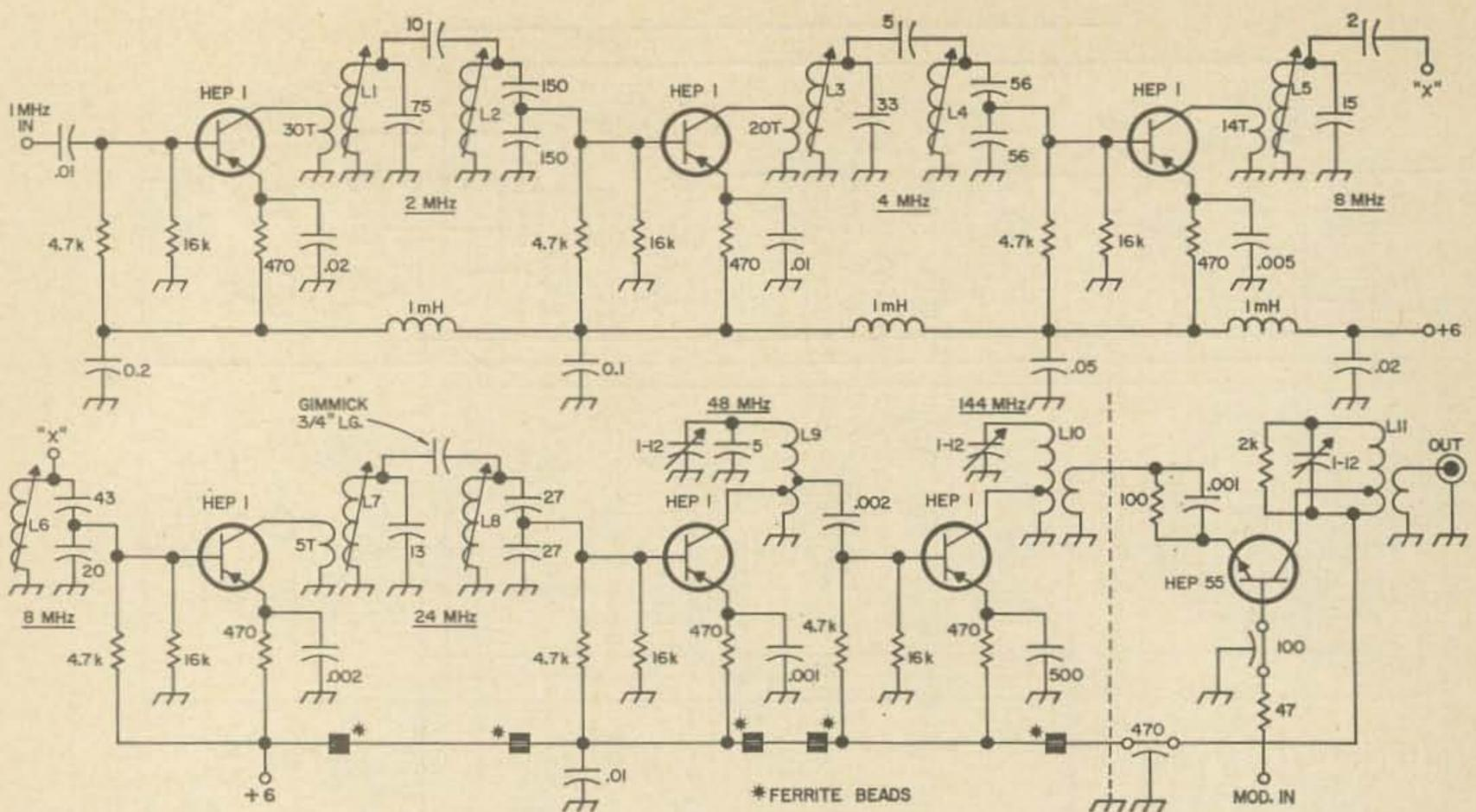
Fig. 8. The times 144 frequency multiplier. A crystal controlled input at 1 MHz provides an output at 144 MHz. Coil information for this circuit is given in Table 1.
