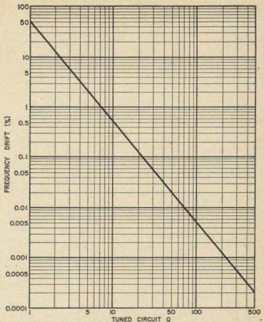
Fig. 7. The affect of tuned-circuit  $Q$  on frequency drift in an oscillator. For maximum frequency stability in a practical circuit, the  $Q$  should be as high as possible.
