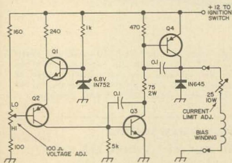
Fig. 1. Circuit diagram of the solid-state automotive voltage regulator. This circuit will provide excellent regulation to over 100 amperes. Although it was designed for use with Leece-Neville alternators, it will work with just about any alternator made. Transistor types may be chosen by referring to Table 1.
