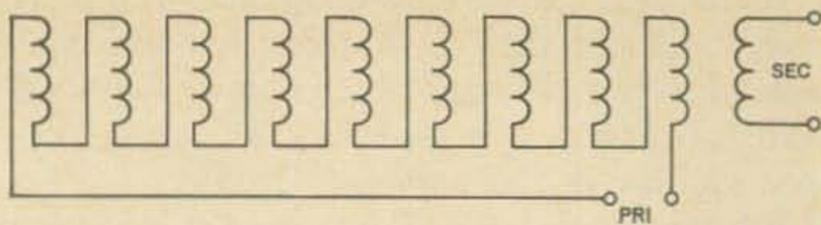
Fig. 4. Method of connecting several windings in series to obtain higher turns ratios. When doing this however, the proper phase relationships between windings must be observed.
