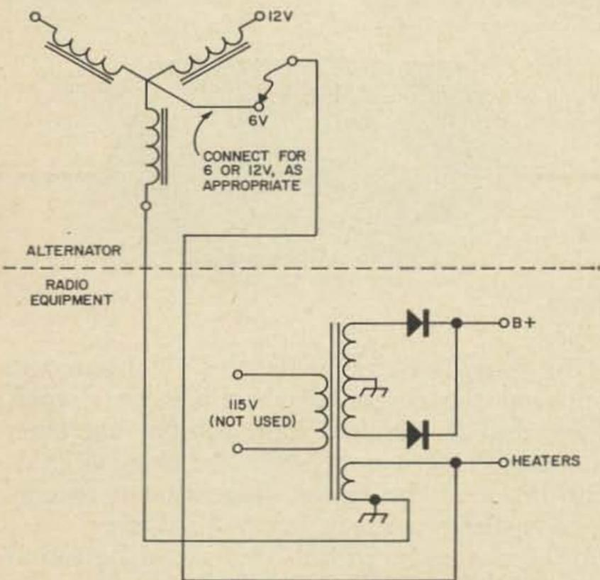
Fig. 7. A simple way to operate radio equipment from low-voltage alternator ac.
