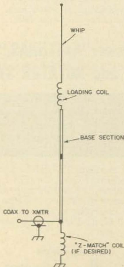
Hooking up the Go-Go Mobile antenna with a Z-match.
