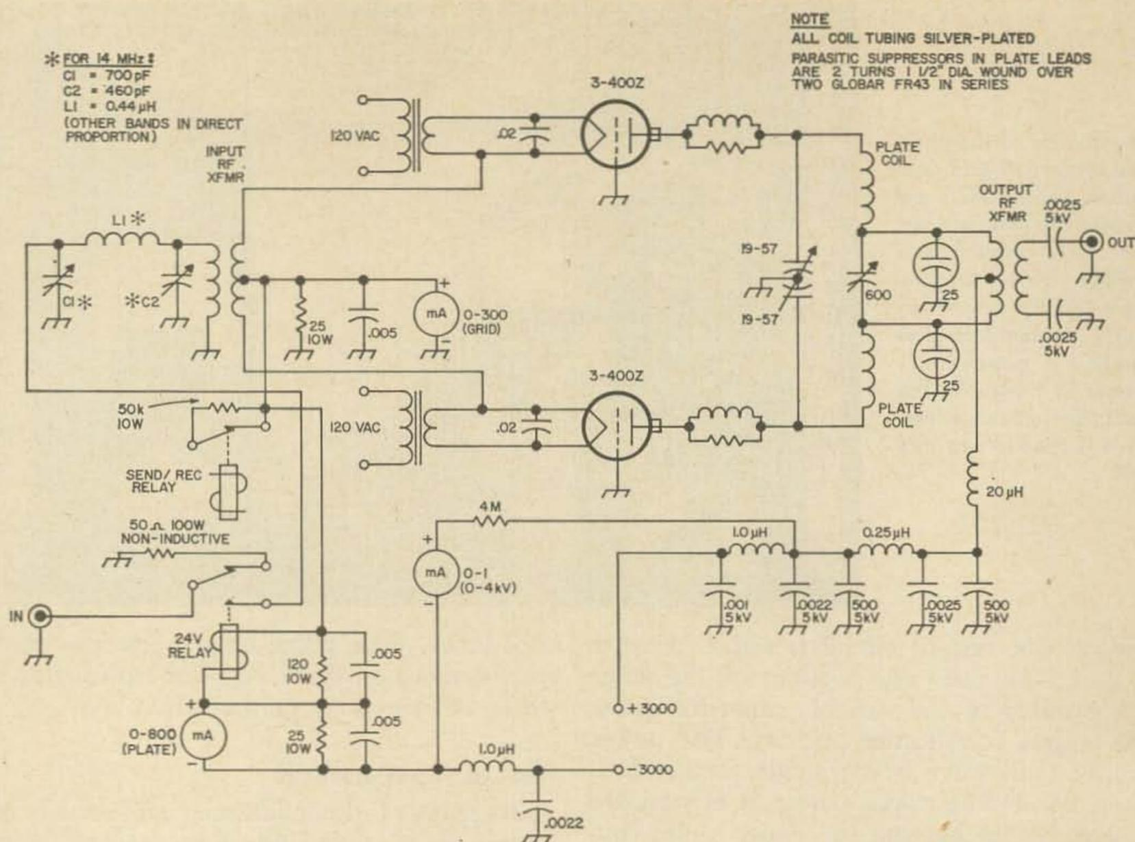
Fig. 1. Schematic of the push-pull grounded-grid class-B linear amplifier. The dual 19-57 pF capacitor in the plate circuit was made from a surplus unit, 0.25 spacing, by removing all but four stator plates per section.
