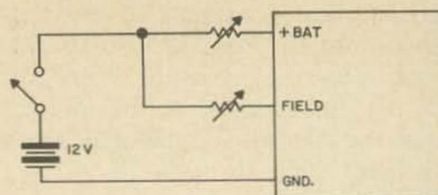
Fig. 6. Arrangement for adjusting the field current to a constant value when the alternator is used to supply ac.
