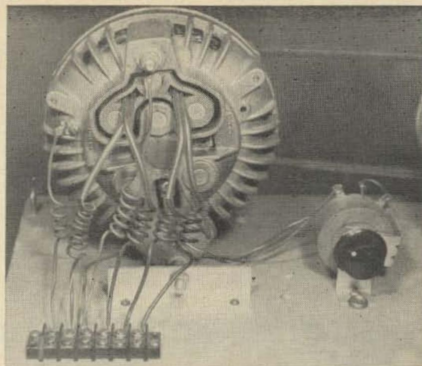
Fig. 8. Method of bringing leads out of the alternator housing without drilling holes in it.
