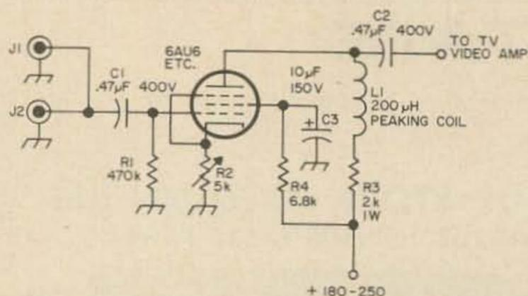
Fig. 7. TV set video preamp. Most TV sets need additional amplification for satisfactory results from one volt of video.
