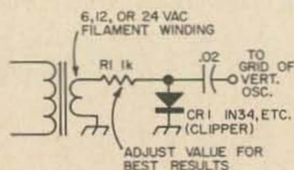
Fig. 10. Vertical oscillator line lock circuit.
