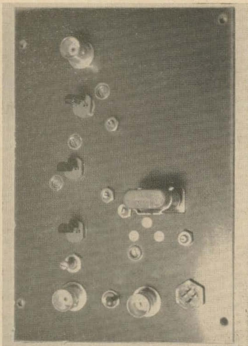
Top view of the FET two meter converter.
