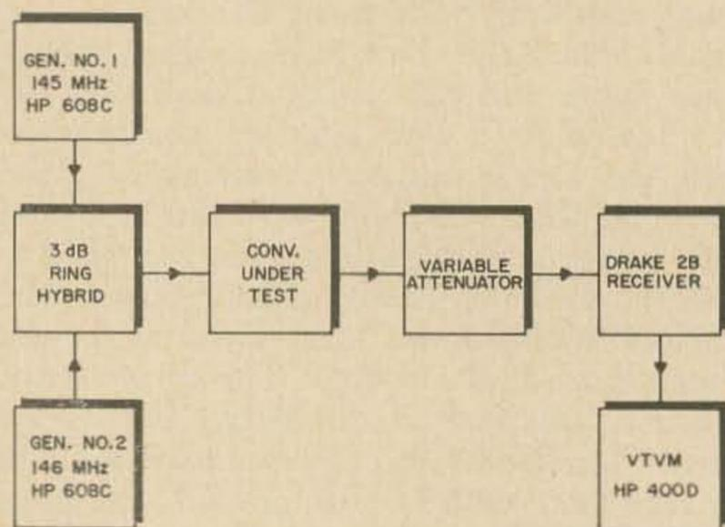
Fig. 2. Test setup used for cross modulation measurements.
