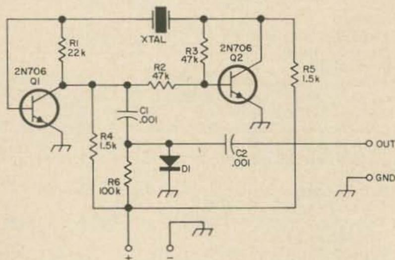
Fig. 1. Schematic of the Multical.
