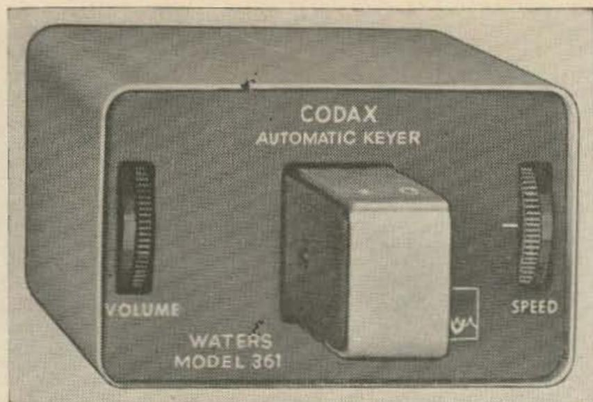
The built-in key of the Waters keyer requires only 20 grams pressure for operation. This keyer will operate for more than 400 hours on its self-contained batteries.
