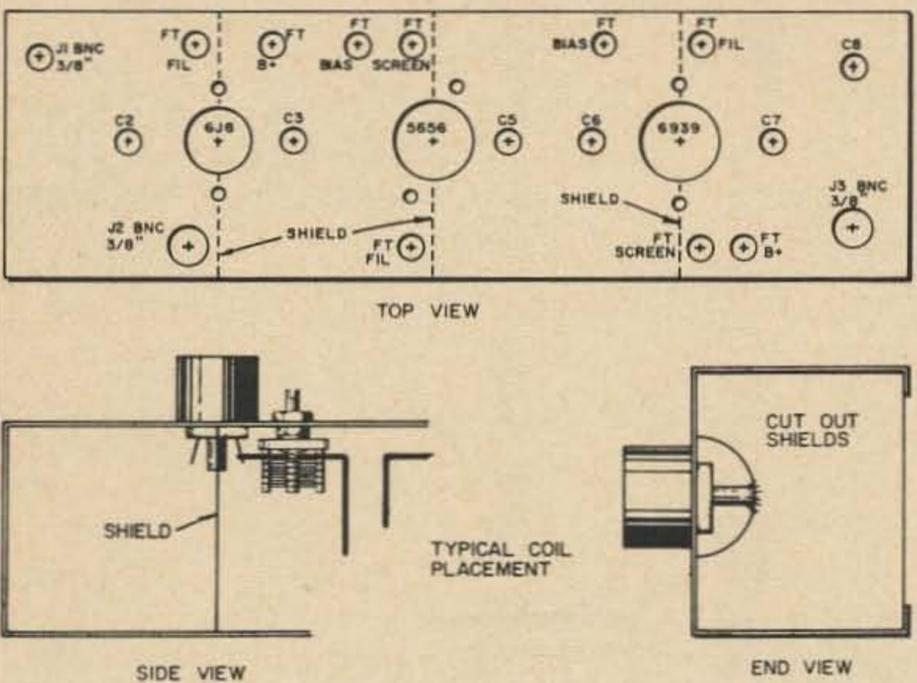
ALL COILS MADE WITH NO. 14 OR 16 TINNED OR SILVER WIRE BEND INTO SHAPES SHOWN AT RIGHT
