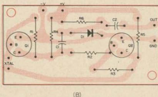
Fig. 2. Suggested printed circuit board layout for the Multical. A gives the copper side, B the component side. A board for the Multical is available for \$1 from the Harris Company, 56 E. Main Street, Torrington, Conn.
