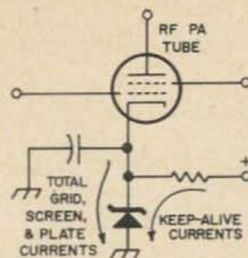
amplifiers is large-signal rf power amplification. The zener diode can fill a very useful spot here. It can replace the cathode bias resistor, offering a bias voltage quite independent of tube current. Fig. 13 shows a zener in this application.
