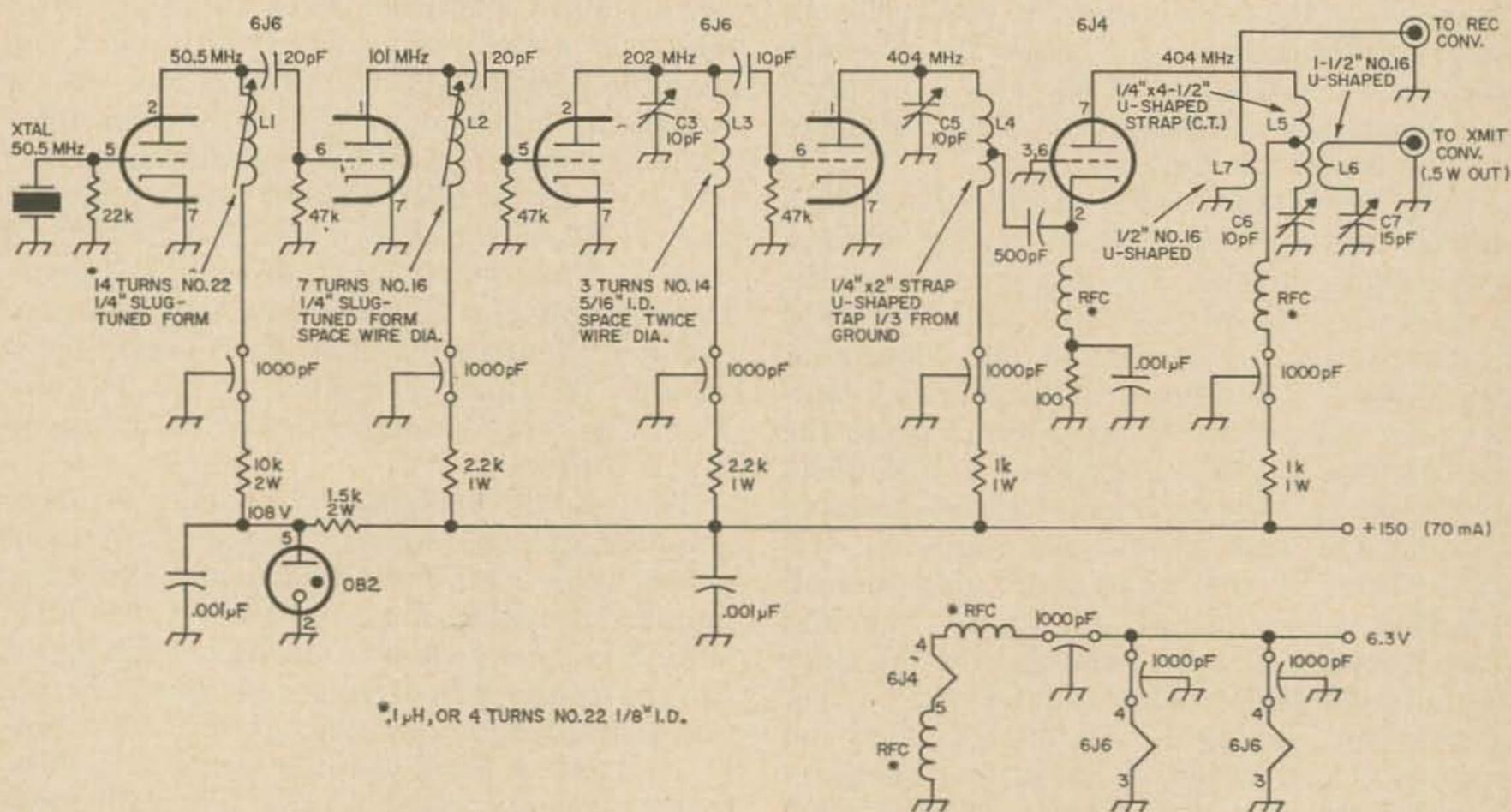
Fig. 1. Schematic of the local oscillator and multipliers for K6RIL's transmitting converter for 432
