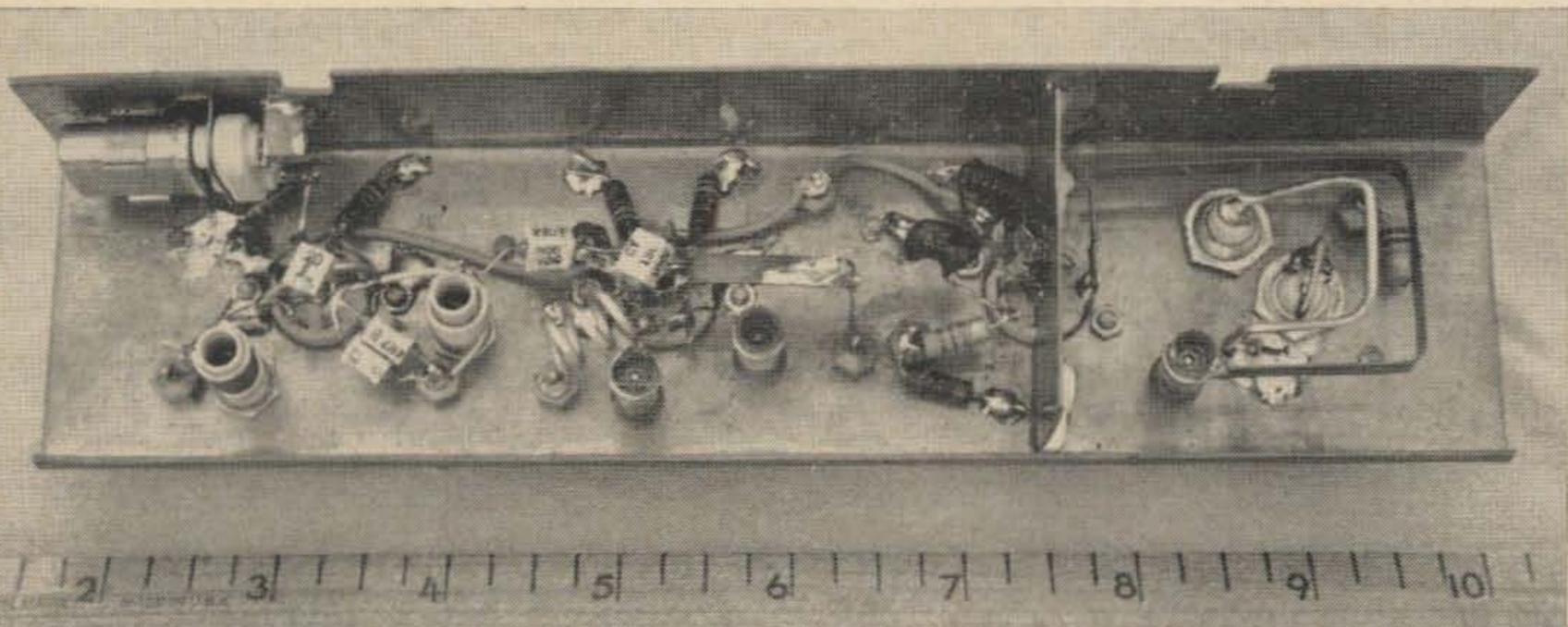
Local oscillator and multipliers shown in Figs. 1 and 2. The crystal is at left and output is at the right. Notice that two output links are shown. The
