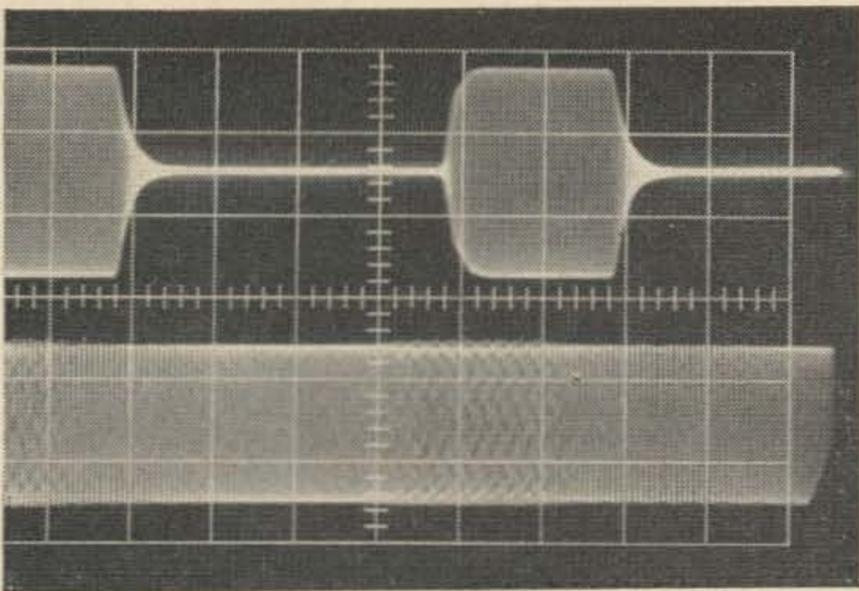
Fig. 3. Upper-modulation pattern from transmitter. Lower-carrier pattern (455 kHz) observed on HQ 160 receiver. Both viewed simultaneously. Moire on carrier caused by double pattern on scope.
