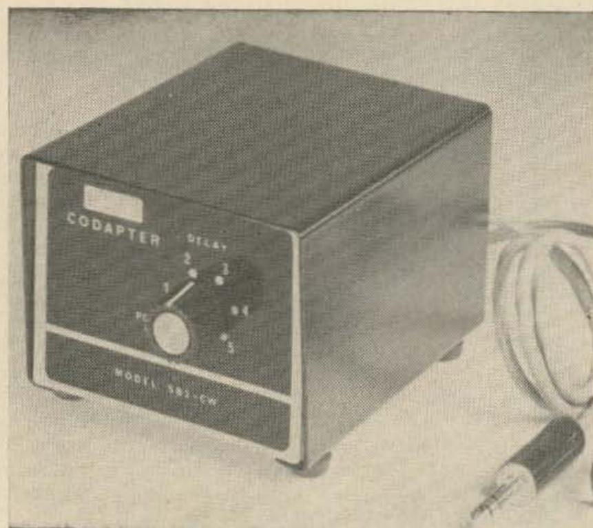
SBE's "Codaptor" allows an SSB transceiver to be keyed with a straight or semi-automatic key. After the key is opened, the transceiver T-R relay remains closed for a time selected by the front-panel "Delay" control.
