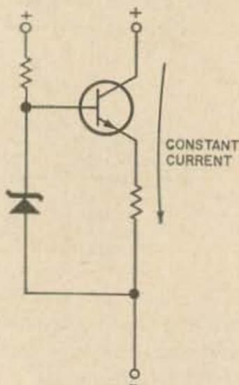
amps. This current through R2 must bring the junction between R1, R2 and the zener to 6 volts. Now there must be 14 volts across R1 and that yields 175 microamps through it. The meter gets 50; 125 microamps pass through the zener and its series resistor. We have it! From the junction through the zener we lost three volts, by design; the remaining three volts at 125 microamps fixes R3 at 24kΩ.
