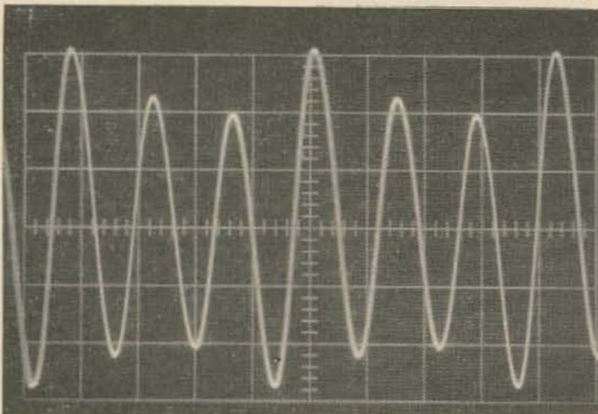
Fig. 1. Output of a frequency tripler.
