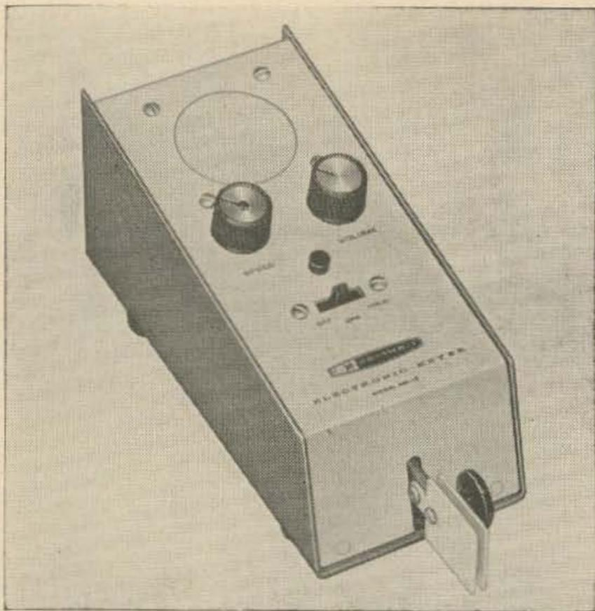
The Heathkit HD-10 has a paddle similar to those of semi-automatic keys. The "hold" position of the on-off switch is for transmitter tune-up.
