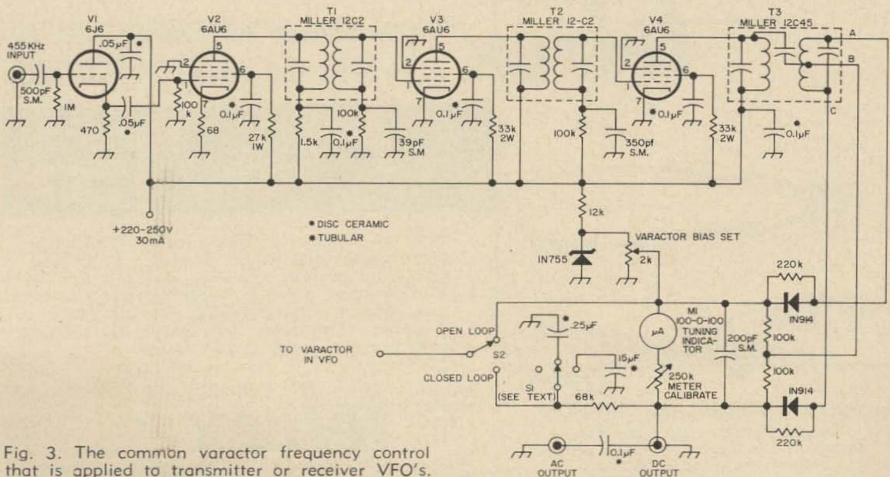
Fig. 3. The common varactor frequency control that is applied to transmitter or receiver VFO's.
