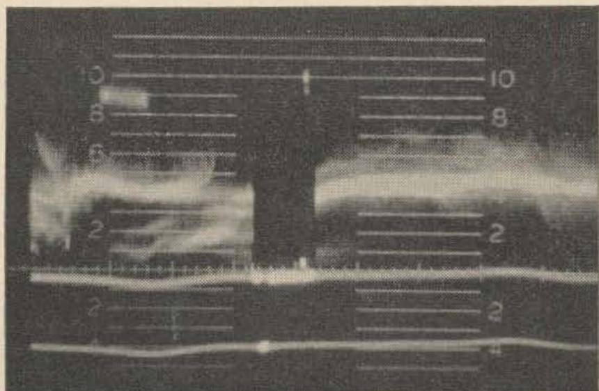
Fig. 2. Standard TV signal. Scope sweep 30 Hz amplitude one volt. The blank interval in the center is vertical blanking. Ten corresponds to 100 IRE units on the scale.
