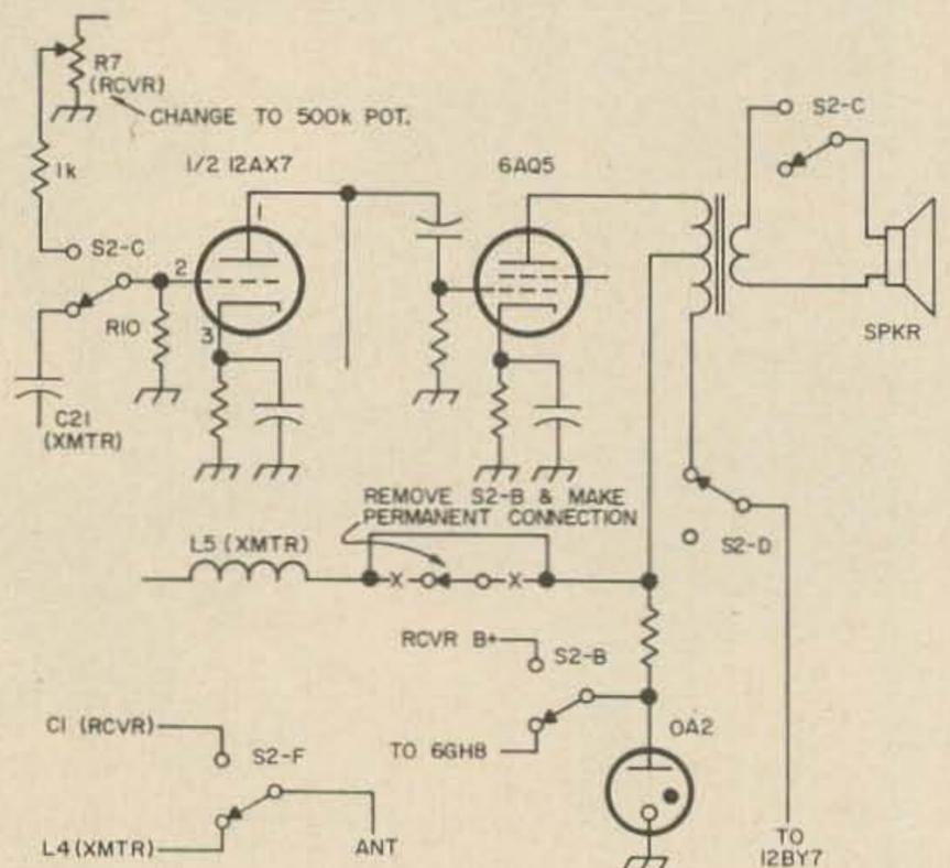
Fig. 3. Break-in schematic for operating the receiver with the Poor Man's 220 Transmitter.
