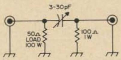
50 Ω LOAD MAY BE ANY DUMMY LOAD WHICH WILL DISSIPATE POWER FROM TRANSMITTER USED. THE HEATH ANTENNA WORKS VERY WELL.
