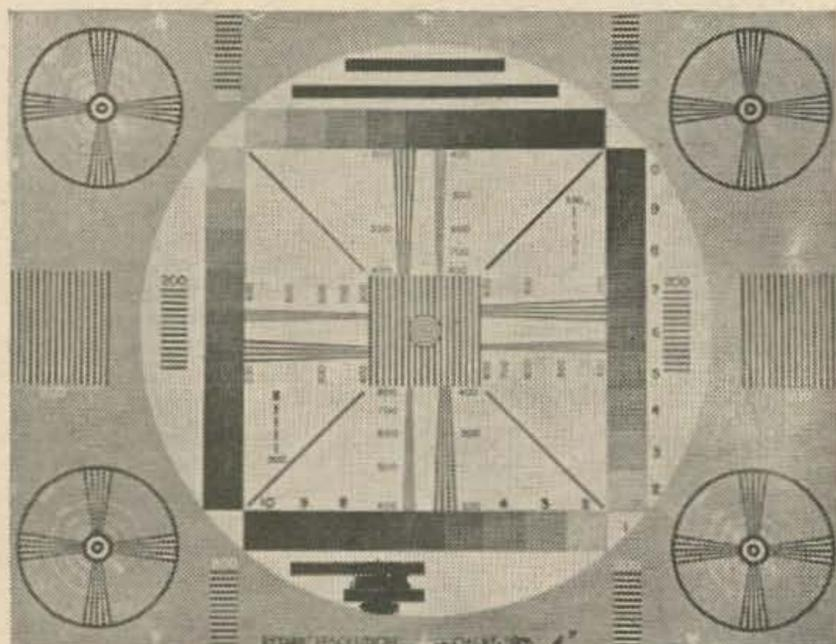
Fig. 8. EIA test pattern
