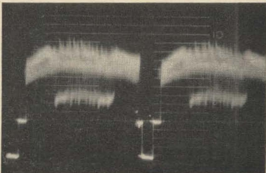
Fig. 3. Standard television signal-horizontal. Scope sweep 7875 Hz. Horizontal sync and blanking are clearly evident. Note also that the black parts of the picture extend down to almost plus 7.5 IRE units.
