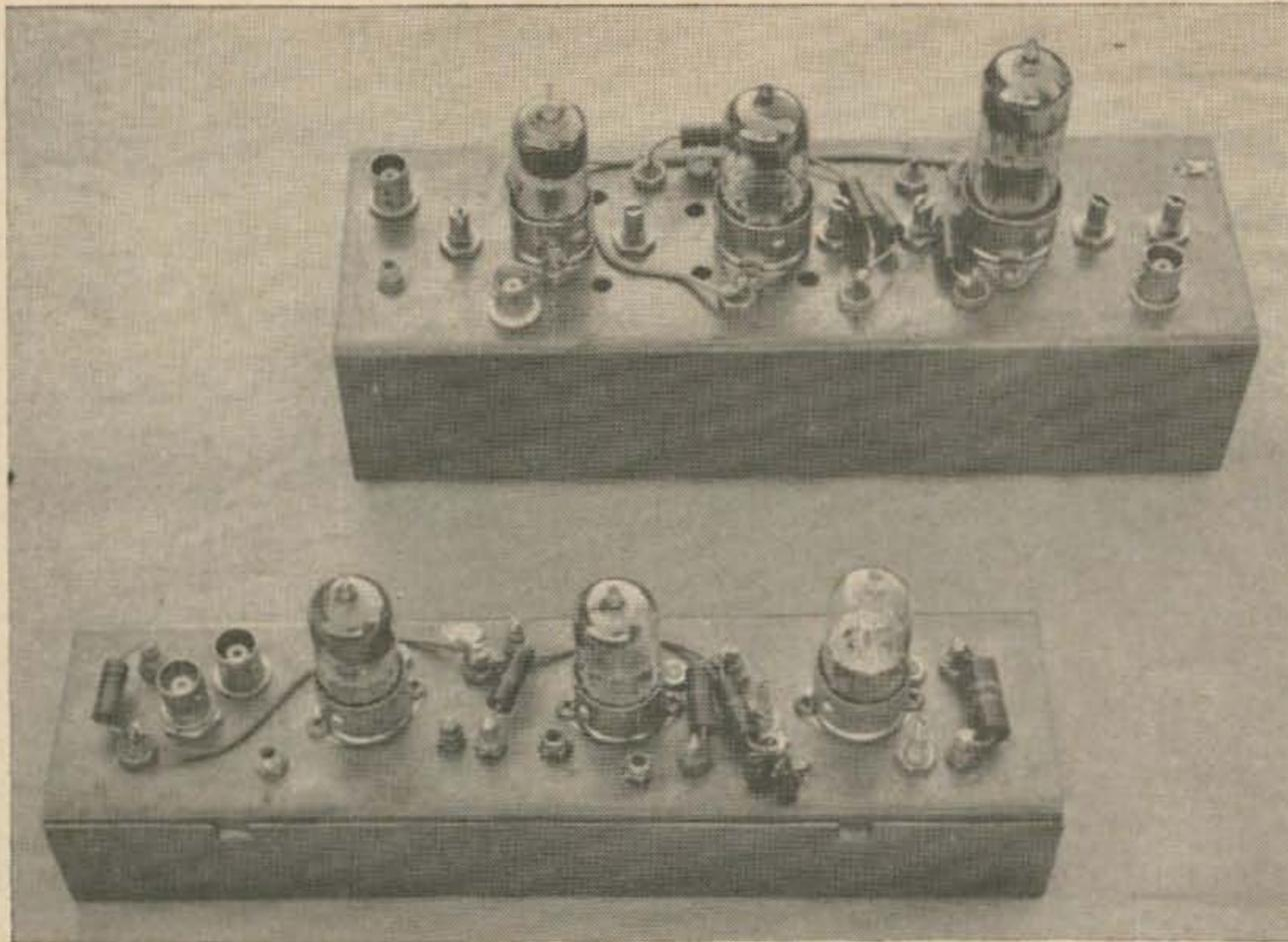
Top view of the 432 MHz mixer (top) and local injection generator.
