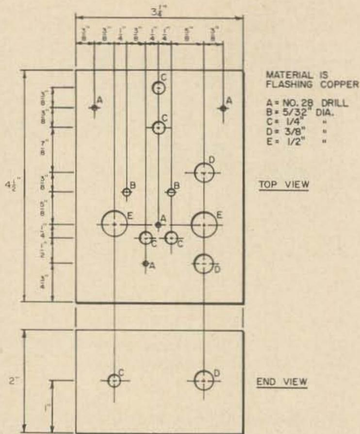
Fig. 2. Layout of the 220 MHz receiver.  $\frac{1}{3}$  size.
