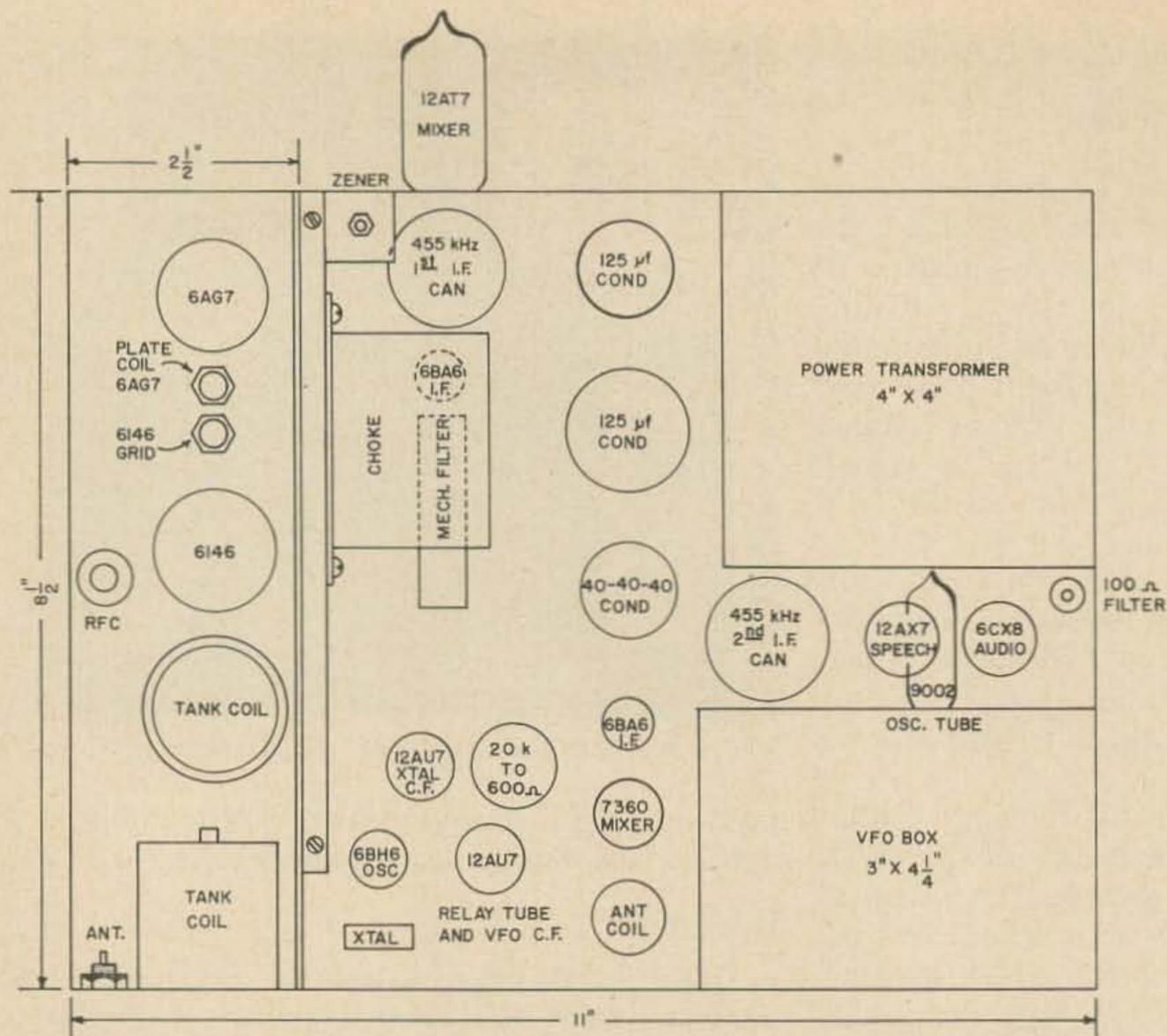
Fig. 3. Layout of El Mariner as built by Ed Marriner W6BLZ.
