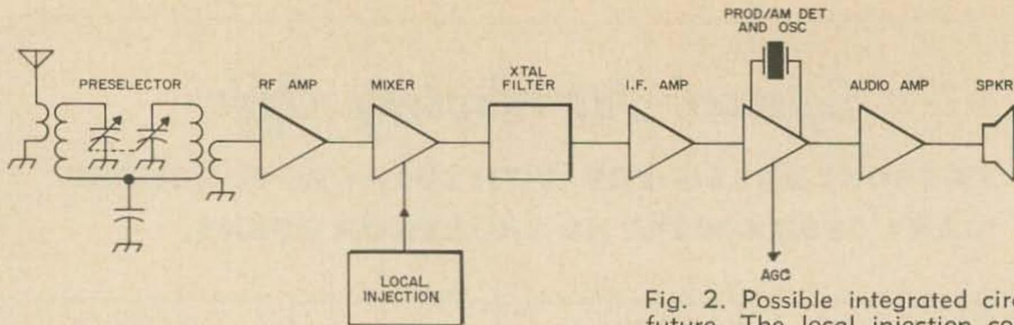
Fig. 2. Possible integrated circuit receiver of the future. The local injection could be a frequency synthesizer or conventional oscillator.
