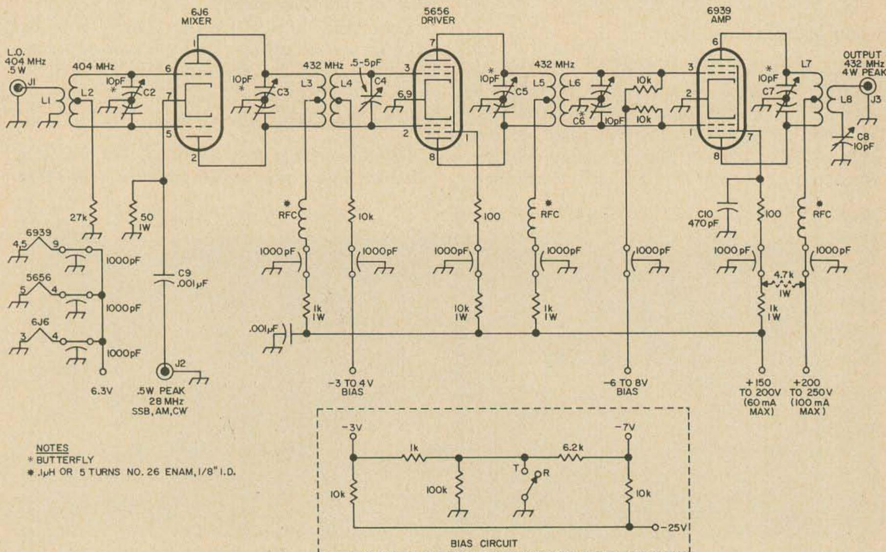
Fig. 3. Schematic of the mixer and linear amplifiers for K6RIL's transmitting converter. L6 should
