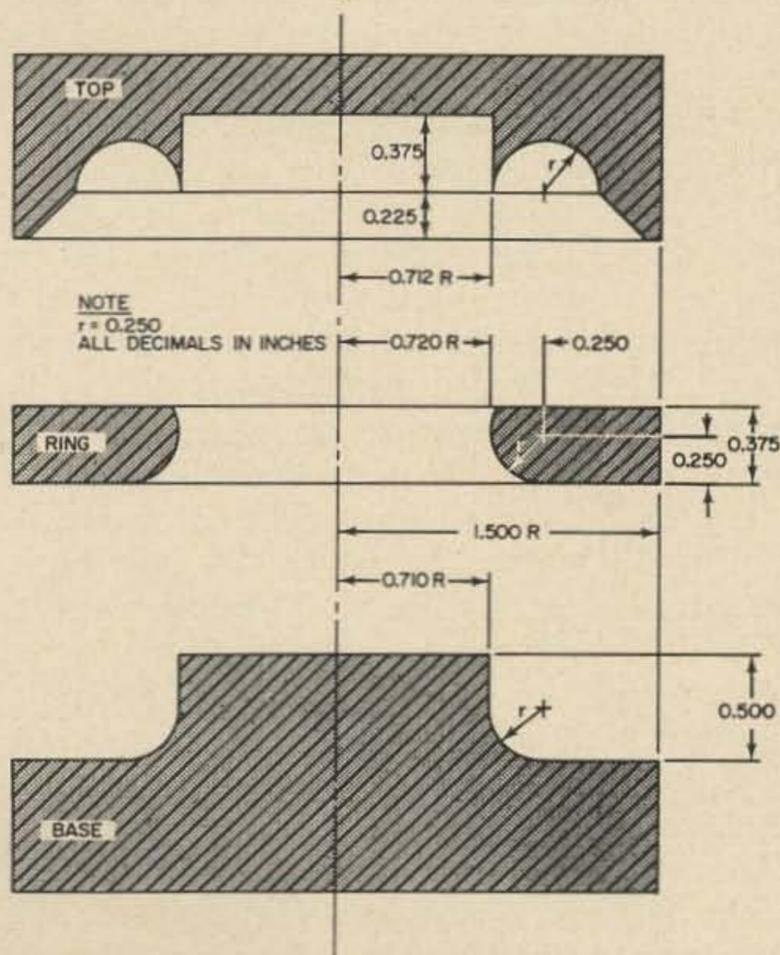
Fig. 2. Cross section of the jig.
