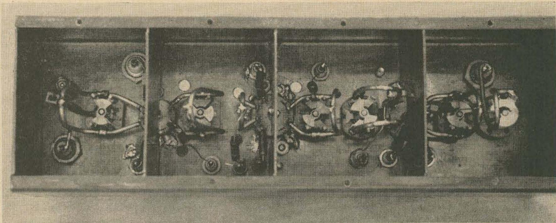
432 MHz transmitting converter. The left compartment is the input from the local oscillator and the 28 MHz exciter. The two center compartments
