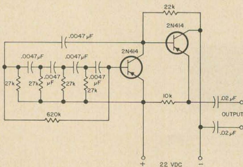
Fig. 5. 1200-Hz tone oscillator for inserting a signal into the microphone jack to produce a signal for tuning. Construction isn't critical.
