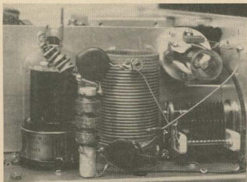
Final amplifier, tank coil and TR switch.
