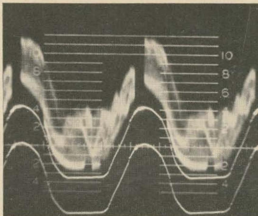
Fig. 9. 60 Hz hum scope at 30 Hz sweep. 120 Hz hum will have twice as many alternations. This amount is severe. Any hum over 10 IRE units is objectionable with levels over 40 IRE units destroying the picture.
