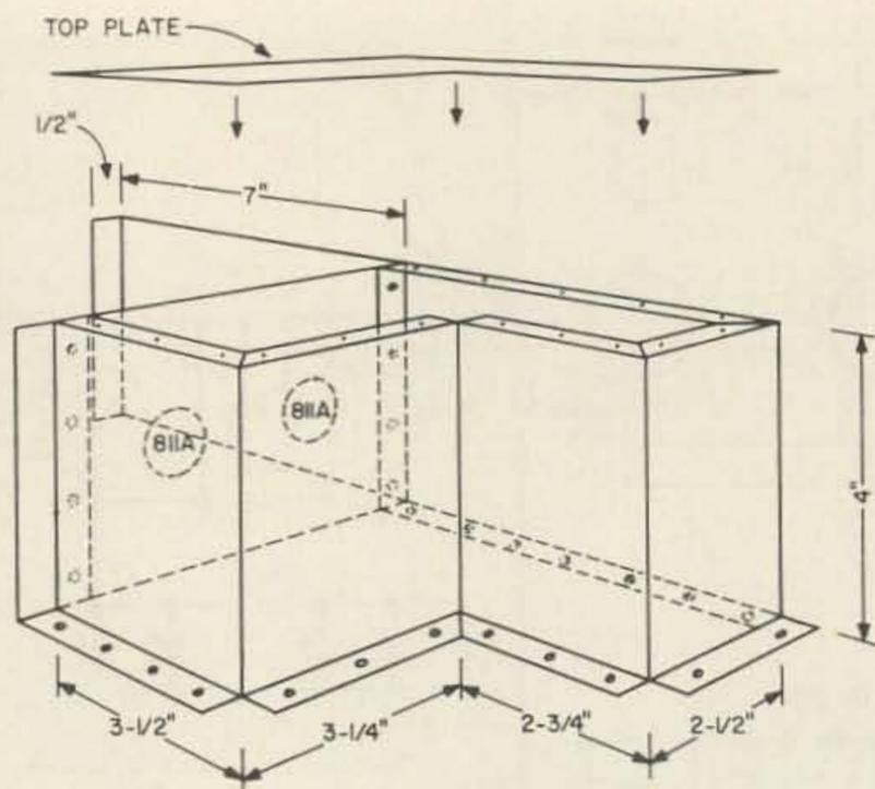
Construction of shield box.
