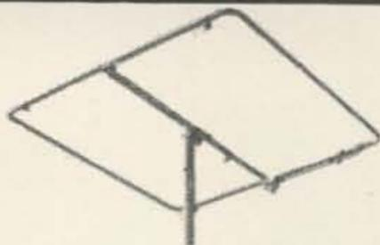
**SQUALO** is a full half wave, horizontally polarized, omni-directional antenna. Outstanding all around performance is achieved through a 360° pattern with no deep nulls. The square shape allows full electrical length in compact dimensions. Direct 52 ohm Reddi Match feed provides ease of tuning and broad band coverage.
