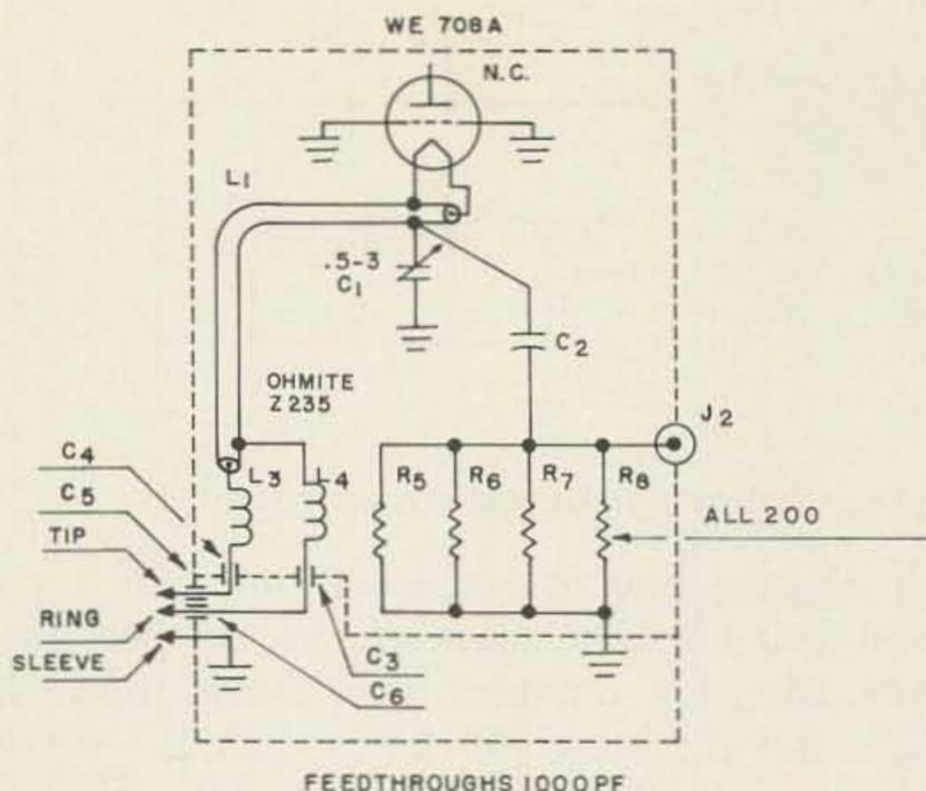
Fig. 4. Circuit of diode noise generator.
