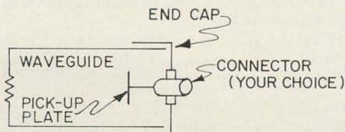
Fig. 2. Detail of pick-up end of attenuator
