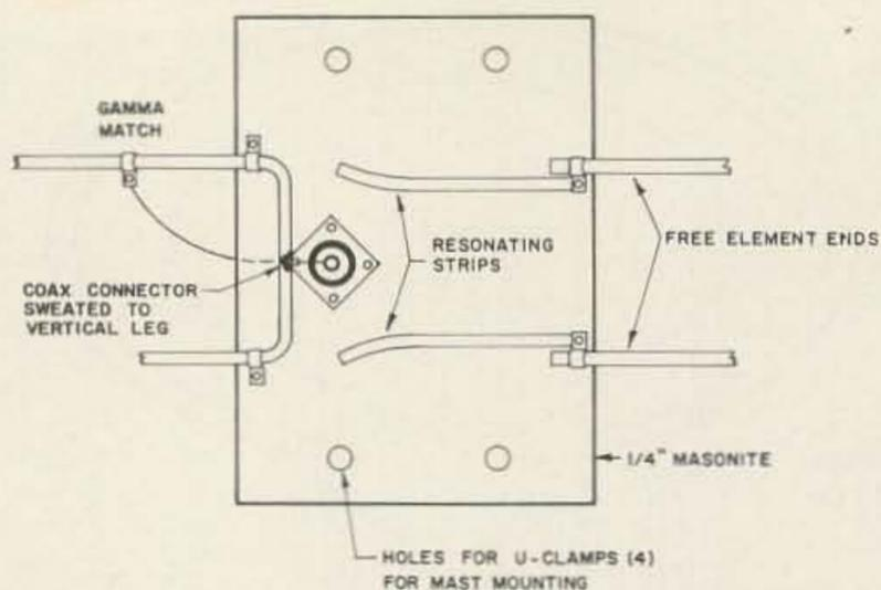
Fig. 2 Double Hula mounting assembly.
