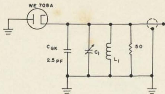
Fig. 2. Basic noise generator circuit.
