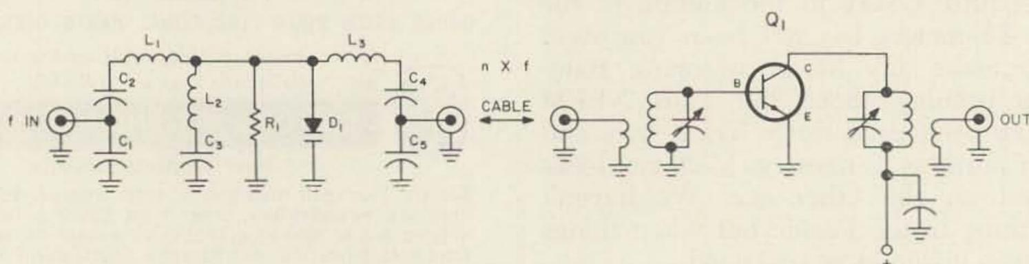
Fig. 2 Parametric multiplier and class C amplifier
