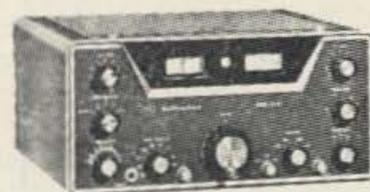
Exceptionally versatile and compact Triple-conversion, super-heterodyne communication-type receiver. Selectivity .5, 2.5, or 5. Sensitivity less than 1  $\mu$ V on AM, less than  $\frac{1}{2}$   $\mu$ V on SSB/CW. T-Notch filter, I.F. type noise limiter, 100 kc xtal Calibrator.
