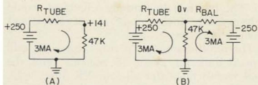
Fig. 2 Balancing input stage
