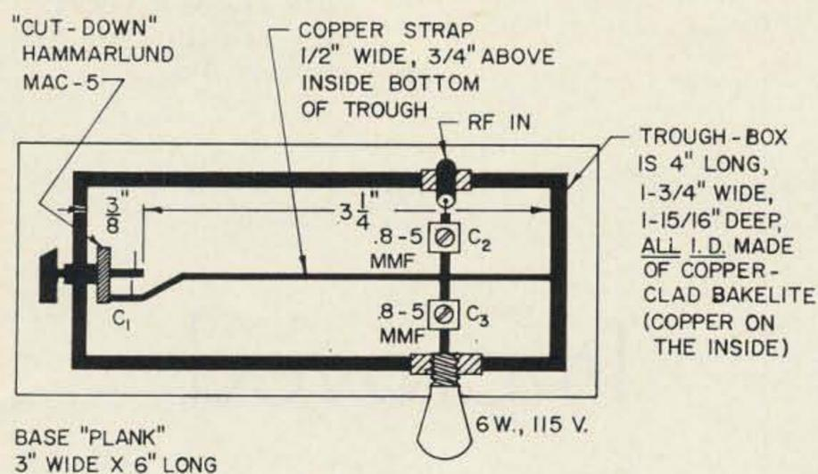
Fig. 1—Visible UHF power load, 6 watts. (At least!)
