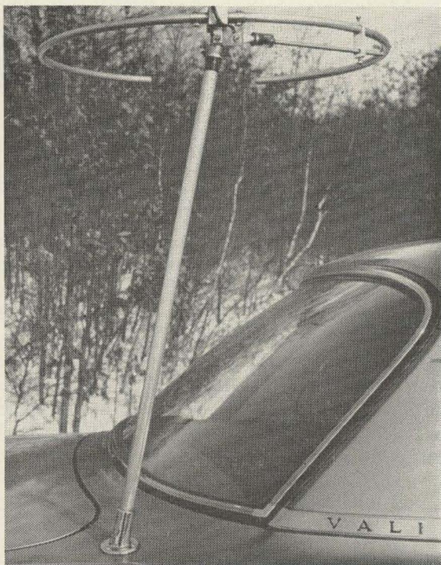
Any marine shop has them at an average of \$1.75 and they conveniently accept a 3/4" OD mast with a nice press fit. The only modification recommended prior to bolting it on your car is to drill and tap the "snoot" to accept one or two set screws of the type used in radio knobs. They will keep the mast from turning no matter how enthusiastic your driving may be yet are small enough to prevent accidental crushing of the mast due to over-tightening.
