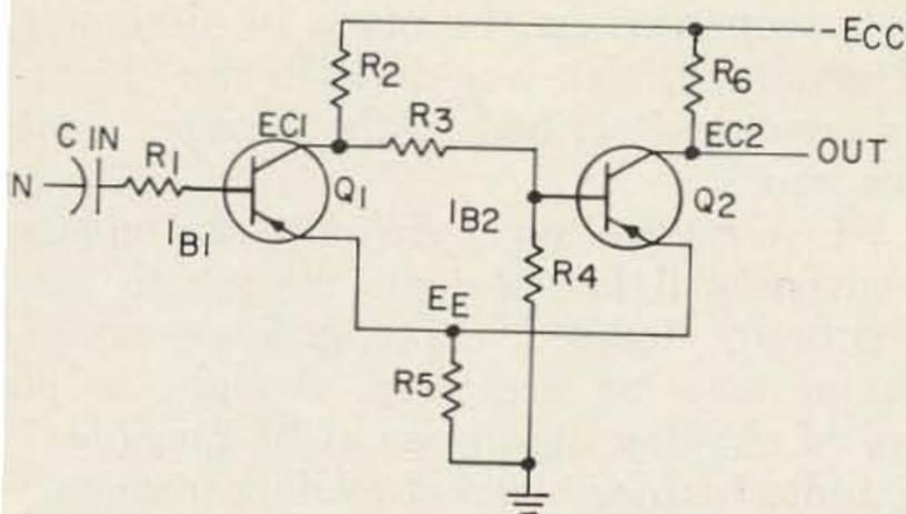
FIG. 2 TRANSISTOR SCHMITT
