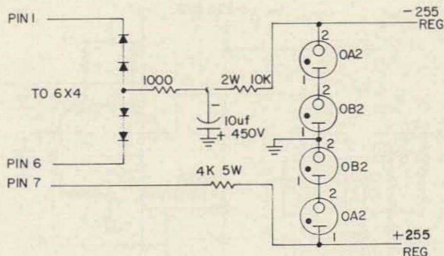
Fig. 3 Balancing power supply
