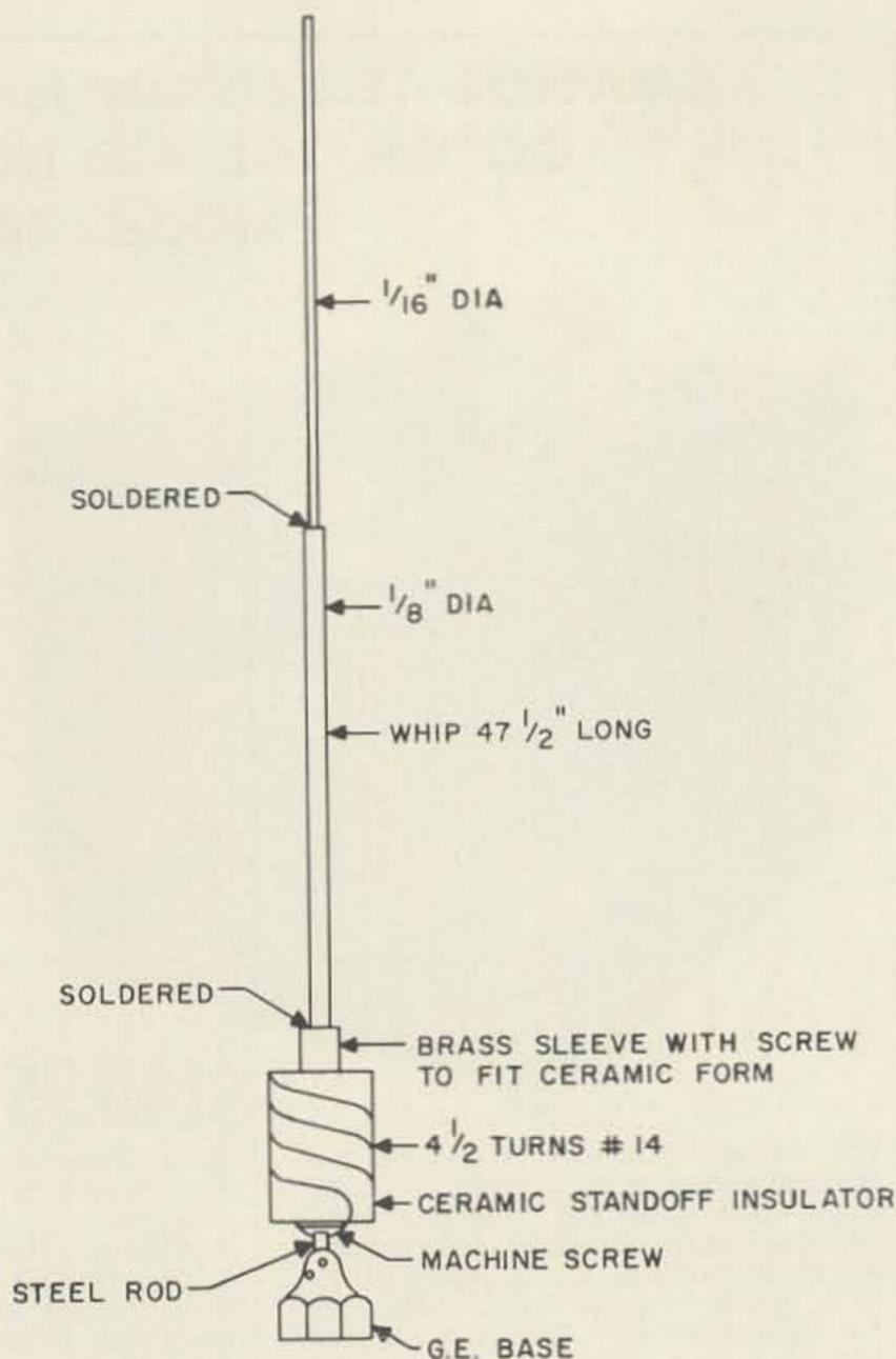
the coupler for a length of  $\frac{1}{4}$ ", the base of the whip is inserted from the opposite end and the three are then soldered together to make a rigid unit. Care should be taken to keep the solder off the threads of the machine screw.
