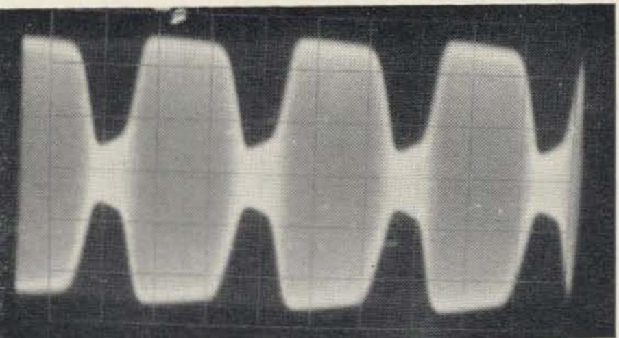
Severe distortion of the modulated RF!
