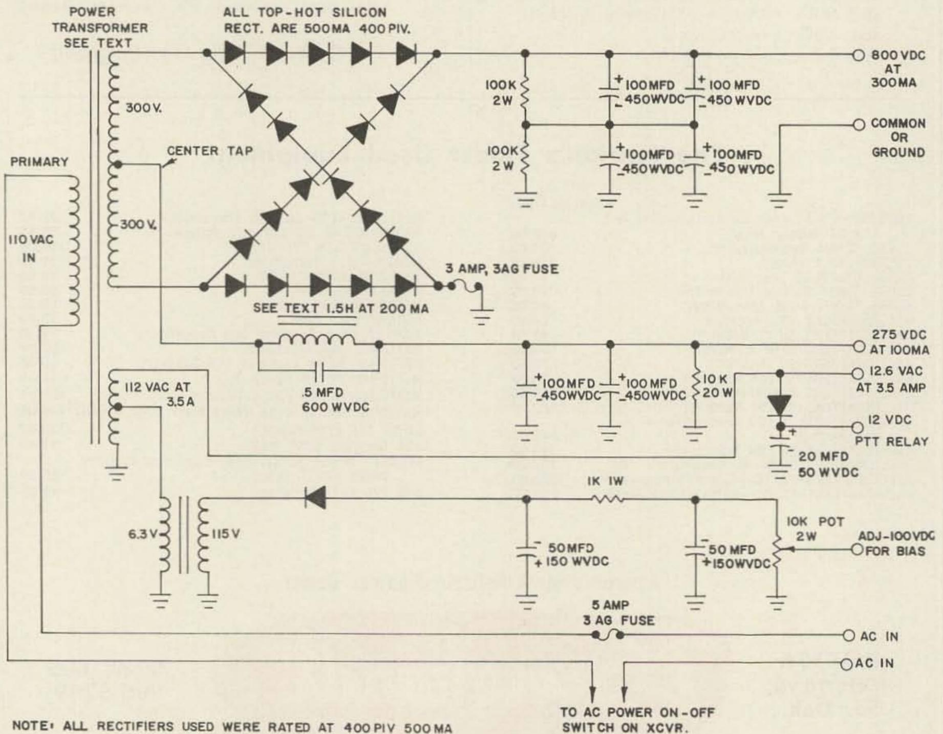
Omit .5 mfd capacitor across choke. Note that the winding labeled 112 vac should be 12.6 vac.
