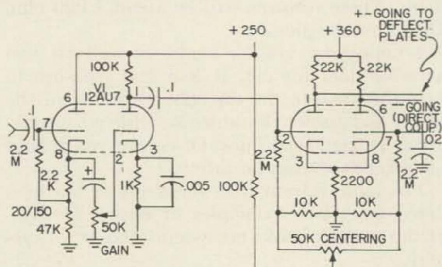
Fig. 1 Original OL-1 amp. circuit
