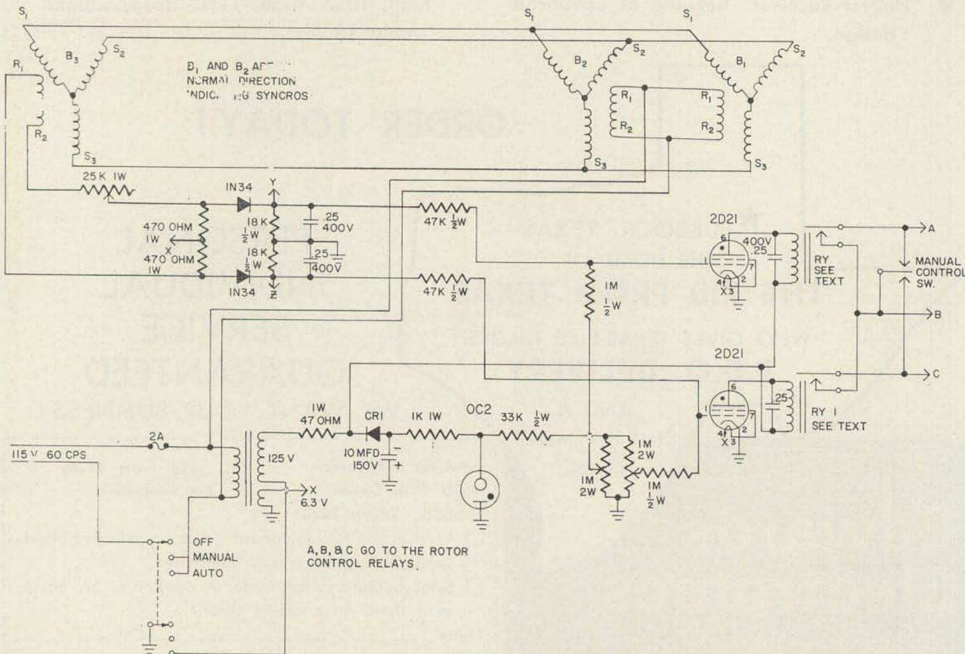
Delete connection from bottom of 125 v secondary to 6.3 v winding. Delete connection from center of left 1 M/2 W potentiometer to top of this pot. The top relay is RY 2.
