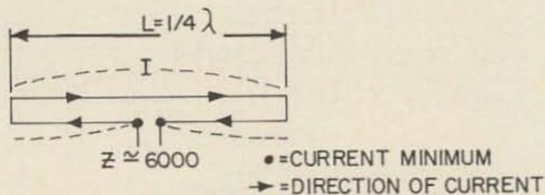
FIG. 3 THE  $\frac{1}{4}\lambda$  FOLDED DIPOLE
