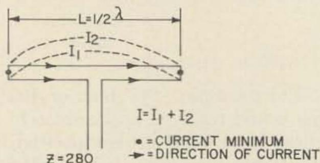
FIG. 1 CURRENT DISTRIBUTION IN  $\frac{1}{2}\lambda$  FOLDED DIPOLE
