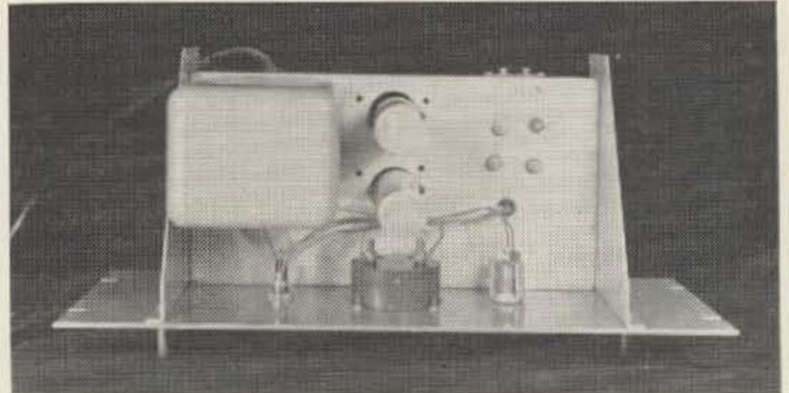
The rectifiers (diodes) used in the original unit were purchased from TAB (111-54 Liberty Street, New York 6, N.Y.) for \$1.15 each. The units selected are the 12 ampere, 70 vrms (100 piv) silicon power diode studs. Be sure to use mica (or equivalent) insulating washers when mounting the diodes to the chassis.
