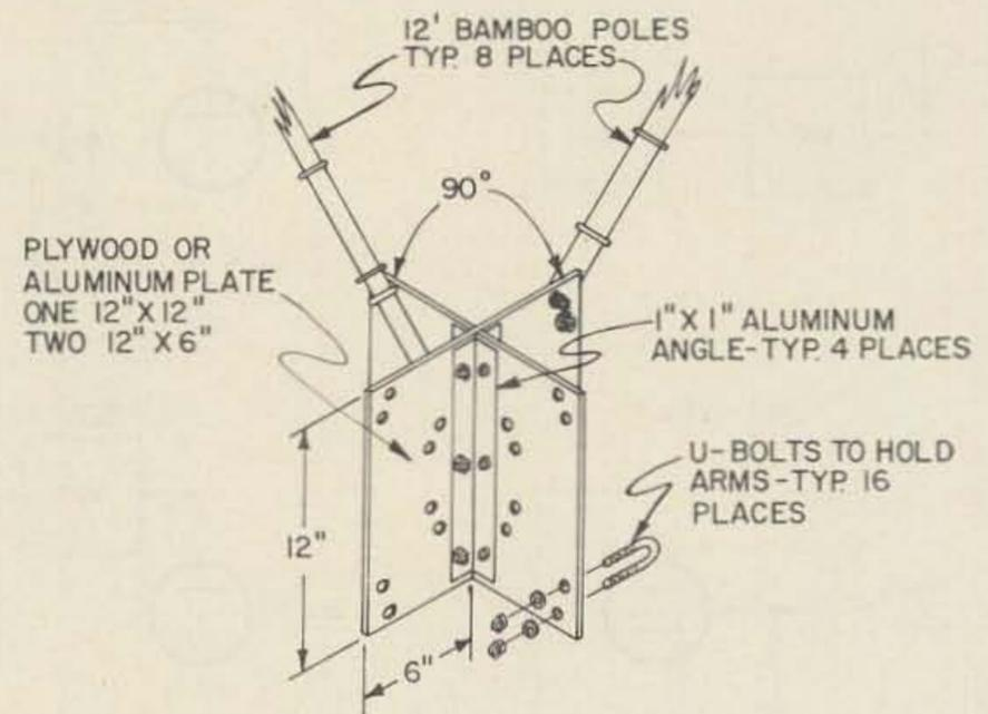
FIG. 2 SPIDER CONSTRUCTION DETAIL
