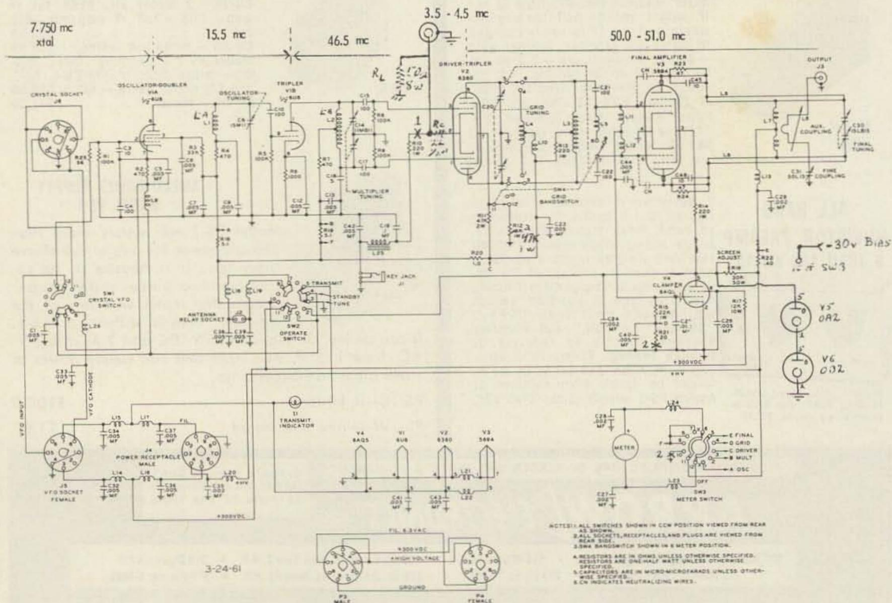
watt carbon resistors in parallel; making the connection on each end of the resistors close to the resistor bodies. Cut off excess wire from each end, leaving one lead at each end to make the connections. Now connect and solder one end of  $R_L$  to the junction of  $R_C$  and the RG-58/U. Solder the other end of  $R_L$  to the ground lug next to the V-2 socket.
