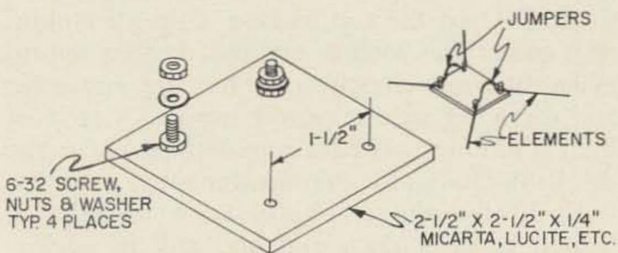
FIG.3 SEPARATOR PLATE DETAIL
