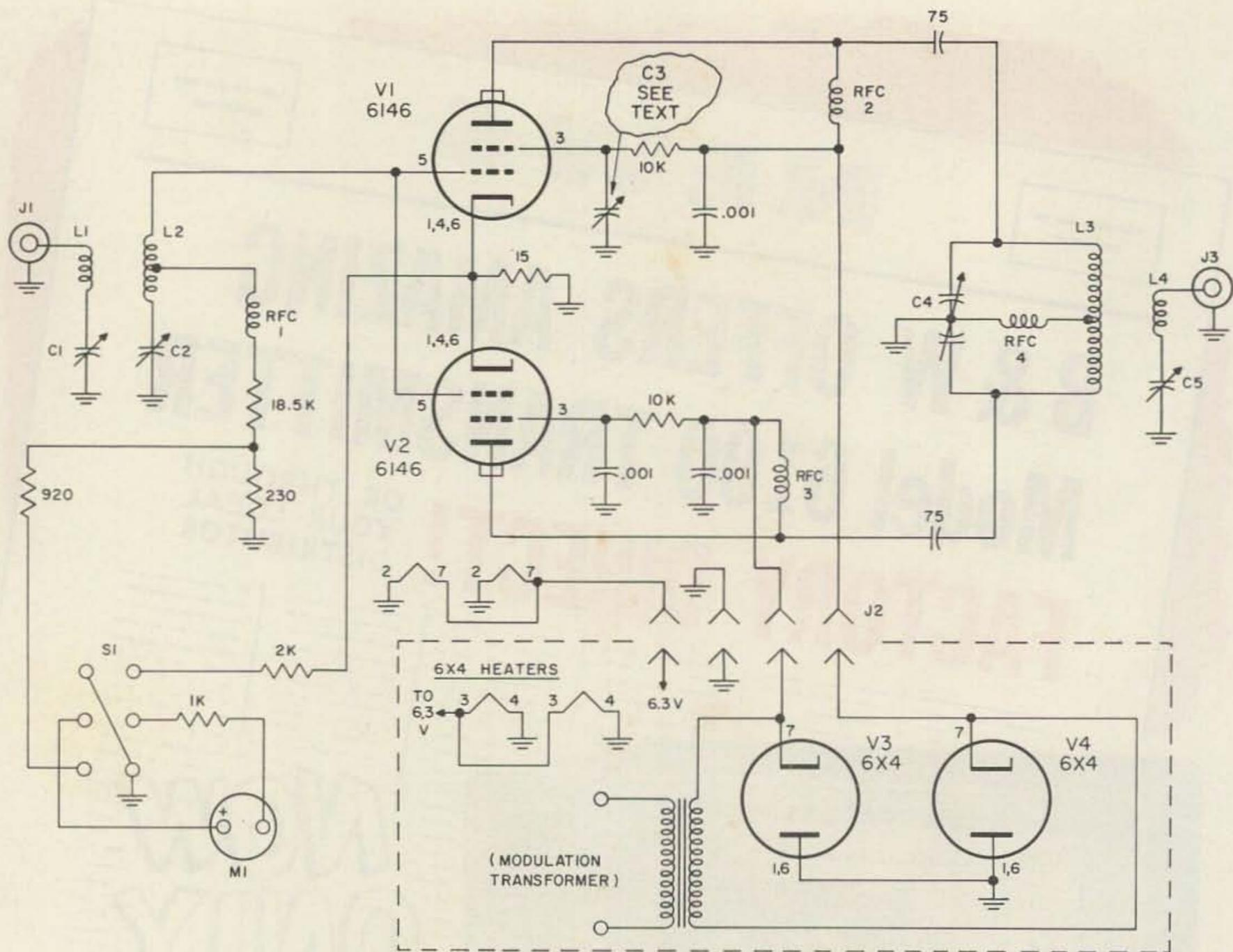
at a time, the non-conducting tube is an effective "neutralizing capacitor" for the other tube.
