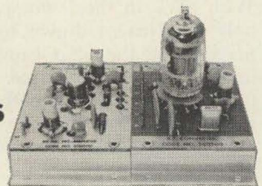
Unbeatable performance at an unbeatable price. **Only \$10.00 ppd.!** Complete with 6U8A, 6CW4 tubes and choice of 36 mc. crystal for 14-18 mc. output or 49.4 mc. crystal for broadcast band output. Fully assembled as shown, tested and guaranteed. .1 microvolt sensitivity. Noise figure 2.5 db.
