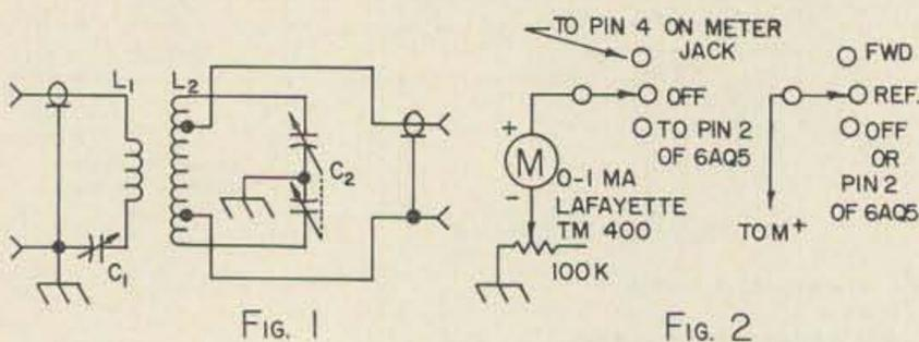
Fig. 1. Coupler diagram.
