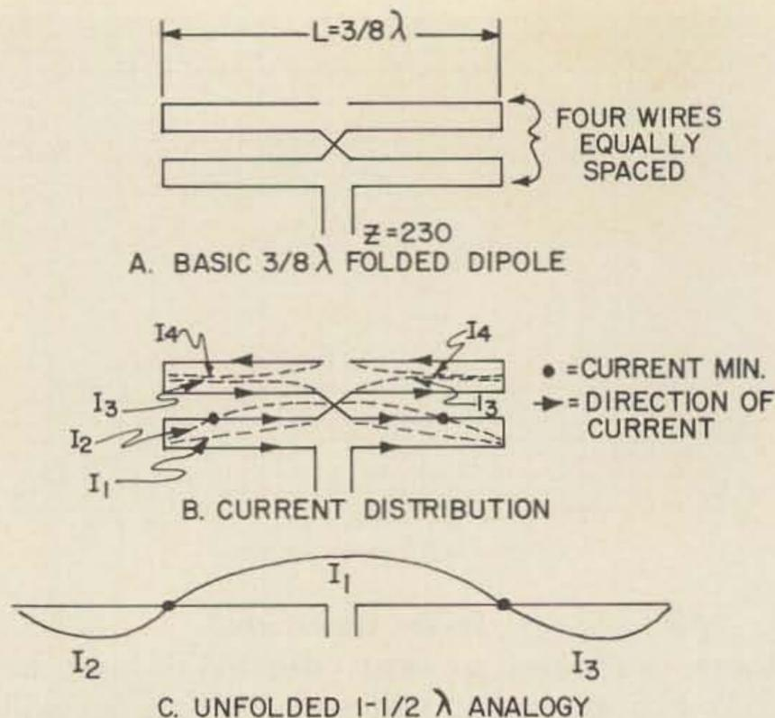
FIG. 2 THE  $\frac{3}{8}\lambda$  FOLDED DIPOLE
