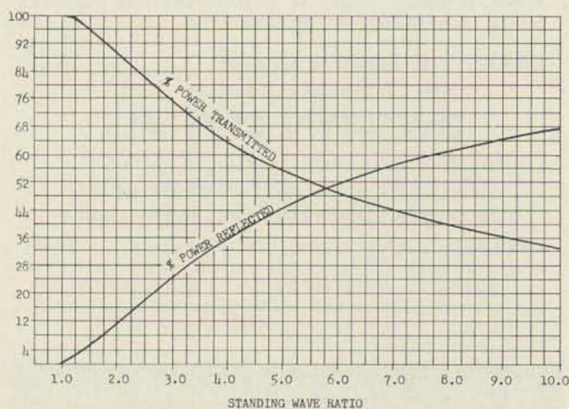
SWR vs % Power Transmitted and Power Reflected
