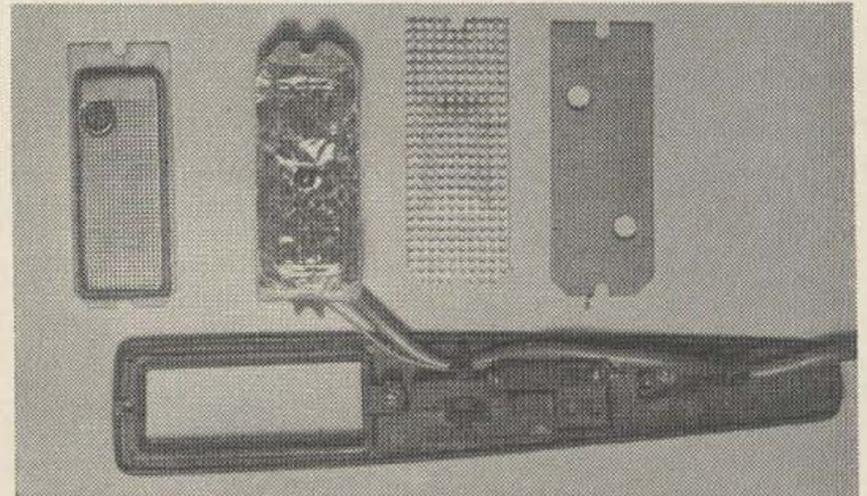
Microphone disassembled and ready for repair. The rectangular object with leads attached is the cartridge.
