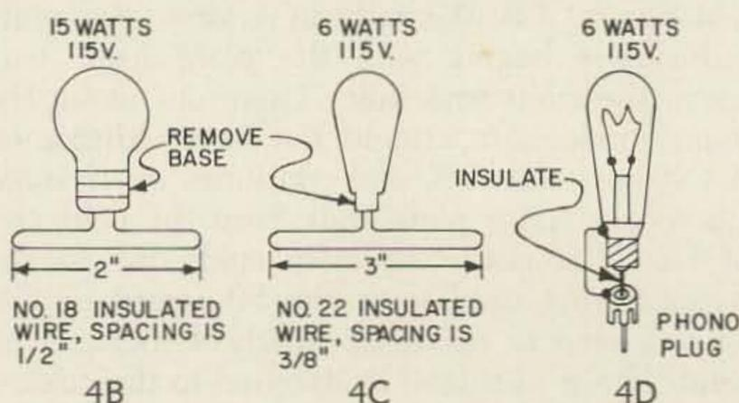
Fig. 4D—Note: 4B and 4C are inserted inside the cavity alongside L1. 4B, 4C, and 4D lamp bulb loads are shown for 432 mc
