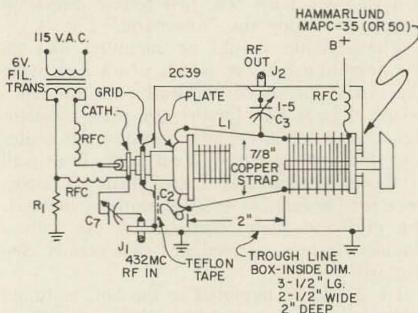
Fig. 4A—2C39 grounded-grid rf final, 432 mc
