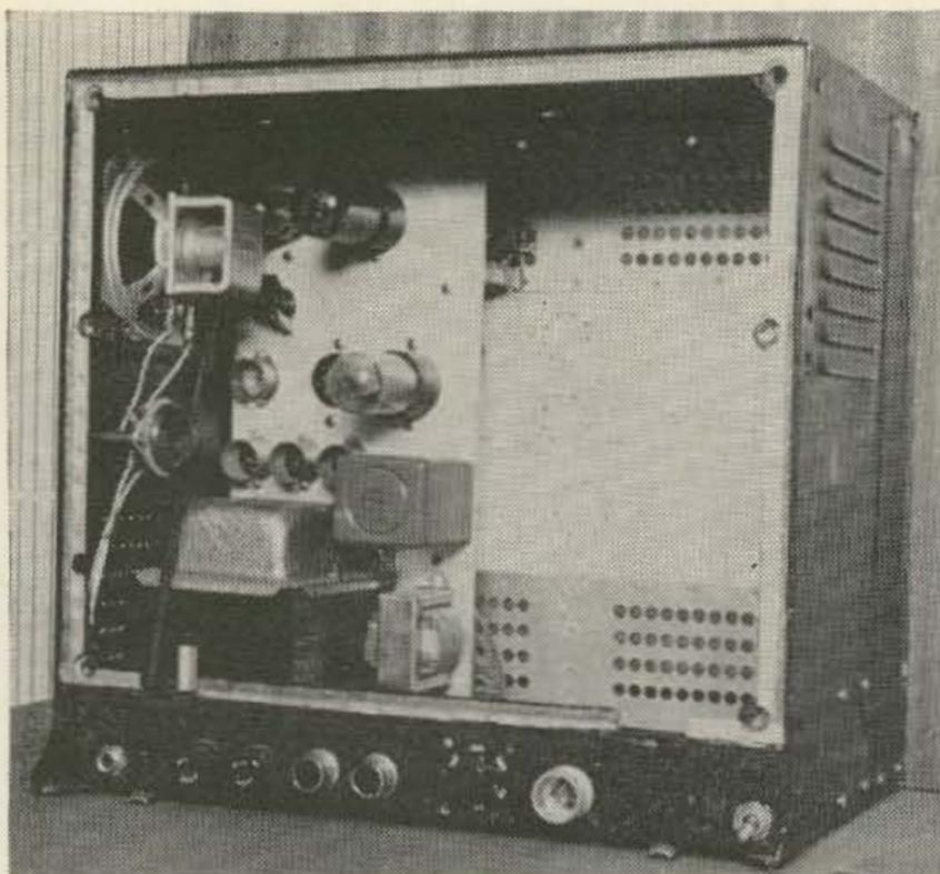
6) View of cabinet and power supply-modulator chassis.
