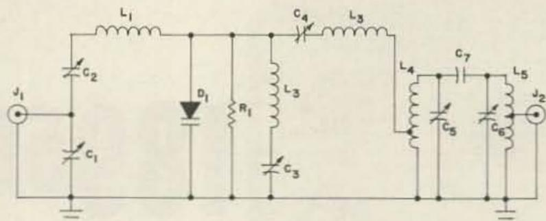
Fig. 3. Schematic diagram of varactor tripler to 432 mcs. See parts list.
