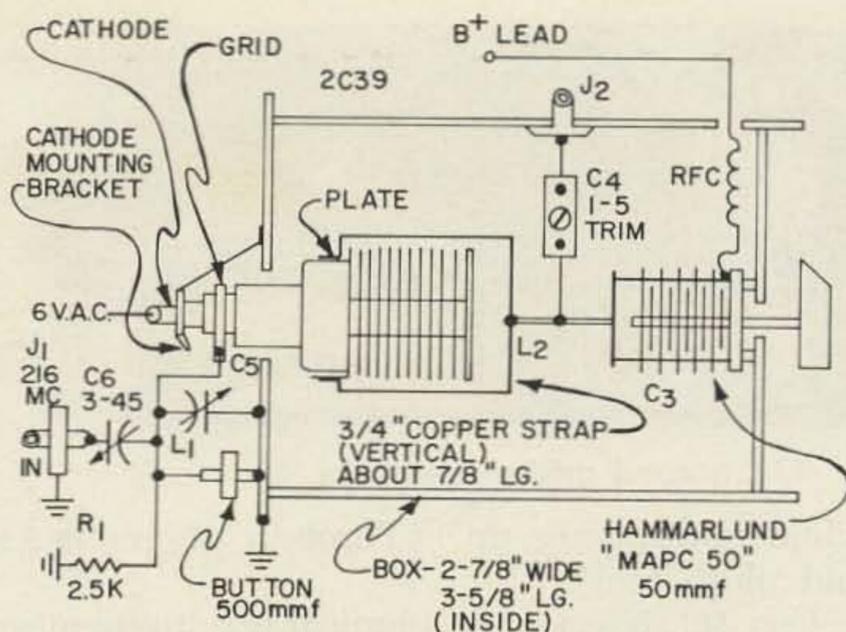
Fig. 3A—Doubler 216 to 432 (top view). L1 = Copper strap,  $\frac{1}{2}$ " wide,  $2\frac{1}{2}$ " long, spaced  $\frac{1}{2}$ " from front wall
