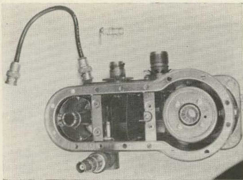
3) Main cavity body after modification. Note how the receiver input link is connected to the N connector.
