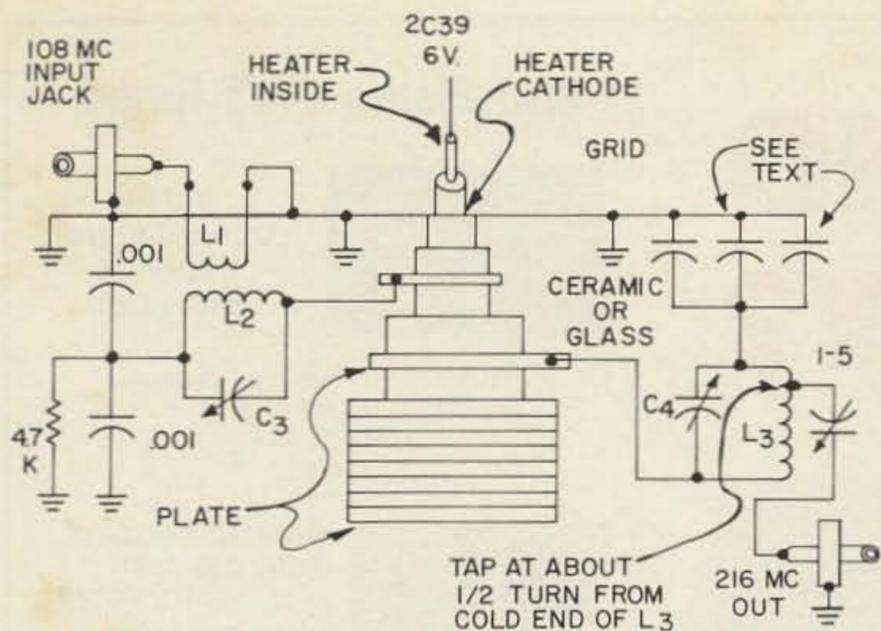
Fig. 2—Power doubler, 108 to 216 mc. L1 = 3 turns interleaved in cold end of L2. L2 = 4 turns no. 16 copper  $\frac{5}{8}$  long,  $\frac{1}{2}$  inch diameter. L3 = 3 turns copper strap,  $\frac{1}{4}$  inch wide,  $1\frac{1}{2}$  inches long winding,  $\frac{9}{16}$  inch diameter O.D. Note: L2 connects to grid ring.
