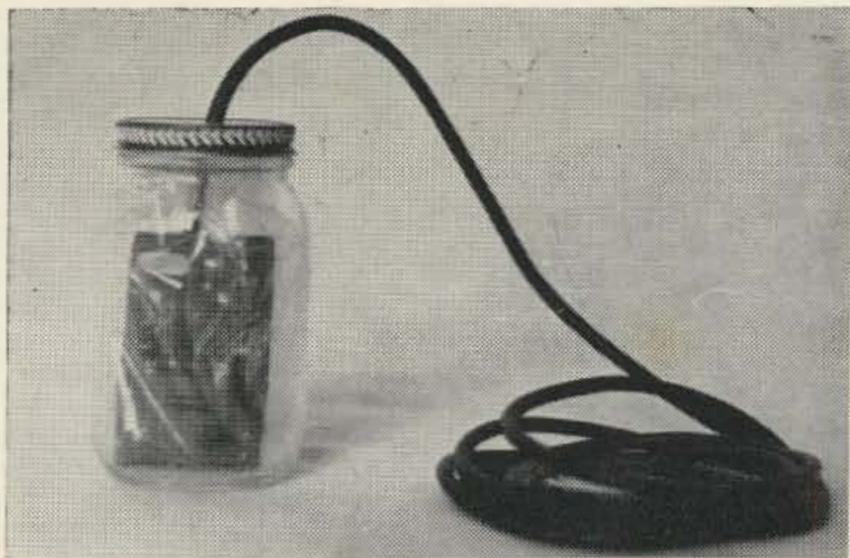
It looked like I was going to have to rely on our wall thermostat for my temperature stabilization, indeed, a sad state of affairs. Then I began thinking: look, the main purpose of a crystal oven is to maintain a *constant* temperature, not necessarily a particular temperature, but a constant one. K2TKN's idea of burying the oscillator was to utilize the near constant temperature of the earth several feet underground, not an attempt to achieve any specific one.
