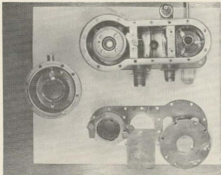
1) Modified cavity assembly: upper right, main cavity body, lower right, cover plate, center left, 2C42 cathode cavity.
