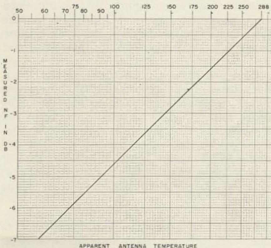
Converting measured NF to apparent antenna temperature (see text). Example: If noise figure measures to be  $-2.8$  db, apparent antenna temperature is  $150^{\circ}\text{K}$ .
