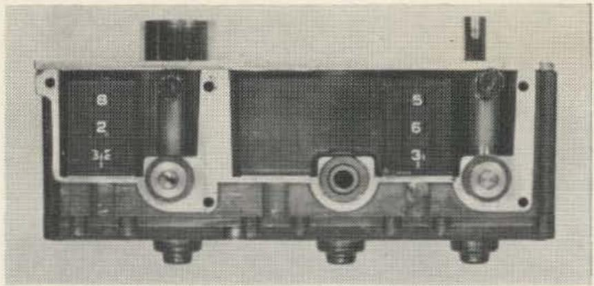
2) Gear drive tuning mechanism after modification.
