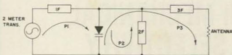
Fig. 2 Basic tripler diagram.
