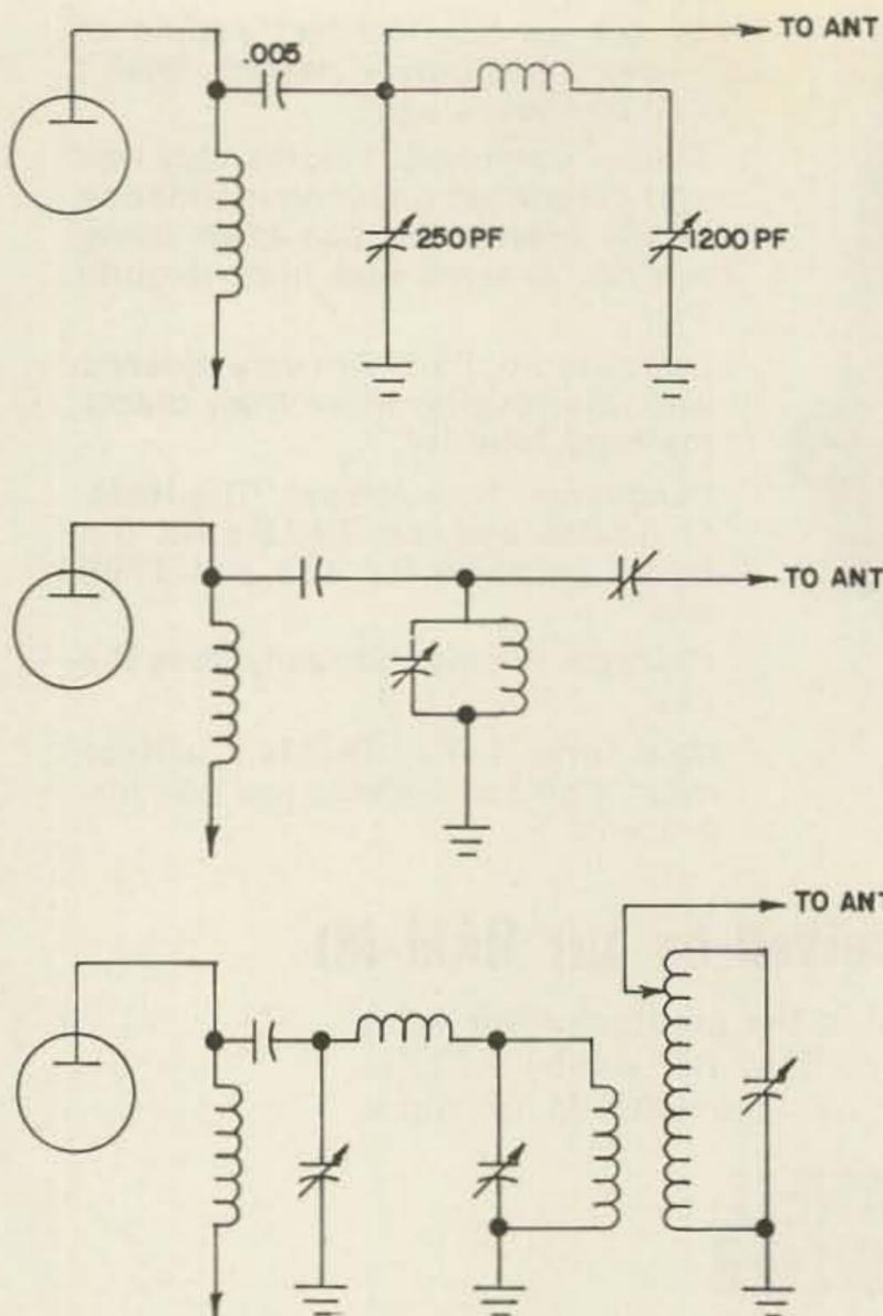
Fig. 2. Alternate output circuits.
