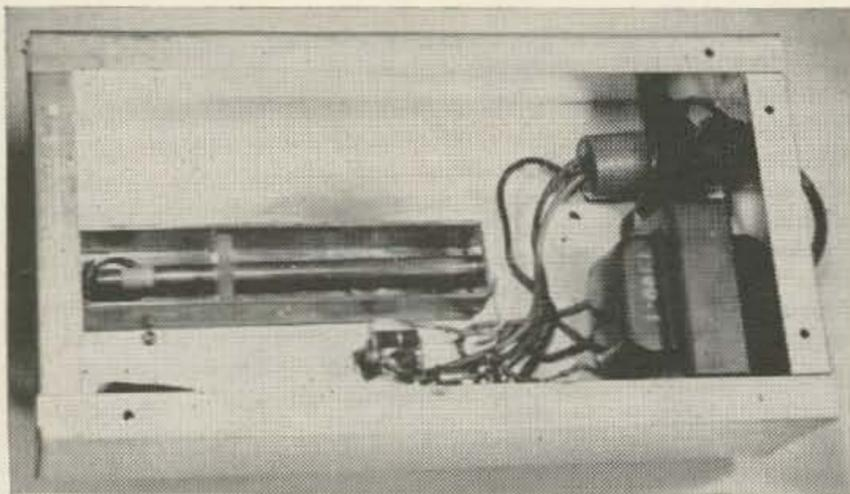
Photo 2—Bottom view of the amplifier showing the plate line and power supply.
