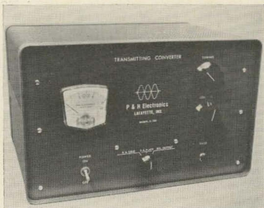
Exciters with outputs of 5 to 25 watts will drive the unit to full power. A switchable (in or out) internal Pi-section pad is used to attenuate the signal from the popular 100 watt class exciters. Also supplied is a large 3 db pad for AM operation and to correct for large differences in power levels.
