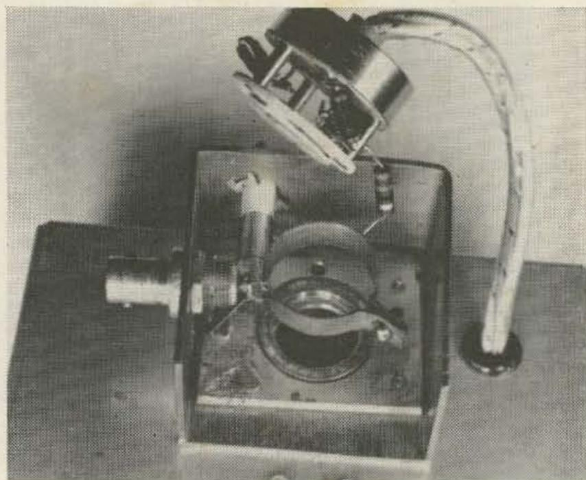
Photo 3—Close up of the cathode box, with tube removed, details of input circuit.
