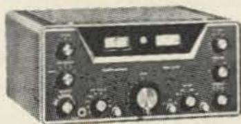
Exceptionally versatile and compact Triple-conversion, super-heterodyne communication-type receiver. Selectivity .5, 2.5, or 5. Sensitivity less than  $1 \mu\text{V}$  on AM, less than  $\frac{1}{2} \mu\text{V}$  on SSB/CW. T-Notch filter, I.F. type noise limiter, 100 kc xtal Calibrator.
