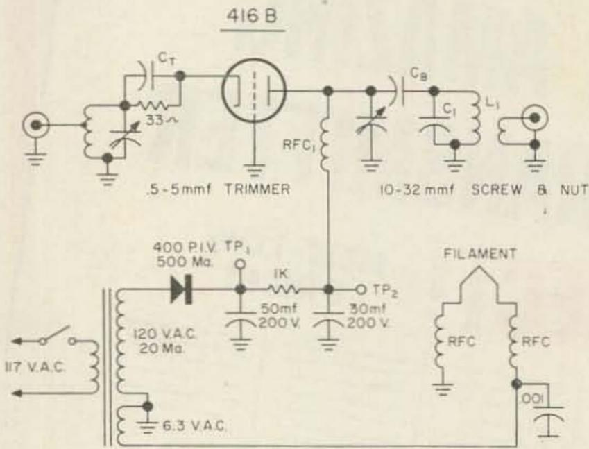
Fig. 1—Schematic diagram. C1L1 Coaxial Tank, CB Plate Blocking Capacitor (see text), CT built in Cathode Capacitor (see text), RFC1 formed by having B+ lead inside plate line, RFC2 filament rf chokes (see text).
