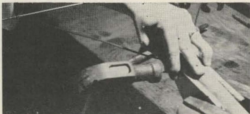
To mount the antenna, cut two triangles of thin plywood and nail them to a second broom handle. Leave space at the top for the antenna boom to fit. Then nail the antenna boom in place as pictured here and you're finished. The completed BH-4 should be mounted at least 20 feet in the air. If you can get hold of a TV rotator it's ideal to turn it, but the Armstrong method also works!
