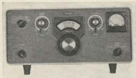
The 62S-1 converts a 14 mc AM, CW, SSB, or RTTY signal to 6 or 2 meters. N.F. 4 db and power input 160 watts. High voltage is taken from the present exciter. Size: 7¾ h, 14¾ w, 13 d. Weight: 25 lbs. Price: \$895.00.
