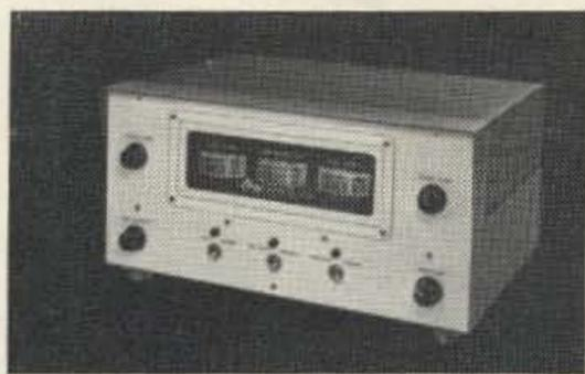
Clegg Apollo 700 six meter linear amplifier. 700 watts PEP with 10 watts of drive. Push pull 8236's. Automatic control with Venus transceiver. Three meters. Built in solid state power supply. 15 x 7 x 10 1/2.
