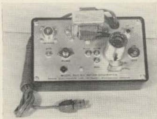
The Model 50-1 6 meter converter uses a 6CW4 and 6U8A to give output on 7-11, 10-14, 14-18, 26-30, 27-31, 28-32, or 30.5-34.5 mc. 1.5 mc bandwidth, self-contained power supply, choice of connectors. Price: \$34.50.
