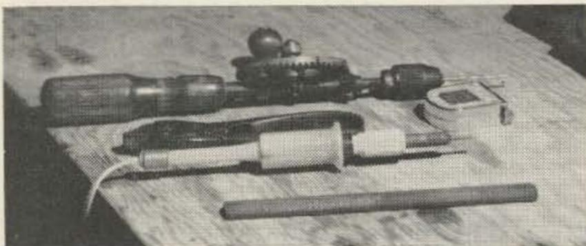
These are the tools you'll need to build your BH-4: hand drill with 3/32-inch bit, pliers, tape measure, soldering iron, and file. You'll also need a hammer and a couple of nails to mount the finished antenna in place atop a second broom handle, and some ordinary insulating tape to fasten the lead-in wire to the supporting mast. Either twinlead or coaxial cable can be used for feedline, but twinlead is recommended since it has far less loss per foot.
