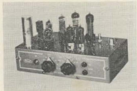
The Criterion converters are available for 50-54, 144-148 and 220-225 mc. Outputs available from 6-50 mc, built-in power supply, 2 tubes, 2 nuvistors, 4 mc flat bandpass. Price: \$54.95.
