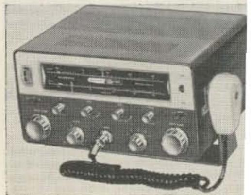
The HW-10 and HW-20 are 6 and 2 meter transceiver kits, respectively. 6 meter Shawnee covers 49.8-54 mc, 2 meter Pawnee 143.3-148.2 mc. Both feature built-in supply for 6, 12 or 120 volts. 10 watt 6360 final, push-to-talk microphone, VFO or crystals, internal speaker, 15 kc selectivity, double conversion, squelch, BFO, AVC. Size: 6 h, 12 w, 10 d. Weight: 34 lbs. Price: \$199.95.
