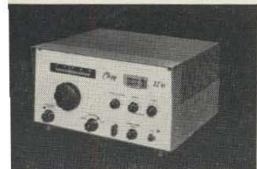
Clegg 22'er two meter transceiver. Double conversion receiver with crystal lattice filter, Nuvistor RF stage, effective noise limiter. Transmitter has broadband exciter stages, 18 watt high level modulated 2E26 final, flywheel tuning and provisions to switch external final and VFO. Built in solid state power supply for 115 vac or 12 vdc. \$239.50.
