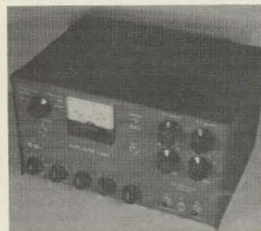
Model 621 six and two meter transmitter. 60 watts to GE 8150, 6L6's plate mod. Xtals or external VFO. Built in dummy load, separate loading controls, spotting button, metering of all stages including rf output using external meter (not supplied). \$229.50.
