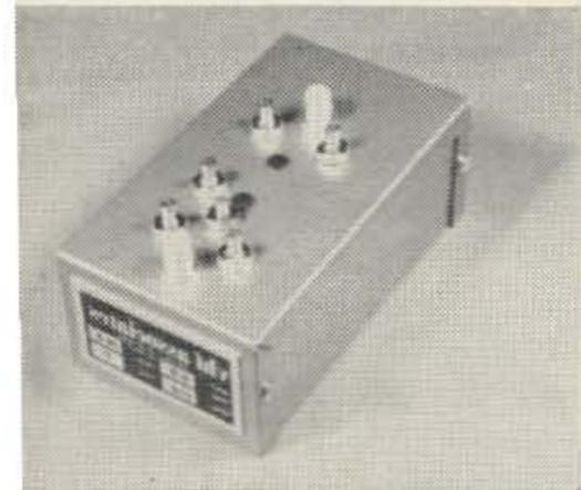
Model 514 Varactor Tripler from 48 to 148 mc. Drive requirements: up to 20 watts RF. Output: 12 watts PEP on AM, 12 watts carrier on FM or CW. No primary power required. Size 3 x 5¼ x 2¾ in. \$54.95.
