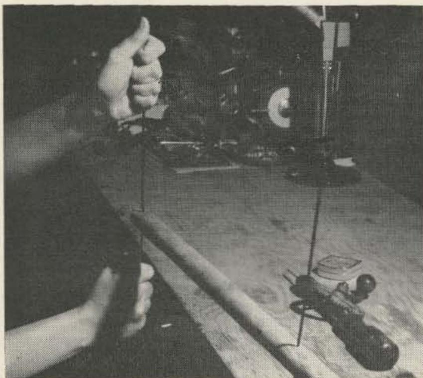
Now it's time to assemble the beam. Put the 40-inch hanger in one of the end holes. The 38-inch element goes in the next hole, the 36-inch next, and the 35 $\frac{3}{4}$  inch one goes
