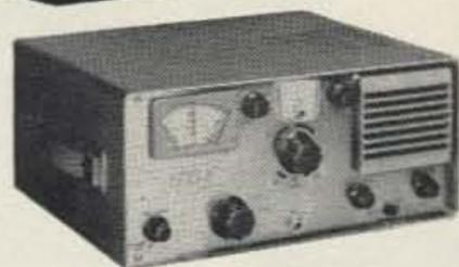
The SBE SB-33 packs plenty of SSB punch on 80, 40, 20 and 15 meters sideband with 135 watts PEP. AC power supply and speaker built-in. Upper or lower sideband selection by a front panel switch. Has a steep-slope Collins Mechanical filter.
