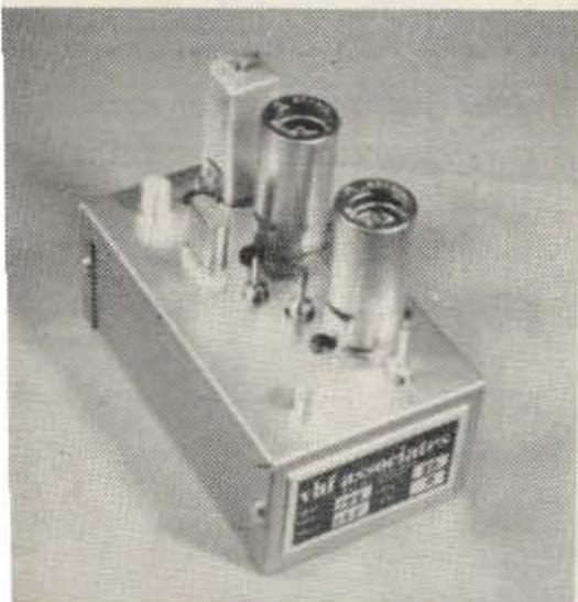
Model No. 145 2 meter converter. 50 to 54 mc. Noise figure better than 5 db. Gain more than 25 db. Requires 100 to 150 vdc and 6.3 v. 3 x 5¼ x 2¾ in. Price \$22.95.
