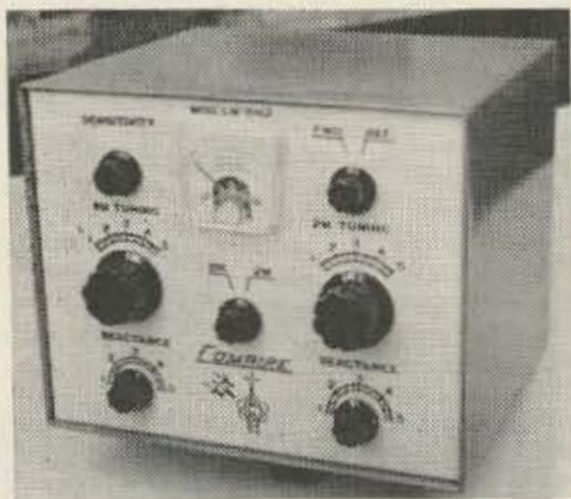
LM-6N2 Line matcher. Combination six and two meter antenna tuner with built in SWR power meter. 500 watts. 7½" x 6" x 7". 8 lbs. Tuners are completely separate. \$59.75.
