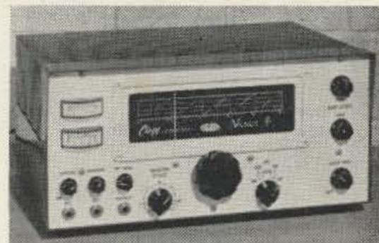
Clegg Venus VI, SSB transceiver for six meters. Receiver tunes 50-50.5 mc (or any other 500 kc band if specified), crystal lattice filter for selectivity, nuvistor front end. Transmitter 85 watts AM, SSB, CW to 6883 final. Tuning dial: 1 kc per division. Receiver may be offset from transmitter frequency by plus or minus 1 kc. Requires separate power supply. \$495. AC power supply \$110, 12 vdc supply \$120.
