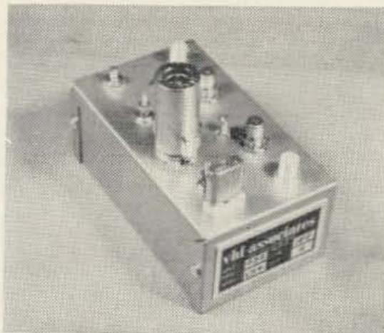
Model 4314 (2 meter output) and 4322 (1¼ meter output) nuvistor converters for the 432-436 mc band. Noise figure 6 db., gain 18 db. use 2 6CW4 and a 6J6. Power required, 100 to 150 vdc and 6.3 v. Size 3 x 5¼ x 2¾. \$44.95.
