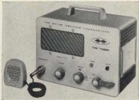
The HW-29A and HW-30, the Sixer and Twoer, are 6 and 2 meter transceiver kits. Crystal controlled transmitters, 5 watts input to a 6CL6, tunable superregenerative receiver, with microphone, less crystal and mobile power supply, built-in ac supply. Weight: 8 lbs. Price: \$44.95, GP-11 mobile power supply kit \$16.88.
