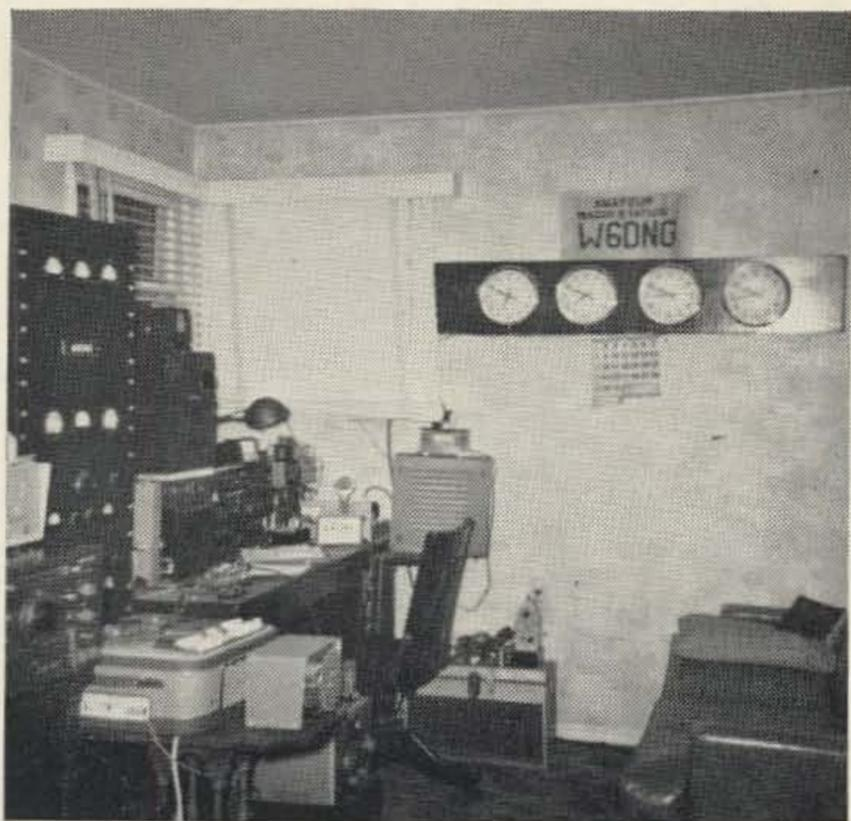
highly stabilized 8 mc oscillator which hasn't turned off for over two years. It doesn't drift. A 5894 buffer drives the PP GG 4X250B's. The receiver starts out with a 416B preamplifier into a nuvistor converter into a 75A4 using a 500 cycle filter and an 80 cycle audio filter. I've got a feedback circuit for noise cancelling built in, but that's another story.
