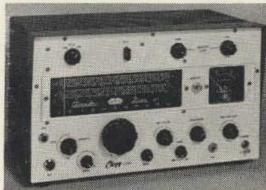
Clegg Zeus six and two meter transmitter. 185 watts AM or CW on both bands to a 7034. 811A's class B plate modulation, 18 db speech clipping with automatic modulation control. Crystal oscillator or built in ultra-stable VFO. Flywheel tuning dial. Power supply and modulator in separate unit with interconnecting cable. \$695.
