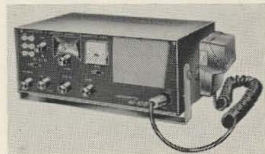
The HE-45-B a 6 meter transceiver with 14 watts input to a 2E26 final. Built-in 12 and 115 volt supplies and speaker. Pi-network, external VFO input, S-meter, spotting switch, noise limiter, superhet receiver. Size: 5 h, 12 w, 8 1/2 d. Weight: 15 lbs. Price: \$119.95.
