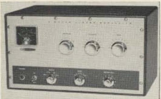
The HA-20 is a 6 meter linear amplifier kit to match the HX-30. 2.5-10 watts drive, 125 watts PEP SSB, 75 watts AM, push-pull 6146's, forced air cooling, self-contained power supply. Size: 10 1/8 h, 16 5/8 w, 10 d. Weight: 43 lbs. Price: \$99.95.
