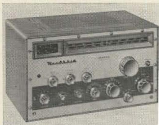
The VHF-1 Seneca is a 6 and 2 meter transmitter kit with 140 watt CW and 120 watt AM input to 2-6146's. VFO, 4 crystal socket carrier control modulation, band switching, power supplies included. Size: 10½ h, 16½ w, 10 d. Weight 50 lbs. Price: \$179.95.
