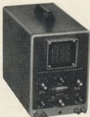
Heathkit General Purpose 3" Oscilloscope Kit
