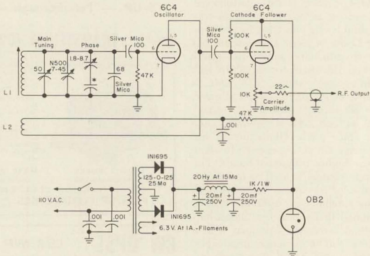
\* #20 solid plastic insulated wire, twisted together 1/2".
