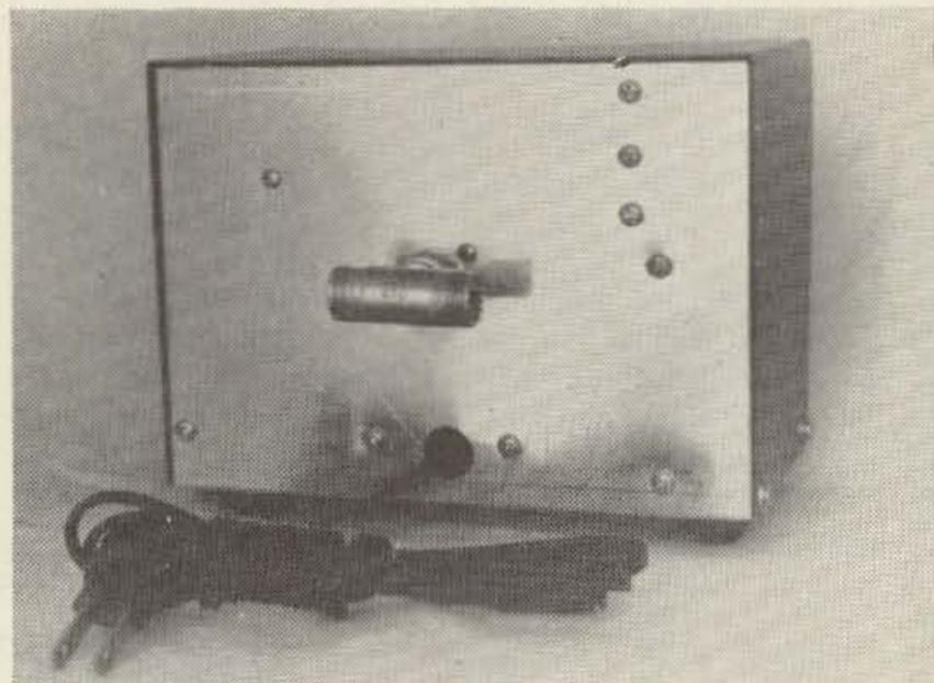
Peak up the receiver for maximum monkey chatter, and then carefully tune the tuning dial of the Deceiver for intelligibility of the signal. The S-meter will indicate when the Deceiver is tuned near the signal frequency. Once the signal is tuned, the Deceiver *phase* control may be used to trim up the voice pitch as the station frequency drifts up or down the band.
