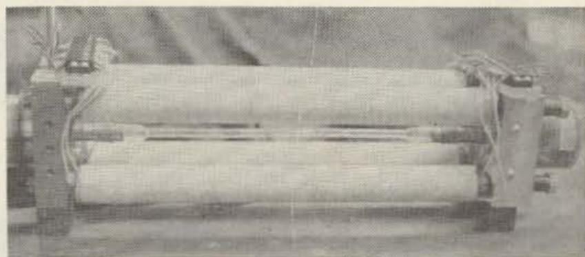
Closeup of Highly stable maser. Four coils are wound around invar rods. The coils are for magnetostriction tuning of maser.
