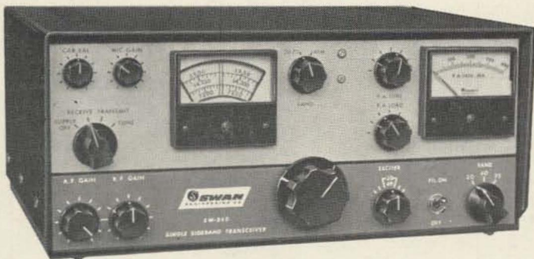
240 watts PEP input. High frequency crystal lattice filter. Precision tuning mechanism. Exceptional frequency stability. Receiver sensitivity better than one microvolt.
