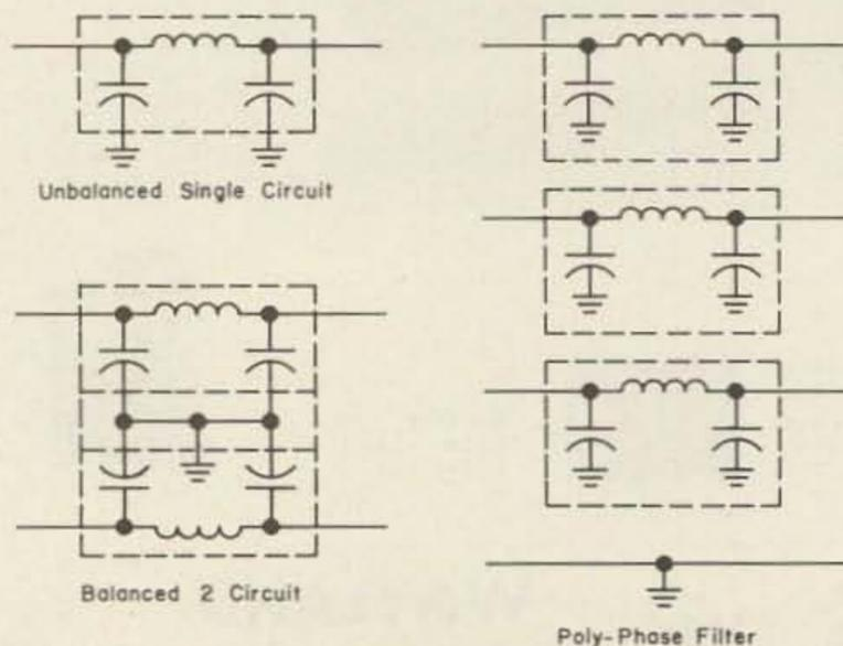
It is more often desirable to have the filter built in at the source of the noise since capacitive or inductive couplings may take place in a power or coaxial transmission line. Doing so will eliminate the need for much complex shielding and grounding to eliminate low level mutual coupling. Filter specifications common to but varying in importance in all filters are:
