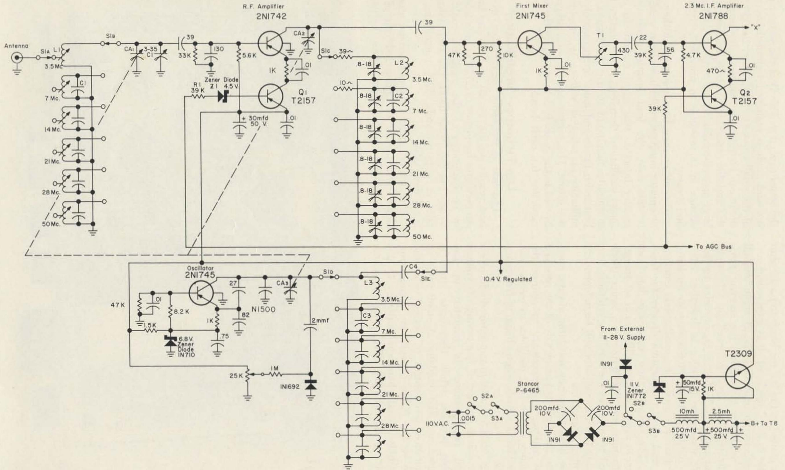
sistor is used in the 3.5 mc band and a 10 ohm resistor in the 7 mc band. It is impractical and unnecessary to neutralize the rf stage and all other amplifiers throughout the receiver since stabilization has been achieved by mismatching impedances. Transistor  $Q_1$  provides *agc* for the rf stage; its operation is described later.
