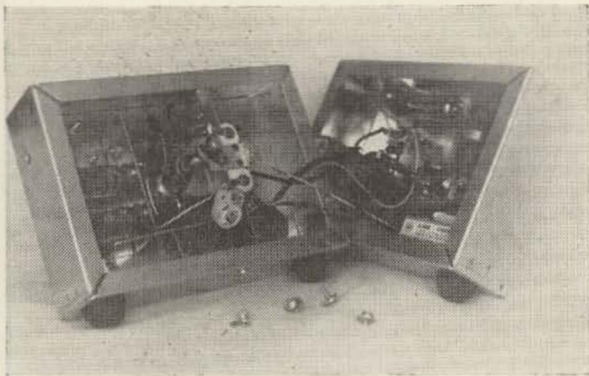
shielded. This dictates the use of a coax fed antenna. If an end fed wire antenna must be used, then it is required that a receiving type antenna tuner or a Balun be constructed to convert the signal to low impedance. The circuit shown is one which worked well at this station. The coil is a modified B&W 75 watt plug-in coil, but a 25 watt coil or piece of Miniductor could also be used.
