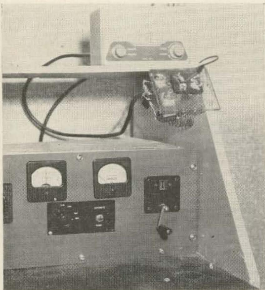
Right center—the phase shift network. Note the removable plug and the components mounted on the back of the board. The linear is a pair of 4X250 B's in grounded grid.
