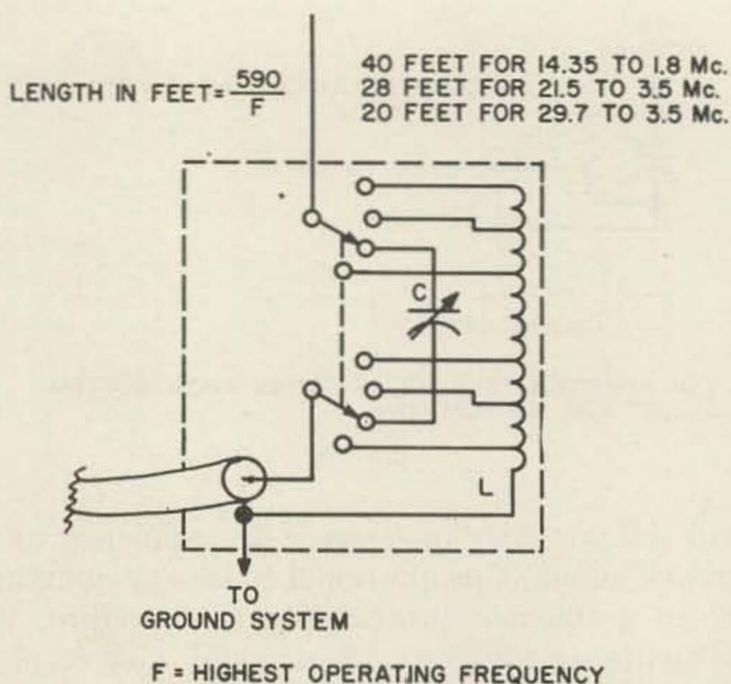
Fig. 5. Simple 3 to 5 band vertical antenna.
