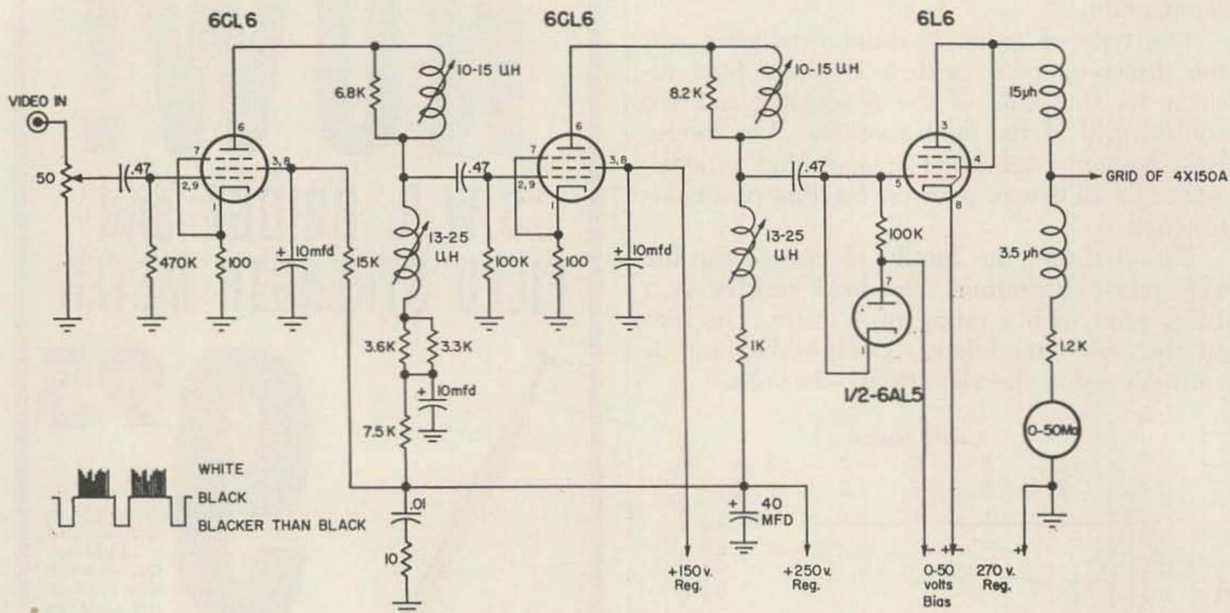
In the process of putting video on the air, it will be necessary to monitor the video in the transmission line. Fig. 5 illustrates a typical detector for the composite video information. The type UG tee connector was modified by removing the dielectric insert and installing a small loop. This which is placed in a plane parallel to the conductor. A 6AL5 is used to demodulate the video from the rf.
