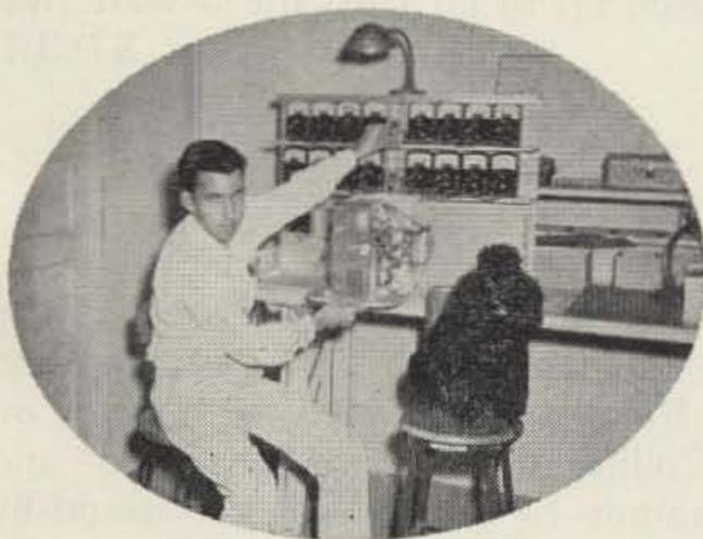
*GONSETT'S OCTOPUS, shown here with Bob Gonsett, WA6QQQ and mascot K9-CINDY, simultaneously makes seventeen resistance measurements to check over 170 individual components prior to power checks. This has eliminated the familiar "60 cycle smoke signal test" and assures that there are no marginal components in the unit.*
