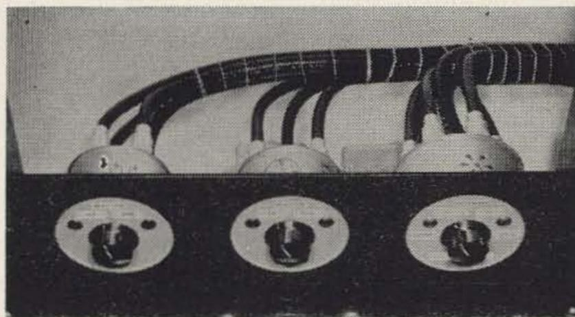
Three types: one pole-six throw for antenna switching, \$12.95; one pole-two throw in case you don't have so many antennas or want to use a dummy load, \$11.45; transfer switch for switching power amplifier in and out, \$11.45. All are canned for protection. All have SO-239 type connectors.
