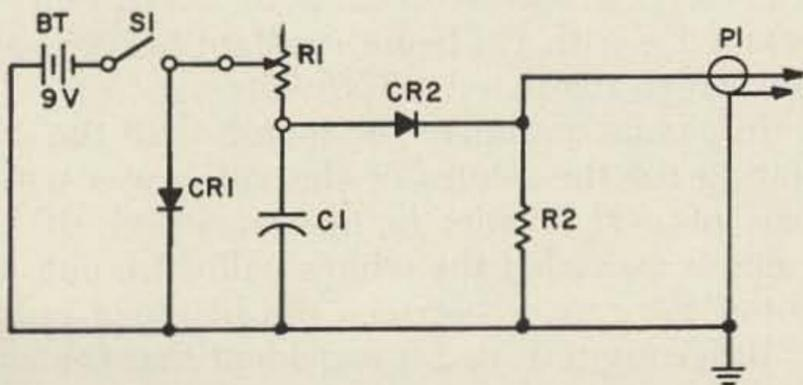
To avoid excess wear and tear on the zener diode and the battery a 200 ohm resistor should be inserted between the 9 v battery and S1.
