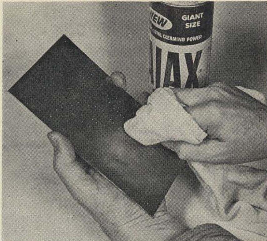
5—Carefully peel the master from the copper and save it. Remove all rubber cement from copper, then scour thoroughly. Avoid touching copper surface from now on.
