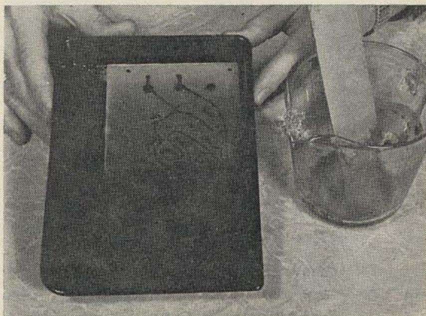
9—A shallow glass or plastic tray should be used to avoid contamination of the etchant.
