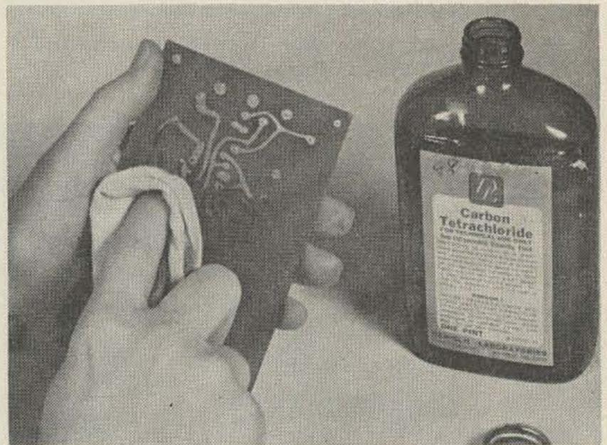
12—Resist may be removed with carbon-tetrachloride. Cleaning should continue until rag shows no trace of resist; otherwise difficulty may be encountered in soldering.
