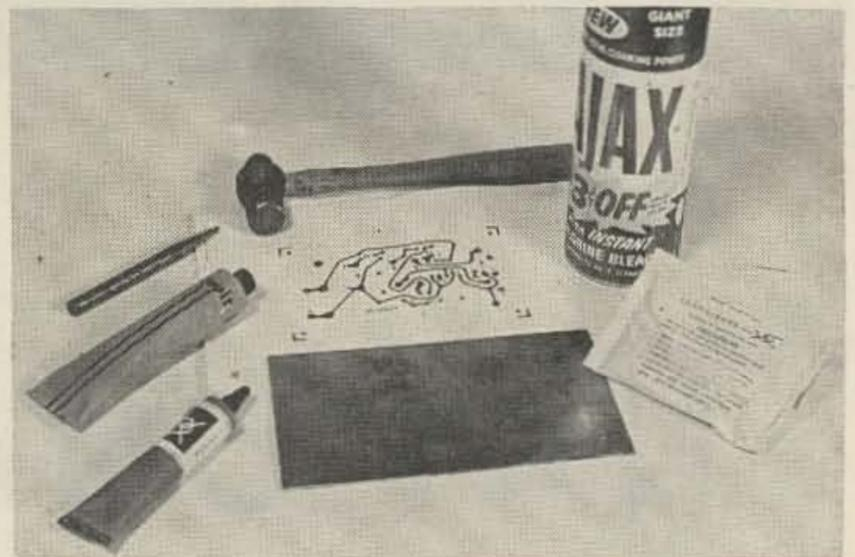
2—Basic materials required. The tubes contain rubber cement and liquid resist, the packet contains etchant.
