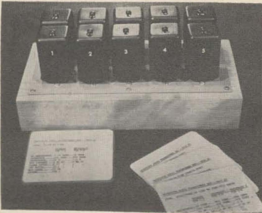
This test transformer set is an example of the use that can be made of surplus relay cans.
