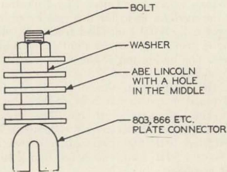
Heat dissipating connector for 715-B.
