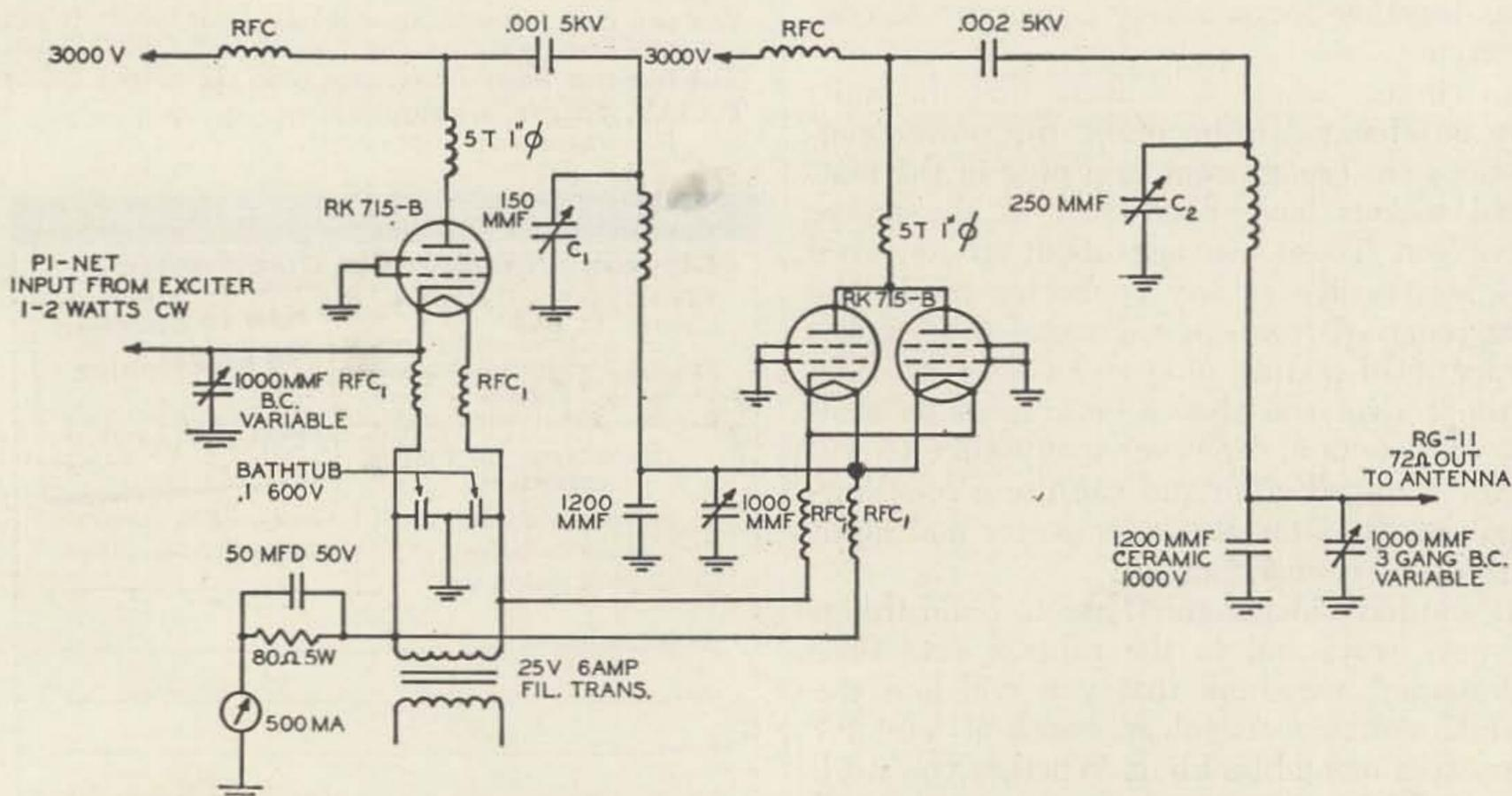
Coil—conventional, from handbook. Pi-net condenser values shown for 80 meters, divide by 2 for 40 meters, by 4 for 20 meters. RFC-1—6v line filter choke from old car radio.
