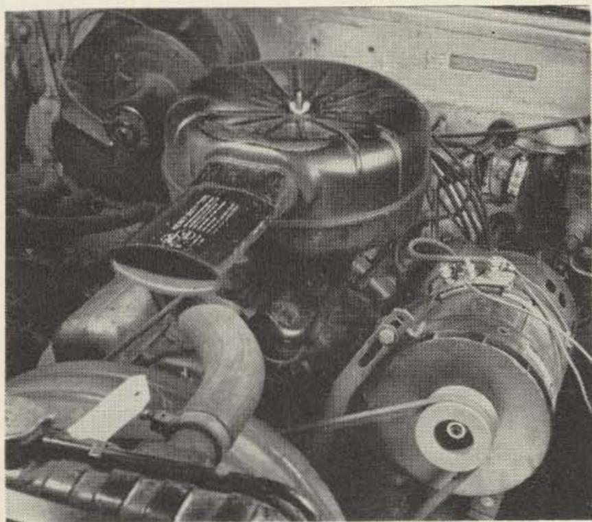
Typical installation of Leece-Neville 60-ampere heavy-duty alternator equipped with silicon rectifier diodes.
