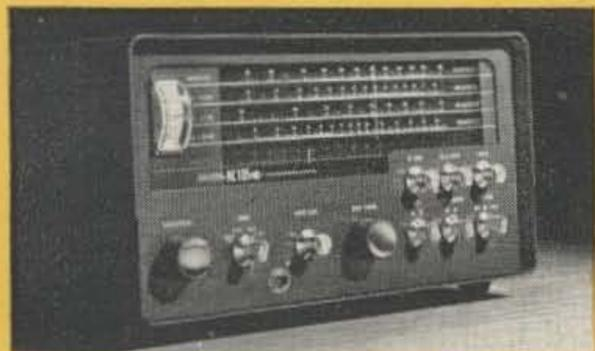
**NC-105** — Designed specifically for the beginning amateur. Offers such needed features as general coverage Q-Multiplier, product detector, S-meter and transformer power supply. Also available in handsome walnut cabinet for use in den or living room as a second receiver. \$119.95
