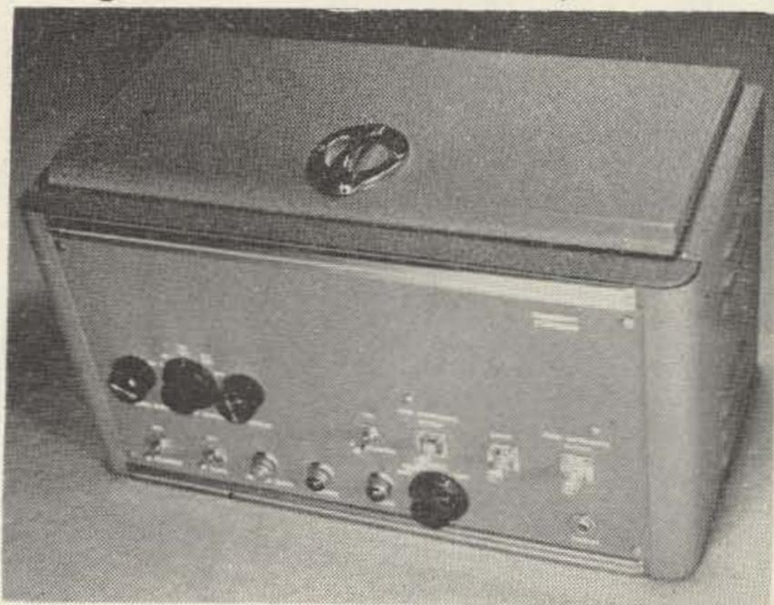
The frequency standard is housed in a stock Par-Metal cabinet.
