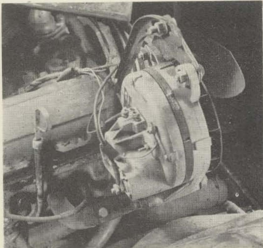
Typical installation of Leece-Neville 40-ampere, 6000 Series alternator with built-in silicon rectifier diodes.
