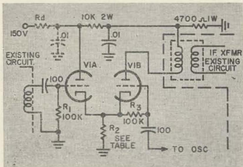
The 73 mixer circuit using a 12AT7 plus half of another 12AT7 as a Pierce oscillator. A 7 mc doublet and the coil-condenser combination in the upper left corner replace the normal IF transformer input. The four crystals permit tuning forty meters on any of the RAX-1 band positions, and certain commercial stations (crystal on the high side by tuning backwards—which is good enough for them).
