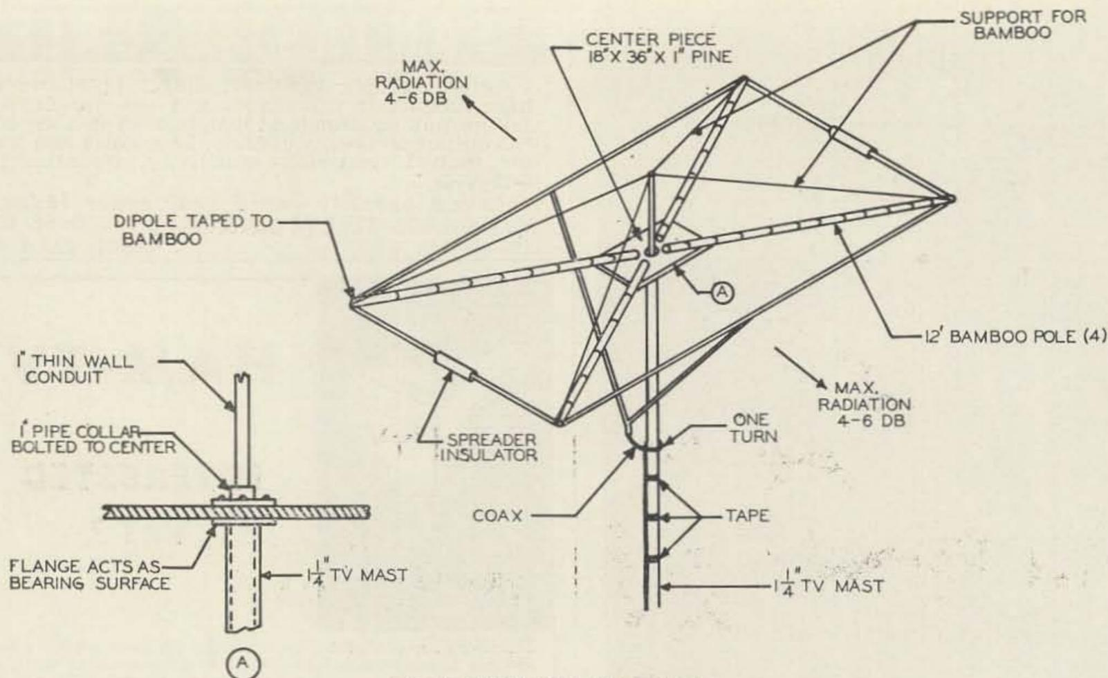
FIG. 2-ROTARY 8JK 14 MC BEAM
