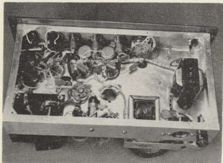
Under-chassis view shows further construction details. The detector-audio amplifier circuit shown on the left side of the chassis is not described in this article.
