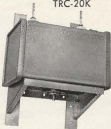
TMC's Model TRC-20K and TRC-5K are recent additions to a family of broadband RF transformers that provide coupling of RF energy from 250 watts average to 40 kw peak power with insertion loss of less than 1 db, and VSWR not exceeding 2:1.
