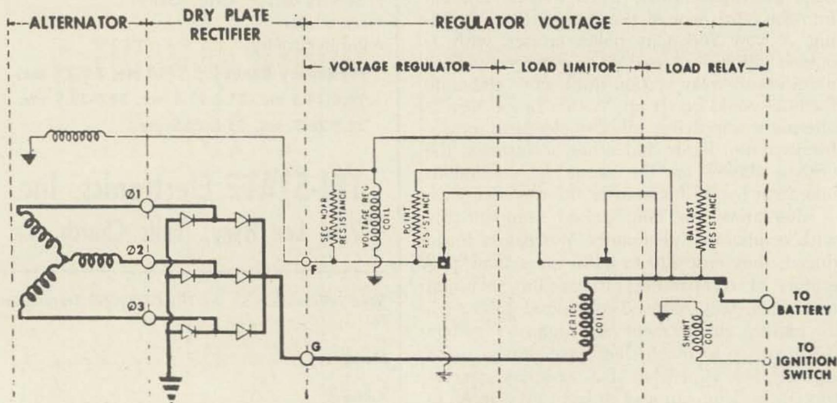
Complete wiring diagram of the negative ground system. The positive ground system is identical except that the diode connections going to terminal G and those going to ground are reversed.
