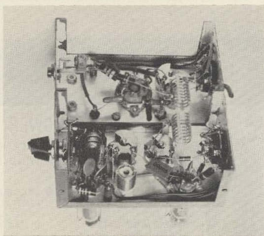
Fig. 7. In many of the modules the power is brought in at the rear of the chassis. An octal socket is used for power and interchassis connections.
