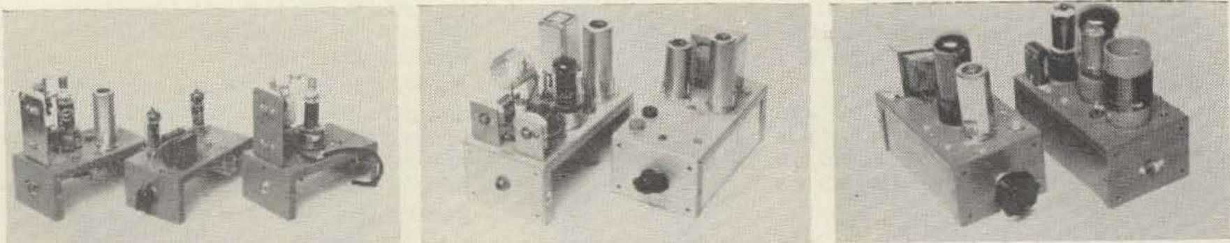
Fig. 1. Three modules can make either a 6 or 2 meter transmitter. The center chassis is an oscillator and multiplier. Two meter final is on the left and the six meter final on the right. Fig. 8 shows an underside view.
