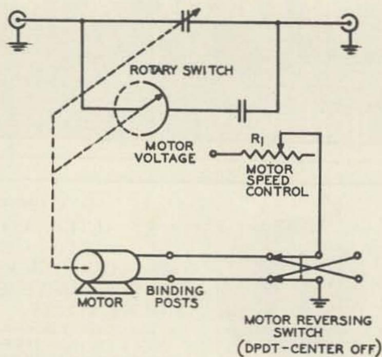
and the motor and switch coupled to it by flexible insulated couplings. A circuit diagram is given in Fig. 4 where the dashed lines indicate mechanical coupling. A speed control potentiometer,  $R_1$ , and a motor reversing switch are shown at the remote control site.
