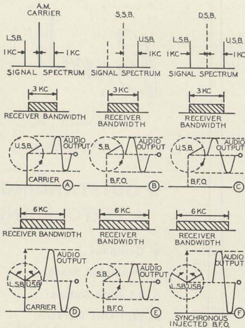
75%. At this efficiency, out of the total of 1800 watts average input power in the optimized AM case, the total average power output will be 1350 watts. Of this, 750 watts will be in the carrier. The average sideband power output will be 600 watts split into two sidebands of 300 watts each.
