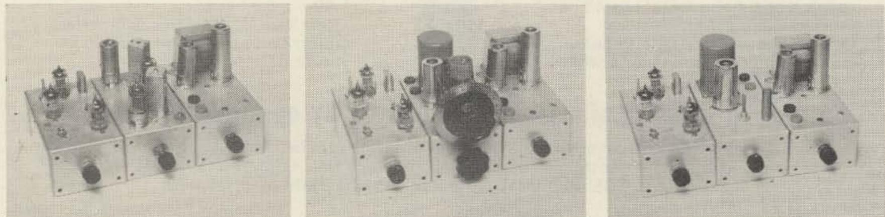
Fig. 4. Three modules will form a crystal controlled receiver. The audio module is the modulator used in the 10 meter rig shown in Fig. 2.
