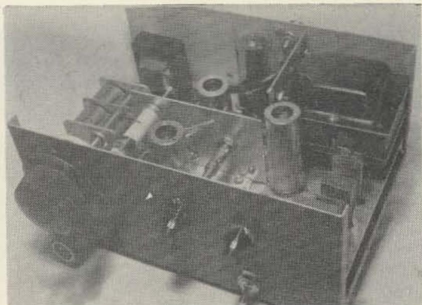
W7ATK's heavy duty model. Rear left rf stage; front left mixer with tapped slug-tuned coil covering 80, 40 and 20; front right 12AT7 oscillator—if cathode follower. Photographed under conditions of constant bragging.
