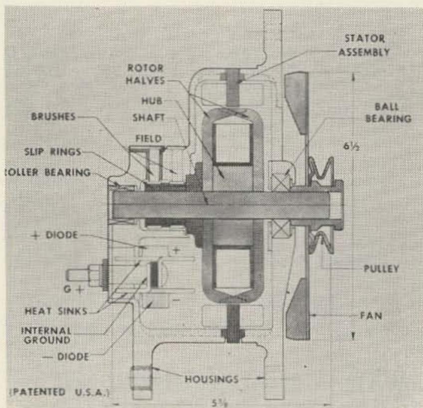
Cross-sectional drawing of Leece-Neville 6000 Series, 40-ampere alternator, used in most passenger cars.
