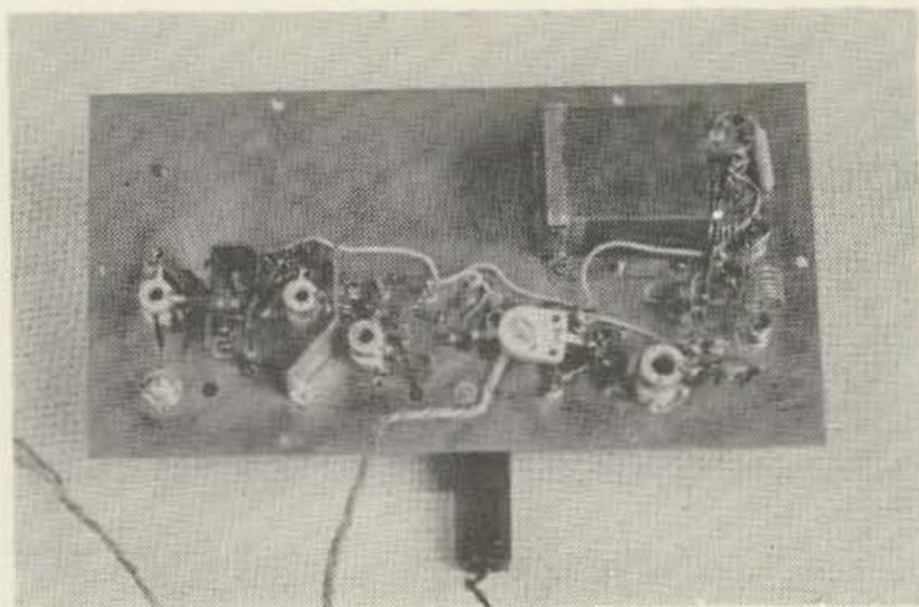
Bottom View—Note the copper enclosure for L<sub>5</sub> in upper right hand corner.
