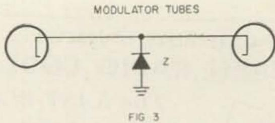
Zener diode (of the right value to provide proper bias) in the common cathode circuit as shown in Fig. 3. Where a conventional cathode resistor will give you a bias which varies with current drain through the tube, the Zener's voltage drop is constant so long as you don't fall below its minimum current or go above its upper current limit; most class B modulators fill both these requirements.
