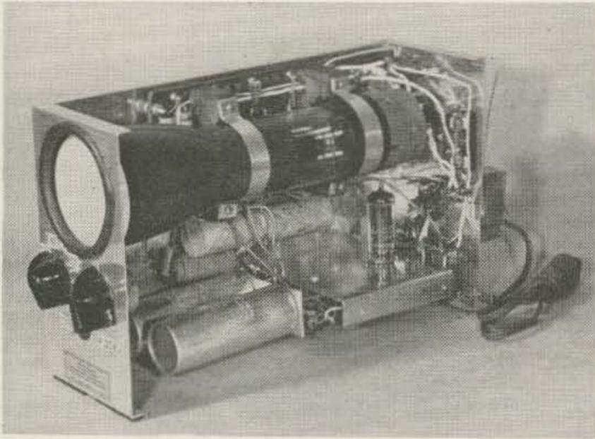
Interior view, showing method of mounting the 3BP1. 'Saddles' are wood, straps of thin (.015") aluminum. Insulation board holds saddles, quadrupler supply, and "Focus" and "Brilliance" controls, is mounted  $\frac{3}{8}$ " away from metal case.
