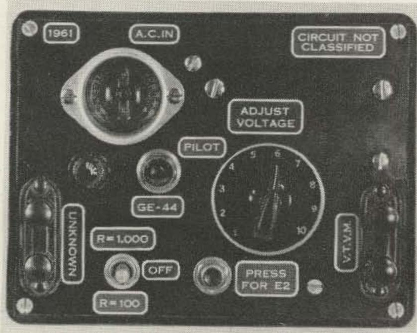
Fig. 4 Panel layout of choke evaluator.
