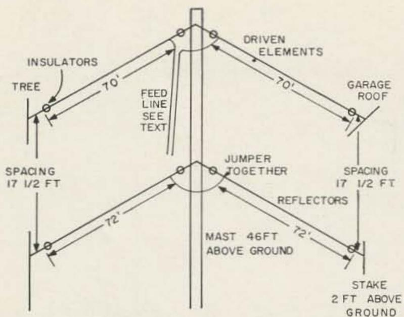
mon 1 inch spaced open wire line that is used in some TV installations also make suitable feeders for the Inverted Vee. The coupler used at W8DLU is on the order of one described in March 1959 QST (McCOY). If open wire or twin lead is used it is desirable to cut feeders  $\frac{1}{4}$  or  $\frac{1}{2}$  wavelength long. However if slightly shorter or longer line is necessary the antenna coupler will tune out enough reactance for desirable operation. Coax feedline may be of any length.
