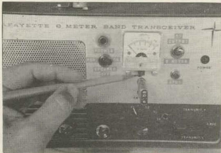
G-16—The front panel of the "Deluxe" HE-35A. The small switch under the meter turns on two small bulbs included in the meter case. Note the added "pointer" on the receiver tuning dial.
