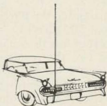
Mast and resonator in mobilizing position
