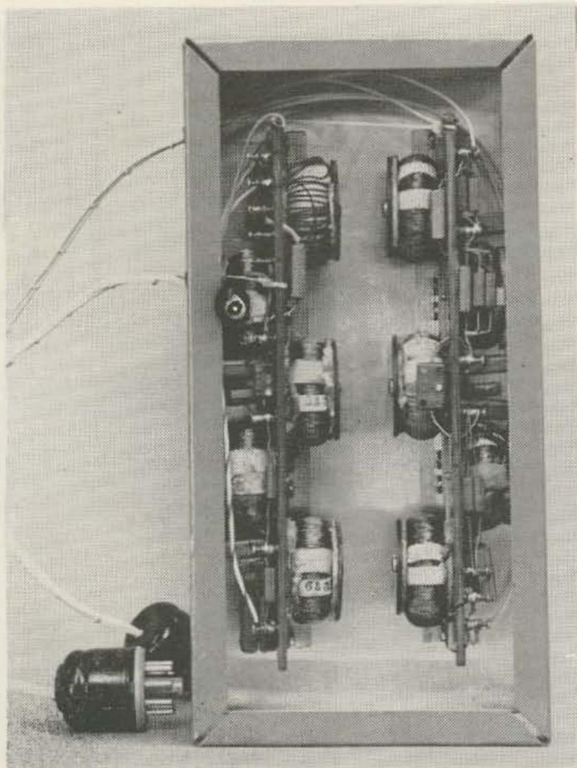
A five section maximally linear phase filter. This does not use 88 mhy toroids but the techniques are identical and the L/C ratios are appropriately scaled.
