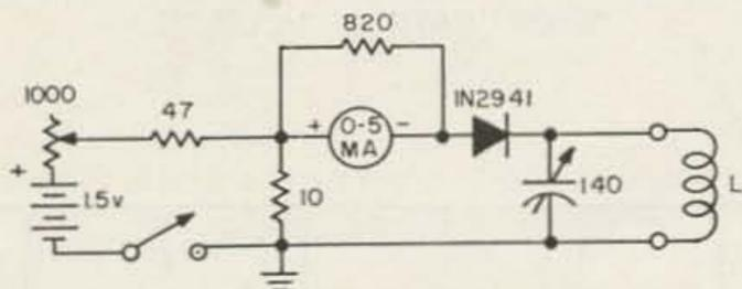
L PLUG-IN COIL TO RESONATE WITH TUNING CAPACITOR AT DESIRED FREQUENCY
