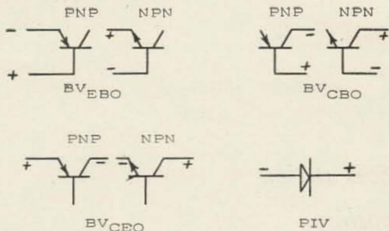
Since a semiconductor rectifying junction acts in a manner similar to an electrolytic capacitor in a test such as this, it was only a matter of making a few experiments to determine if the RC Bridge could be used for checking transistors and rectifiers. Fig. 1 gives the hook-ups needed to measure the various breakdown voltages such as  $BV_{EBO}$ ,  $BV_{CBO}$ ,  $BV_{CEO}$ , and the peak inverse voltage of rectifiers.
