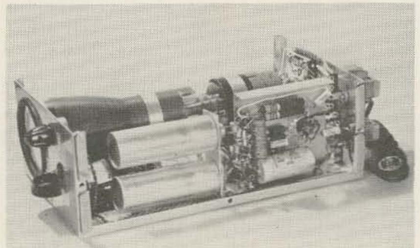
Underneath view, showing amplifier layout. Tie point strip (center) holds voltage-doubler supply connections and parts. Each electrolytic can contains two 20mfd 450 volt electrolytics, with separate positive and negative leads. Upper can is used for the doubler circuit.
