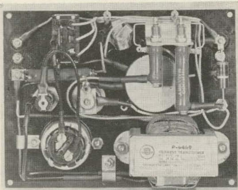
Fig. 5 Interior of choke evaluator.
