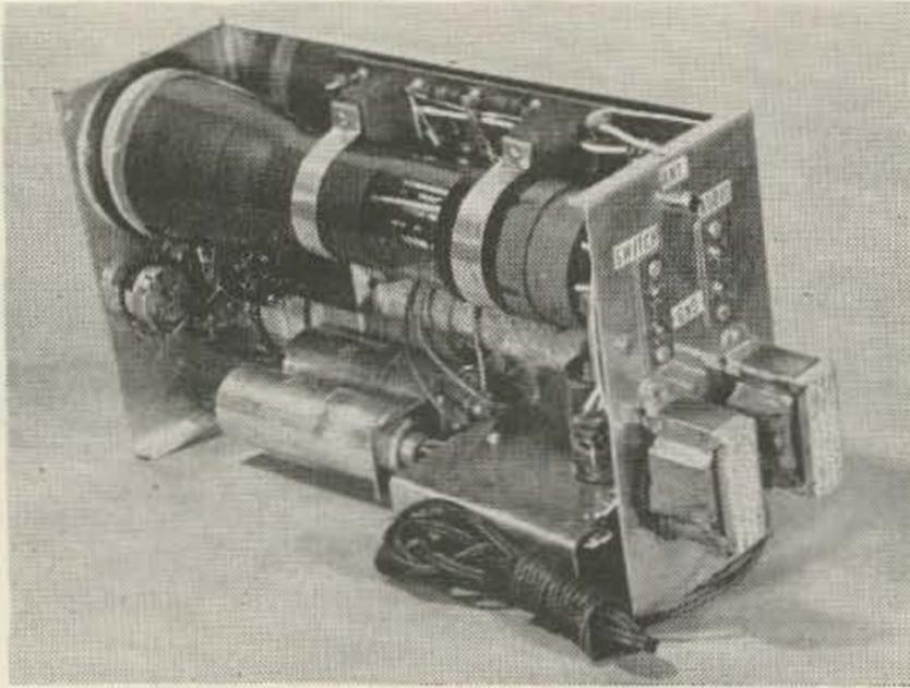
Rear terminals and transformer mounting. The "RCVR" phono jack is at center, bottom, hidden by the transformer, for short lead to the amplifier.
