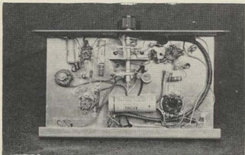
If you don't own a signal generator, try a BC set tuned to 1445 kc (good about half a mile). Peaking should be sharp but not jumpy. Turn off the signal, and maybe you can do it on noise (I did). Next make the oscillator go. Remember if things are tuned below 26.5 it may decide that 8.8 mc is where to oscillate—be sure it is working properly.
