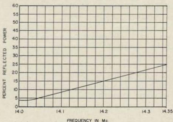
Fig. 4—A 20-meter dipole exhibiting good broad-band characteristics, but too long for optimum performance across the whole band. It should be trimmed to raise the resonant point up into the band for better efficiency across a larger portion of the band.
