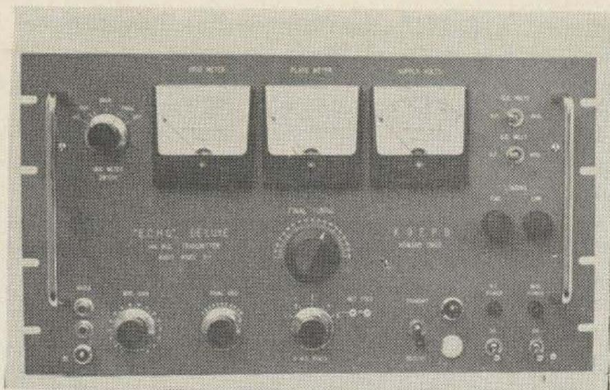
The engraved front panel showing handles for protection of meters and dials. The final tuning knob is driven by a 2 to 1 gear ratio.
