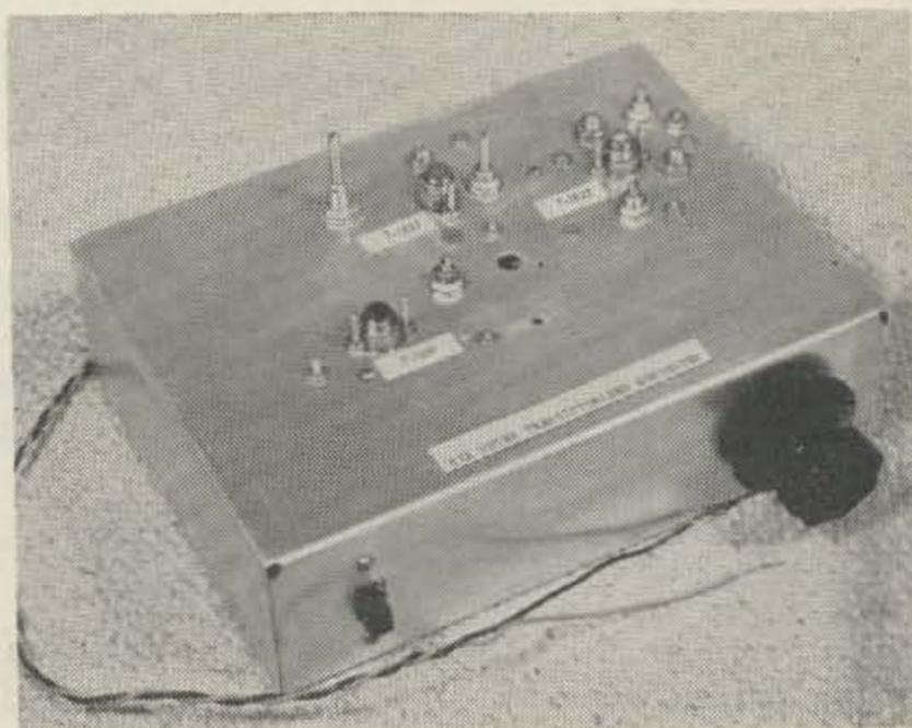
**T**HE article describes a six meter converter using three Philco MADT VHF transistors. It operates at a supply voltage of 12 volts and works into a communications receiver capable of tuning the 7 to 11 mc frequency range.
