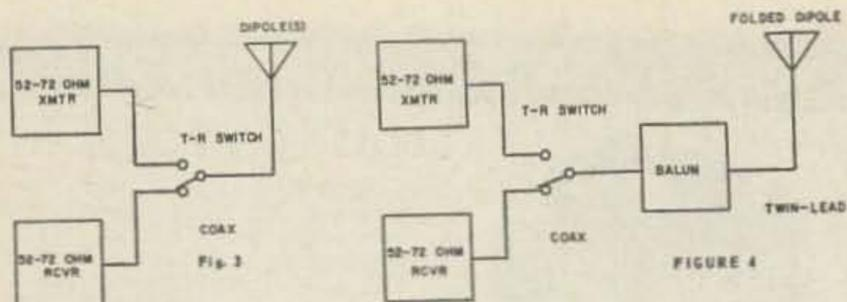
ohms and 72 ohms. The closer the impedance of the feedline matches the impedance of the antenna, the more power will be transferred between the antenna and the feedline, and the lower will be the standing wave ratio. Therefore, if the impedance of an antenna (as determined from Fig. 2) will be higher than 62 ohms, it should be fed with 72-ohm twin-lead or coax. If the impedance will be lower than 62 ohms, the antenna should be fed with 52 ohm coax.
