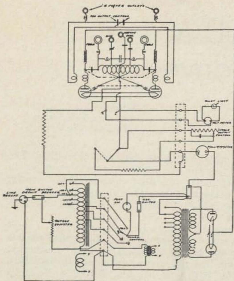
Fig. 1: Schematic diagram of a typical diathermy unit. This equipment was manufactured by Burdick Corporation and provided output on 3.75, 13 and 50 MC.
