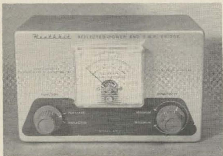
Fig. 1—The Heathkit Reflected Power and SWR Bridge is typical of several such instruments currently on the market.
