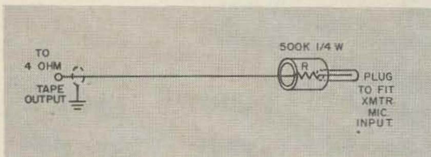
Tape output may be up to 16 ohms Z. If 500 raise value of R to prevent input stage overload. Try 3 megohms to start, and adjust as required.
