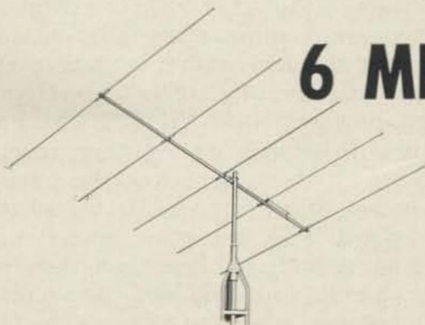
**8 Elements.** The Hy-Gain Model 68B develops the tremendous forward gain of 12.1 db with 25 db F/B ratio. Weighing only 9 lbs., this 6M beam may be rotated by any TV rotator. Boom 18 ft., longest element 9 ft. 8 in. Beta match and factory pretuned, **\$32.95**
