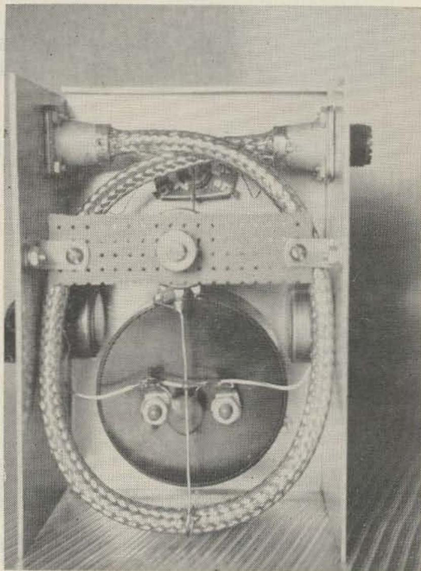
great degree. The ends of the shield braid are trimmed back far enough to be soldered to Amphenol 83-1H hoods. The inner insulation is trimmed off so as to expose about 3/16" of the inner conductor. The inner conductors are then soldered to Amphenol 83-1R female type chassis mount coax connectors. The coupler may now be set aside and the rest of the meter constructed.
