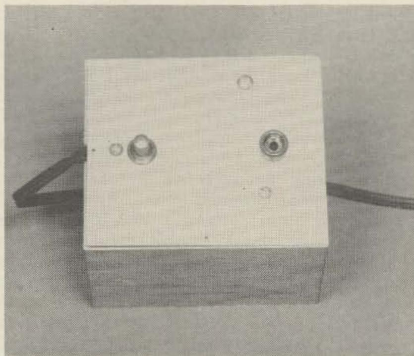
reduction. The main idea is that with a scope to show just what is happening, and the Pop Box to cause it to happen, a noise limiter circuit can be adjusted for best performance in your receiver. . . . K8ERV
