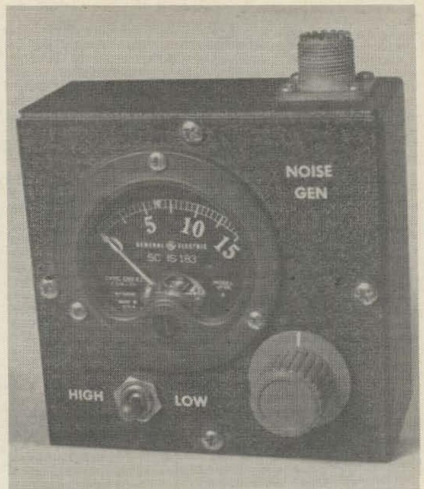
majority of amateurs something less expensive and more readily available is needed. A crystal noise generator, which can be constructed for a few dollars and which will enable anyone to make before and after comparisons of noise figure, is such a device.
