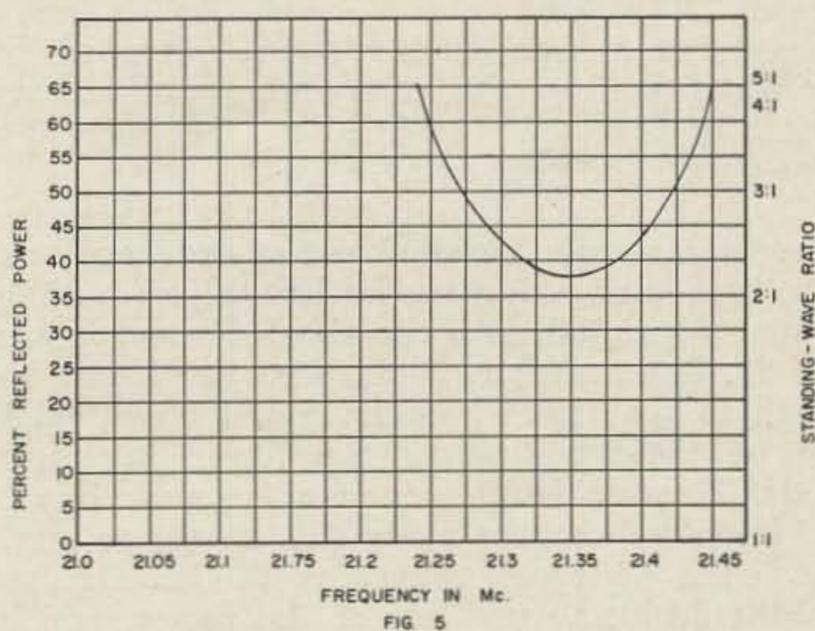
Fig. 5—Third harmonic performance of an inductively loaded 40-meter dipole on 15-meters. Optimum efficiency is not very good since the SWR does not drop below 2:1 at the resonant frequency. This antenna could be used with fair effectiveness only in the 'phone sub-band.
