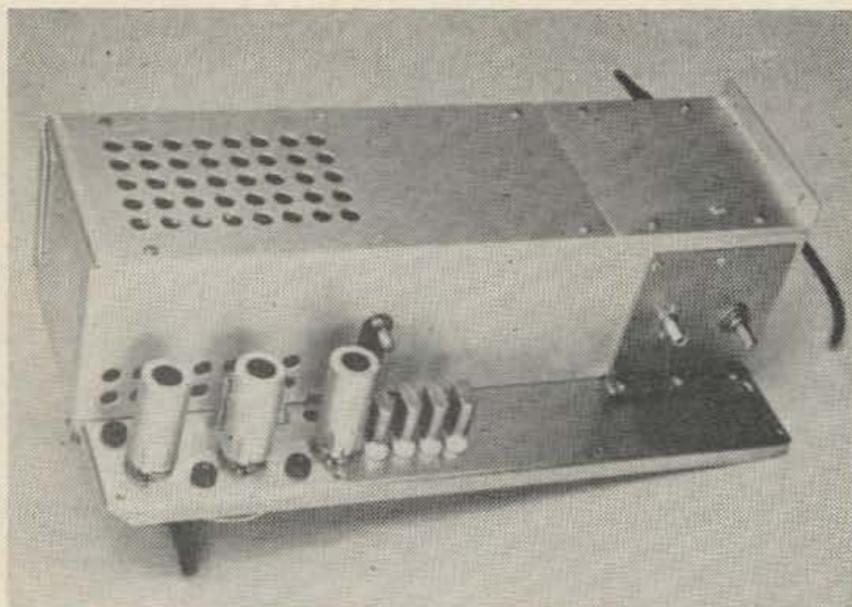
Photo showing the complete rf module.
