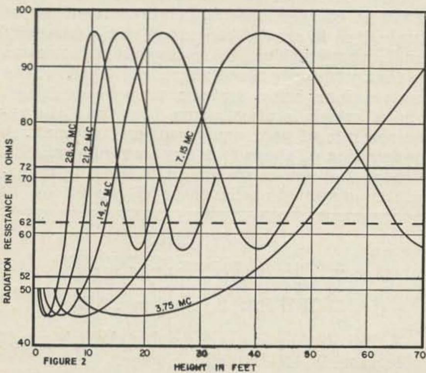
Actual measurements\* over "real" ground, however, have shown that the antenna impedance falls no lower than about 45 ohms at 0.06 wavelength (16 feet at 3.75 mc), and in fact begins to rise quite rapidly as antenna height decreases further. Fig. 2 shows the antenna impedances to be expected on the h-f bands for heights up to 70 feet or 0.7 wavelength, whichever is lower for a particular band.
