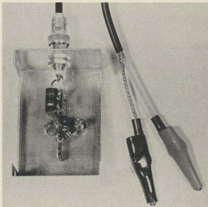
and the hot lead of the adapter probe. For instance, 200 ohms may be matched to the meter by inserting a 150 ohm series resistor. Power as shown with this adapter would then, of course, be one fourth that which was actually available. The voltage indicated would also be one fourth, minus the .1 volt diode drop, of the actual voltage available. This technique has proven handy when developing oscillator, doubler and driver stages.
