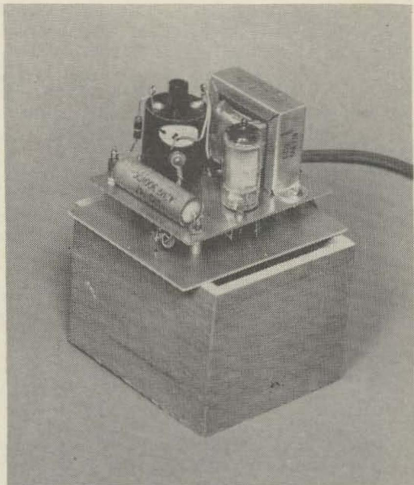
of insulated wire wrapped around the HV terminal on the coil couples the spark pulse to the antenna jack. The spark gap is not critical so long as a stable spark is obtained. My gap was about  $\frac{1}{8}$ ".
