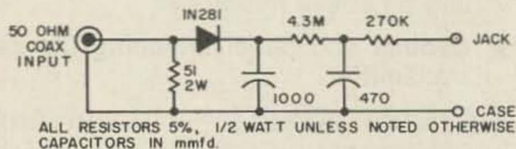
type 1N281. The following filter is capacitor input and in operation charges up to one half the peak rf voltage applied across the load resistor. The 4.3 megohm and 270K resistors, combined with the 11 megohm impedance of a typical VTVM, form a voltage divider, so arranged that the VTVM will read a dc voltage equal to .707 times the voltage the .001 capacitor has across it. Net result—the VTVM reads rms rf voltage. One tenth of a volt should be
