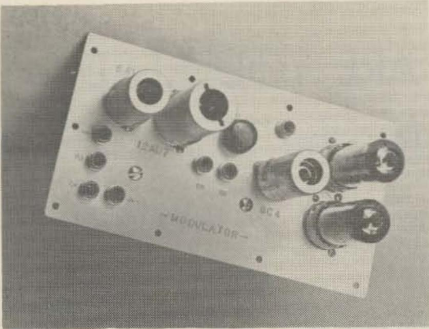
Photo showing the complete audio section jack 1 to 6 are for jumpers to by-pass the clipper if desired.
