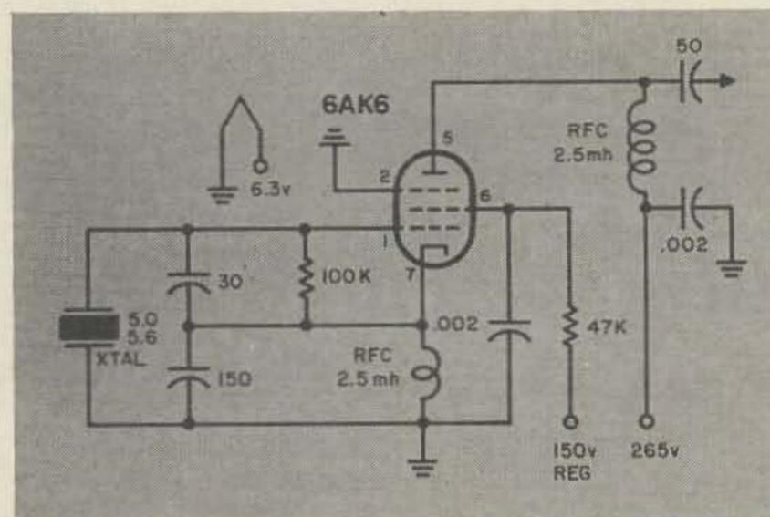
output to spare. The circuit works with any crystal. There are no tuning adjustments, and the electron coupling in the tube provides good isolation. Even the high impedance output with the coax cable capacity shunting the output still permits adequate drive to the mixer. Even with these losses, the output may still be more than is required. This is easily corrected by increasing the value of the 47K screen resistor. Also note that this oscillator runs continuously as did the VFO.
