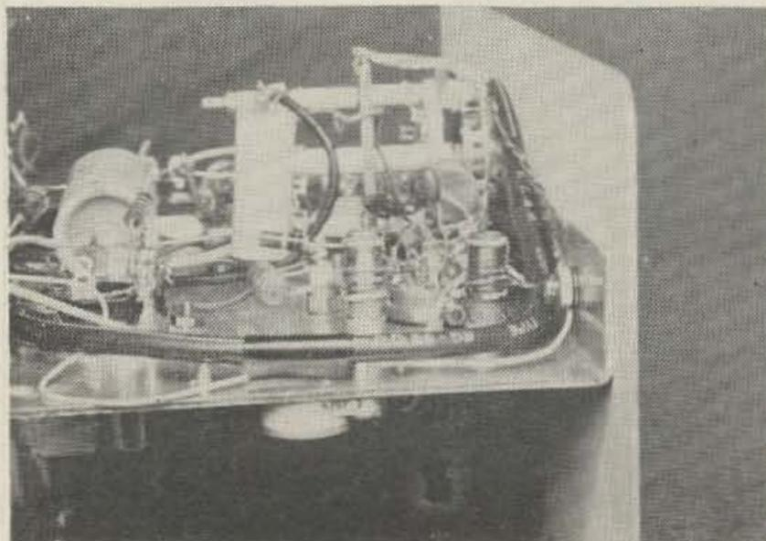
inch brass did this; the switch was stretched, for convenience, by putting it on a separate index assembly (PA-302). The other shielding problem was that I forgot to ground the metal plate between the stators of the tuning condenser. The 6BJ6 oscillated until I remembered.
