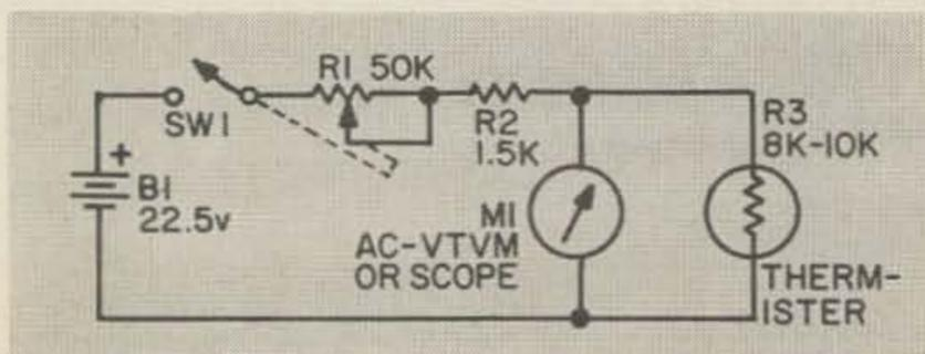
Fig. 1. Schematic of gravity detector.
