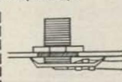
Mounts flat; only uses 3/8" inside roof.
