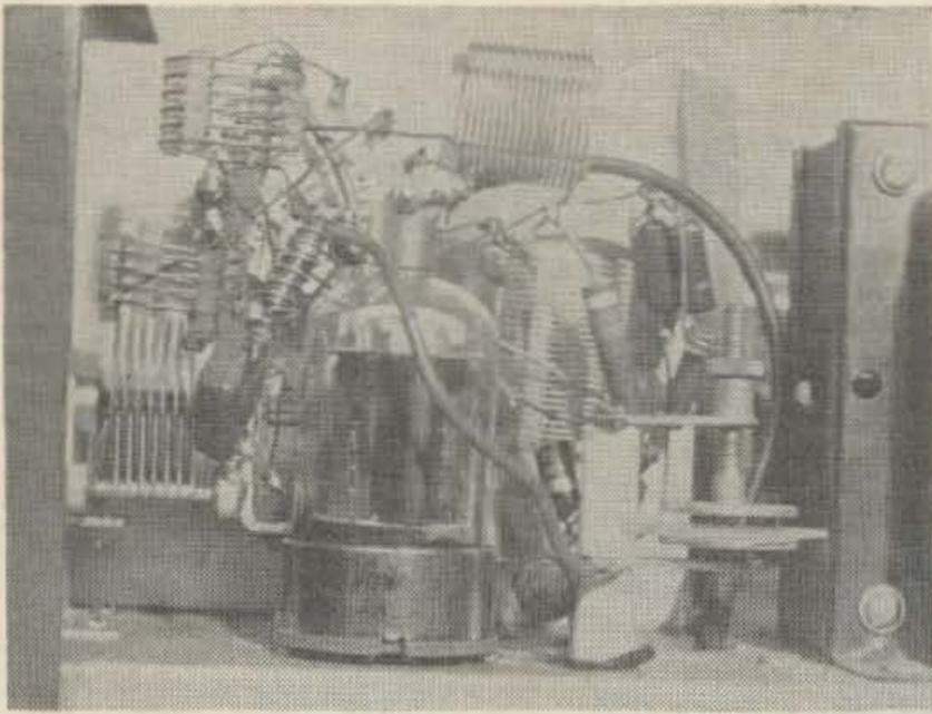
End view showing how amplifier coils grouped around amplifier tube and bandswitch. 20-meter coil hidden behind the tube. See text for more details. (That's why it was written.)
