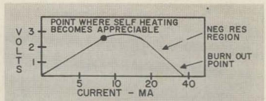
Fig. 2. Characteristic curve for a bead thermistor. Values may vary widely.
