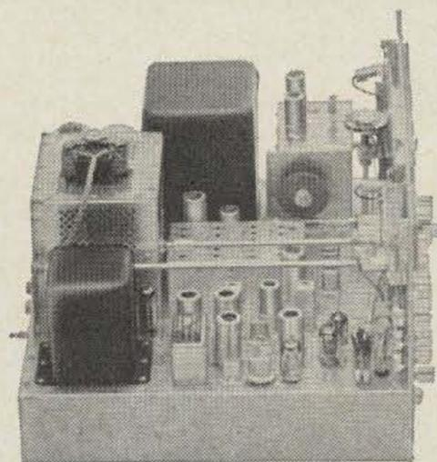
**TOP VIEW**—Quality components used throughout assure years of dependable, trouble-free performance. Shielded final amplifier is forced-air cooled by a noise-free fan. Chassis screening clearly identifies all tubes, adjustments, etc. for future reference.
