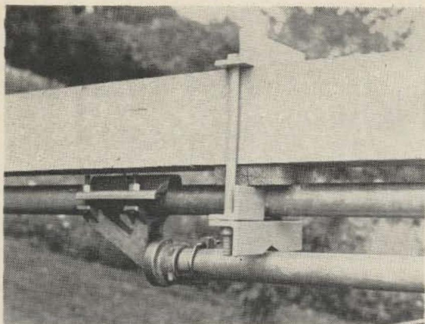
Fig. 5. Clamping arrangement detail.
