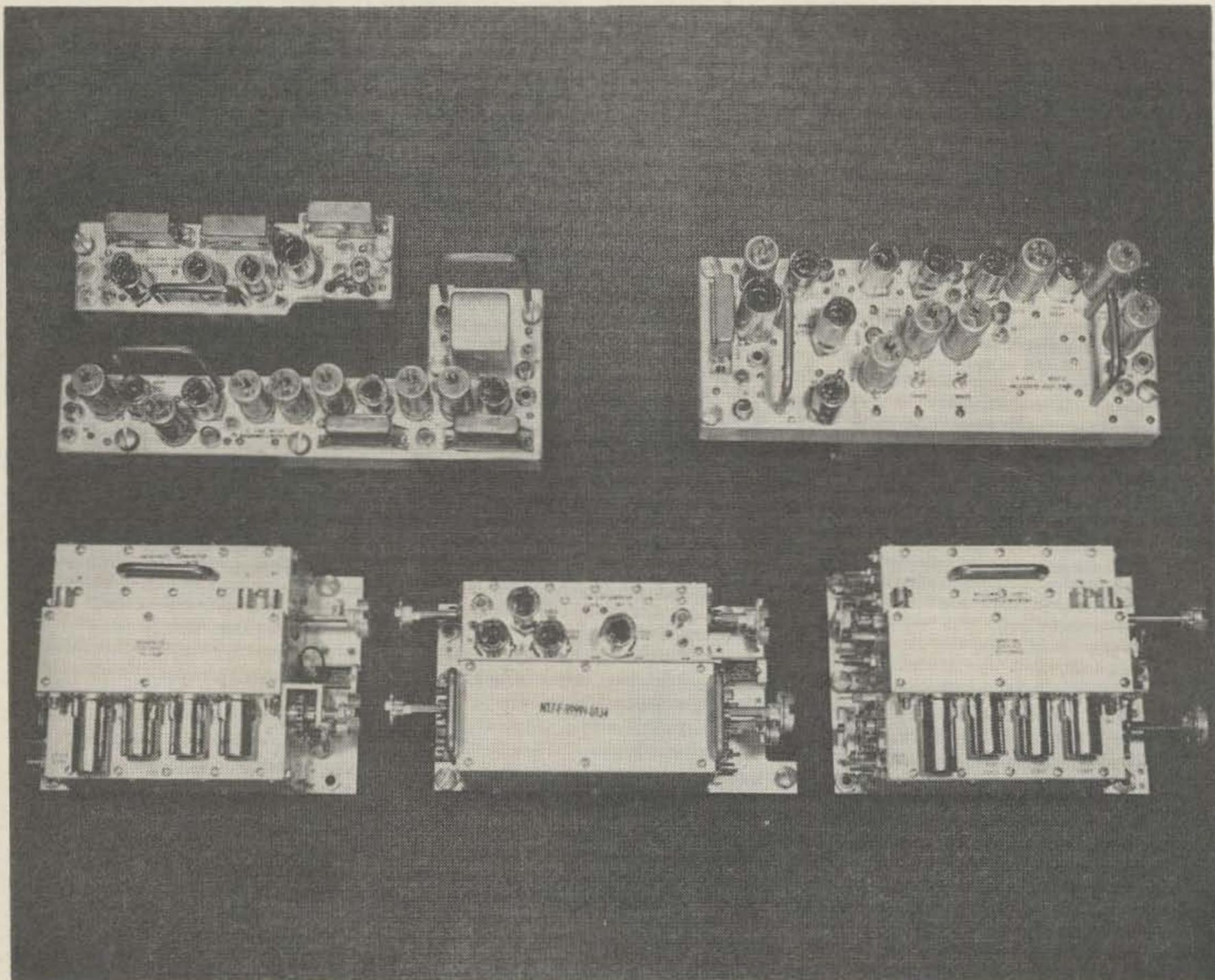
Available AN/SRT-14 sub-assemblies are shown above. They are, left to right and top to bottom, Frequency Converter Unit 11B, 1 mc Step Generator Unit 10, Frequency Converter Unit 9,
