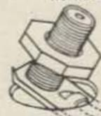
Mounts from outside by insertion through 7/8" hole.
