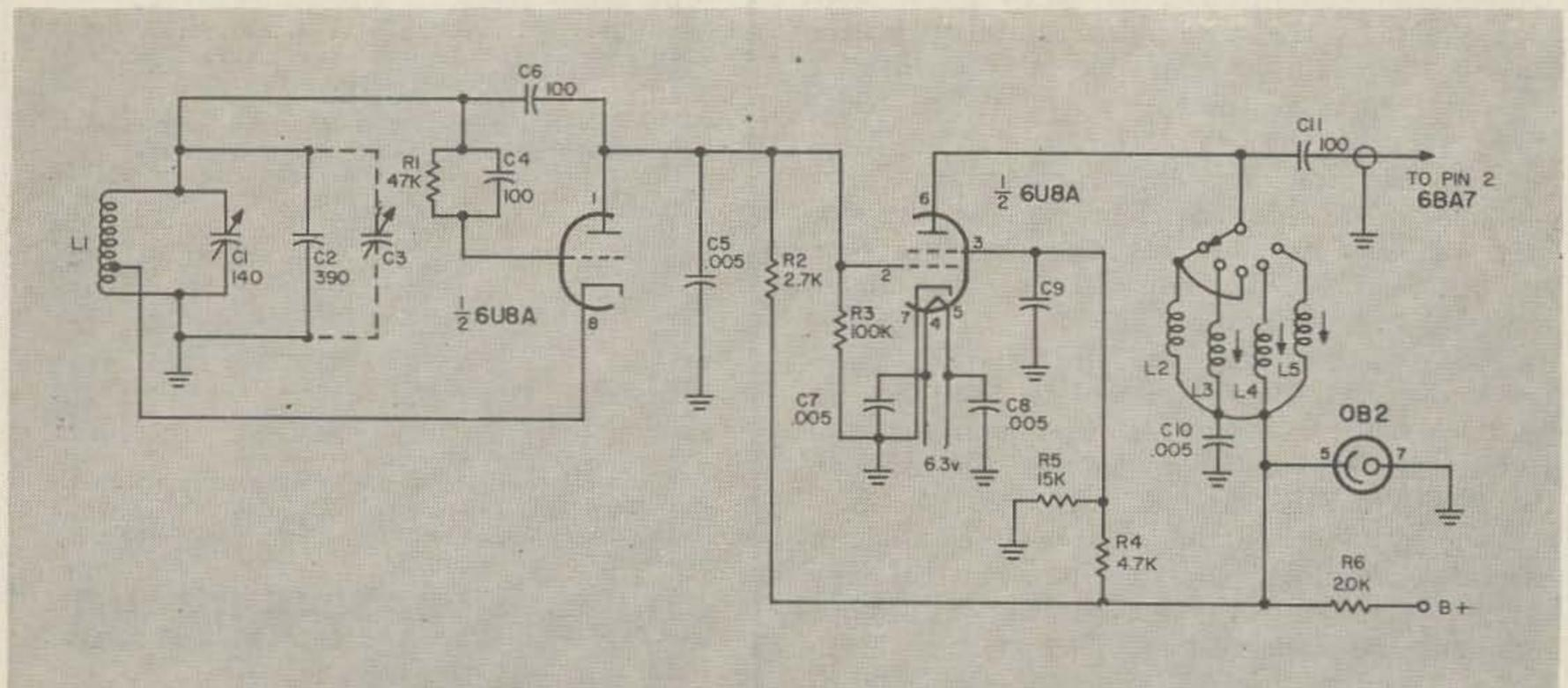
Fig. 2. Diagram for VFO and frequency multiplier for SSB exciter.
