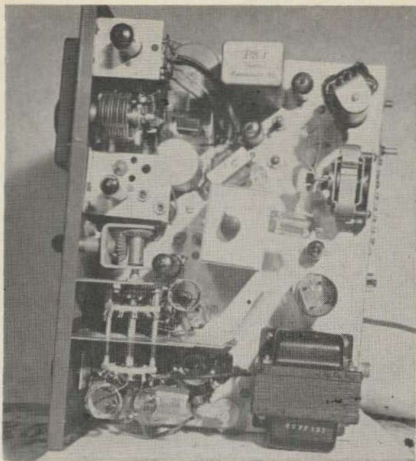
Top view gives bird's eye view of added band-switch, VFO and fan.
