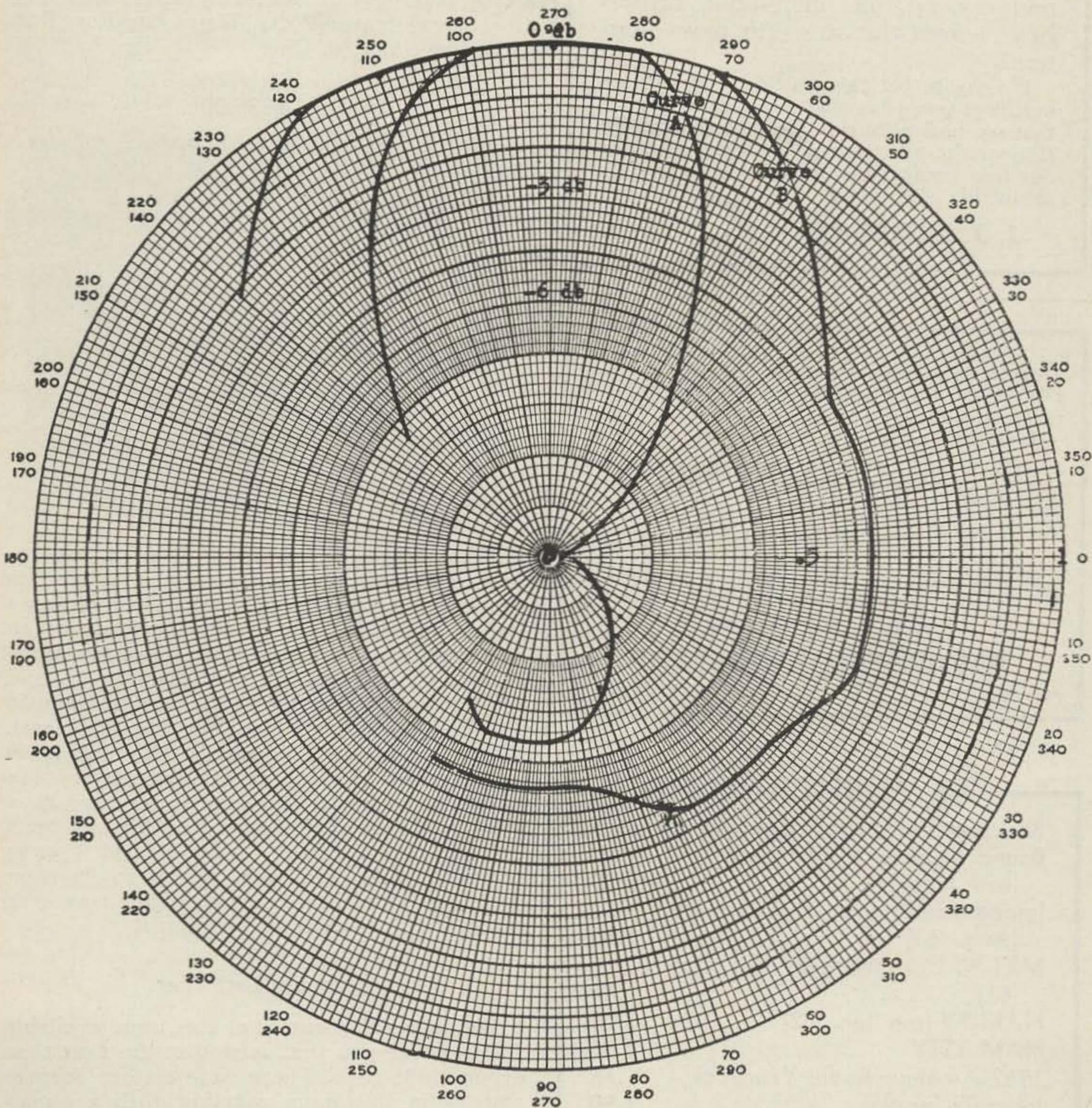
Curve A: Rotating 32 elements. Curve B: Rotating upper 16 elements, lower 16 elements fixed.
