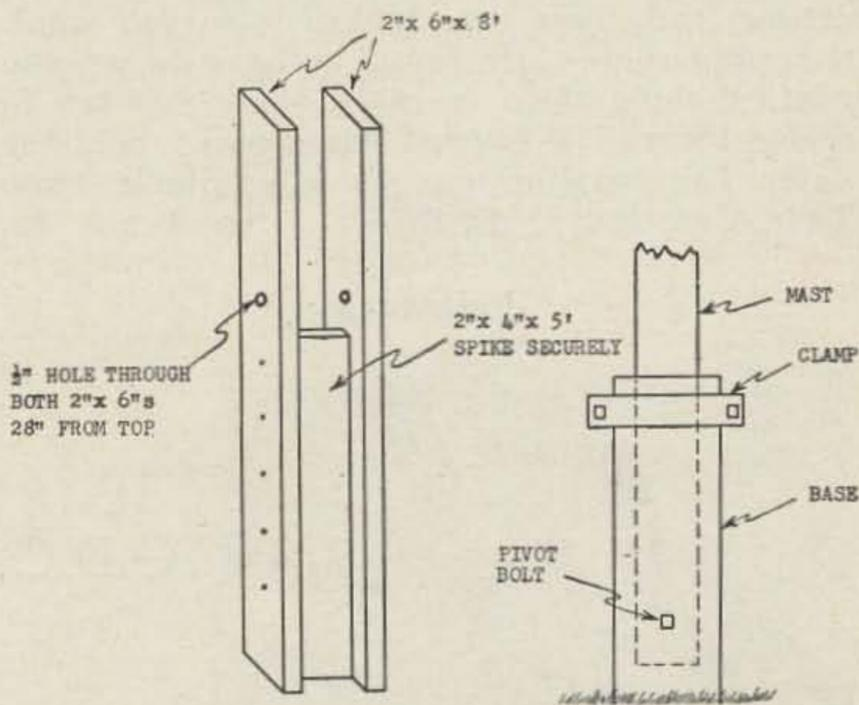
Fig. 3. Base. Fig. 4. Base clamp on base.
