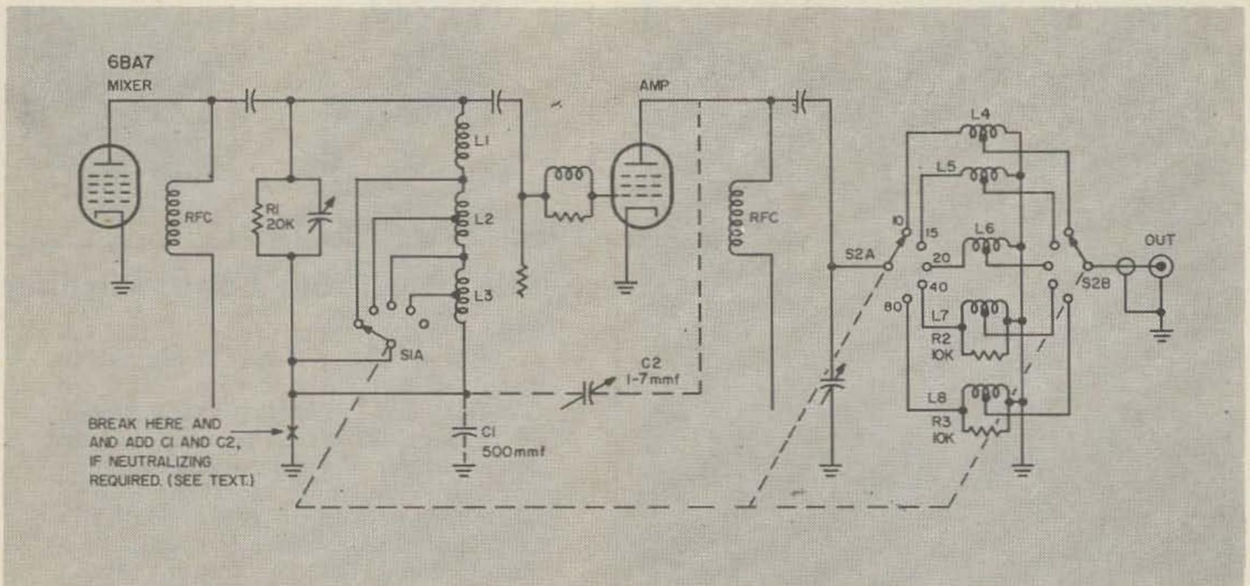
Fig. 1. 10A/10B mixer and amplifier tank circuits modified for bandswitching. Neutralizing circuit in dashed lines required only if 6AG7 amplifier is replaced with a 6146.
