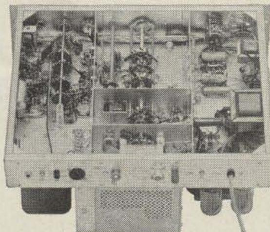
**BOTTOM VIEW**—Compartmental construction provides necessary isolation and shielding of transmitter sections for top performance. . . adds rigidity to the chassis for rugged, dependable service and long life. Neat circuit layout through careful design and a pre-cut, cabled wiring harness permit easy assembly.
