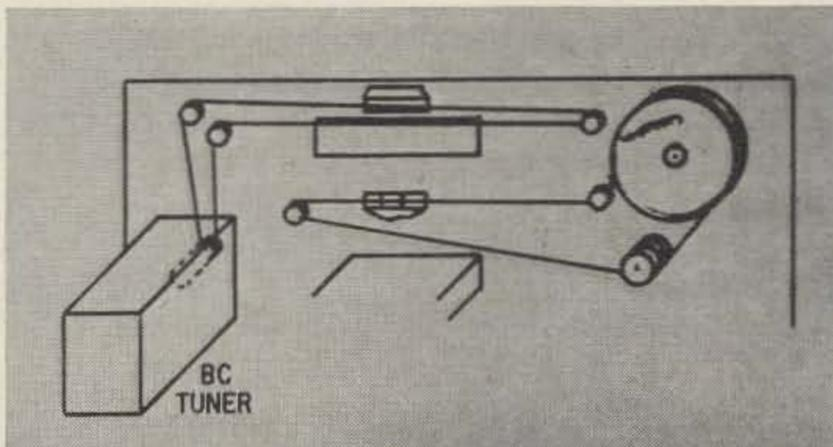
Dial cord stringing. The dial cord goes around the shaft in the BC tuner four times and then goes through a hole in the shaft and around the shaft again four times in the opposite direction. The knot in the cord is at the pointer clip.
