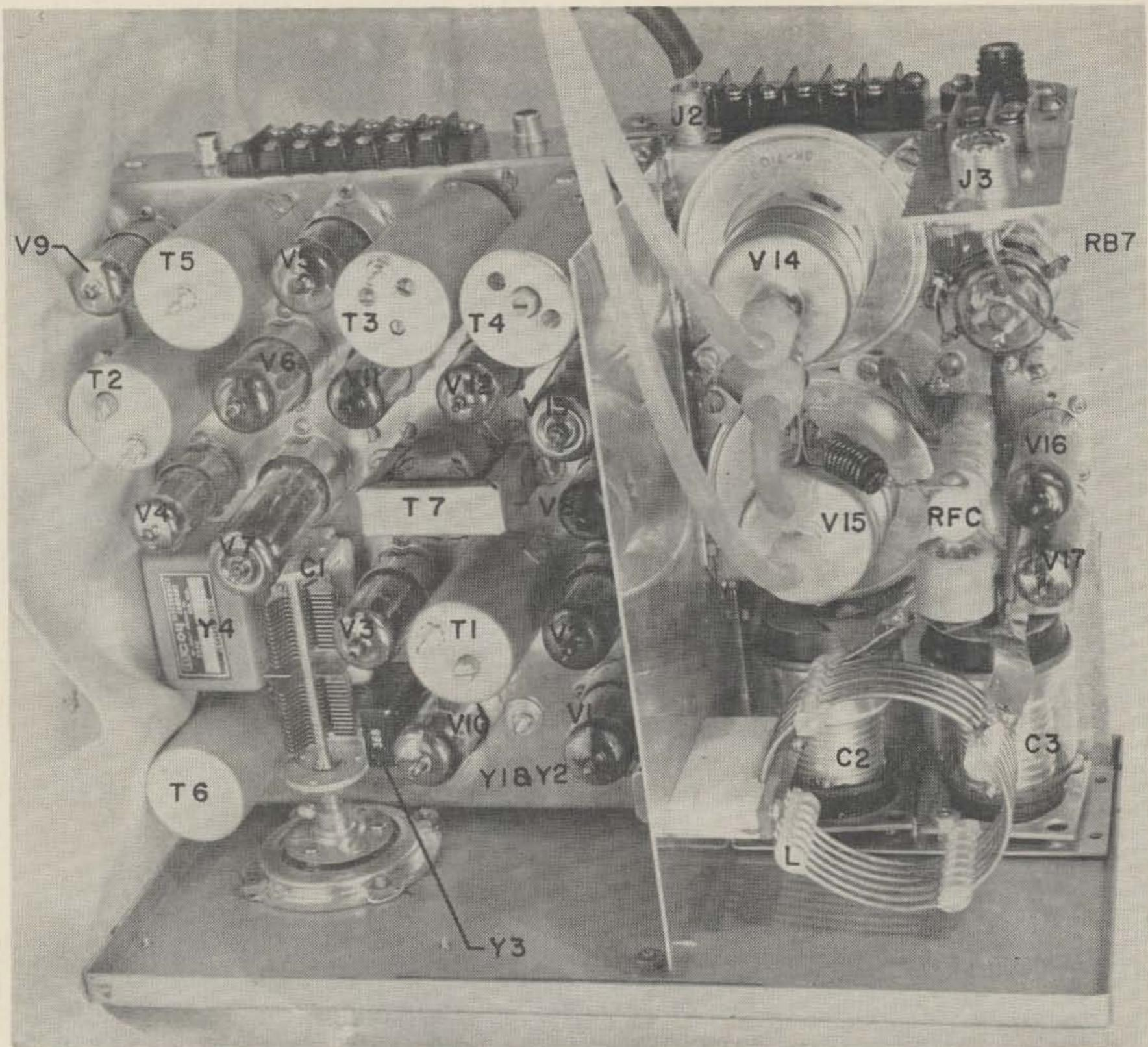
The high frequency oscillator is common to both transmitter and receiver. It is a "rubber crystal" circuit, good for 10 kc variation. The rubber crystal gives sufficient stability for mobile single side band work. The transceiver covers 30 kc in the 40 meter band.
