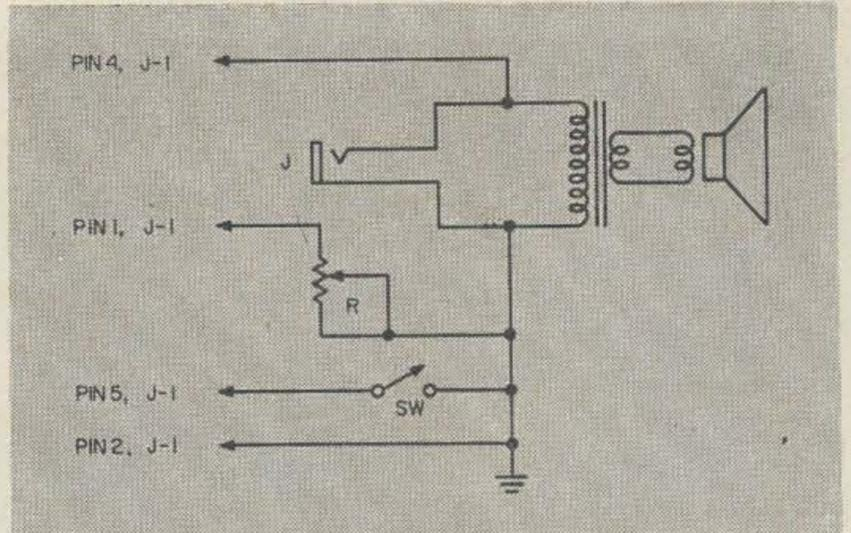
Fig. 2. Wiring for installation of 1 1/2" speaker in Command Set receiver local control filler panel.
