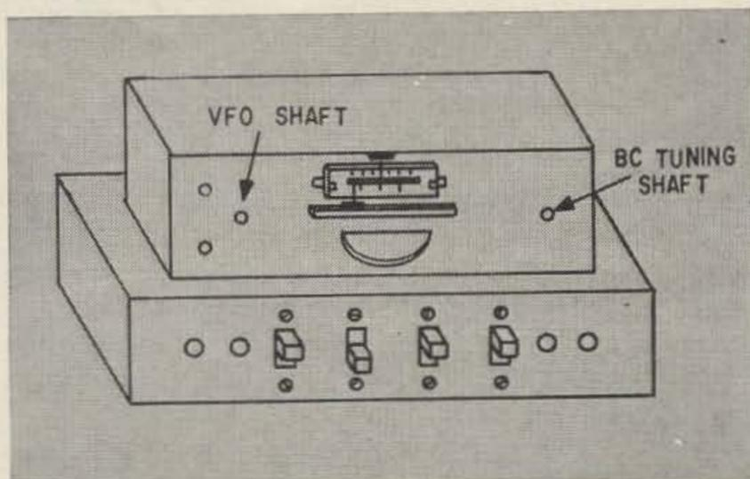
The sub-panel is recessed  $\frac{1}{4}$ " from the front or main panel, which attaches to the chassis via pot and switch nuts of various controls. The screws holding the slide switches are counter-sunk flat head type so as not to appear on the main panel. Sub-panel has hole cut behind dial for lighting. The top pointer (receiver) rides on the top edge of the sub-panel. The bottom pointer rides in a slot cut in the sub-panel above the meter opening.
