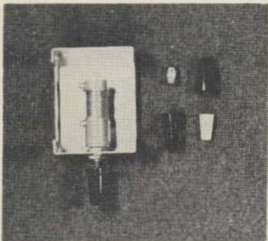
Electrical solderless connectors, of the insulated type, are a readily available source of attractive, functional control knobs. These insulated fittings are available in two general types and a wide range of sizes which make them ideal for use with those odd size control shafts.
