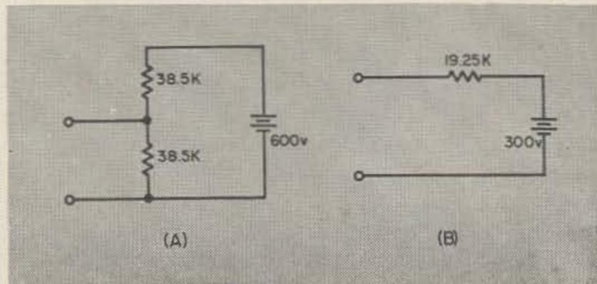
Fig. 2. A voltage divider and its Thevenin equivalent circuit.
