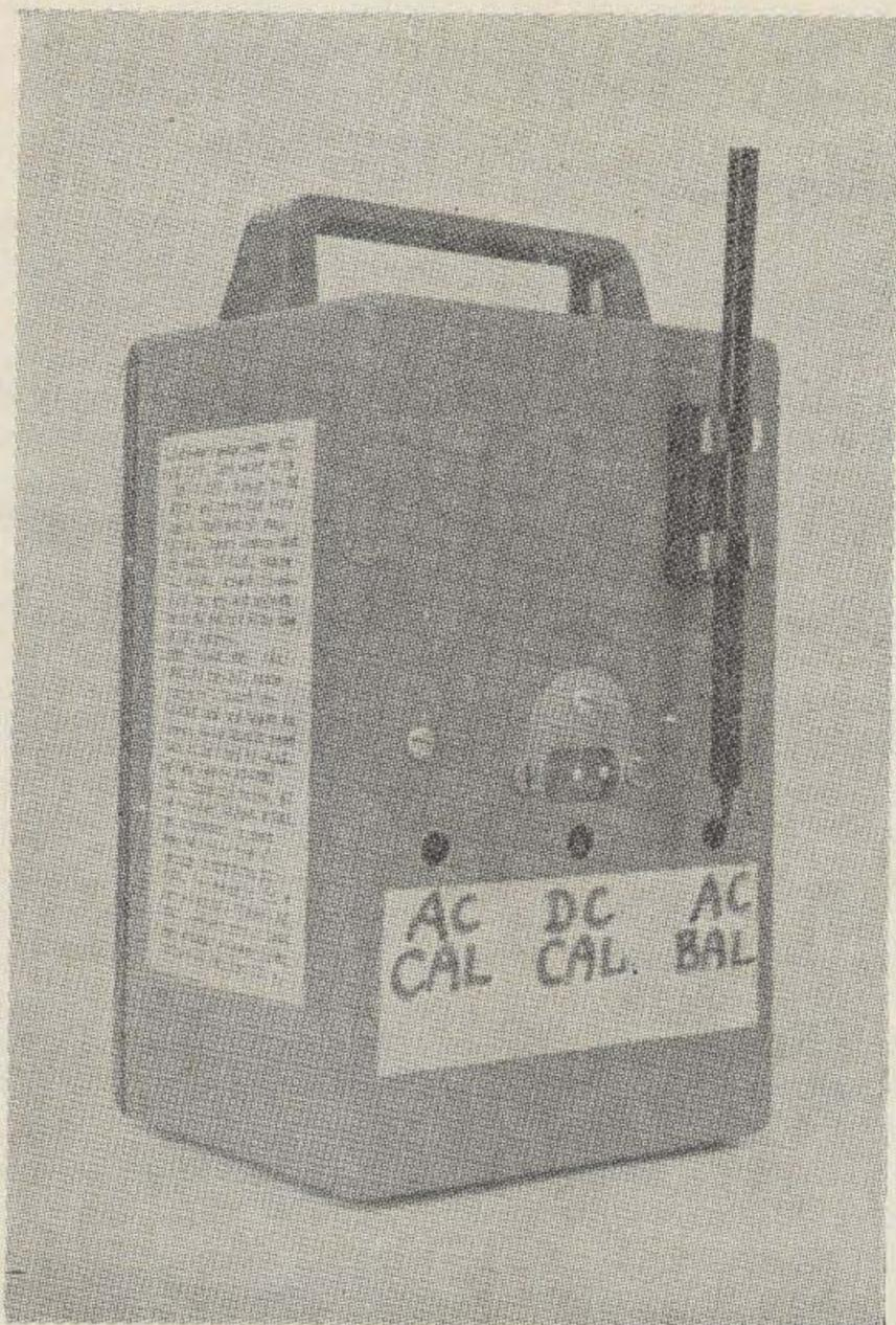
Step two is to make the calibration controls easily available without the bother of removing the case. Drill three holes, each a little more than  $\frac{1}{4}$  inch in diameter, in the back of the case. Carefully align the drilling marks so that the holes will be in line with the calibration pots. Press a wide strip of adhesive plastic tape (white) into place below the three holes. With an instant-drying marker pen, label the access holes according to function.
