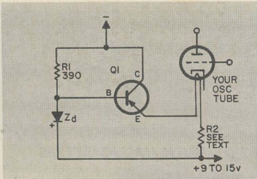
it). Target value is 6.5 to 6.6 volts, which would allow replacement of R2 with a wire. A lesser voltage will not allow 6.3 volts at the tube. A higher voltage will require use of R2 in the circuit.
