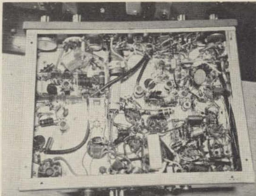
Underside of chassis. Looks like a rats nest, but isn't. Note VFO coil mounting on switch in upper left. Antenna relay space created by modulation transformer above chassis. A copper shield divides the chassis with transmitter rf on one side and receiver and modulator on the other. Shields are used between the oscillator and driver sockets, mounted across each socket.
