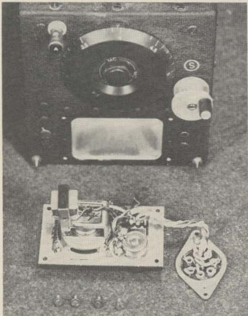
Seeing is believing. The blank control panel from the front of the receiver mounts the speaker, line matching transformer, phone jack, RF gain control and BFO switch.
