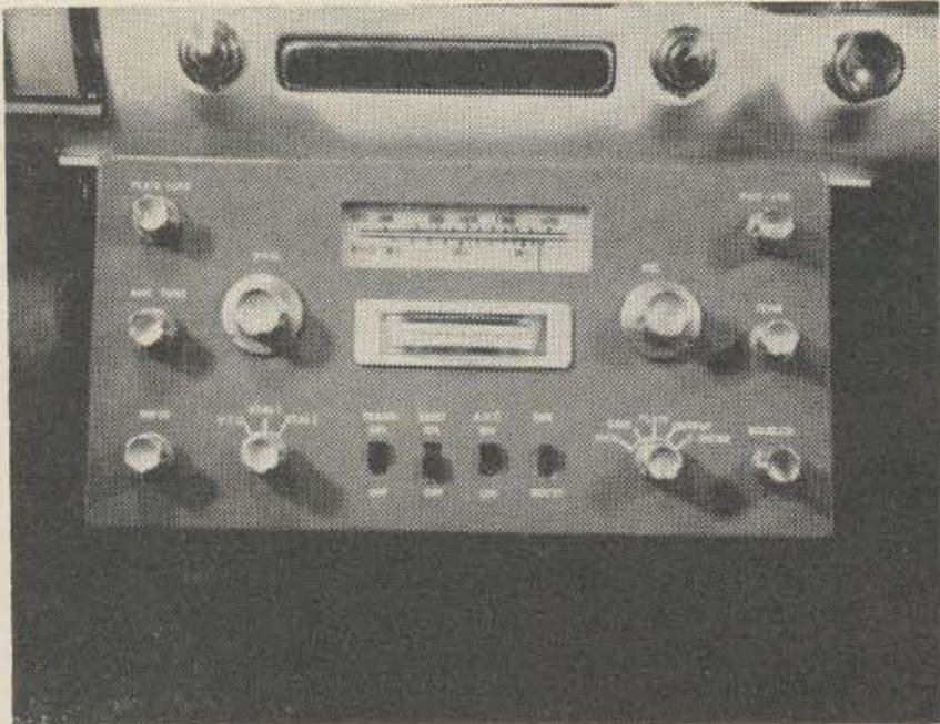
Rig is attached to underside of dash with bolts and heavy gauge aluminum angle.
