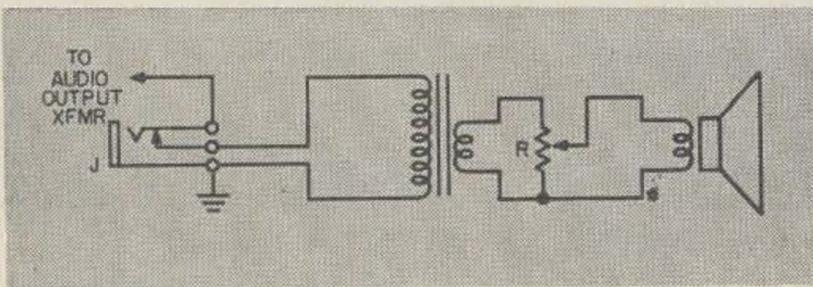
Fig 1. Revised wiring of the Lafayette SK-145 speaker for use with Command Set receivers.
