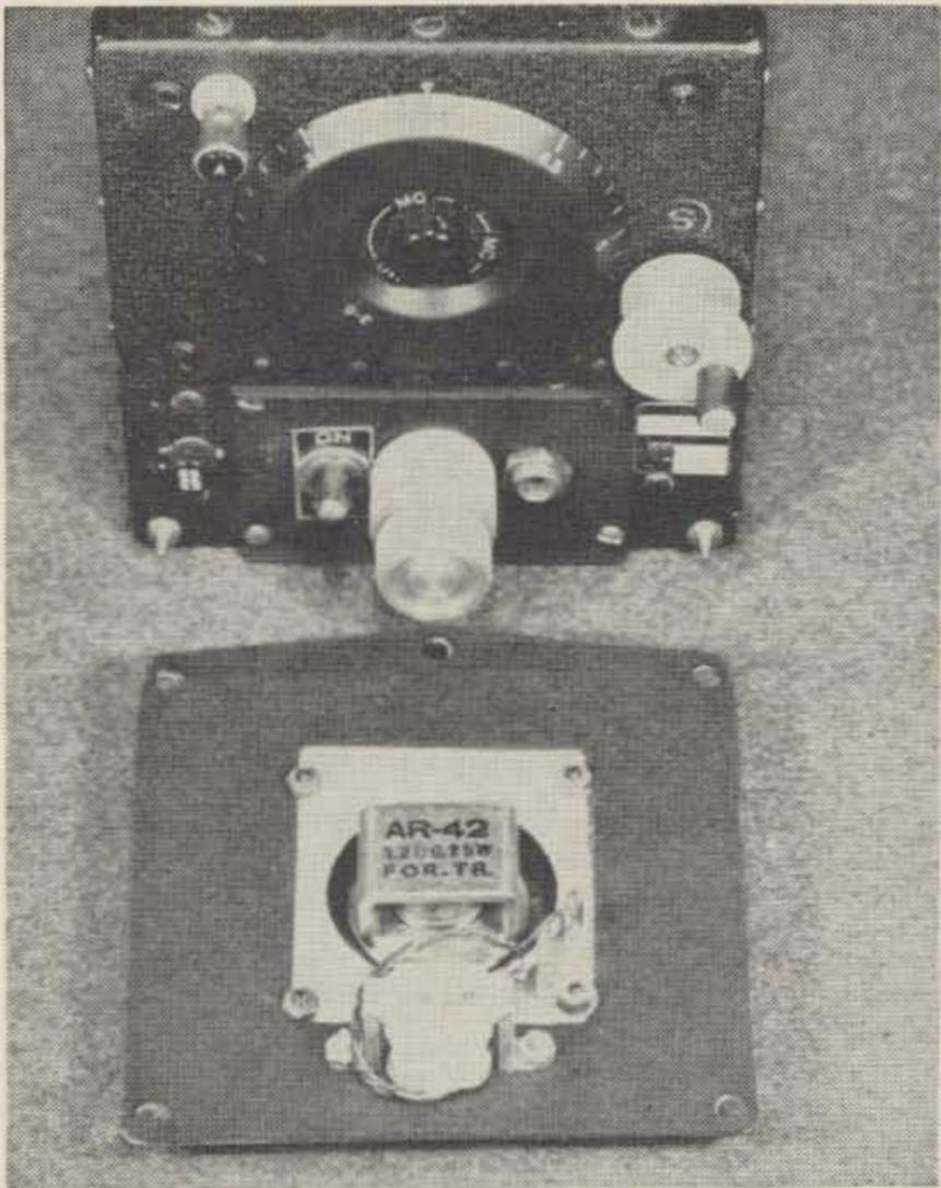
A 2 1/2" PM speaker and miniature line matching transformer fits on the tube access cover plate of the Command Set receiver. Speaker grill is the insert from a dime store, plastic flower pot.
