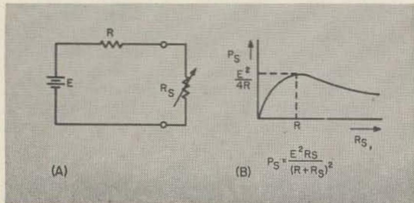
Fig. 1. Change in screen dissipation as the screen resistance varies.
