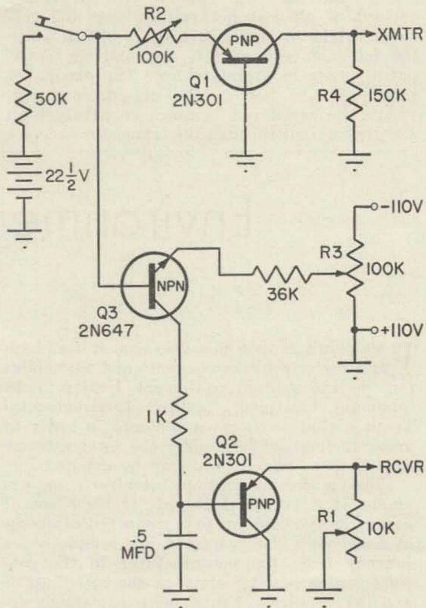
Fig. 4—DeLuxe transistor break-in circuit with blocking bias circuit for TR switch.
