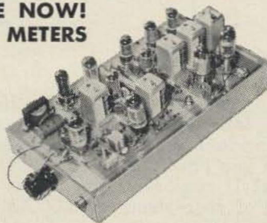
Originally described in the May, '61 issue of 73 Magazine (P. 57-58). This rugged filter type transceiver makes SSB available to all AT MODERATE COST. The Mark 2B is a single sideband transmitter and receiver delivering a conservative 2 watts output into a 50 ohm load. The basic unit is supplied on 40 or 80 meters, wired and tested. You may provide power supply, 455kc mechanical filter, tubes, carrier crystal and VFO or buy direct from us.
