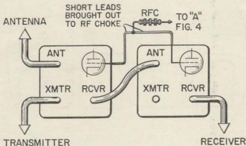
Fig. 5—Using two TR switches to increase isolation between transmitter and receiver.
