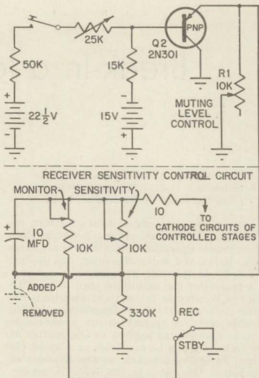
Fig. 2—Receiver muting with a transistor.
