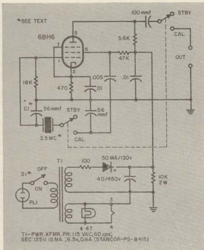
um at your shack, the on-off switch and the line plug can be eliminated and the ac line connected across the receiver's ac input so that the calibrator comes on whenever the receiver is turned on. A high density selenium rectifier was used and this contributes greatly to the compactness of the unit. The whole thing runs very cool and even after 24 hours operation, still isn't hot.
