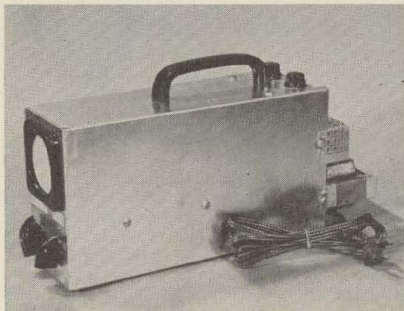
transformer. In general, this means six inches distance. Don't depend on a cabinet to "shield" the transformer, either. You may have to experiment a bit to see where it will work best. Turn the Simplescope on, get a fine spot on the face of the tube, and move the scope around, seeing where you can put it where, (A) you can see the tube face clearly without glare, and (B) where the spot is not moved by either 60 cycle or audio fields from transmitter or receiver.
