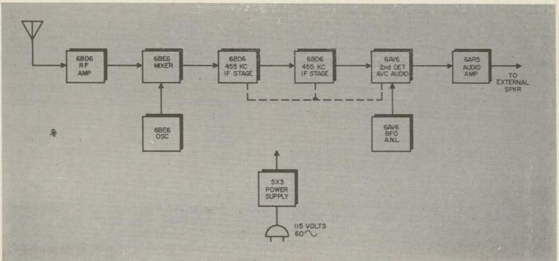
Figure 1. Block diagram of KT-200.
