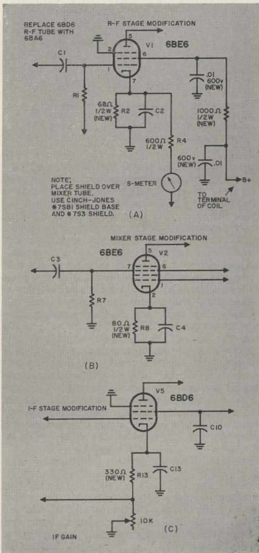
Figure 2. Circuit modifications for the KT-200 receiver.
