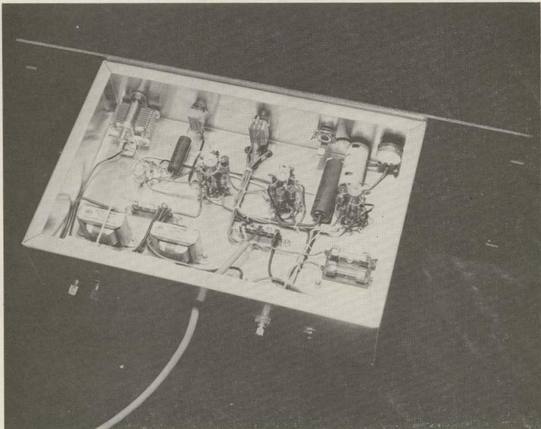
thermionic type is a bit more rugged. A bit of rf filtering and the detector output becomes the transmitter output envelope. This signal is fed right into the grid of the dc amplifier. No blocking capacitor is used nor needed.
