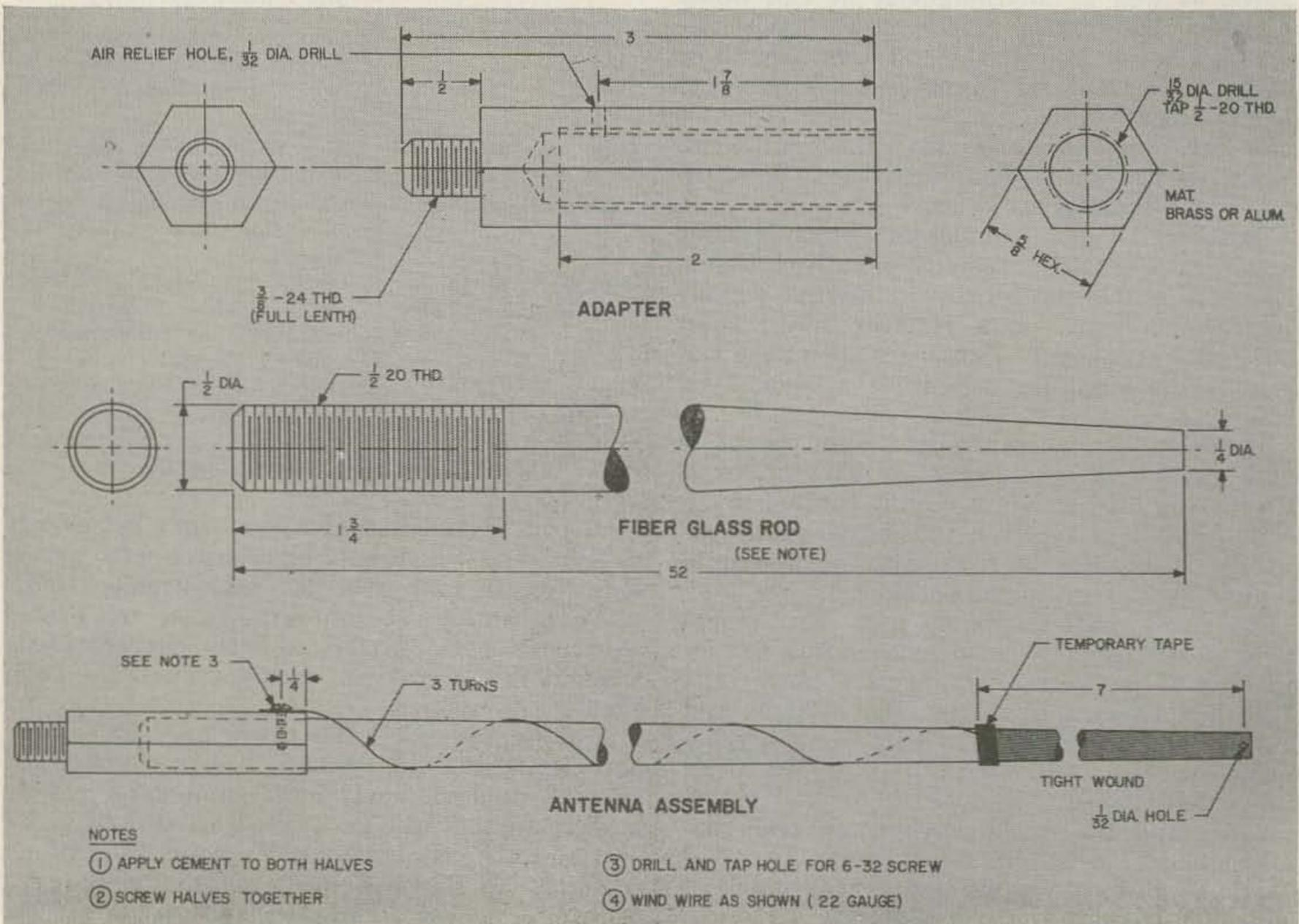
the desired frequency, it will be necessary to coat it with several protective layers of varnish or lacquer. Krylon or lacquer in pressurized cans is very convenient. After the first coat is dried the tape may be removed and the additional coats applied. Allow ample drying time between coats.
