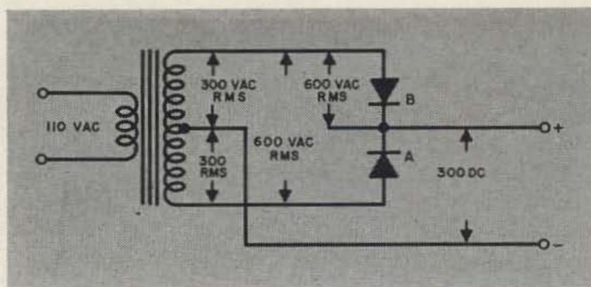
to change 750 volt supplies to 1500 volts for 811A's or 2000 volt supplies, at which voltage 4-250A's and 4-400A's are notoriously inefficient, to 4000 volts. The space saved by this application will readily strike the prospective user and make possible a conversion that may have not otherwise been considered feasible.
