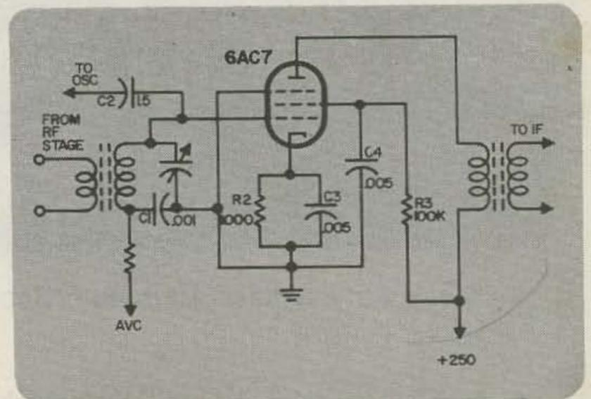
Fig. 6. The 6AC7 mixer circuit shown here gives lowest mixer-stage noise output of any frequency converters tested, according to research reports. Its major disadvantage is the extensive set surgery required for installation.
