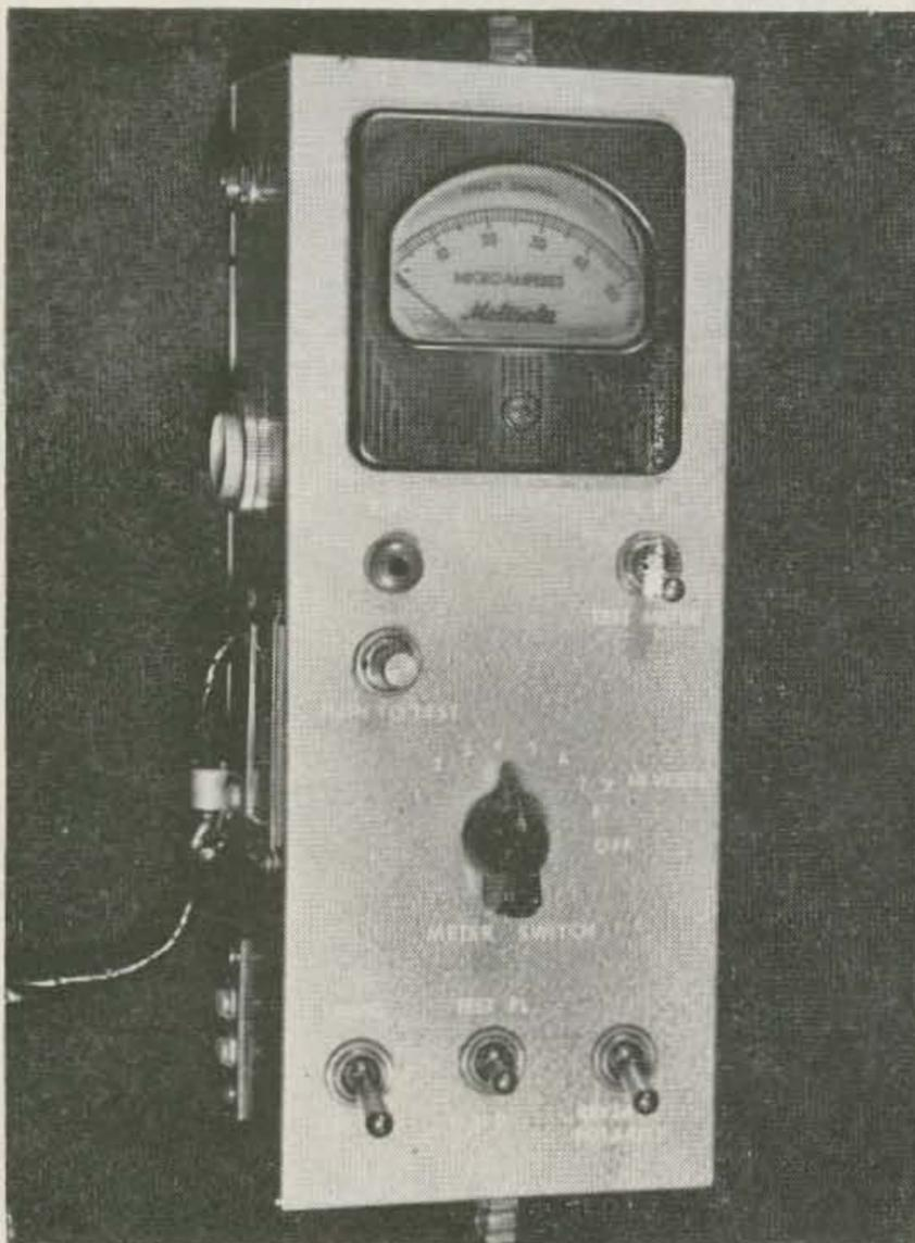
THE unit pictured is a handy gadget to have around on one's workbench while converting the popular FM two-way radio surplus equipment to the six and two meter amateur frequencies.
