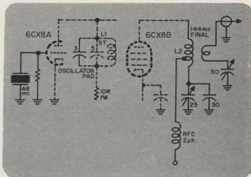
between turn 1 and 2 from the plate end of the final coil. Solder the 2 µh RFC choke 1 turn from the capacitor end.
