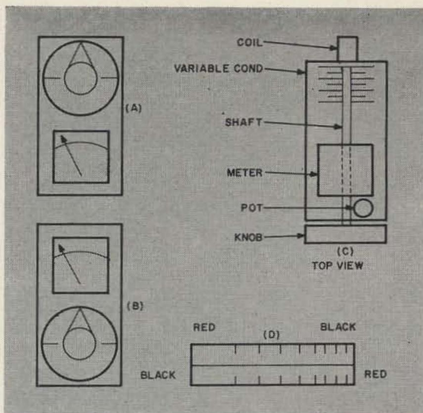
selves to only 2 pins we cannot use this approach and a potentiometer has been substituted for the fixed resistors. This produced a bonus in that it is possible to set the pot for relatively weak oscillations. Under such conditions the meter will give a good dip with very loose coupling to the tuned circuit.
