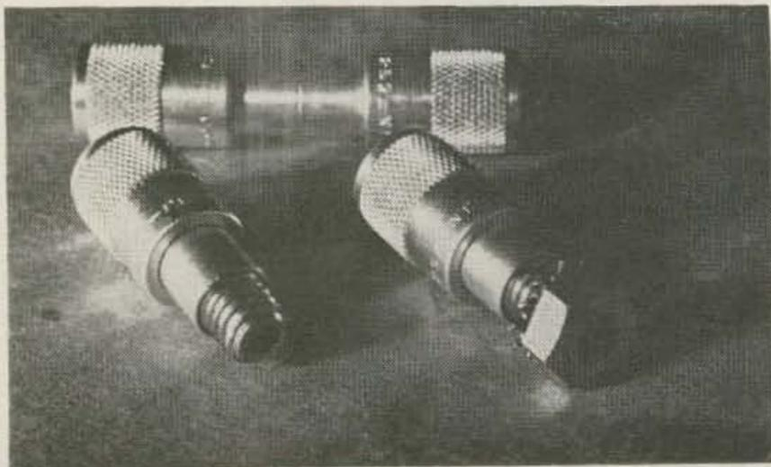
PL-259 plugs on a chassis by using a standard National Coarse thread cap screw. A hex head, 7/16-14 brass bolt, about 1/2" long, is ideal for this purpose since the threads mate perfectly with the cable retaining threads in the plug body. A clearance hole for the connecting lead, up to 5/16" in diameter, should be drilled the length of the bolt. A lock washer should be used for secure mounting.
