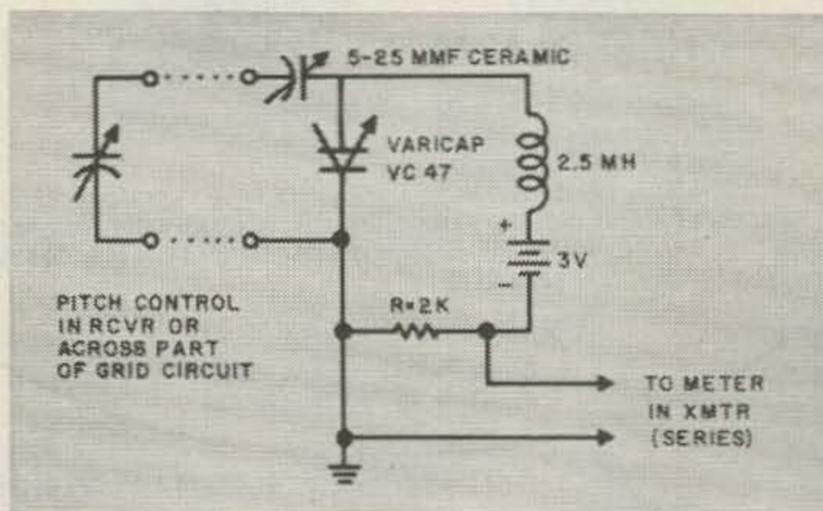
the current the higher the pitch will be. Tune for maximum pitch which will be maximum grid current. Now turn switch to amplifier plate and tune for minimum pitch. Minimum pitch will indicate minimum plate current.
