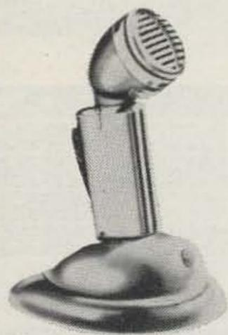
Here is a mike that is designed specially for SSB ops. It has sharp cutoff below 300 cps and above 3000 cps, making it ideal for ham communications. It is rugged, being of magnetic design, and won't boil away in the sun or dissolve when it rains. Output is -52.5 db at 100,000 ohms. For \$28.50 the Model 440SL comes complete with grip-to-talk switch, mike stand and cable. Same deal, marked Model 440, less stand, switch and mike connector is only \$15!
