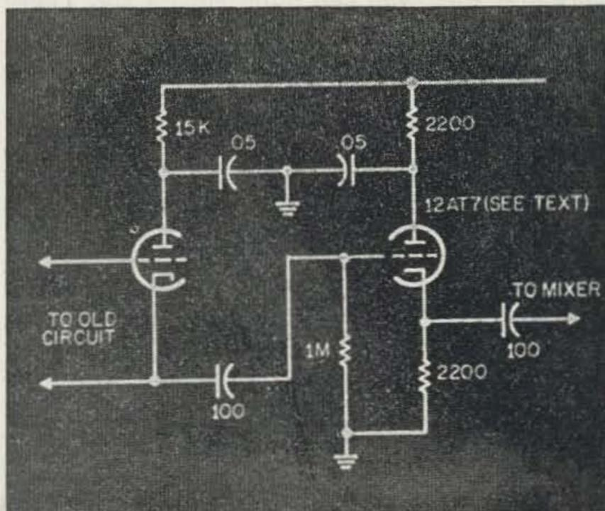
Fig. 1—This circuit, substituted for your receiver's present oscillator stage, will substantially reduce frequency drift. Parts values are non-critical, but lead dress must be direct and short. Use of a Vector 6-N-6T socket or an Amphenol type 59-369 socket will simplify wiring and installation of the stage.
