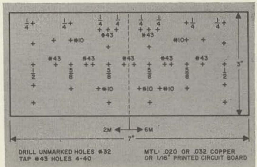
The printed circuit board is considerably easier to solder to than is the copper sheet. Now mount all parts, and wire. The small color coded wires removed from 8-wire TV rotor cable are ideal for the hookup and the coil links. If only one converter is to be built simply split the chassis layout down the center. Except for the extra hole for C9 the 6&2 layouts are identical.
