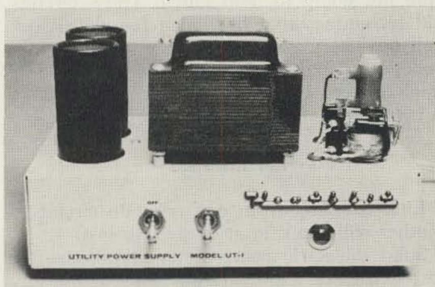
Power supply showing relay installed and extra (transmit) switch.
