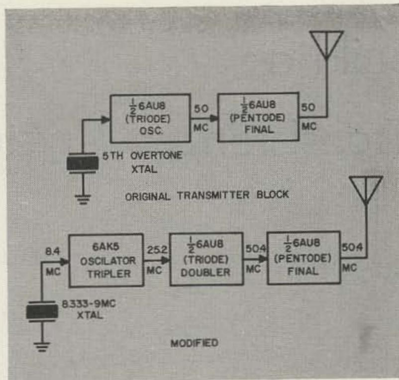
Block diagram of transmitter before and after modification.
