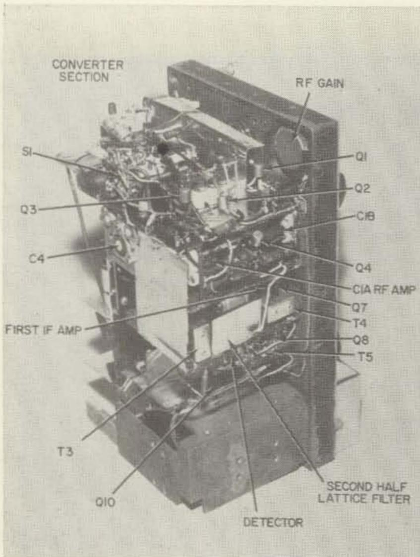
tor (at 480 kc) to the base of the 2nd mixer. Connect a voltmeter across the diode load (10K) and adjust the *if* transformers for maximum gain (keep reducing the signal so that the diode voltage reads less than one volt. Insert the crystals and repeak the transformers on each side of the filter for the strongest signal, consistent with flat response.
