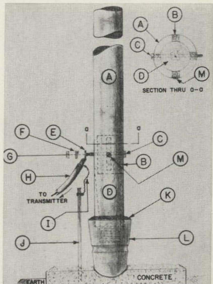
conformity with your calculations. Remember to measure from the point of feeder connection at the base ("C" in Fig. 2) to what will be the top of the mast.
