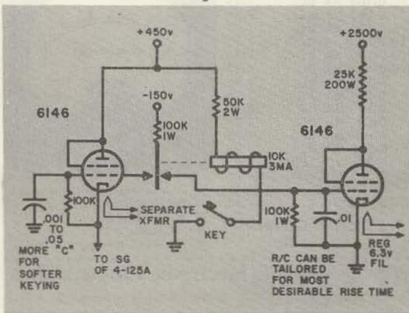
bleeder clamp tube. Under "key-up" conditions the bias cuts off the keyer tube. Under "key-down" conditions bias is shifted from the keyer tube, allowing it to conduct, and is put on the grid of the bleeder clamp tube cutting off the current in the bleeder. A small plate relay, single pole, double throw, is used to do the keying and steals a few mills from the low voltage power supply.
