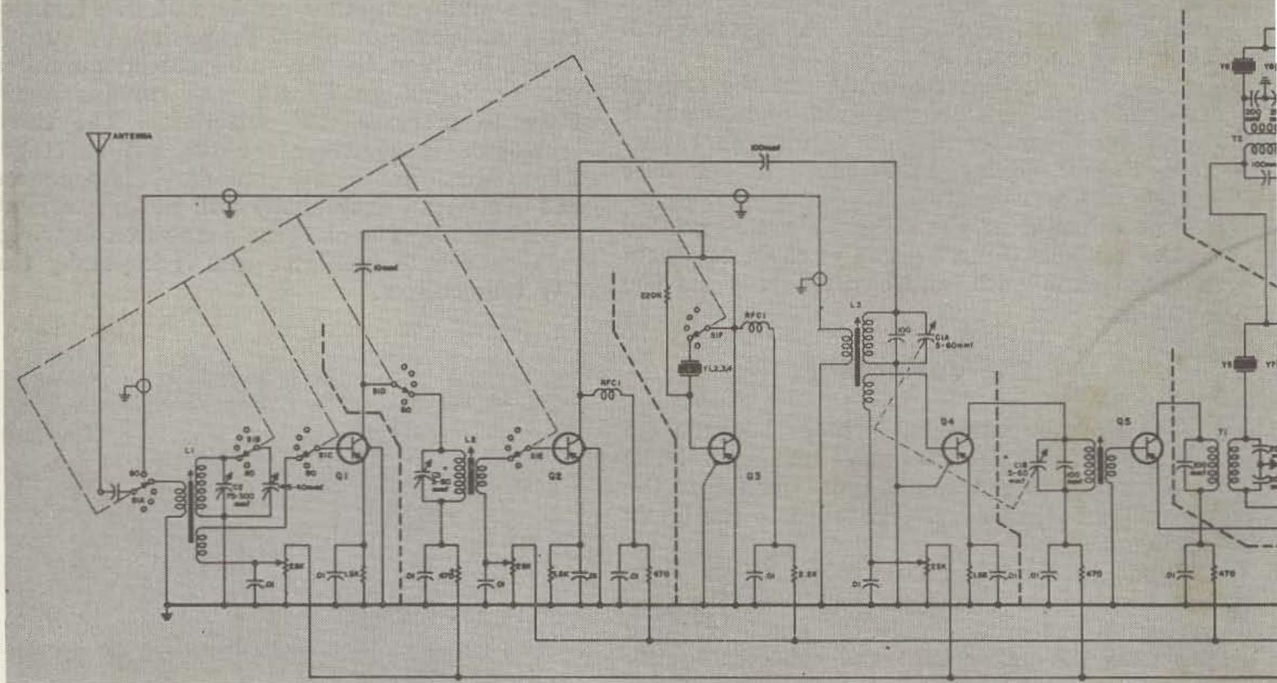
Fig. 1—Schematic diagram for the transistorized receiver. All 0.01 capacitors are
