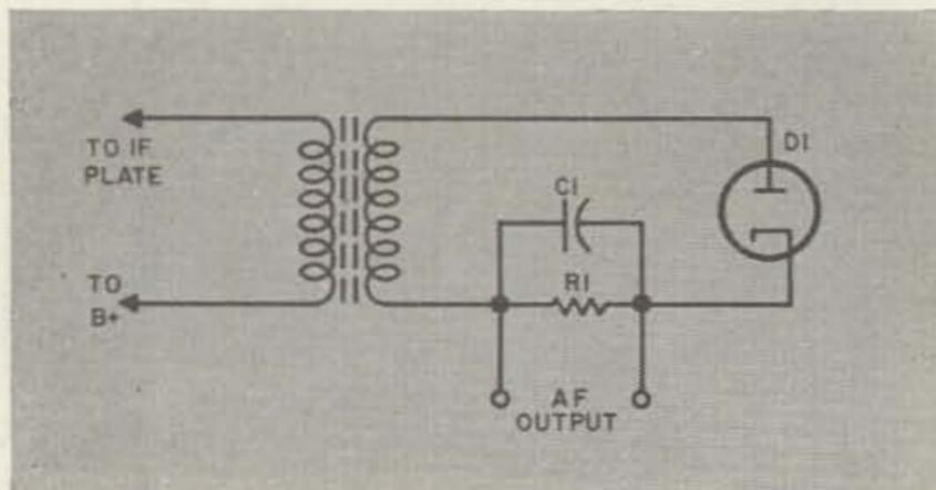
voltage output varies with the square of input voltage rather than varying linearly. Square-law detectors produce excessive distortion of AM signals, but are useful as mixers.
