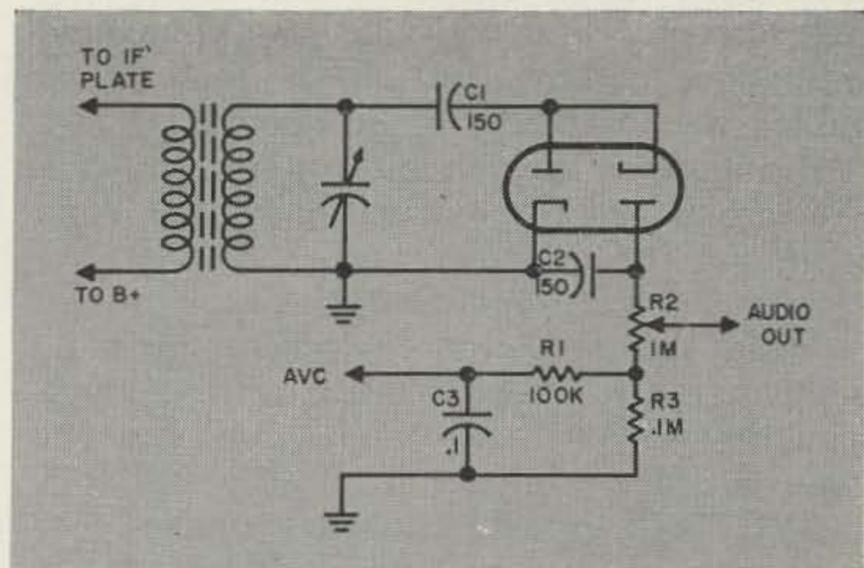
Fig. 2. The diode integrator, sometimes called a peak-to-peak detector, provides a virtually open-circuit load to the *if* transformer secondary. All distortion resulting from asymmetrical transformer loading is thereby eliminated, and detector efficiency is increased.
