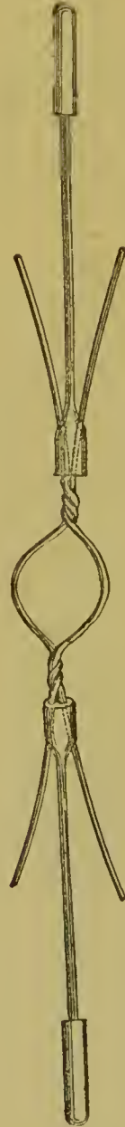
FIG. 15. DEFAYS' WIRE EXTRACTOR WITH THE TORSION RODS
