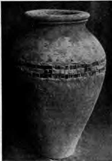
FIG. 49—CONCRETE VASE, MODELED DIRECTLY IN CONCRETE BY MEANS OF TEMPLATES
