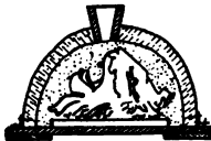
FIG. 52—SECTION VIEW TO SHOW THE USE OF A PLASTER SHELL, TO BE PLACED OVER MODEL AND FILLED AROUND MODEL WITH GELATIN FOR MOLD
