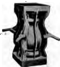
FIG. 82—STOCK MOLD OF IRON FOR BALUSTER
