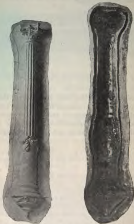
FIG. 53—PLASTER MODEL AND SHELL TO COVER IT WHILE SPACE BETWEEN IS FILLED WITH GELATIN
