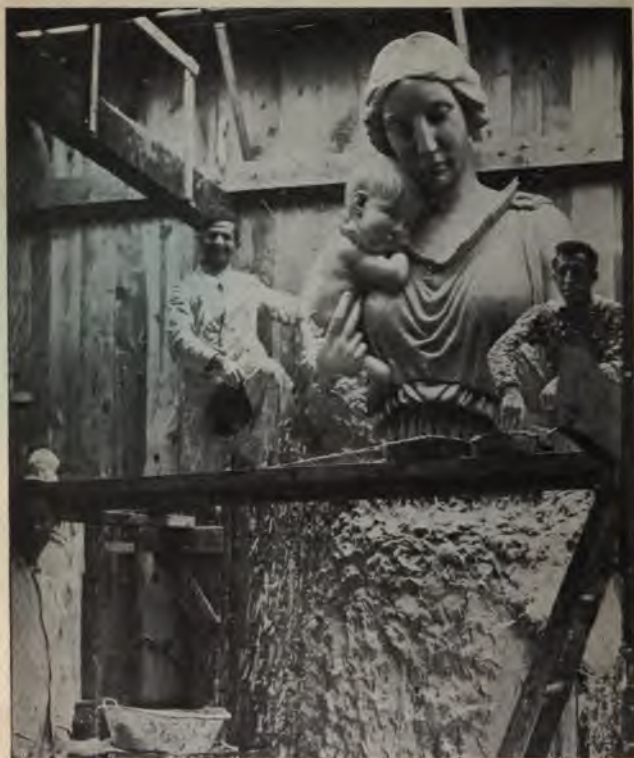
FIG. 44—COVERING CLAY MODEL WITH PLASTER, WORKING FROM BOTTOM UP—MOLD STANDS IN PIT AND FULL HEIGHT IS NOT EVIDENT
