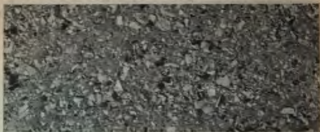
FIG. 68—BLOCK SPRAYED WHEN FIRST MADE AND BRUSHED A FEW HOURS LATER—FACING OF MICA SPAR CRYSTALS—R. F. HAVLIK
