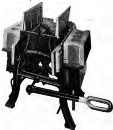
FIG. 18—DOUBLE-SIDED FACE-DOWN BLOCK MACHINE Cores are withdrawn downward after block has been turned over
