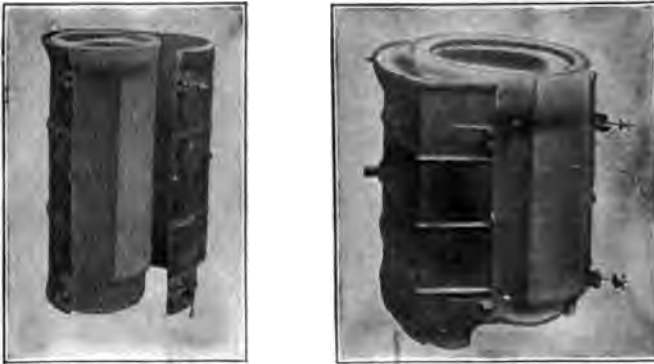
Fig. 475.—Showing Manner of Stripping Shell from Pipe.
