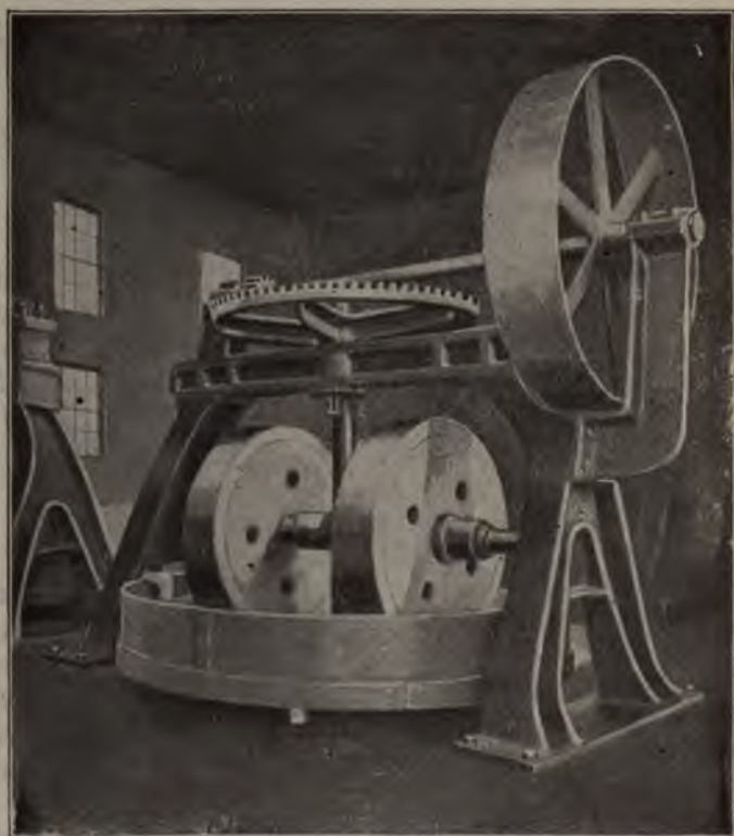
Fig. 10.—Mixing Pan for Marl and Clay. Edge Runner Type.
