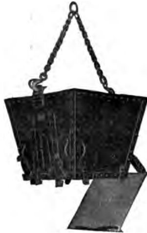
Fig. 49.—Cyclopean Bottom-Dumping Bucket.
