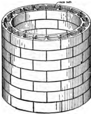
Fig. 705.—Two-Piece Blocks Used for a Circular Stack.
