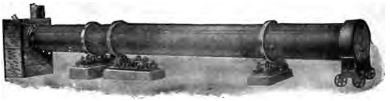
Fig. 9.—Rotary Kiln as Made by the Bonnot Co.
