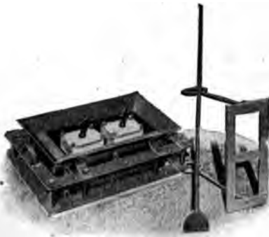
Fig. 711.—Pettyjohn Machine Ready for Depositing the Concrete.
