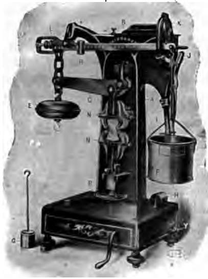
Fig. 13.—Improved Form of Fairbanks Testing Machine.
