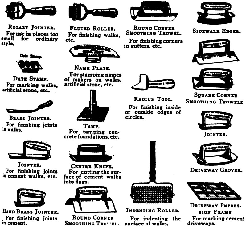
Fig. 60.—Tools Used in Finishing Cement Surfaces.
