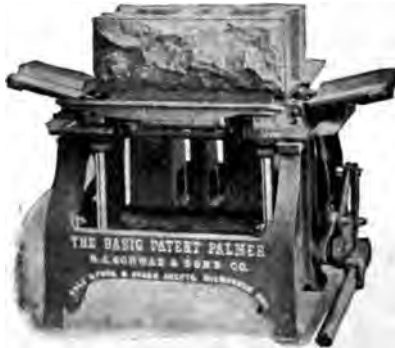
Fig. 708.—Palmer Block Machine Ready for Removing Block.
