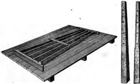
Fig. 563.—Mould for Fence Posts, with Four Tapering Sides.
