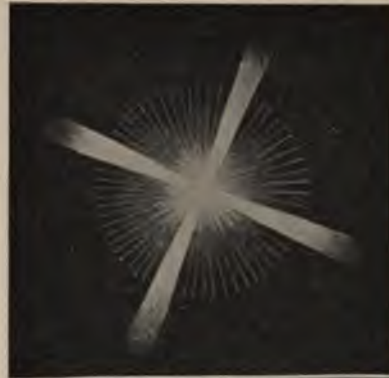
Figs. 238. — Fixed and Flashing Light. 4 flashing panels of 45° each; 4 fixed panels of 45° each.
