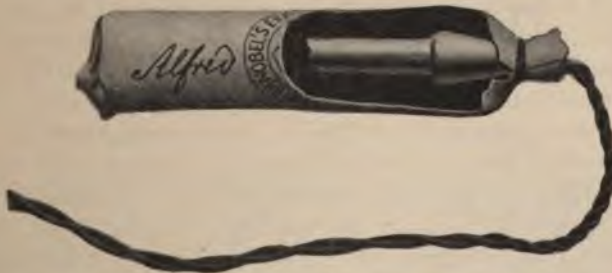
FIG. 79.—Electric Detonator Fuse inserted in Cartridge.
