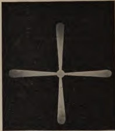
Figs. 241.—Single Flashing Light, 4 panels of 90°.
