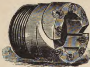
FIG. 74.—Core-bit or Cutting Edge of Rotary Drill, set with Diamonds.
